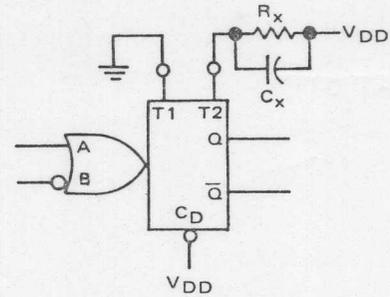
FIGURE 12 — Elimination of Power-Up Pulse Width
