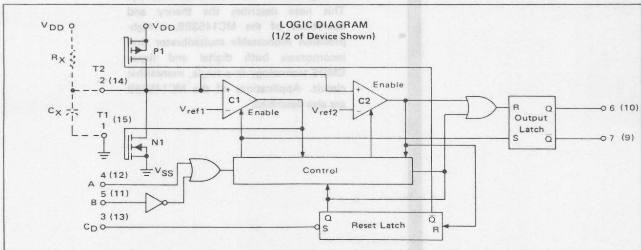
FIGURE 1 - Block Diagram of the MC14538B
