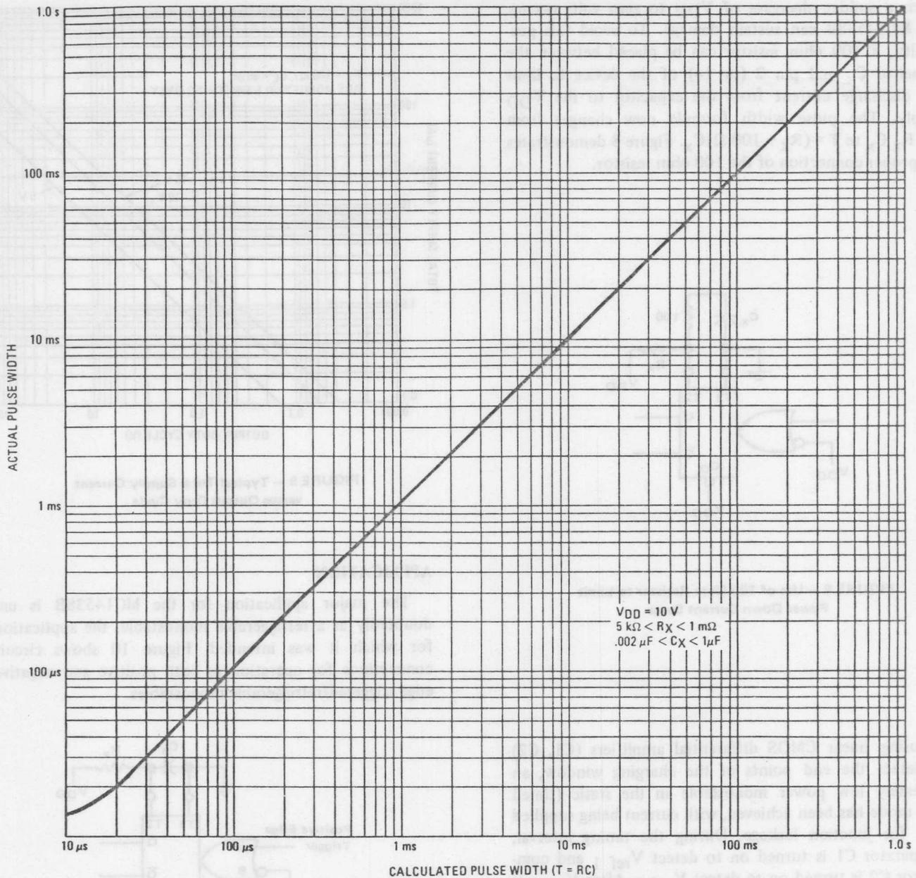
FIGURE 7 – Typical Pulse Width versus  $T = RC$
