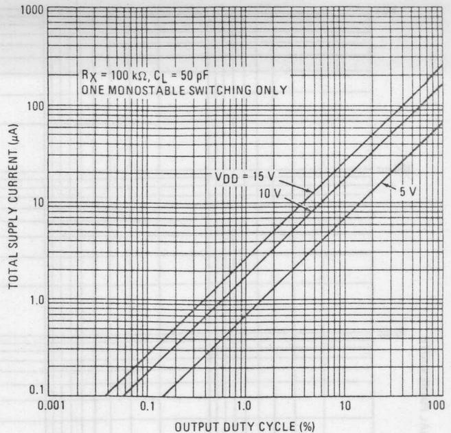
FIGURE 9 — Typical Total Supply Current versus Output Duty Cycle
