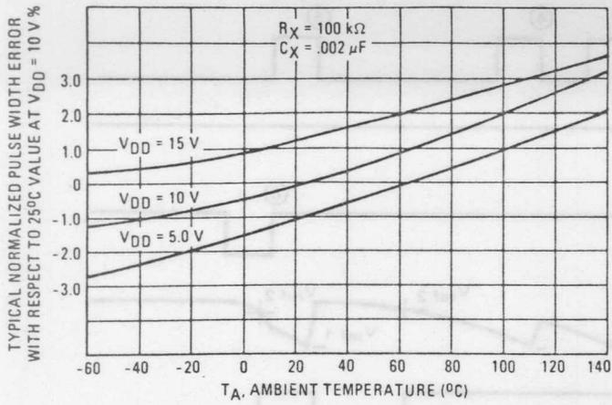
FIGURE 5 – Typical Pulse Width Error versus Temperature
