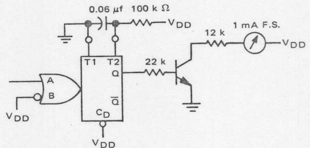
FIGURE 13 — Precision Analog Tachometer
