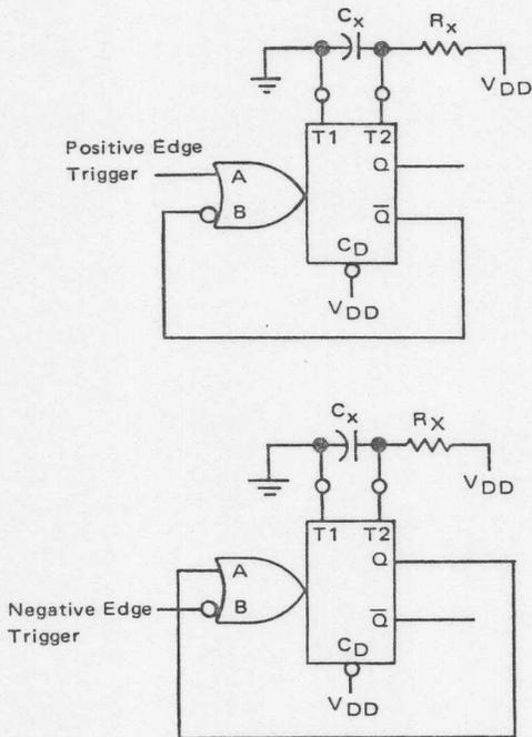
FIGURE 11 — Non-retriggerable Monostables Circuitry
