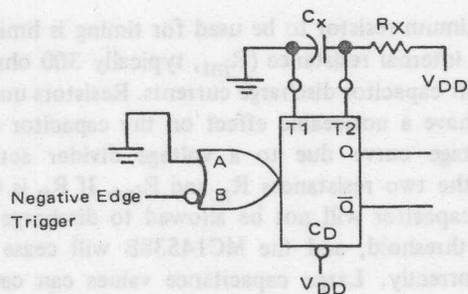
FIGURE 10 — Retriggerable Monostables Circuitry
