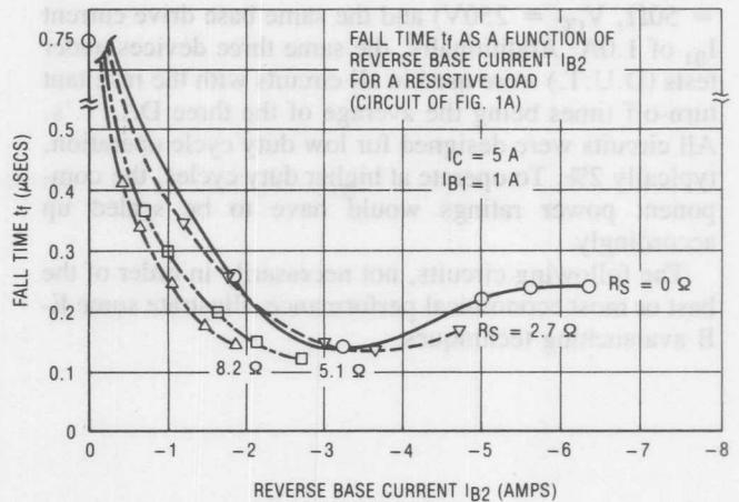
2. Collector current fall-time decreases with increasing off-bias until transistor action ceases ( $I_{B2} \approx I_C$ ) and increases thereafter.
