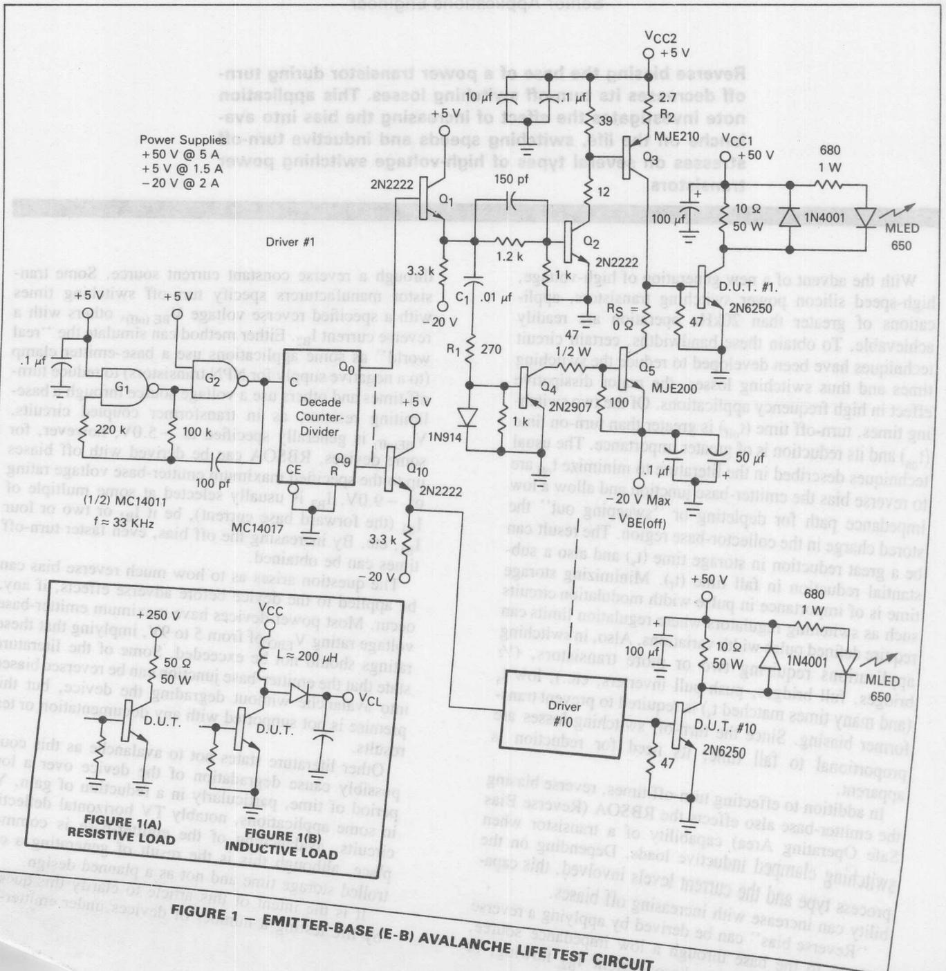
Eight of the ten devices were emitter-base (E-B) avalanched with the listed reverse bias; the two remaining transistors were not biased and were used as a parameter standard. Additionally, another transistor was used as a measurement standard, never being powered, but always remeasured when the test devices were measured. This ensured measurement repeatability. For all tests,  $h_{FE}$  (and the other parameters) were remeasured after 1 day, 1 week, 3 weeks, 6 weeks, etc.
