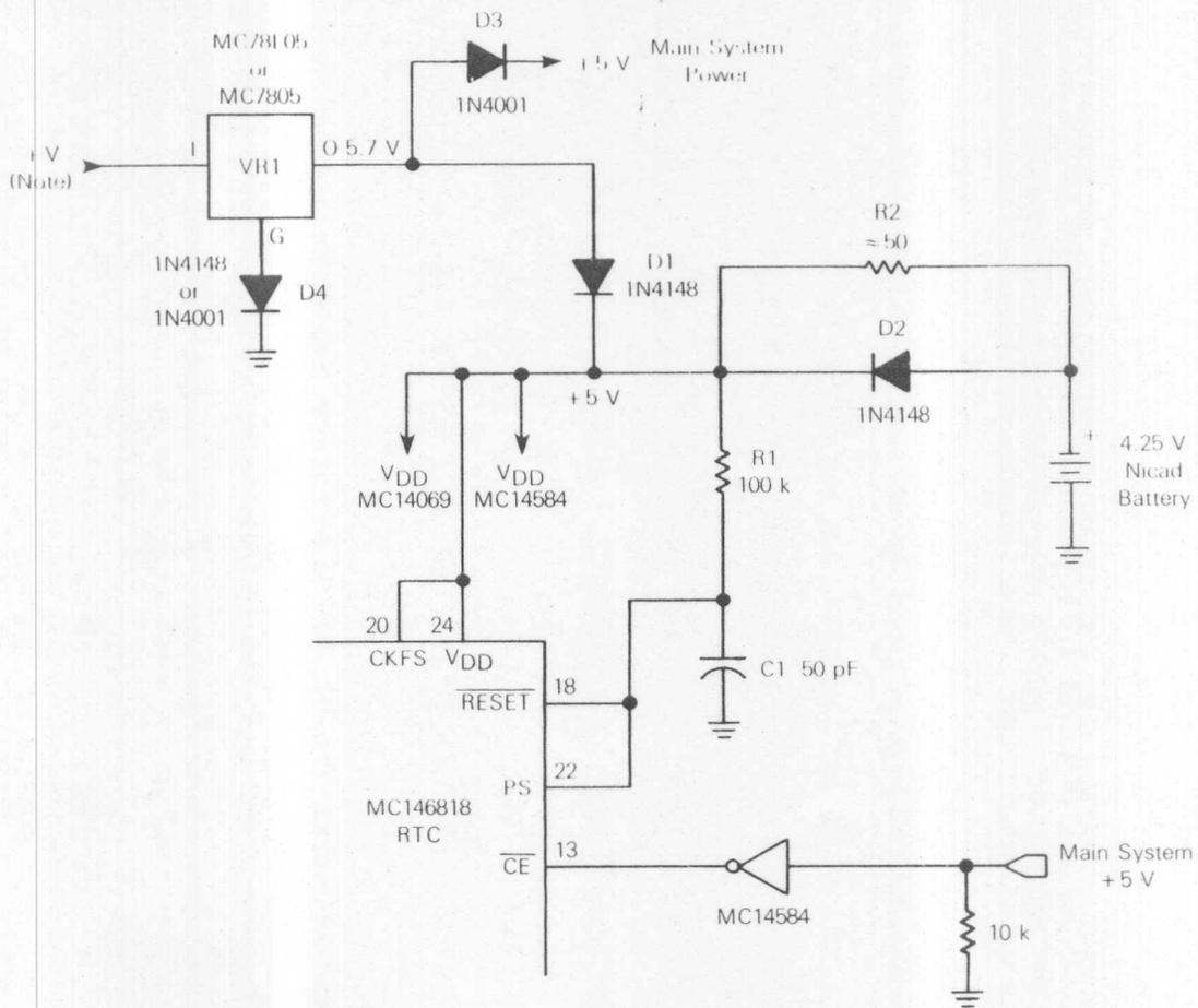
NOTE: Input voltage to VR1 should be more than +8 V but less than the rated input of VR1. Input to VR1 may be regulated or unregulated.
