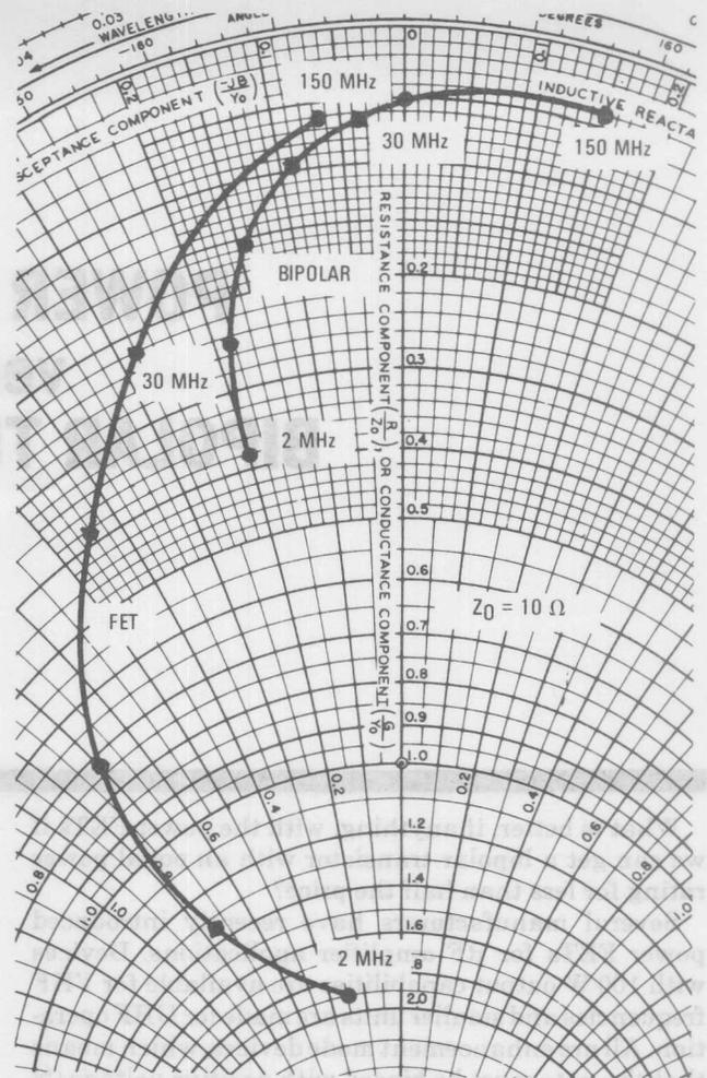
FIGURE 1 — 150 Watt MOSFET and Bipolar Comparison
