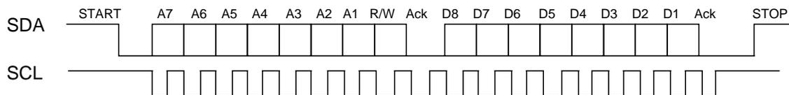
**Figure 2. Example of I<sup>2</sup>C Transfer Timing**
