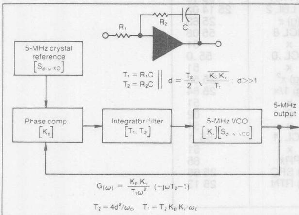
6. The phase-output noise in this type-2 second-order PLL can be optimized by adjusting the damping factor ( $d$ ) in relation to the oscillator-noise crossover frequency ( $f_d$ ).
