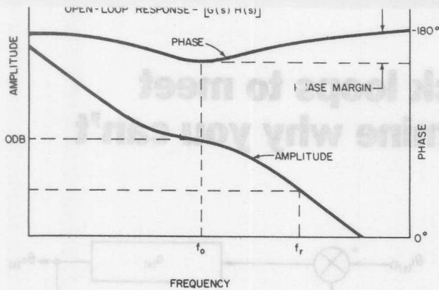
2. This open-loop gain/phase plot shows a typical phase displacement from  $-180^\circ$ . When the frequency,  $f_0$ , which corresponds to 0-dB gain, is made to align with the maximum phase displacement, calculating  $T_1$ ,  $T_2$  and  $T_3$  is simplified.
