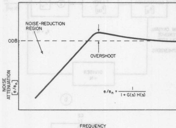
3. Increase  $f_0$  and you increase the noise-reduction region—the shaded area bounded by the 0-dB line and the noise-attenuation curve.
