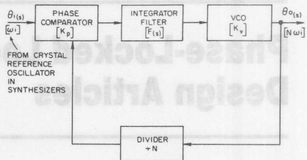
1. A type-2 phase-lock loop has two true integrators—the integrator/filter ( $F_s$ ) and the VCO ( $K_v$ ). Replacing the integrator/filter with a passive-RC network converts the circuit to a type-1 system.
