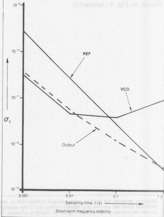
8. The phase-noise characteristics of the reference oscillator and the VCO can be expressed with three straight-line segments (I, II, and III); and the PLL output, by two (top). The short-term stability in terms of the Allan variance can then be calculated by keying the required coefficients as determined from the coordinates of these line-segment ends into the calculator (see Table) and plotting the results (bottom).
