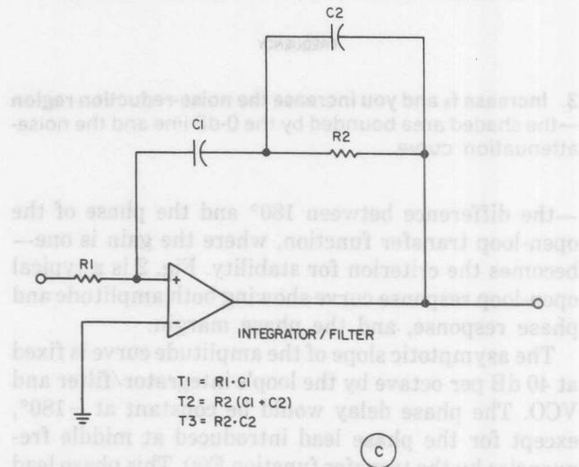
1. A phase-lock loop (a) with two integrators (b) is classified type 2. And the order—third, in this case—is established by the characteristics of the integrator/filter (c). Time constants  $T_1$ ,  $T_2$  and  $T_3$  determine the integrator/filter's detailed performance.
