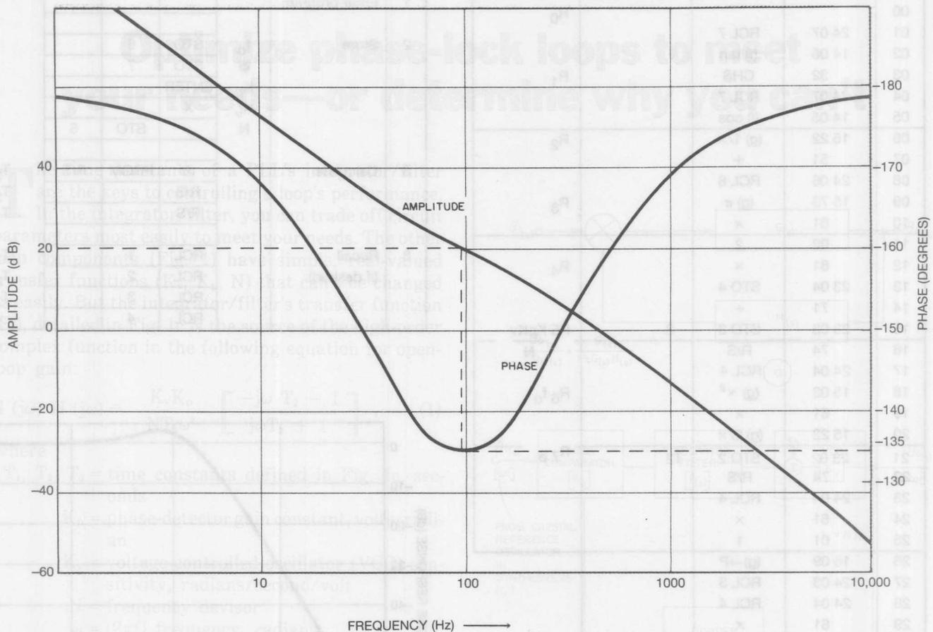
4. This plot of a PLL's open-loop transfer function confirms the design-parameter choices—a 45° phase margin
