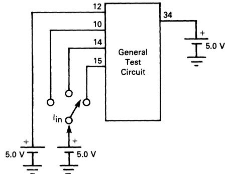
Measure  $I_{in}$  at each of three inputs. For each, calculate:
