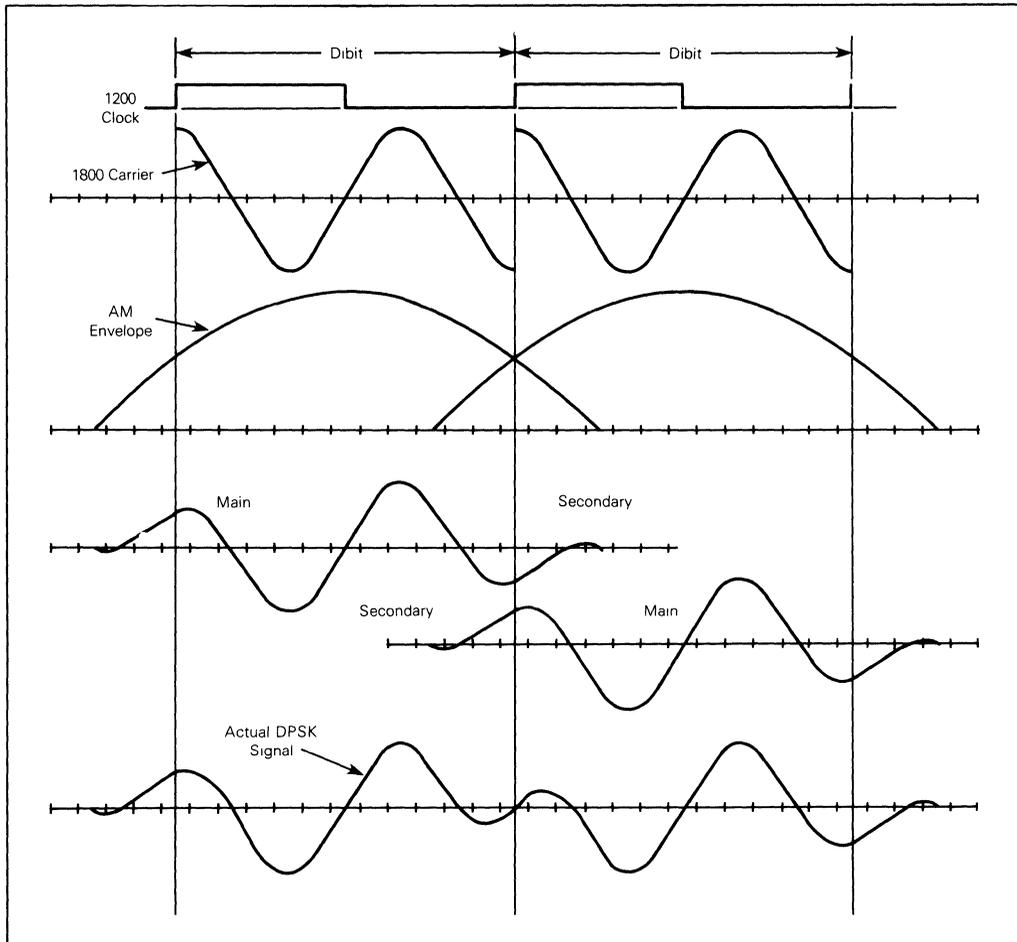
FIGURE 2—DPSK Waveforms
