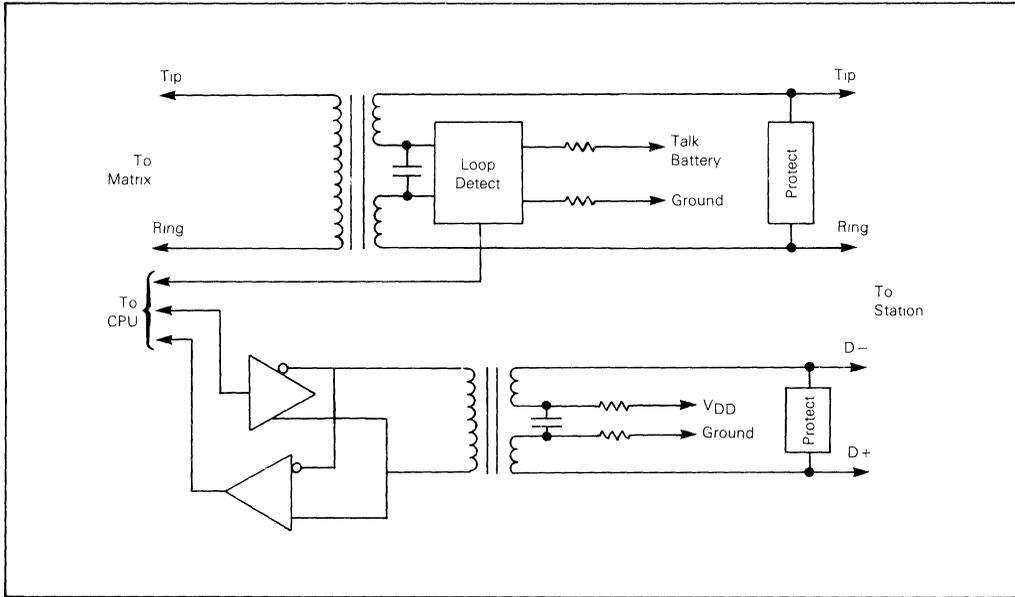
FIGURE 5 — Station Interface (Without Ring Generator)
