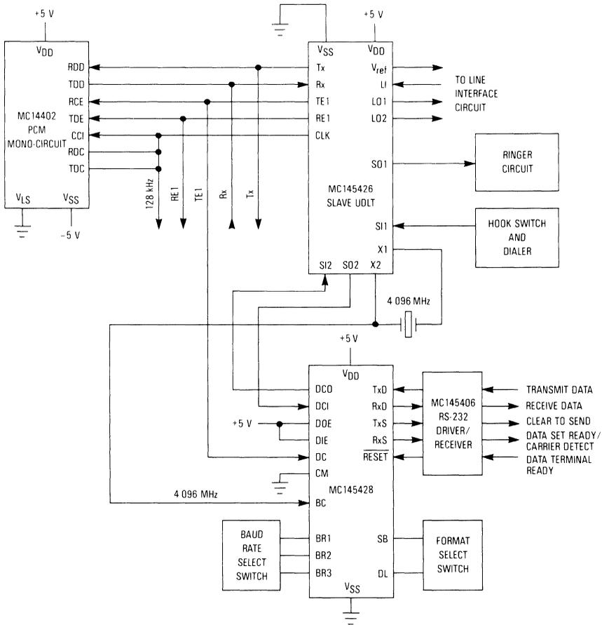
NOTE Some pin connections on the MC145426 and MC14402 have been omitted. Consult MC145426 and MC14402 data sheets for more details.
