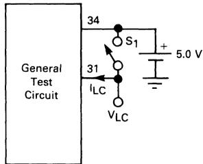
With  $S_1$  open measure  $V_{LC}$ .
