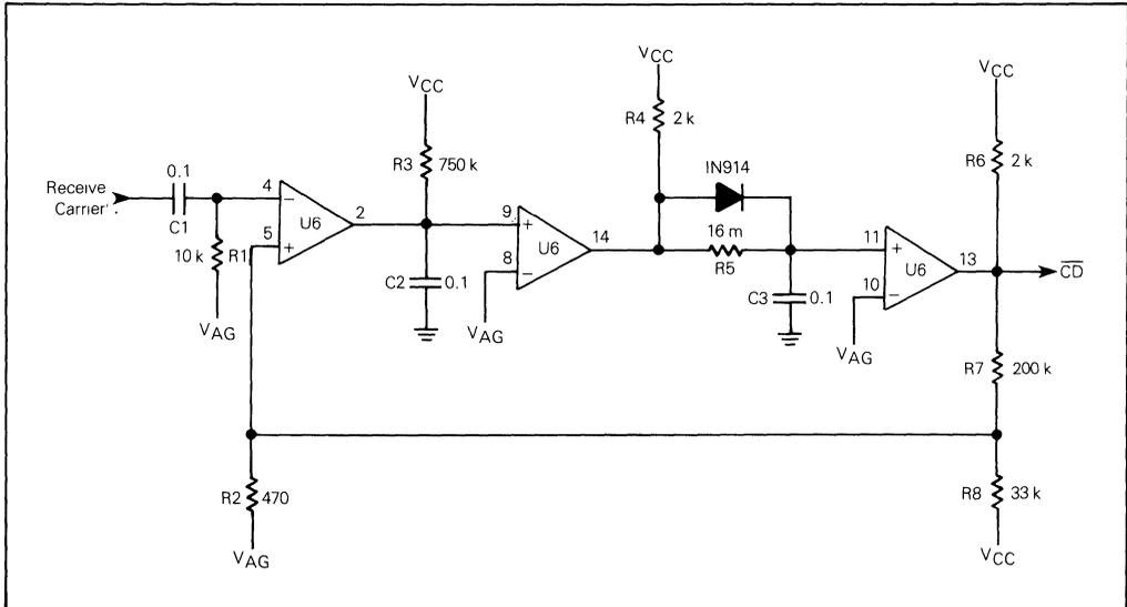
FIGURE 2 — CARRIER DETECT
