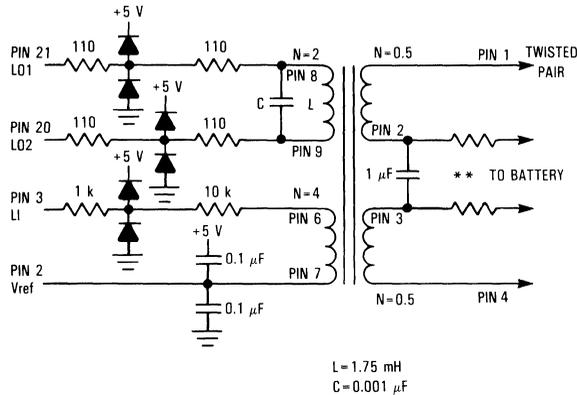
\*\* Battery Feed limiting resistors. (optional)
