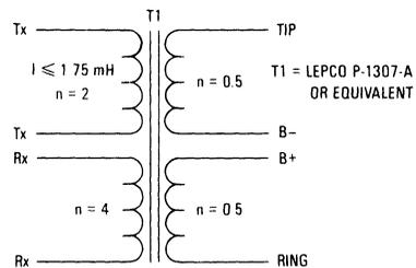
Figure 3. DLT Coupling Transformer
