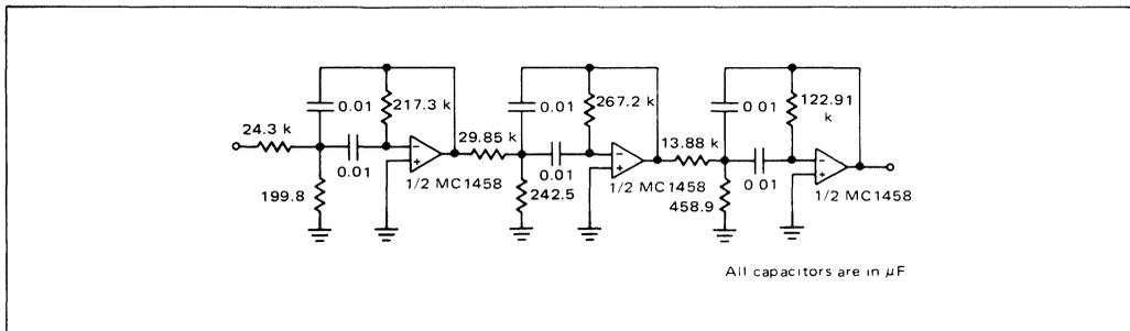
FIGURE 14a – Originate Filter Component Values
