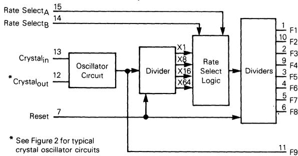
\* See Figure 2 for typical crystal oscillator circuits
