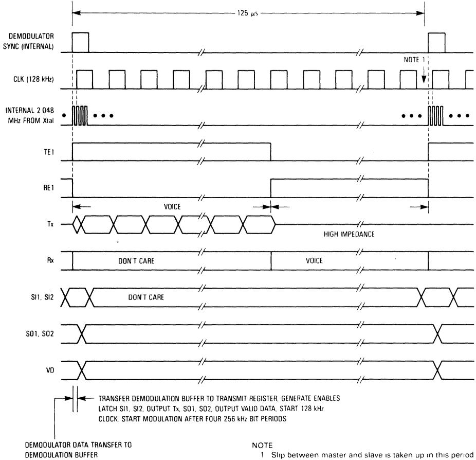
Figure 13. Slave DLT Timing
