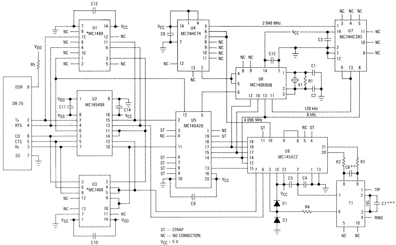
Figure 5. Master Limited Distance Modem
