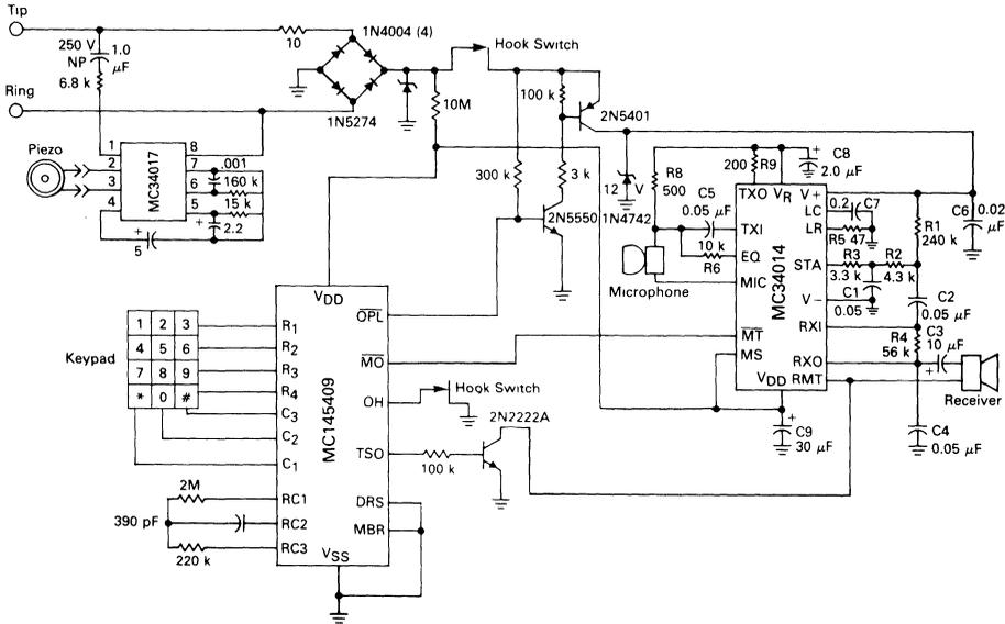
FIGURE 23 — SWITCHABLE HANDSET/HANDSFREE SYSTEM
