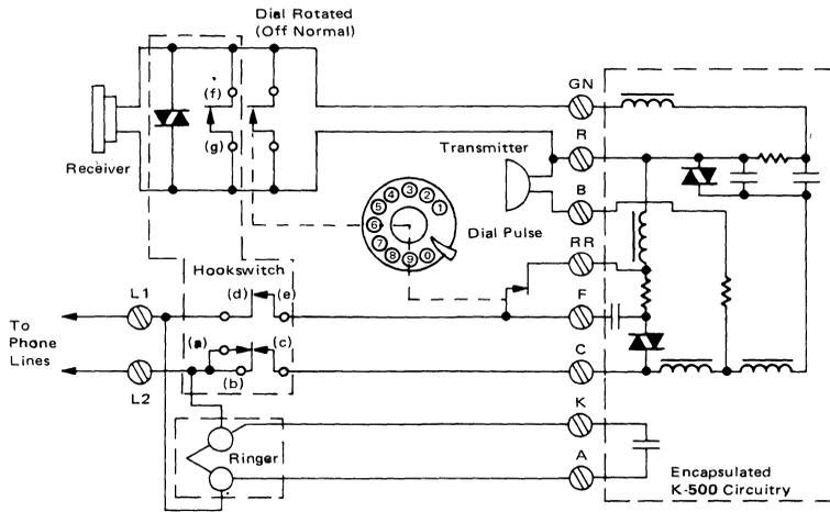
FIGURE 11 — MODIFIED K-500 TELEPHONE
