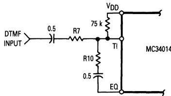
Figure 5. Alternate Biasing
