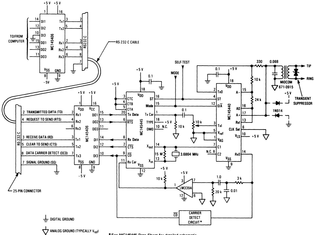
Figure 3. 5 Volt 300 Baud Modem with RS-232-C Interface
