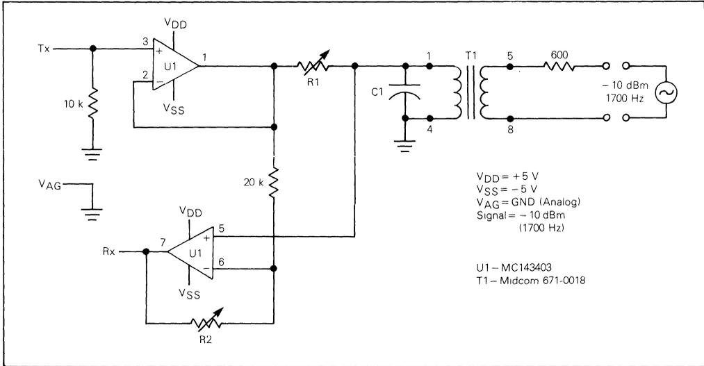
FIGURE 1 – Duplexer Circuit
