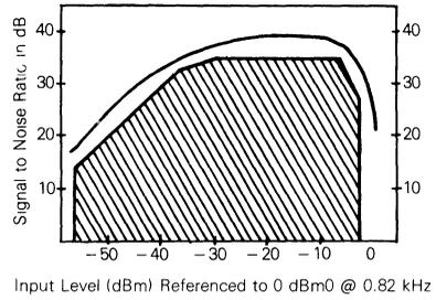
SINUSOIDAL GAIN TRACKING
