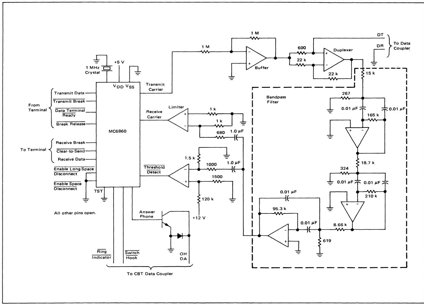
FIGURE 9 - Originate Modem
