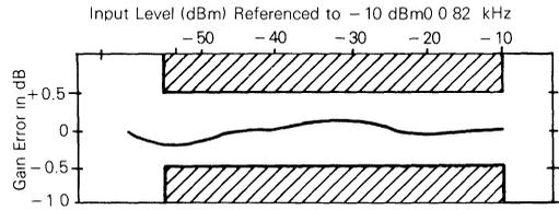
GAIN vs FREQUENCY, SINUSOIDAL
