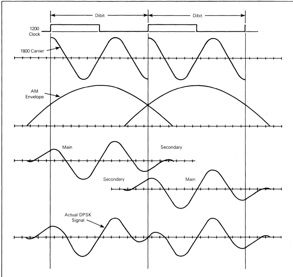
FIGURE 2—DPSK Waveforms
