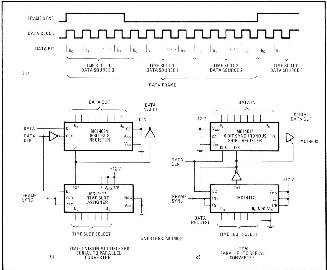
**The right slot.** Time-domain multiplexing (a) assigns to data from several sources specific time slots in a serial data stream. Capturing data from a specific slot is made easy with the MC14417 time-slot assigner (b), which works with the MC14094 shift register to provide data from the source dictated by the select inputs of the 14417. The versatile chip can also provide parallel-to-serial multiplexing (c).
