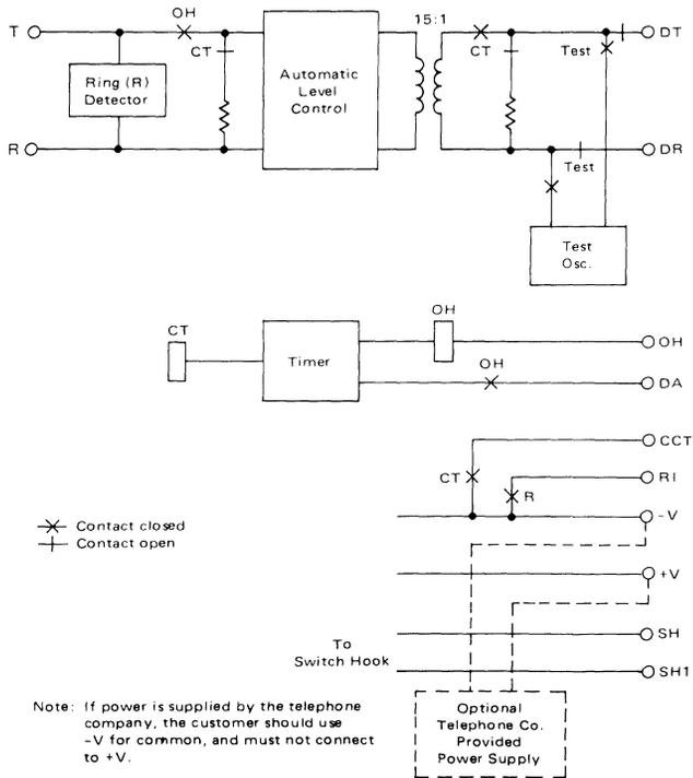
Note: If power is supplied by the telephone company, the customer should use -V for common, and must not connect to +V.
