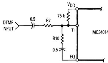
Figure 5. Alternate Biasing
