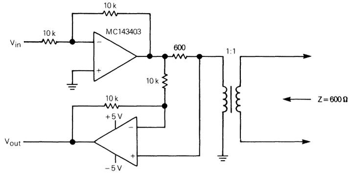
FIGURE 4 — HIGH POWER DUPLEXER (2-Wire to 4-Wire Converter)
