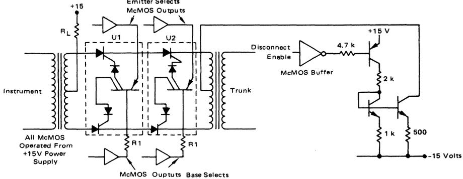
FIGURE 22 - TYPICAL INSTRUMENT TO INSTRUMENT CONNECTION
