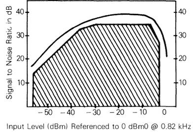
SINUSOIDAL GAIN TRACKING
