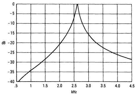
FIGURE 4 — Notch Frequency Response
