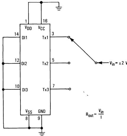
Figure 1. Power-Off Source Resistance (Drivers)
