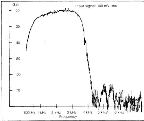
**2. The switched-capacitor low-pass filter limits both input and output frequencies to about 3.7 kHz, as reflected by the system frequency response curve. Input frequencies are limited to prevent aliasing; filtering the output smooths it out. Bandwidth for the circuit ranges from 500 Hz to 3.7 kHz.**
