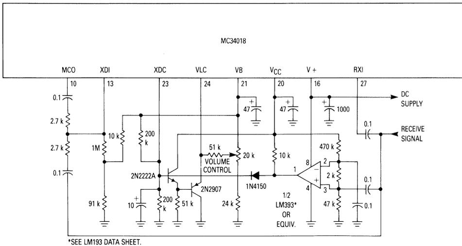
Figure 1. Receive-Idle Circuit
