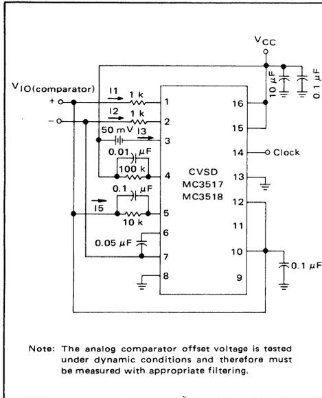
**FIGURE 4 – INTEGRATOR AMPLIFIER OFFSET VOLTAGE AND CURRENT**
