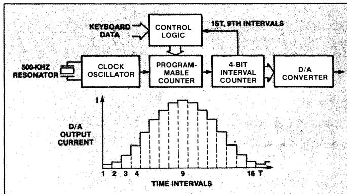
Fig. 2 The DTMF frequency synthesis technique.
