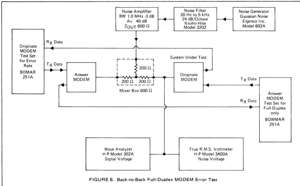
FIGURE 6. Back-to-Back Full-Duplex MODEM Error Test
