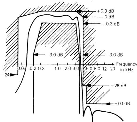
GAIN vs FREQUENCY, SINUSOIDAL
