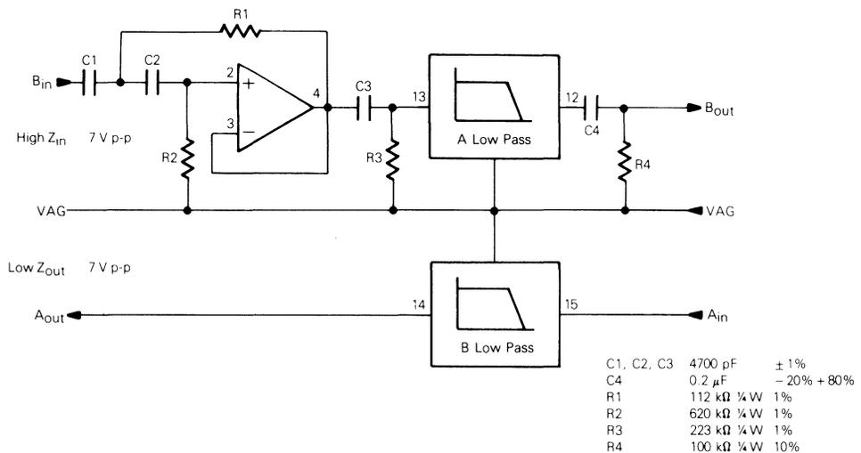
NOTE: In noisy environment, R1-R4 should be 10 kΩ or less to minimize pickup.
