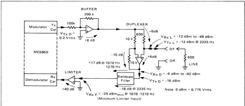
FIGURE 12 – System Level Constraints
