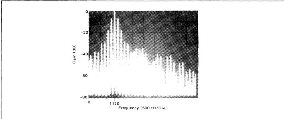
FIGURE 4 – Modulation Spectrum for Alternate Mark/Space
