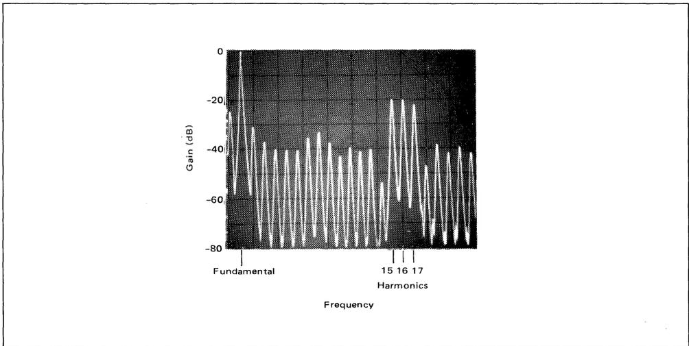
FIGURE 3 – Frequency Spectrum of MOS Sine Wave
