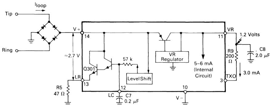
FIGURE 6 — INTERNAL CURRENT versus VOLTAGE
