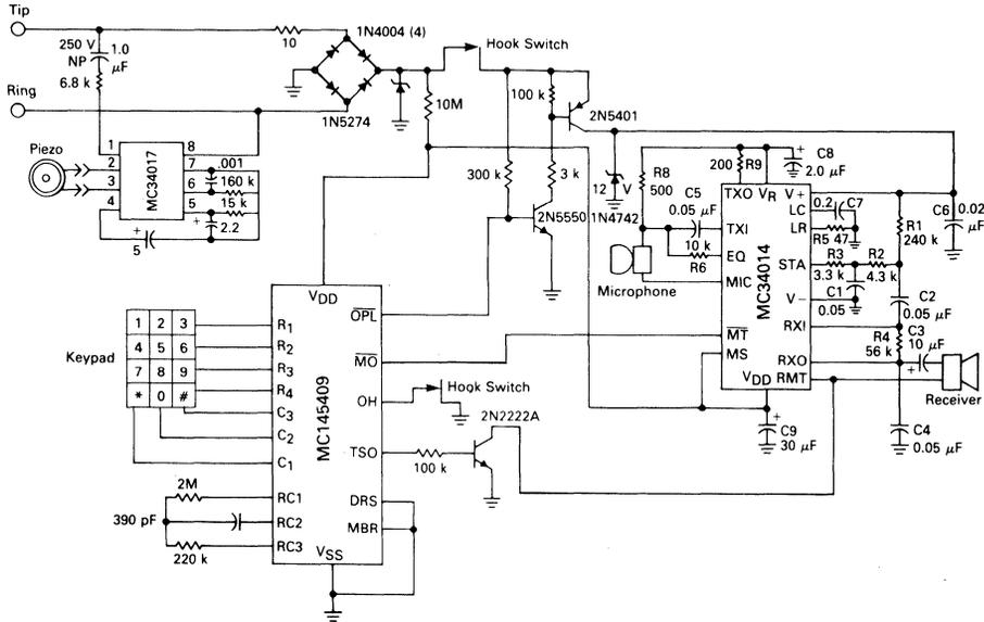
FIGURE 23 — SWITCHABLE HANDSET/HANDSFREE SYSTEM
