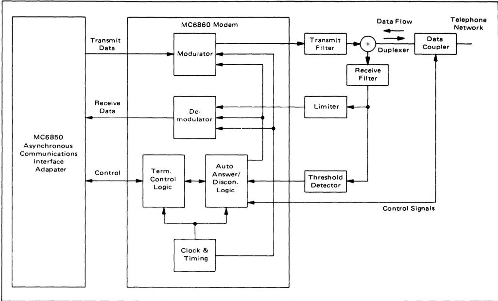
FIGURE 8 – Typical MC6860 Modem System
