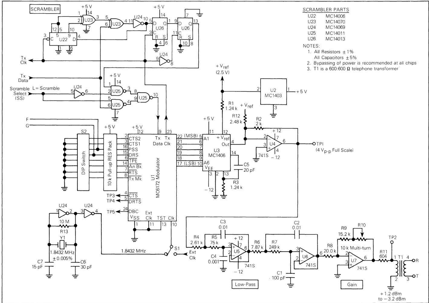
FIGURE 4 — 2400 BPS DPSK Modulator System
