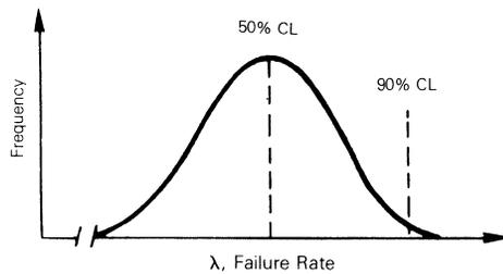
Both the infant mortality and random failure rate regions can be described through the same types of calculations. During this time the probability of having no failures to a specific point in time can be expressed by the equation:
