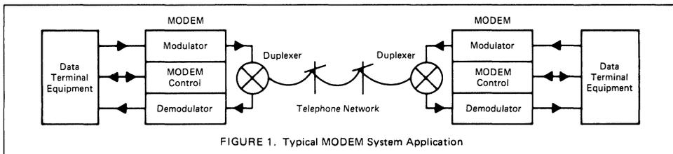
FIGURE 1. Typical MODEM System Application
