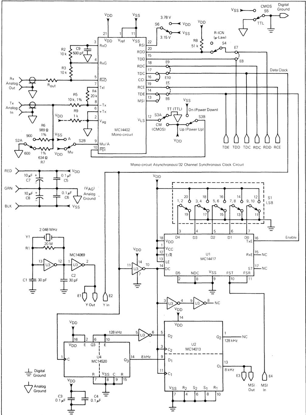
FIGURE 1 — MC14402 Switch Programmable Evaluation Board P/N 618-1030
