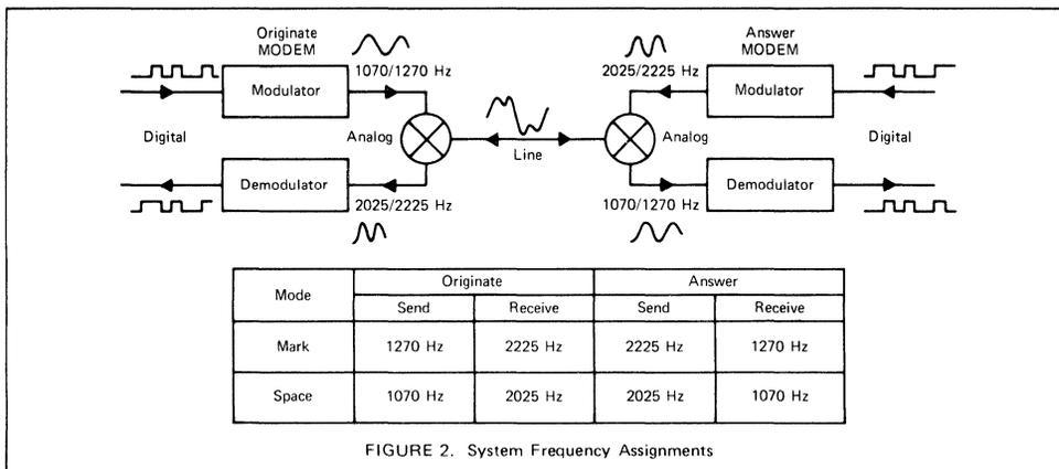
FIGURE 2. System Frequency Assignments
