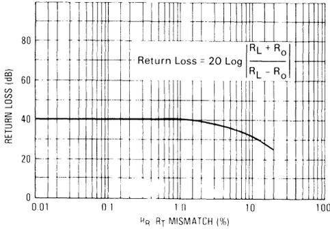
**FIGURE 9 — TRANSHYBRID REJECTION versus TIP/RING RESISTOR MISMATCH**
