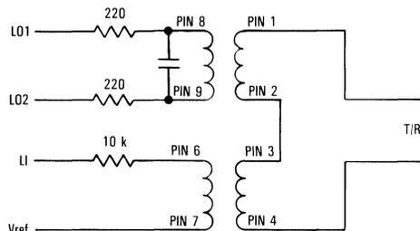
Figure 3. Transformer Configuration
