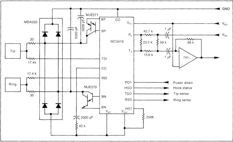
**2. A line-driver card requires a SLIC, two Darlington pairs, a rectifier bridge for lightning protection, and an operational amplifier. A resistor in the op amp's feedback path adjusts the transmission output gain.**
