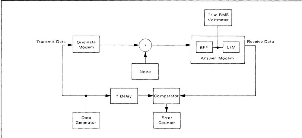
FIGURE 16 – Modem Test Equipment Configuration
