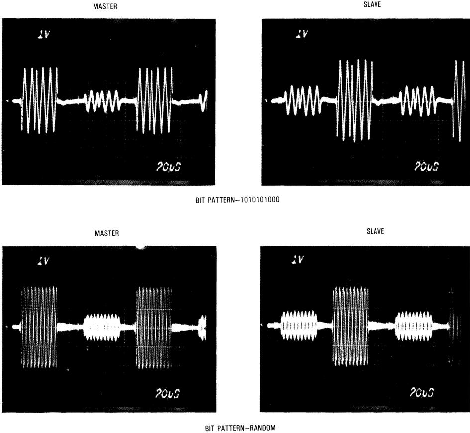
Figure 14. Typical Signal Waveforms at Demodulator
