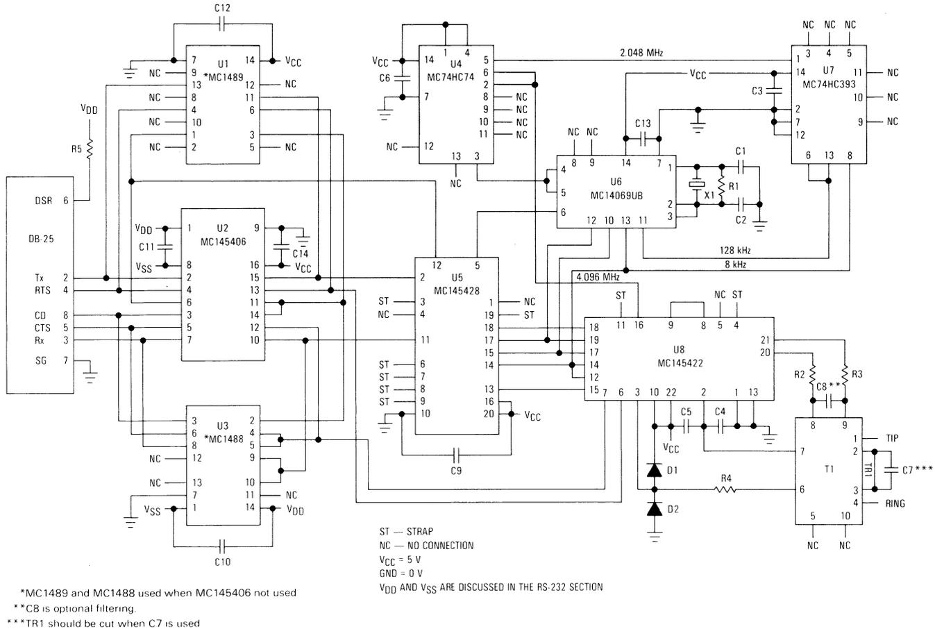
Figure 5. Master Limited Distance Modem
