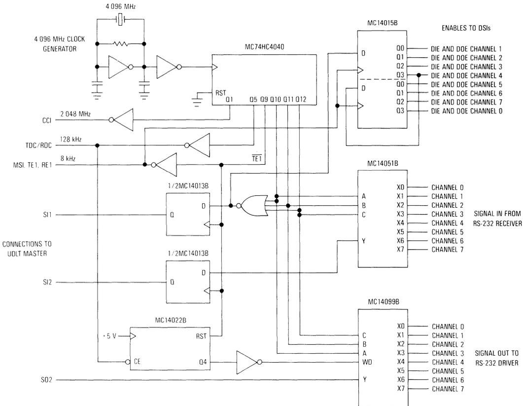
Figure 7. Master Sequencing and Signalling
