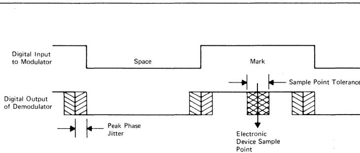
FIGURE 5. Demodulator Data Bit Output
