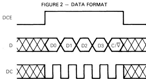
When C/V is "1", D0-D3 are loaded into the configuration register. The four configuration register bits then address a ROM which has outputs to control the analog subsystem elements, enable the appropriate volume register, select the appropriate volume register for the speaker/ringer volume control, and provide the SAE output.
