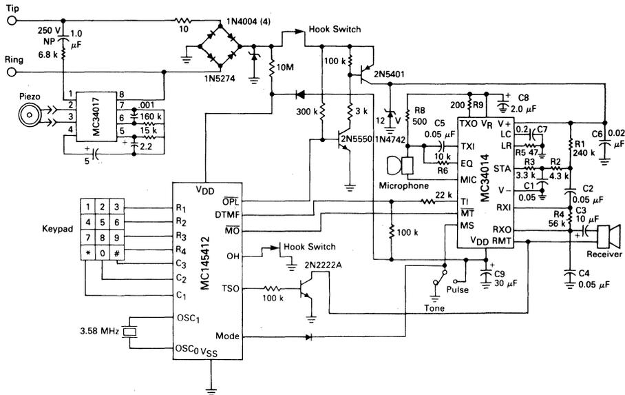
FIGURE 22 — COMPLETE TELEPHONE WITH PULSE DIALING
