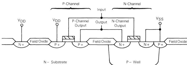
FIGURE 4 – LATCH UP CIRCUIT SCHEMATIC
