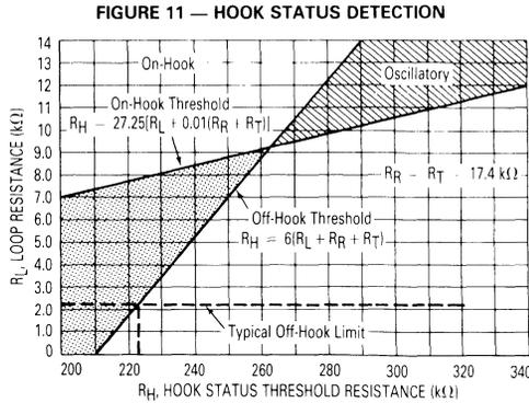
Figure 11 shows such a graph using 17.4 kΩ as the values for  $R_R$  and  $R_T$ . Note the oscillatory condition to the right of the crossing point. Selection of  $R_H$  in this region is usually not a problem since the majority of telephone lines do not fall into this resistance range.  $R_H$  always ties to  $V_{QB}$  and HST and will give reliable hook status information regardless of power supply voltages and  $PDI$ .
