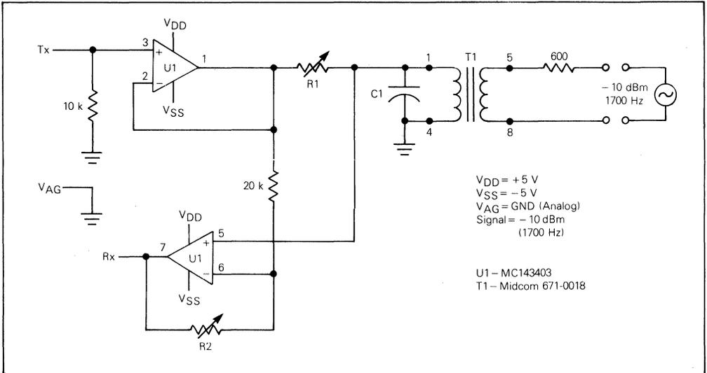
FIGURE 1 — Duplexer Circuit
