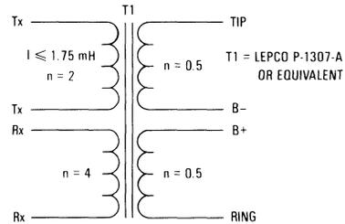
Figure 3. DLT Coupling Transformer
