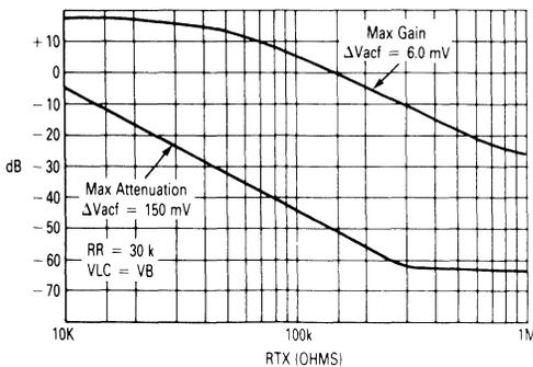
FIGURE 3 — RECEIVE ATTENUATOR versus RRX
