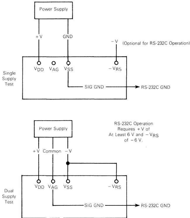
FIGURE 5 — Power Supply Set-Up
