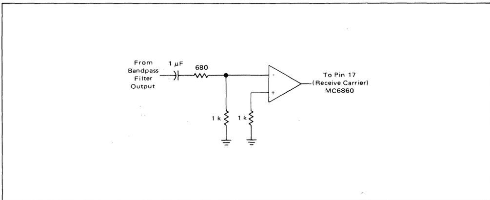
FIGURE 11 – Limiter Schematic
