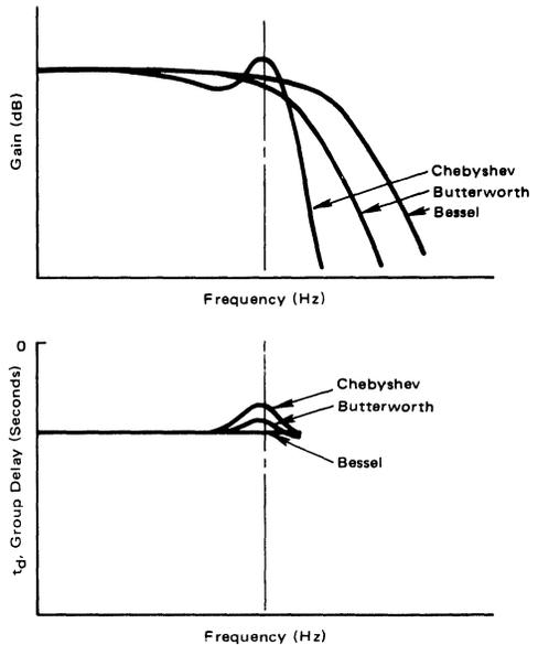
FIGURE 10 – Filter Approximation Characteristics
