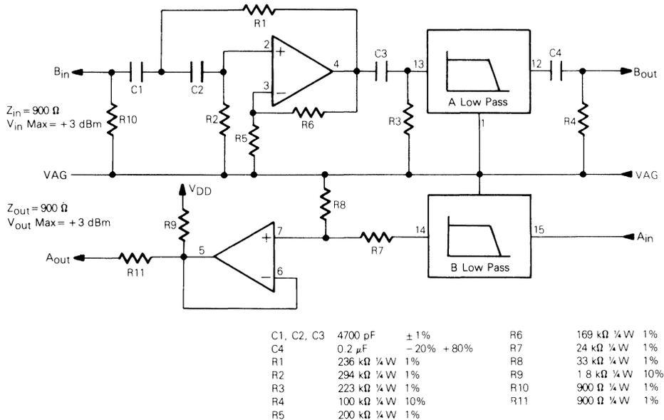
NOTE: In noisy environment, R1-R4 should be 10 kΩ or less to minimize pickup.
