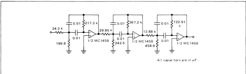
FIGURE 14a – Originate Filter Component Values
