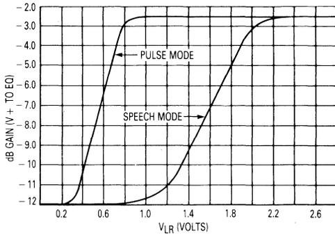
FIGURE 12 — EQ (PIN 6) DC VOLTAGE
