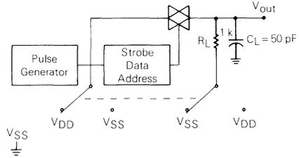
FIGURE 3 – BANDWIDTH AND FEEDTHROUGH ATTENUATION
