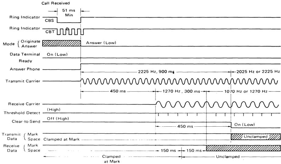
FIGURE 5 – AUTOMATIC DISCONNECT – LONG OR SHORT SPACE
