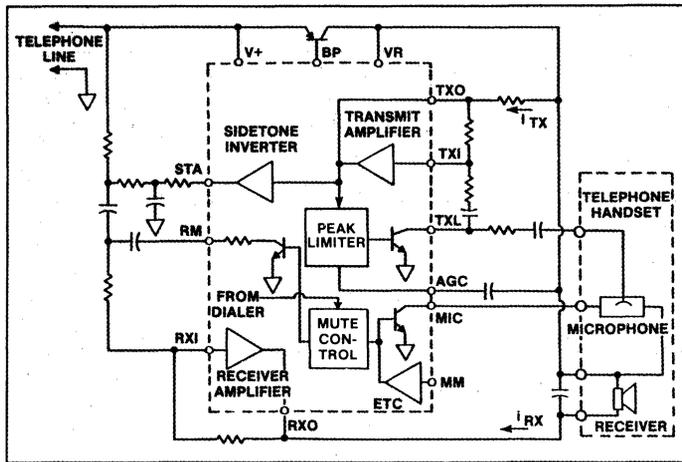
Fig. 4 Speech network block diagram.
