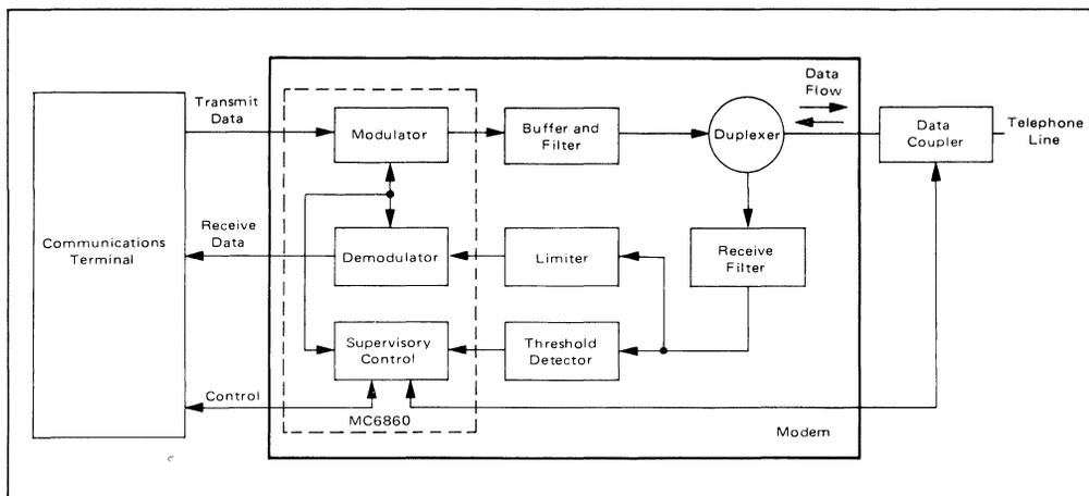
FIGURE 1 – Low-Speed Modem and Interconnections
