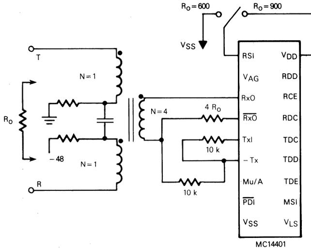
Simplified Transformer Hybrid Using MC14401
