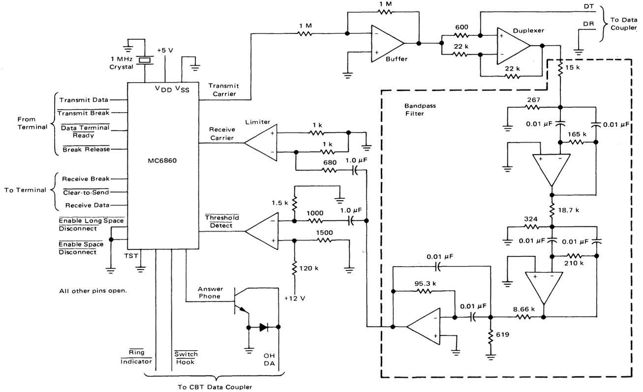
FIGURE 9 – Originate Modem
