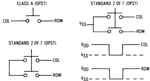
Figure 1. Keyboard Configurations
