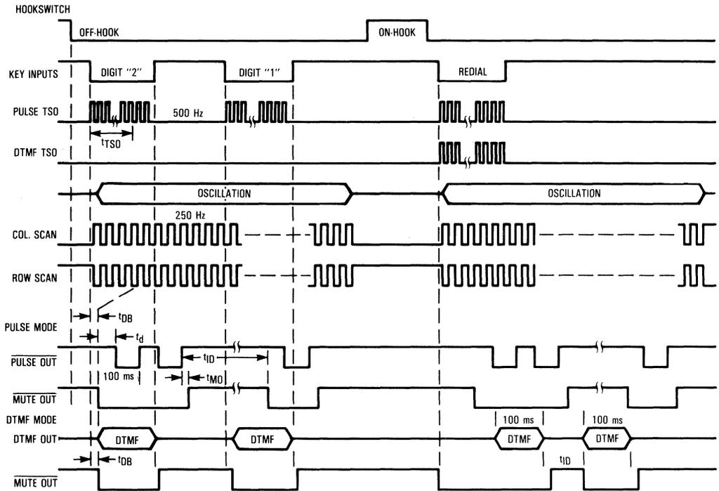
Figure 2. Timing Diagram
