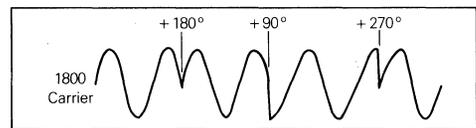
FIGURE 1—DPSK Format
