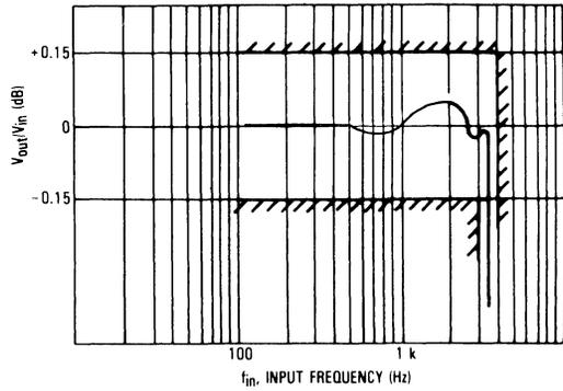
FIGURE 3 — TRANSMIT FILTER TYPICAL AND GUARANTEED PERFORMANCE (MC14413-1, -2 AND MC14414-1, -2 USING FIGURES 10 AND 11)
