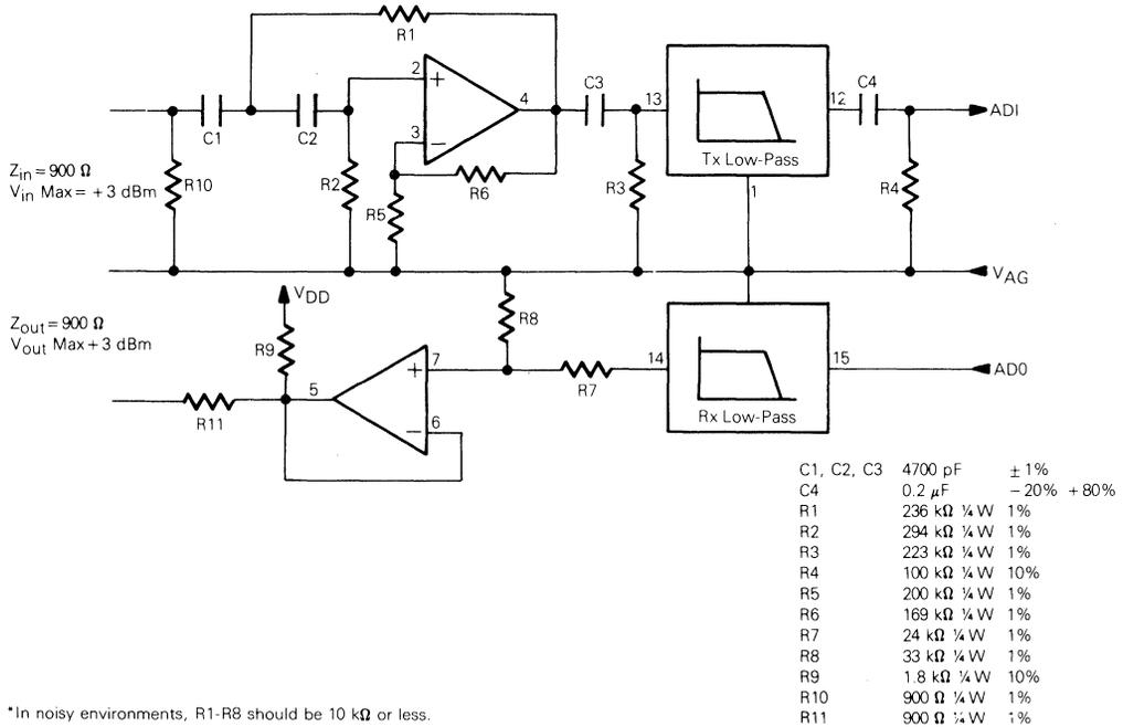
FIGURE 12 — TYPICAL 2-WIRE PORT INTERFACE USING MC14413
