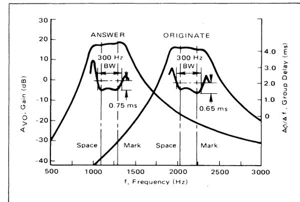
FIGURE 17b – Switchable Filter Response
