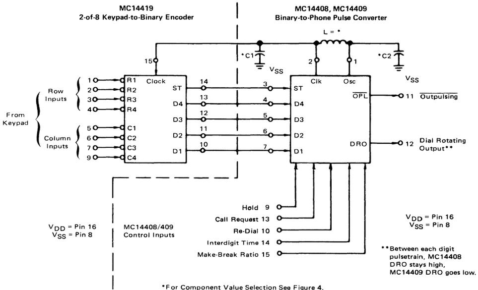
FIGURE 10 — STANDARD K-500 TELEPHONE
