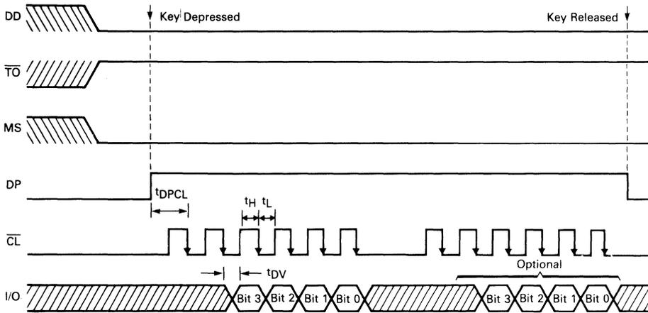
FIGURE 10 — INPUT DATA CYCLE TO MC34010
