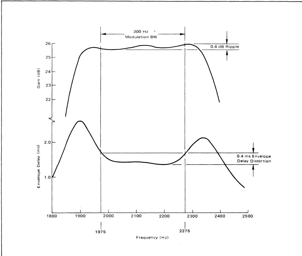
FIGURE 10 – Originate Bandpass Filter Characteristics
