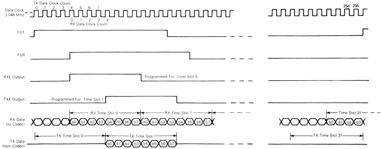
FIGURE 7 — DATA MULTIPLEX TIMING FOR 1.544 MHz
