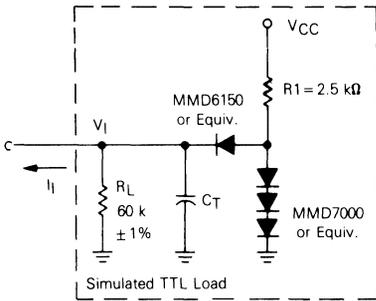
$C_T = 20 \text{ pF}$  = total parasitic capacitance, which includes probe, wiring, and load capacitances.
