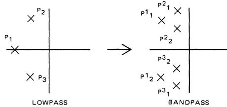
The bandpass filter will take on a form of three 2-pole bandpass filter sections in cascade. When bandpass sections are cascaded, each section center frequency and Q must be determined from the low pass damping factors (ξ) and natural frequencies (ω).
