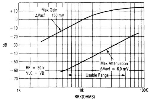
FIGURE 4 — GAIN AND ATTENUATION versus RESISTOR RATIOS
