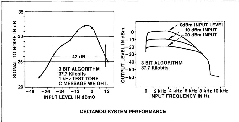
FIGURE 4 — SIGNAL TO NOISE PERFORMANCE AND FREQUENCY RESPONSE
