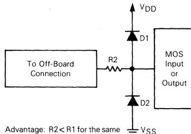
Advantage:  $R2 < R1$  for the same level of protection. Impact on ac and dc characteristics is minimized.
