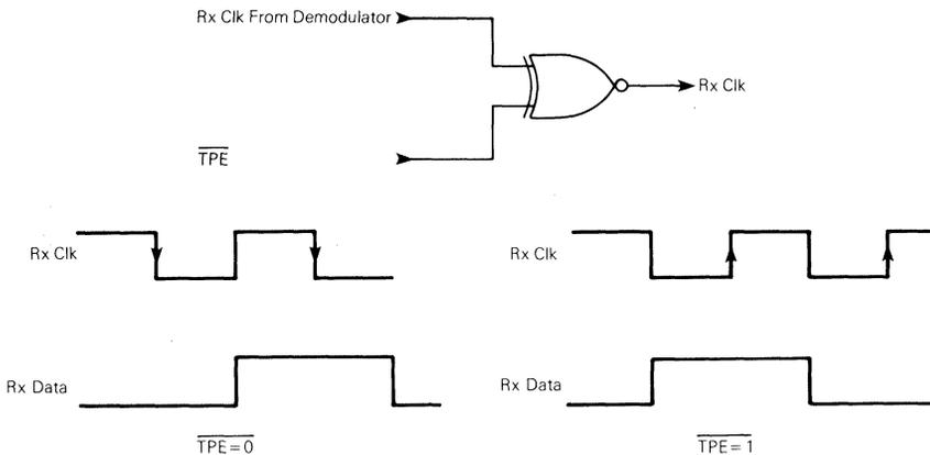
FIGURE 11 — PHASE-SHIFT SELECT DEMULTIPLEXER FOR TEST PATTERN ENABLE
