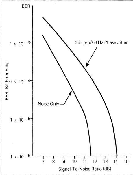
FIGURE 10 — B Mod 2400 BPS Back-To-Back 511 Test Pattern
