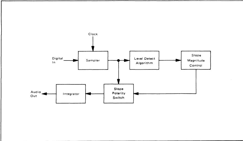
FIGURE 14 – 16 kHz SIMPLEX VOICE CODEC
