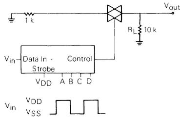
FIGURE 6 – CHANNEL RESISTANCE ( $R_{ON}$ ) TEST CIRCUIT
