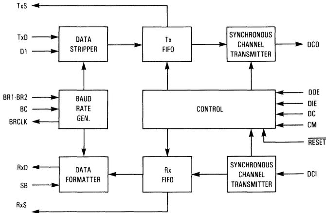
Figure 2. Block Diagram of the Data Set Interface
