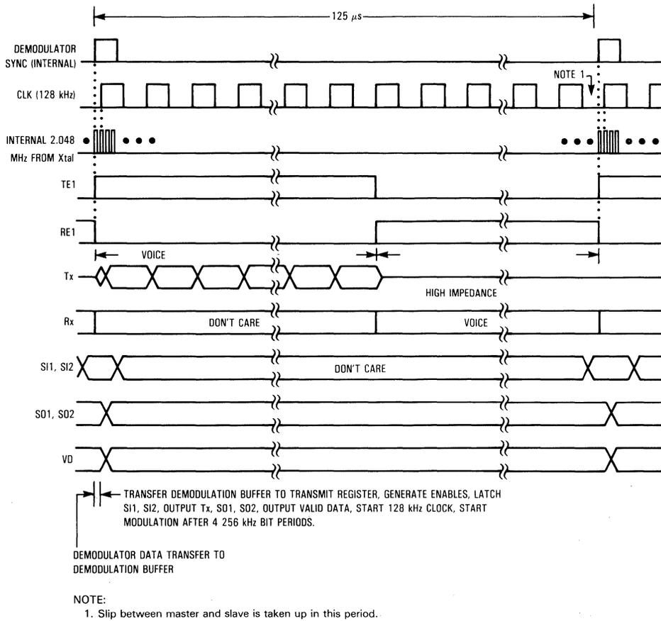
Figure 11. Slave UDLT Timing
