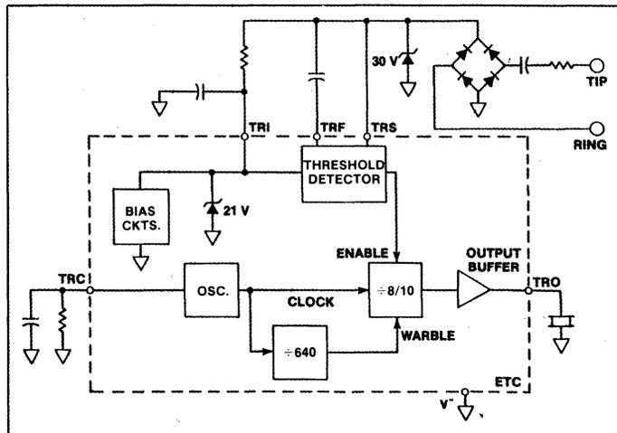
Fig. 5 Tone ringer block diagram.
