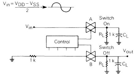
FIGURE 5 – CROSSTALK CONTROL TO OUTPUT
