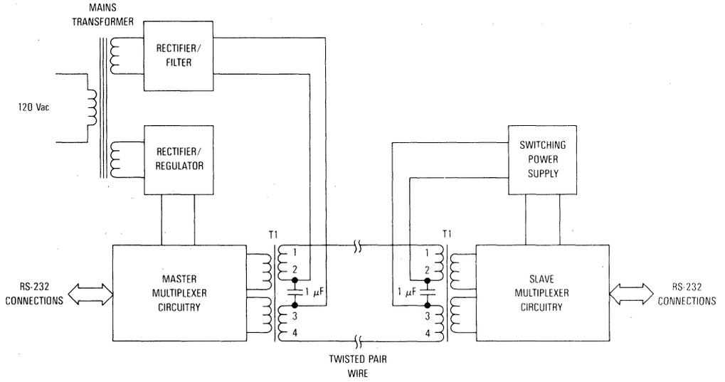
Figure 10. Powering Slave Unit From the Twisted Pair
