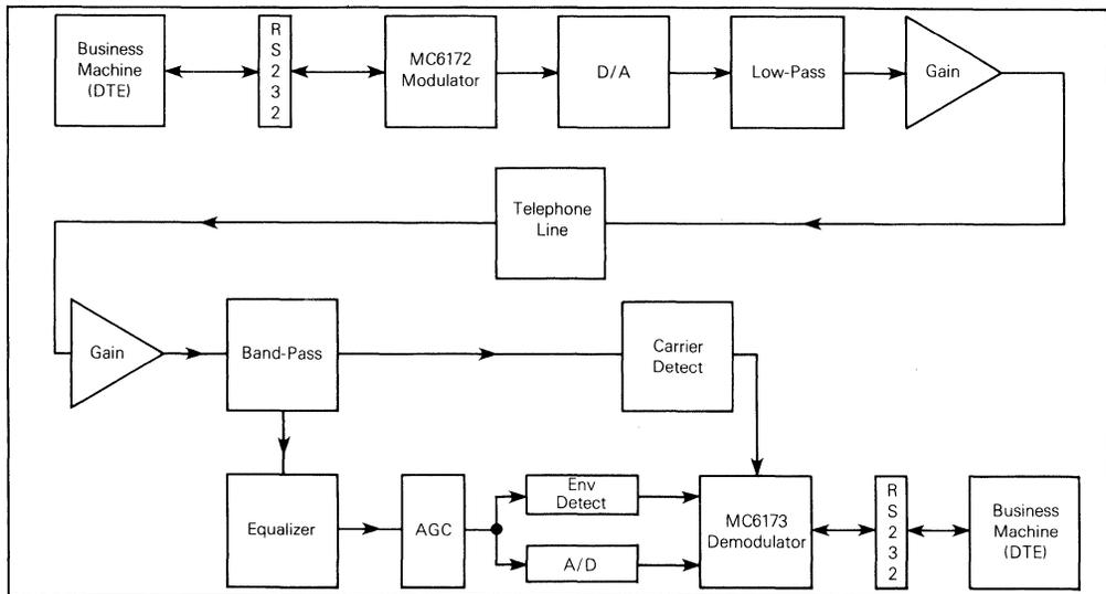
FIGURE 3—MC6172/6173 Modem Block Diagram
