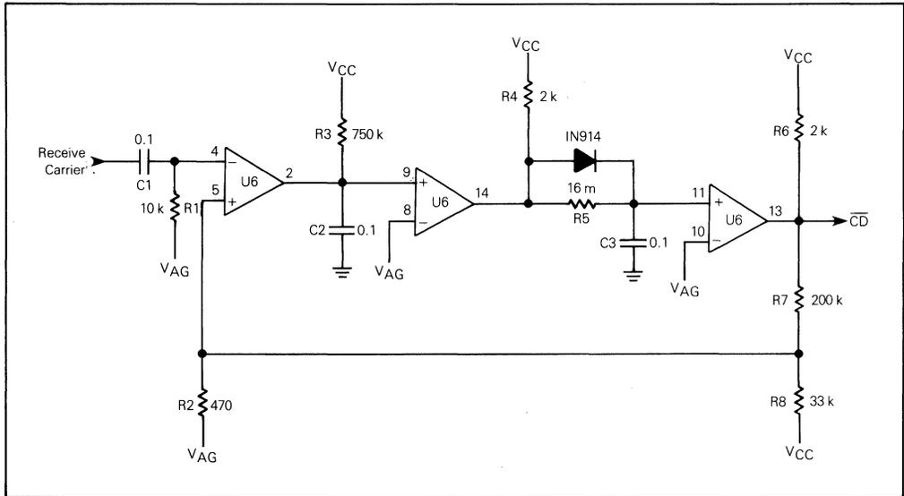
FIGURE 2 — CARRIER DETECT
