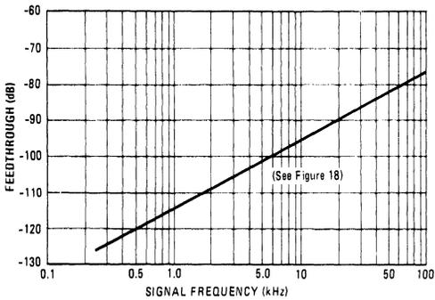
FIGURE 17 – CROSSTALK versus SIGNAL FREQUENCY
