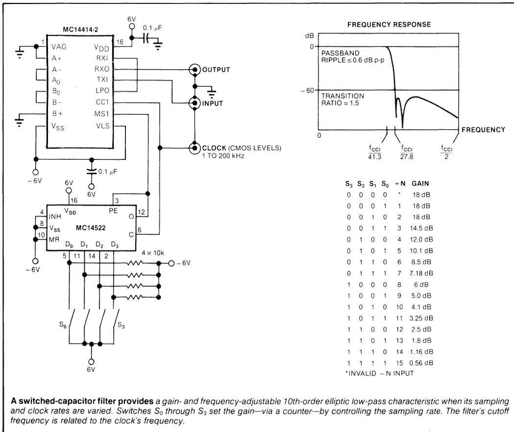
A switched-capacitor filter provides a gain- and frequency-adjustable 10th-order elliptic low-pass characteristic when its sampling and clock rates are varied. Switches  $S_0$  through  $S_3$  set the gain—via a counter—by controlling the sampling rate. The filter's cutoff frequency is related to the clock's frequency.
