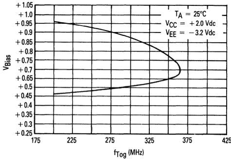
Figure 2 illustrates the variation in toggle frequency with the dc offset voltage ( $V_{Bias}$ ) of the input clock signal.
