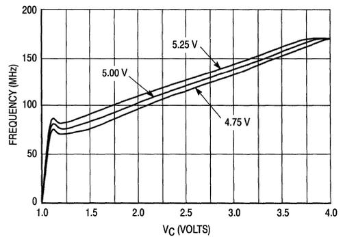
**Figure 9.  $V_C$  versus Output Frequency**
