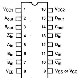
Pin assignment is for Dual-in-line Package.
