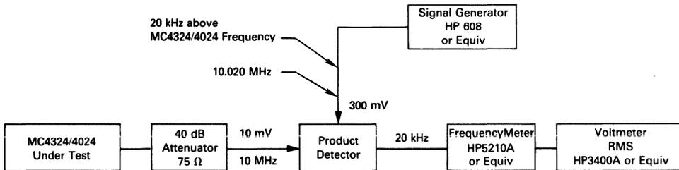
$$\text{Frequency Deviation} = \frac{(\text{HP5210A output voltage}) (\text{Full Scale Frequency})}{1.0 \text{ Volt}}$$
