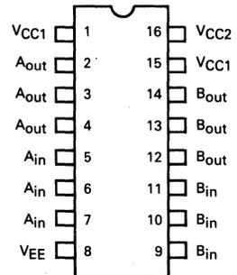
Pin assignment is for Dual-in-line Package.
