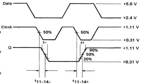
**FIGURE 3 – RESET to OUTPUT**
