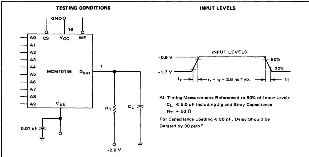
Guaranteed with  $V_{EE} = -5.2 \text{ Vdc} \pm 5.0\%$ ,  $T_A = 0^\circ\text{C}$  to  $75^\circ\text{C}$  (see Note 1). Output Load see Figure 1.
