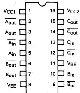
Pin assignment is for Dual-in-line Package.
