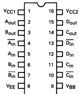
Pin assignment is for Dual-in-line Package.
