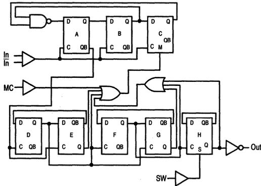
Figure 1. Logic Diagram (MC12052A)
