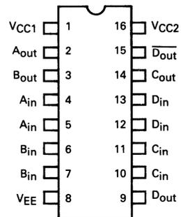
Pin assignment is for Dual-in-line Package.
