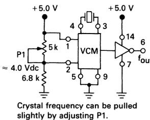
**FIGURE 3 — VOLTAGE-CONTROLLED MULTIVIBRATOR**
