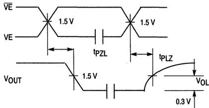
Figure 5. 3-State Output Low Enable and Disable Times
