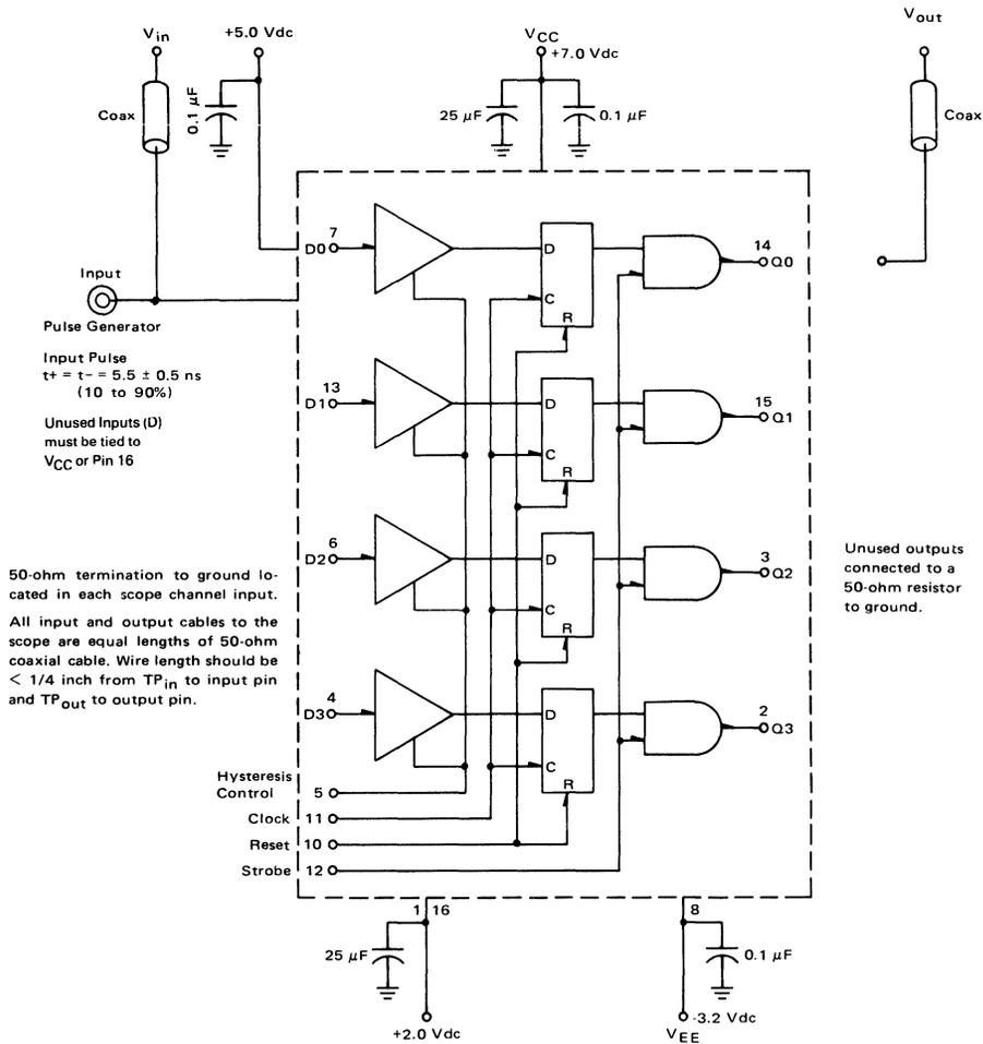
NOTE: All power supplies and logic levels are shifted 2 volts positive.
