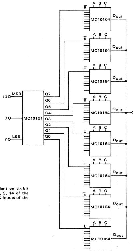
The Bit chosen is dependent on six-bit code present on inputs 7, 9, 14 of the MC10161 and the A, B, C inputs of the MC10164.
