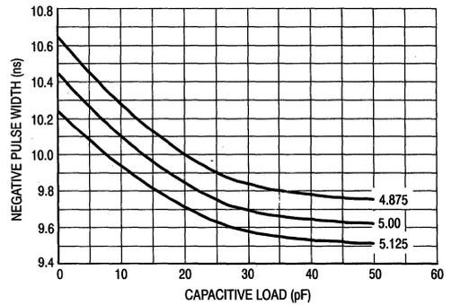
Figure 4. MC10H642 Negative PW versus Load
