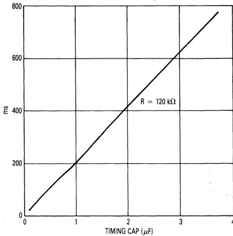
Figure 9-7. Jabber Time Constant versus Capacitance
