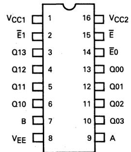
Pin assignment is for Dual-in-line Package.
