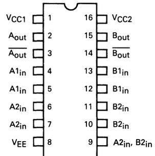
Pin assignment is for Dual-in-line Package.
