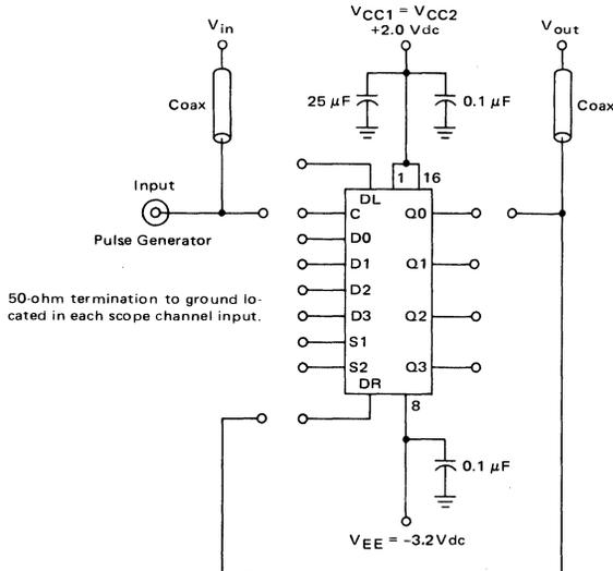
All input and output cables to the scope are equal lengths of 50-ohm coaxial cable. Wire length should be  $< 1/4$  inch from  $TP_{in}$  to input pin and  $TP_{out}$  to output pin.
