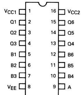
Pin assignment is for Dual-in-line Package.
