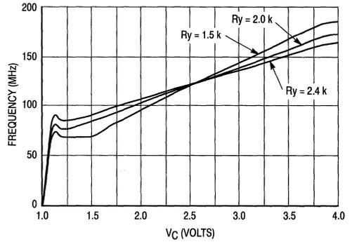
**Figure 7.  $V_C$  versus Output Frequency**
