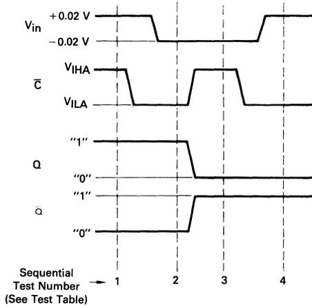
FIGURE 6 — TRANSFER CHARACTERISTICS (Q versus V<sub>in</sub>)
