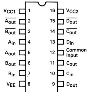
Pin assignment is for Dual-in-line Package.
