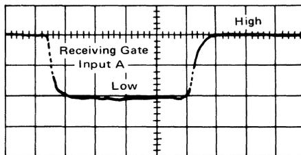
FIGURE 2b — PROPERLY TERMINATED TRANSMISSION LINE (Ground Plane Added)
