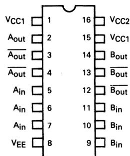
Pin assignment is for Dual-in-line Package.
