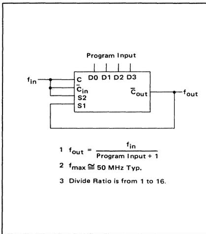
FIGURE 4 — 100 MHz PROGRAMMABLE COUNTER
