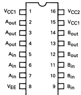
Pin assignment is for Dual-in-line Package.
