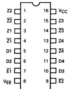
Pin assignment is for Dual-in-line Package.
