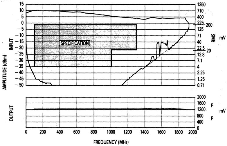
Figure 1. MC12076 Input Signal Amplitude versus Input Frequency
