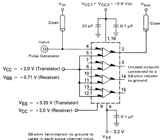
50-ohm termination to ground located in each scope channel input.
