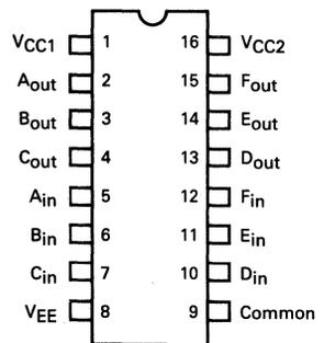
Pin assignment is for Dual-in-line Package.
