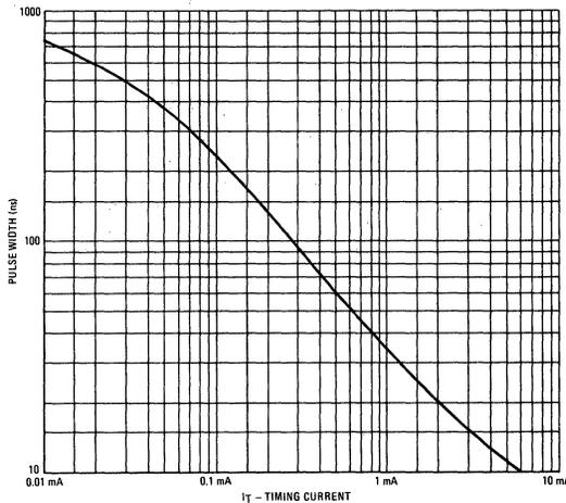
(b) A control voltage can also be used to vary the pulse width using an additional resistor (Figure 6). The current ( $I_T + I_C$ ) is set by the voltage drop across  $R_{Int} + R_{Ext}$ . The control current  $I_C$  modifies  $I_T$  and alters the pulse width. Current  $I_C$  should never force  $I_T$  to zero.  $R_C$  typically  $1$  k $\Omega$ .
