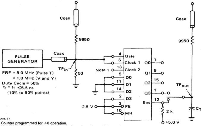
The coax delays from input to scope and output to scope must be matched. The scope must be terminated in 50-ohm impedance. The 9950-ohm resistor and the scope termination impedance constitute a 200:1 attenuator probe. Coax shall be CT-070-50 or equivalent.
