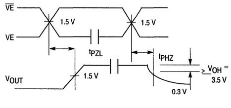
Figure 6. 3-State Output High Enable and Disable Times
