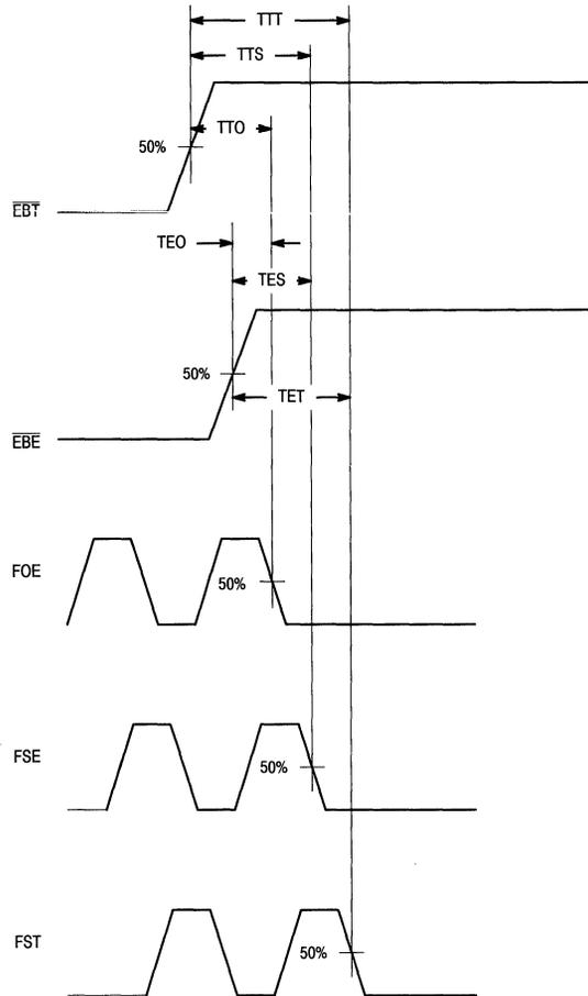
Figure 5. Switching Waveforms
