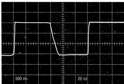
FIGURE 2A — +64, 500 MHz, 5.0 V, +25°C, OUTPUT LOADED
