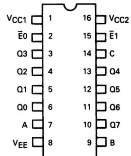
Pin assignment is for Dual-in-line Package.
