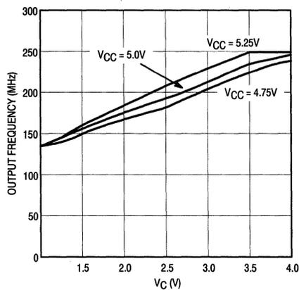
Figure 9.  $V_C$  versus Output Frequency
