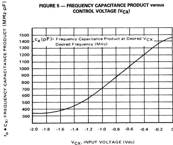
$V_{EE} = -5.2 \text{ V}$ ,  $V_{CC} = 0 \text{ V}$ .
