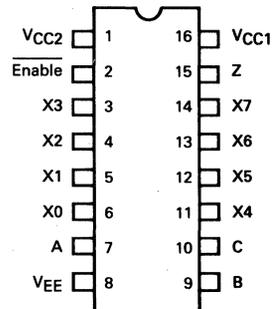
Pin assignment is for Dual-in-line Package.
