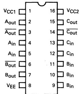
Pin assignment is for Dual-in-line Package.
