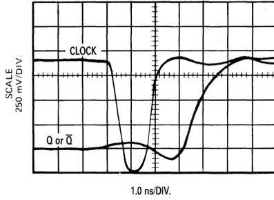
**FIGURE 5 — MINIMUM "UP TIME" TO CLOCK
