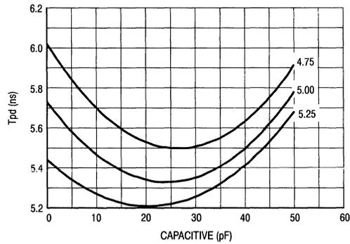
Figure 7. MC10H642 + Tpd versus Load,  $V_{CC} \pm 5\%$ ,  $T_A = 25^\circ\text{C}$
