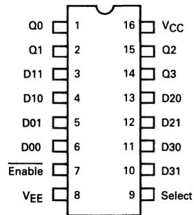
Pin assignment is for Dual-in-line Package.
