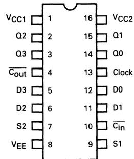
Pin assignment is for Dual-in-line Package.
