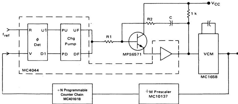
1 See Motorola Application Note AN-535 and the MC4344/4044 Data Sheet for detailed explanation of overall circuit operation.
