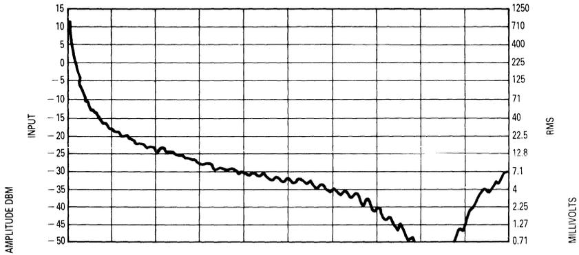
FIGURE 4B — OUTPUT AMPLITUDE versus INPUT FREQUENCY
