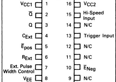
Pin assignment is for Dual-in-line Package.
