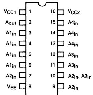
Pin assignment is for Dual-in-line Package.
