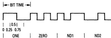
Figure 6-1. Encoded Data Representation
