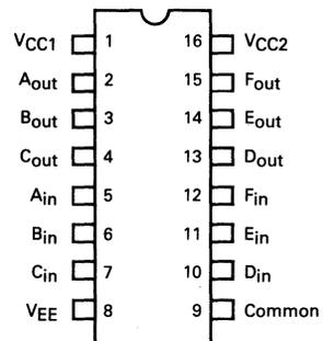
Pin assignment is for Dual-in-line Package.
