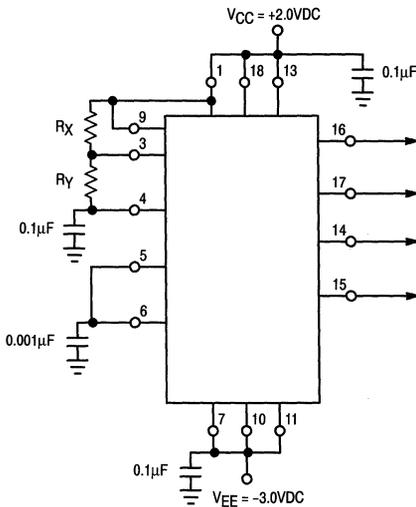
Figure 3. AC Test Circuit (FO/t<sub>rE</sub>/t<sub>fE</sub> Measurement)
