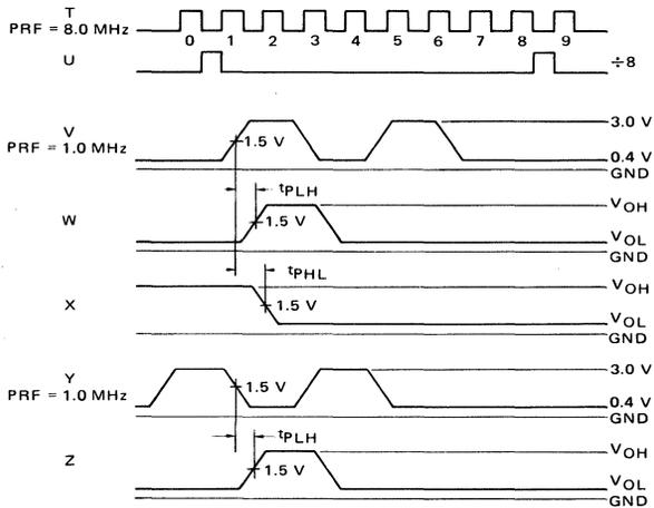
SWITCHING TIME TEST PROCEDURES ( $T_A = 25^\circ\text{C}$ )
