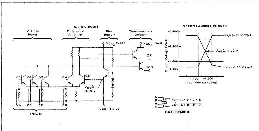
FIGURE 3 — MECL 10K GATE STRUCTURE AND SWITCHING BEHAVIOR
