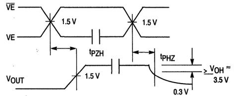
Figure 6. 3-State Output High Enable and Disable Times
