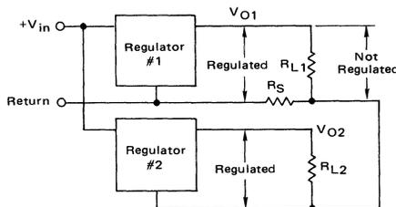
One solution to the ground-coupled noise problem is to lay out the return path with the most sensitive regulated circuit at the farthest point from power supply entry as shown in Figure 26.
