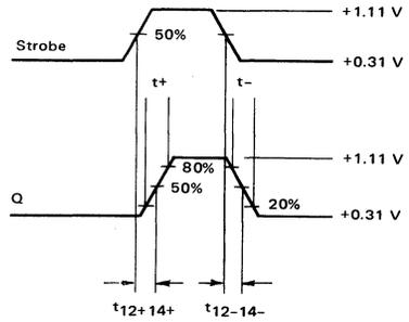
**FIGURE 4 – CLOCK to OUTPUT**
