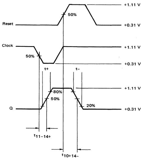
**FIGURE 5 – TSET UP AND THOLD WAVEFORMS**
