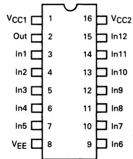
Pin assignment is for Dual-in-line Package.
