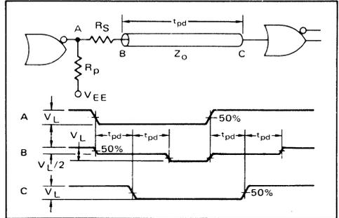
The advantages of series termination include ease of driving multiple series-terminated lines, low power consumption, and low cross talk between adjacent lines. The disadvantage of this system is that loads may not be distributed along the transmission line due to the one-half logic swing present at intermediate points.
