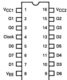
Pin assignment is for Dual-in-line Package.
