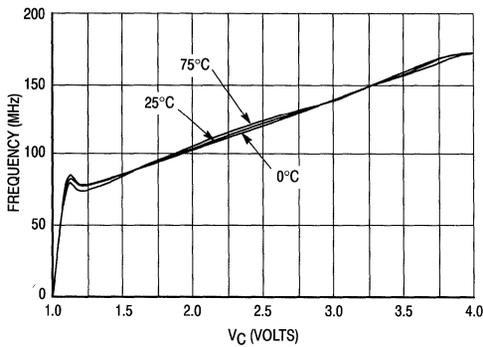
**Figure 8.  $V_C$  versus Output Frequency**
