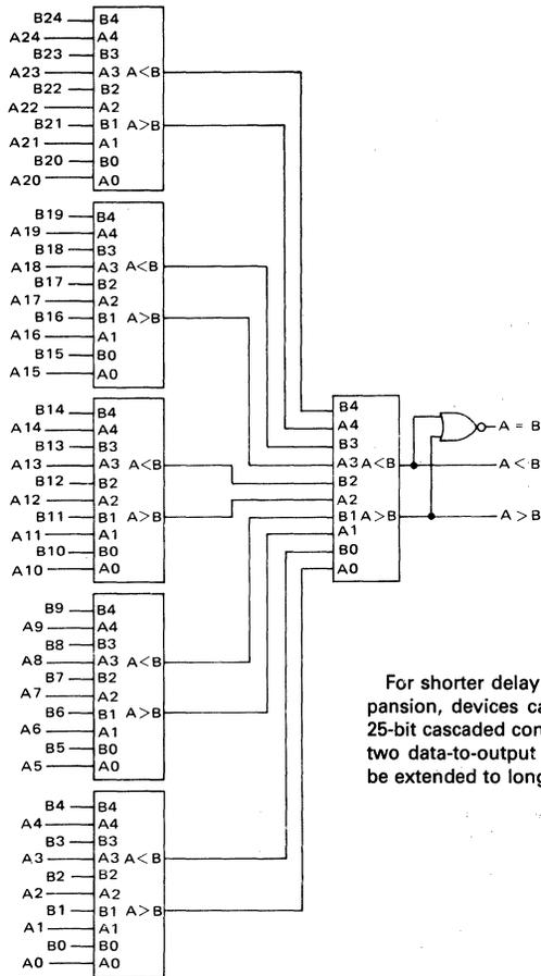
For shorter delay times than possible with serial expansion, devices can be cascaded. Figure 2 shows a 25-bit cascaded comparator whose worst case delay is two data-to-output delays. The cascaded scheme can be extended to longer word lengths.
