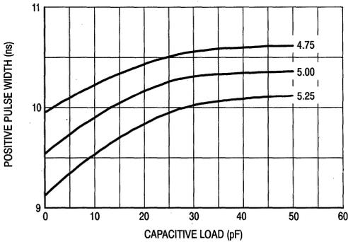
Figure 1. MC10H642 Positive PW versus Load
