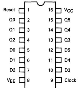
Pin assignment is for Dual-in-line Package.
