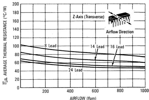
**FIGURE 17D — AIRFLOW versus THERMAL RESISTANCE (PLCC PACKAGE)**
