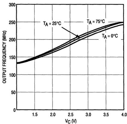
Figure 8.  $V_C$  versus Output Frequency
