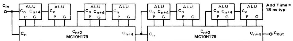
FIGURE 2 — 16-BIT FULL LOOK-AHEAD CARRY ARITHMETIC LOGIC UNIT
