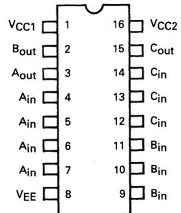
Pin assignment is for Dual-in-line Package.
