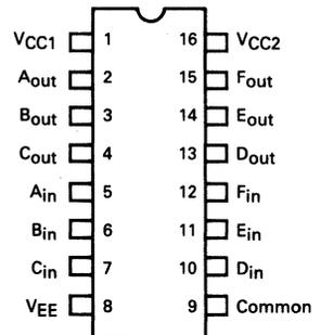
Pin assignment is for Dual-in-line Package.
