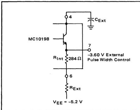
Figure 2 shows typical curves for pulse width versus  $C_{Ext}$  and  $R_{Ext}$  (total resistance includes  $R_{Int}$ ). Any low leakage capacitor can be used and  $R_{Ext}$  can vary from 0 to 16 k-ohms.
