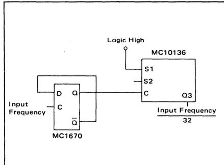
FIGURE 3 — 50 MHz PROGRAMMABLE COUNTER
