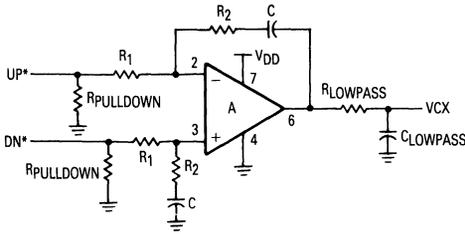
Figure 5-5A. Active Filter Using Op Amp
