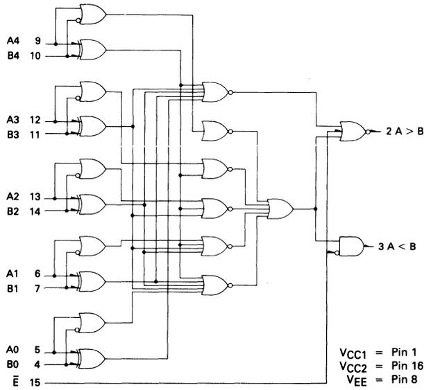
FIGURE 1 — 9-BIT MAGNITUDE COMPARATOR
