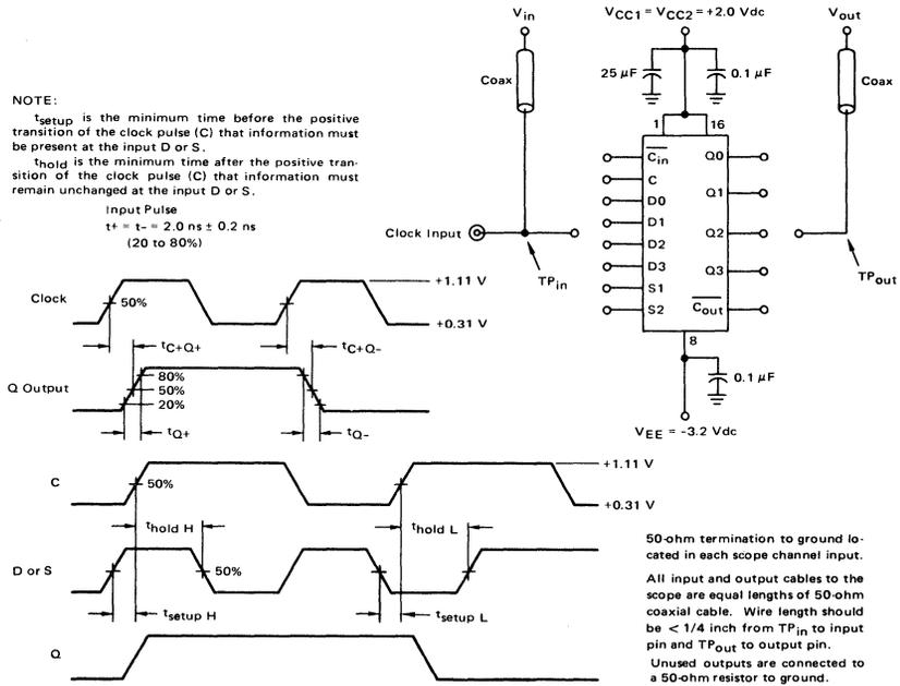
CARRY IN SET UP AND HOLD TIMES
