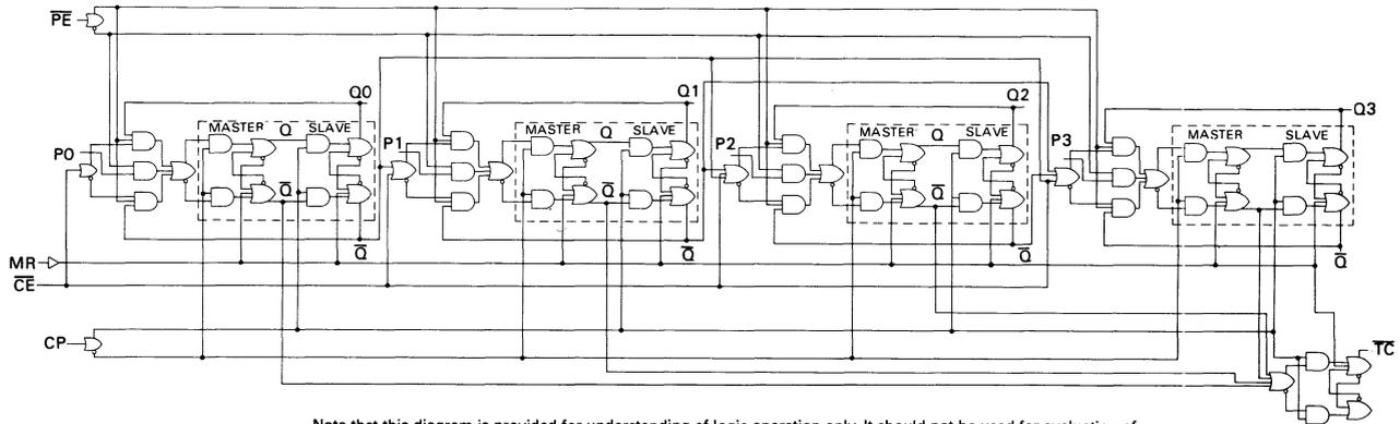
Note that this diagram is provided for understanding of logic operation only. It should not be used for evaluation of propagation delays as many gate functions are achieved internally without incurring a full gate delay.
