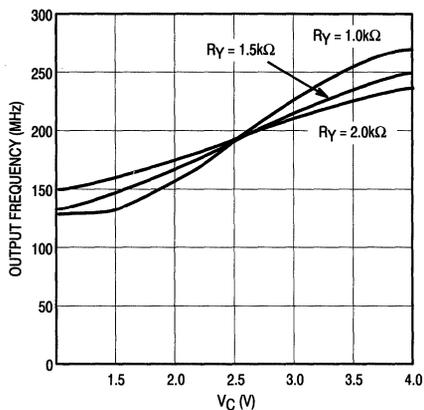
Figure 7.  $V_C$  versus Output Frequency
