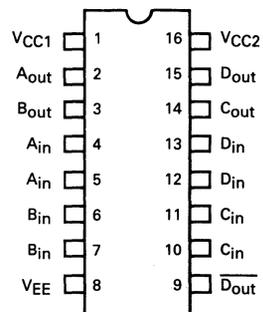
Pin assignment is for Dual-in-line Package.
