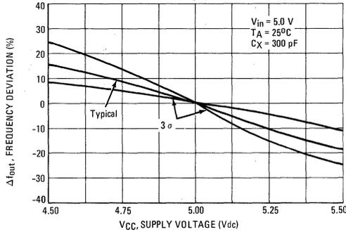
FIGURE 8 — TYPICAL FREQUENCY DEVIATION versus SUPPLY VOLTAGE
