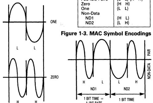
Figure 1-4. Phase-Coherent Modulation Scheme
