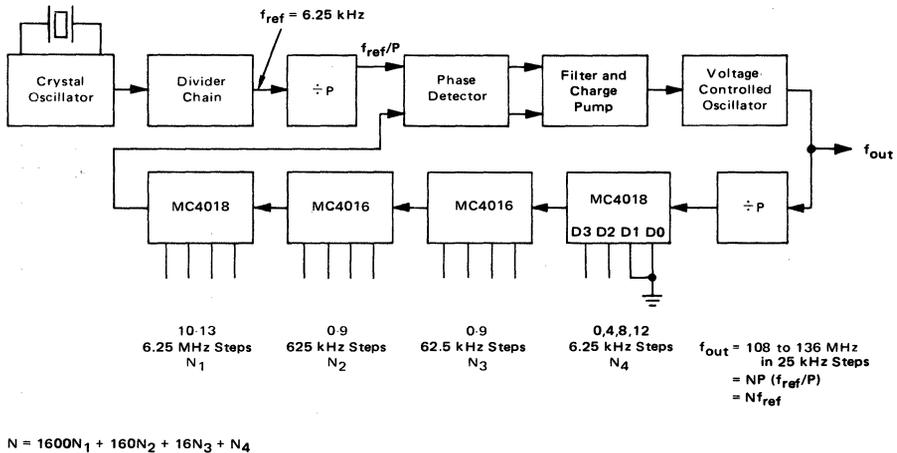
Figure 11 shows the FM band implemented with the MC4016 and has a 100 kHz reference frequency. The MC4316/4016 covers phase-locked loop applica-
