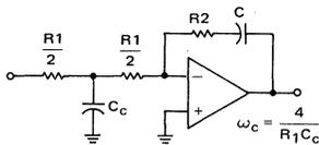
FIGURE 16 — IMPROVED TRANSIENT SUPPRESSION WITH  $R2 - C_c$
