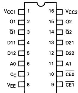
Pin assignment is for Dual-in-line Package.
