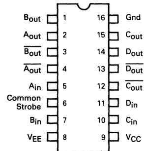
Pin assignment is for Dual-in-line Package.
