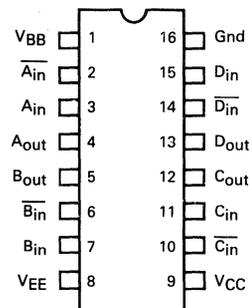
Pin assignment is for Dual-in-line Package.
