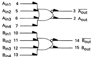
$$\text{out} = \text{in1} + \text{in2} + \text{in3} + \text{in4}$$
