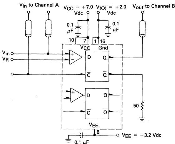
50 ohm termination to ground located in each scope channel input.
