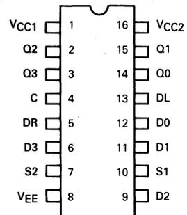
Pin assignment is for Dual-in-line Package. For PLCC pin assignment, see tables on page 1-35.
