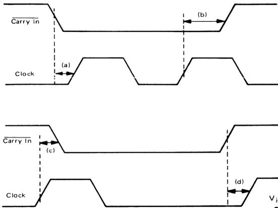
(a) is the minimum time to wait after the counter has been enabled to clock it.
