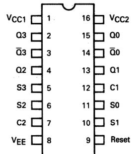
Pin assignment is for Dual-in-line Package.
