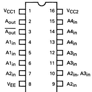
Pin assignment is for Dual-in-line Package.
