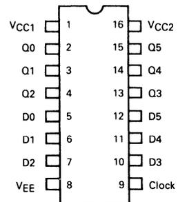
Pin assignment is for Dual-in-line Package.
