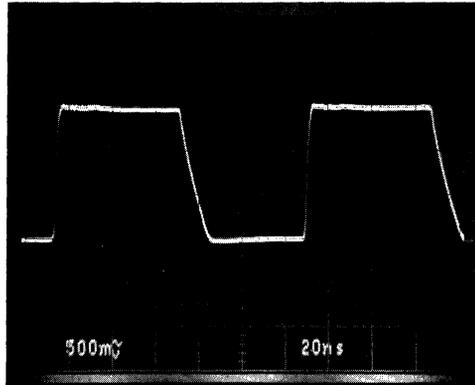
FIGURE 2B — ÷ 128, 1.1 GHz, 5.0 V, +25°C, OUTPUT LOADED
