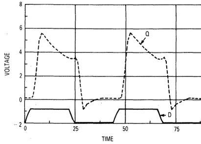
*Example 2.* In a memory system application, use of an external source resistor is suggested. Simulations run with  $RS = 8\Omega$  and  $CL = 300 \text{ pF}$  leads to clean waveforms both at the output, Q, and at point Qp:
