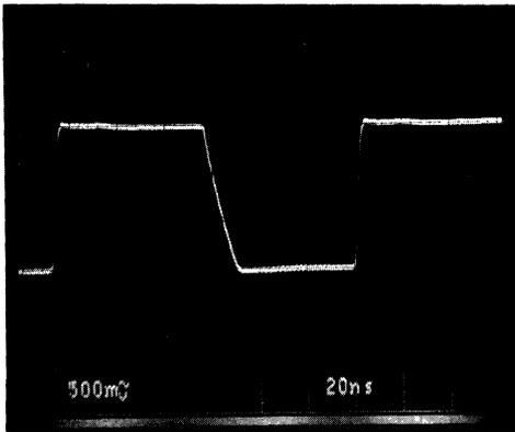
FIGURE 2A — ÷64, 500 MHz, 5.0 V, +25°C, OUTPUT LOADED
