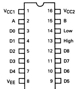
Pin assignment is for Dual-in-line Package.
