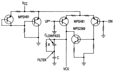
Figure 5-5B. Charge Pump/Filter
