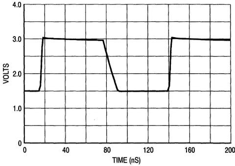
Figure 3. -64, 500 MHz, 5.0 V, +25°C, Output Loaded
