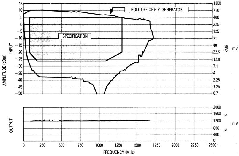
Figure 1. MC12078 Input Signal Amplitude versus Input Frequency
