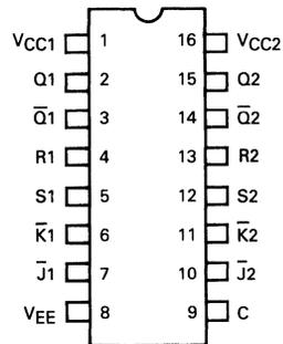
Pin assignment is for Dual-in-line Package. For PLCC pin assignment, see tables on page 1-35.
