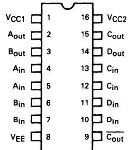
Pin assignment is for Dual-in-line Package.
