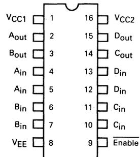
Pin assignment is for Dual-in-line Package.
