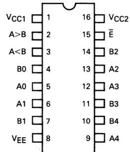
Pin assignment is for Dual-in-line Package.
