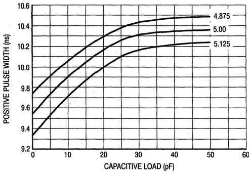
Figure 3. MC10H642 Positive PW versus Load
