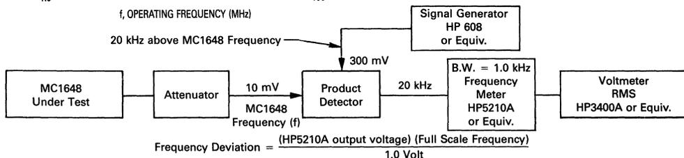
NOTE: Any frequency deviation caused by the signal generator and MC1648 power supply should be determined and minimized prior to testing.
