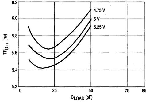
Figure 7. TP versus Load Typical at  $T_A = 25^\circ\text{C}$
