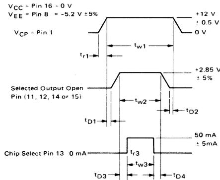
The timing diagram is shown for programming one bit. Note that only one bit is blown at a time. All addressing must be done 100 ns prior to the beginning of the  $V_{CP}$  pulse, i.e.,  $V_{CP} = 0 V$ . Likewise, strobing of the outputs to determine success in programming should occur no sooner than 100 ns after  $V_{CP}$  returns to 0 V.
