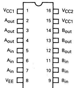
Pin assignment is for Dual-in-line Package.
