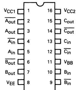
Pin assignment is for Dual-in-line Package.
