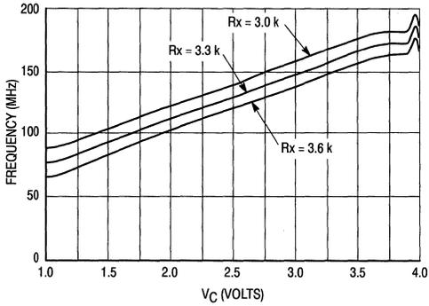
**Figure 6.  $V_C$  versus Output Frequency**
