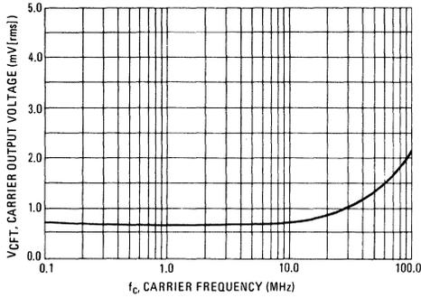
FIGURE 4 — CARRIER FEEDTHROUGH VERSUS FREQUENCY (Test 2)
