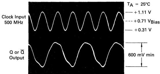
The maximum toggle frequency of the MC1690 has been exceeded when either:
