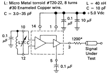
\*The 1200 ohm resistor and the scope termination impedance constitute a 25:1 attenuator probe. Coax shall be CT-070-50 or equivalent.
