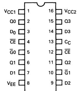
Pin assignment is for Dual-in-line Package.
