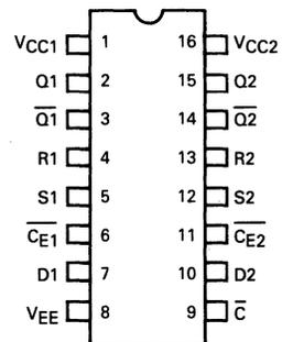
Pin assignment is for Dual-in-line Package.
