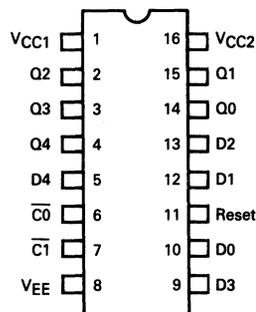
Pin assignment is for Dual-in-line Package.
