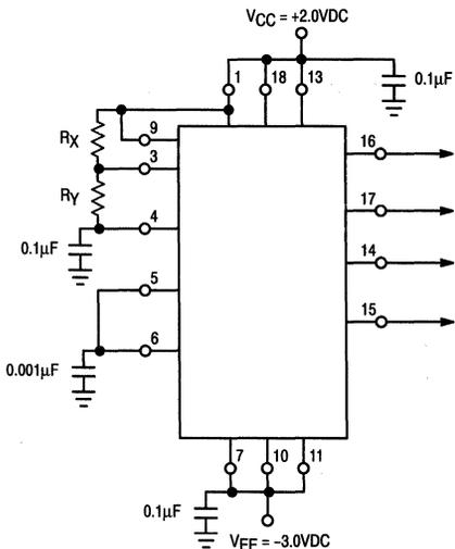
Figure 3. AC Test Circuit (FO/t<sub>RE</sub>/t<sub>FE</sub> Measurement)
