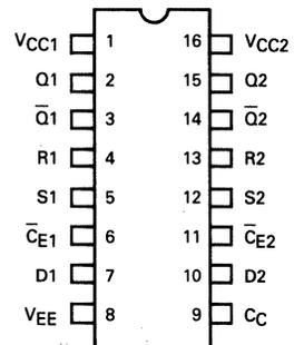
Pin assignment is for Dual-in-line Package.
