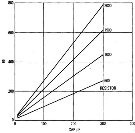
Figure 9-3. One Shot Pulse Width versus Rext/Cext
