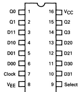
Pin assignment is for Dual-in-line Package.
