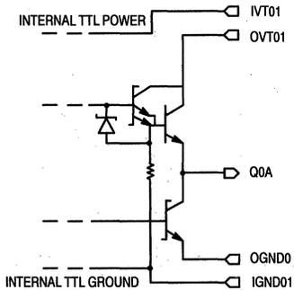
Figure 1. Output Structure
