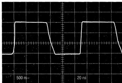
FIGURE 2B — +128, 1.1 GHz, 5.0 V, +25°C, OUTPUT LOADED
