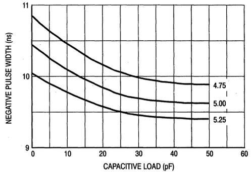
Figure 2. MC10H642 Negative PW versus Load
