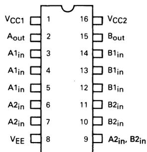
Pin assignment is for Dual-in-line Package.
