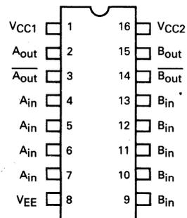
Pin assignment is for Dual-in-line Package.
