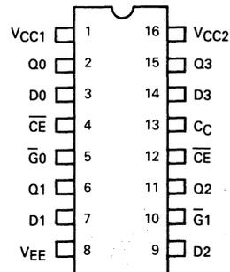
Pin assignment is for Dual-in-line Package.
