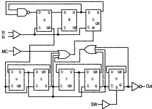
Figure 1. Logic Diagram (MC12022TVA)
