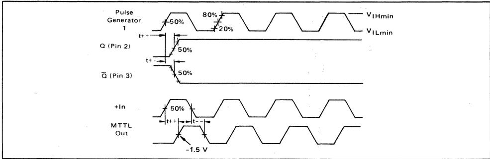
FIGURE 4 – SETUP AND RELEASE TIME WAVEFORMS
