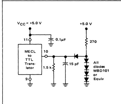
FIGURE 12 — NOISE MEASUREMENT TEST CIRCUIT
