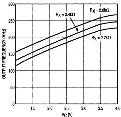
Figure 6.  $V_C$  versus Output Frequency
