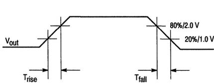
Figure 3. WAVEFORMS: Rise and Fall Times
