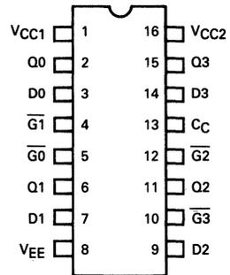
Pin assignment is for Dual-in-line Package.
