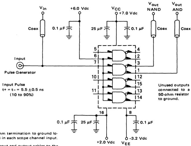
NOTE: All power supply and logic levels are shown shifted 2 volts positive.
