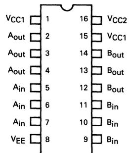
Pin assignment is for Dual-in-line Package.
