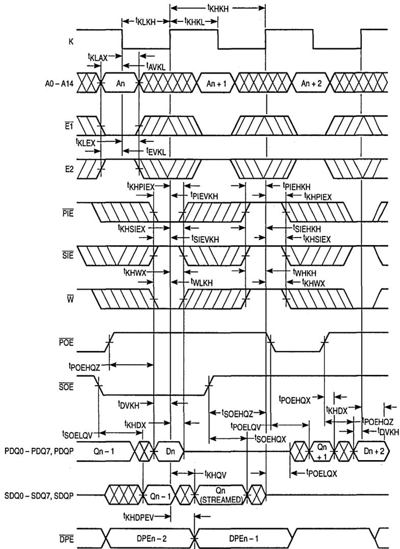
NOTE:  $\overline{DPE}$  is valid exactly one clock cycle after the output data is written.
