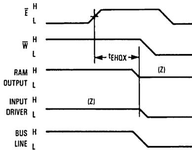
Figure 2c. Using  $\bar{E}$  to Avoid Bus Contention
