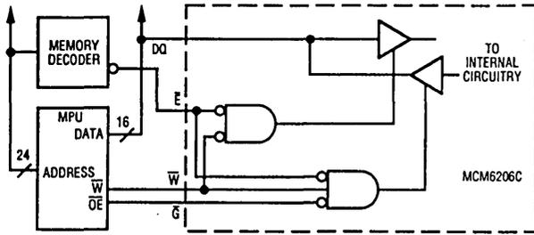
Figure 4a. Using  $\bar{G}$  to Avoid Bus Contention
