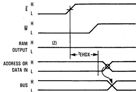
Figure 3c. Using  $\bar{E}$  to Avoid Bus Contention
