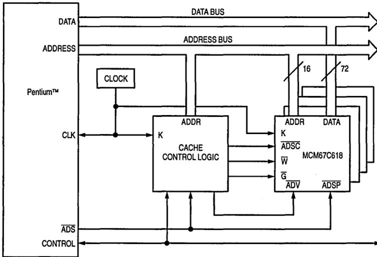
512K BYTE BURSTABLE, SECONDARY CACHE USING
