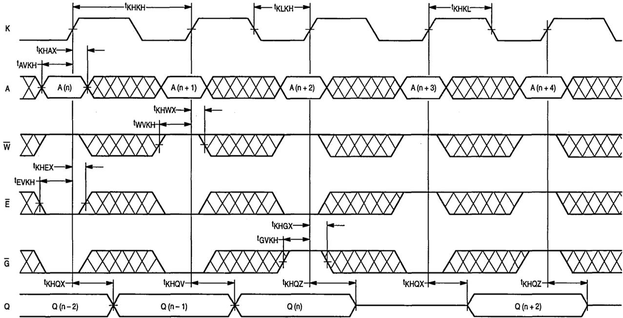
WRITE AND DATA PASS-THROUGH CYCLE TIMING
