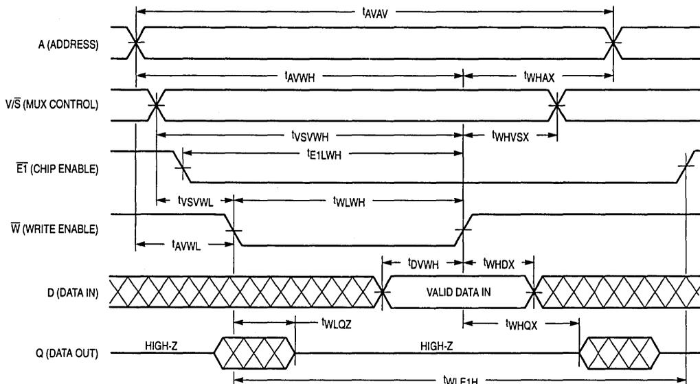
**WRITE CYCLE TIMING** (Chip Enable Initiated, See Note 1)
