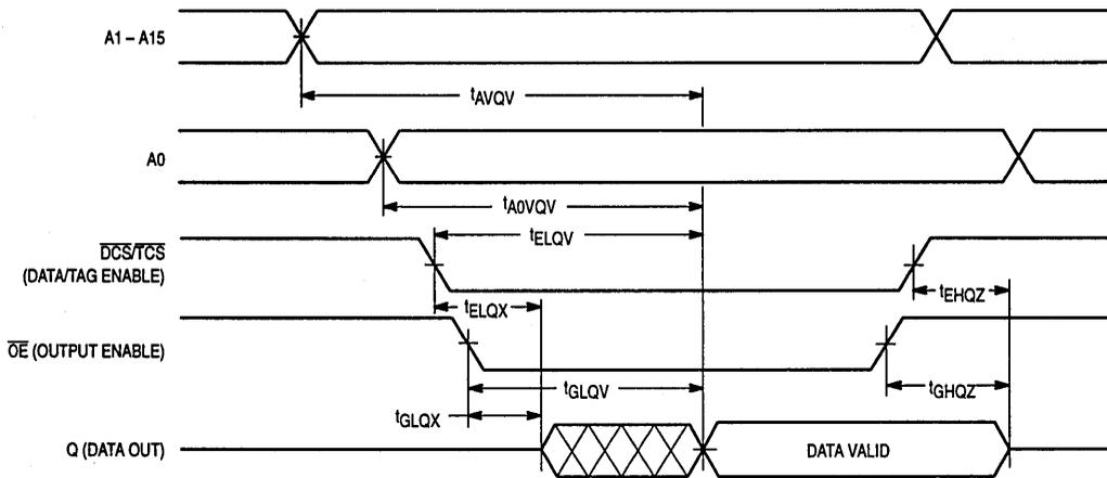
NOTE: Address valid prior to or coincident with  $\overline{DCS}$  or  $\overline{TCS}$  going low.
