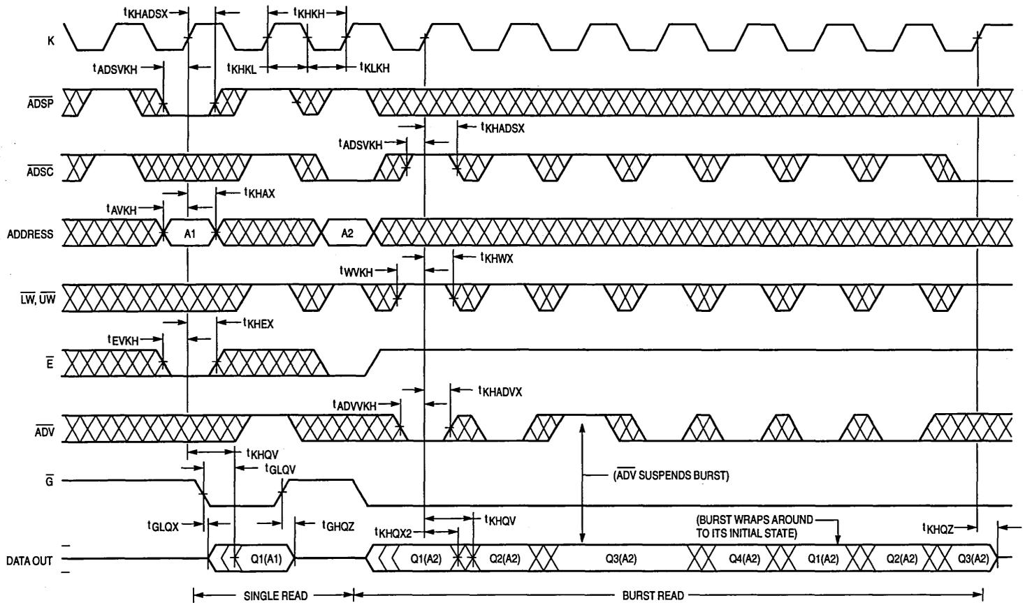
NOTE: Q1(A2) represents the first output data from the base address A2; Q2(A2) represents the next output data in the burst sequence with A2 as the base address.
