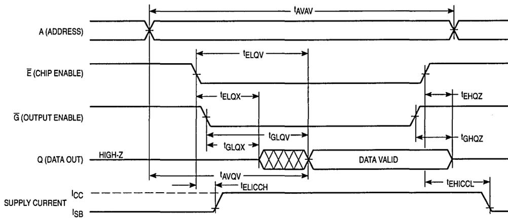
NOTE: Addresses valid prior to or coincident with  $\bar{E}$  going low/ $\bar{E}$  going high.
