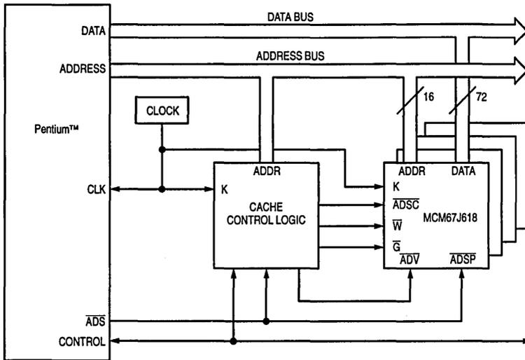
512K BYTE BURSTABLE, SECONDARY CACHE USING
