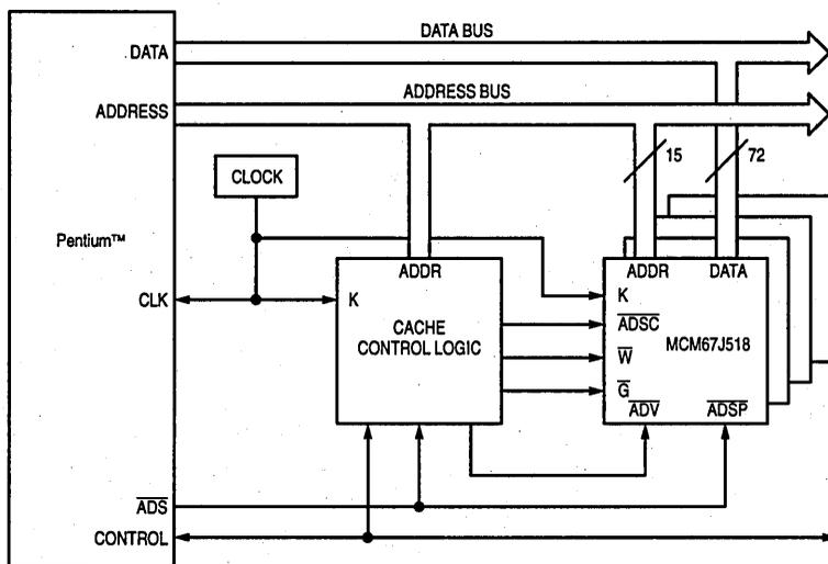
256K BYTE BURSTABLE, SECONDARY CACHE USING
