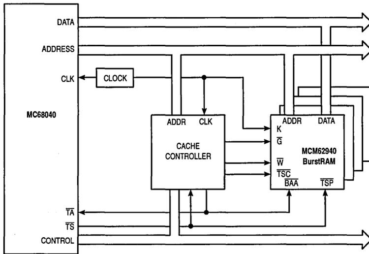
Figure 6. MC68040 128K Byte Burstable Cache Memory Block Diagram
