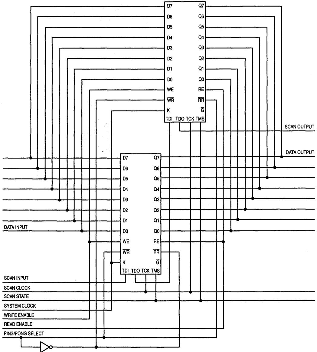
Figure 8. "Ping-Pong" Synchronizing Buffer (8192 Pixels Maximum)
