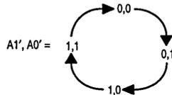
NOTE: The external two values for A1 and A0 provide the starting point for the burst sequence graph. The burst logic advances A1 and A0 as shown above.
