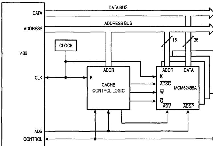
128K BYTE BURSTABLE, SECONDARY CACHE USING
