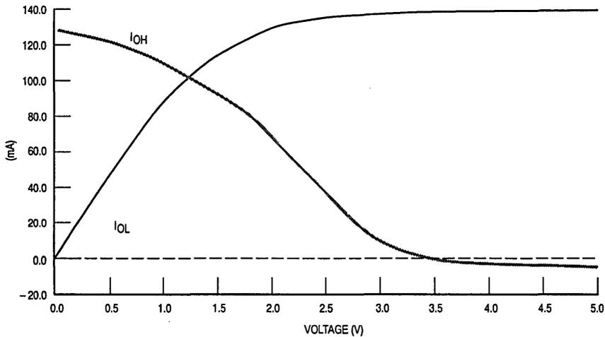
**Figure 7.  $I_{OL}/I_{OH}$  Output Buffer Characteristics ( $I_{out}$  vs  $V_{out}$ ) for MCM67A518, MCM67B518, MCM67C518, MCM67H518, MCM67J518, MCM67M518, MCM67W518, MCM67A618, MCM67B618, MCM67C618, MCM67H618, MCM67J618, MCM67M618, MCM67W618**
