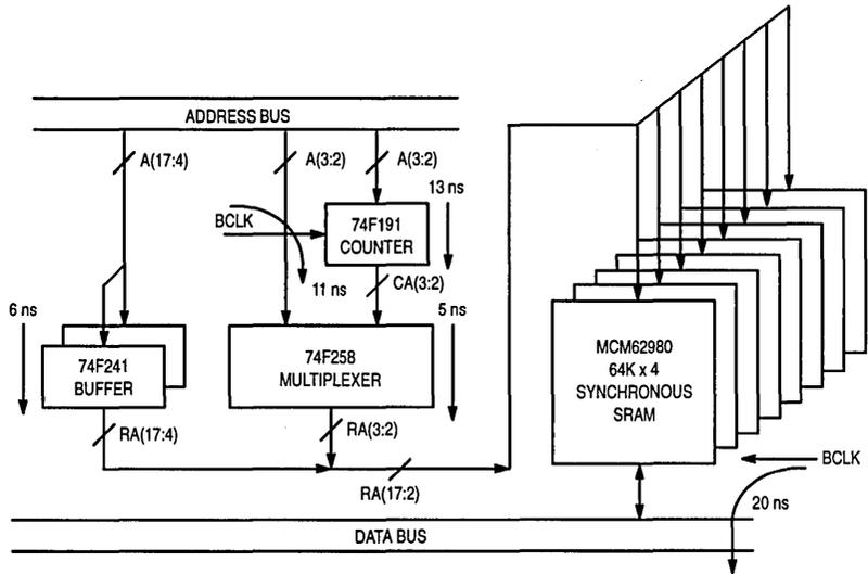
Figure 2. Burstable 64K x 32 Memory Array
