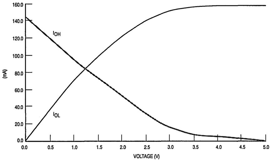
**Figure 6.  $I_{OL}/I_{OH}$  Output Buffer Characteristics ( $I_{out}$  vs  $V_{out}$ ) for MCM62110, MCM62486A, MCM62940A, MCM62990A, MCM62995A, MCM62996**
