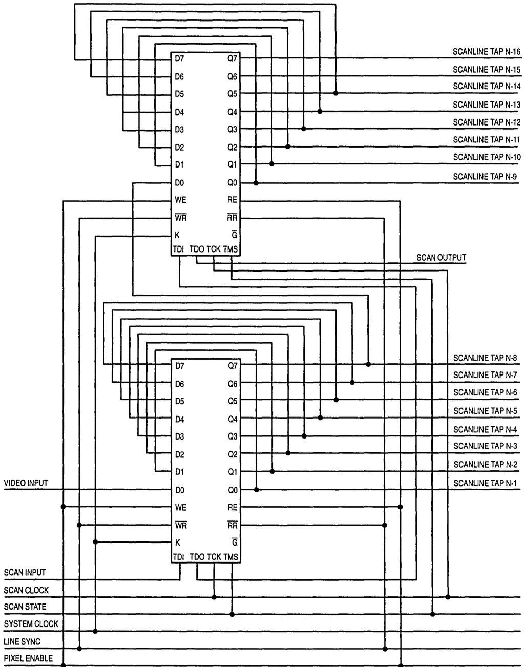
Figure 7. Multi-Stage 1-Bit Video Scanline Delay (8192 Pixels Maximum)
