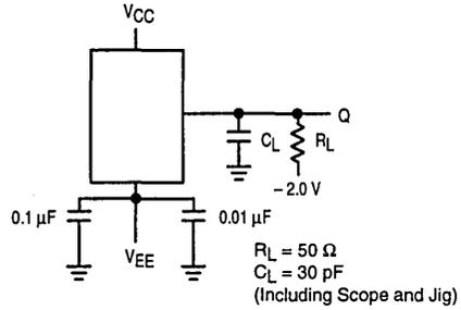
Figure 2. AC Test Circuit
