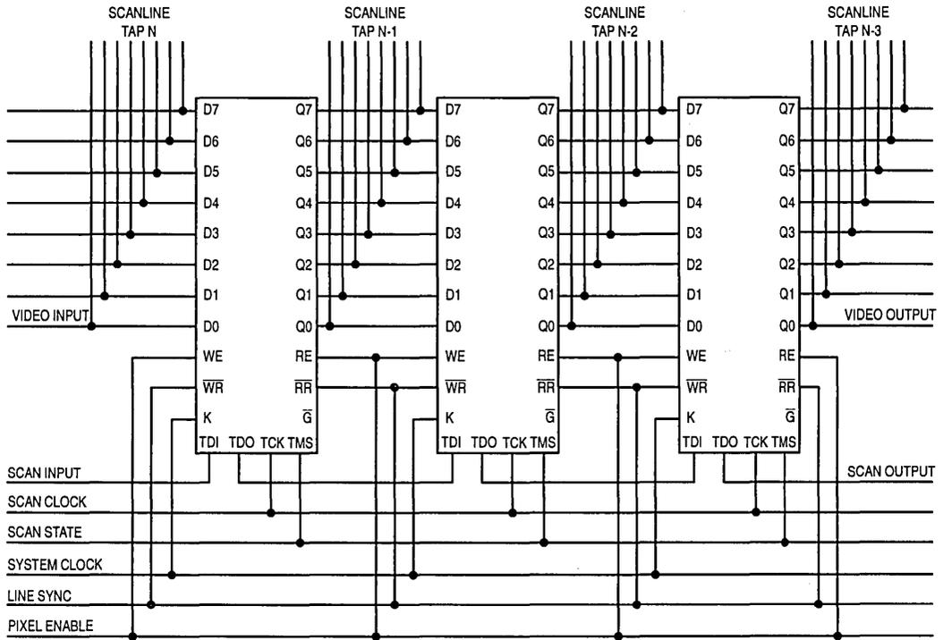
Figure 5. Multi-Stage 8-Bit Video Scanline Delay (8192 Pixels Maximum)
