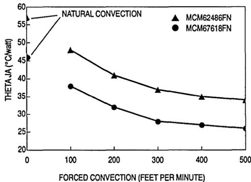
**44 and 52 Lead PLCC, Copper Leadframe, Single Layer PCB Simulated Results**
