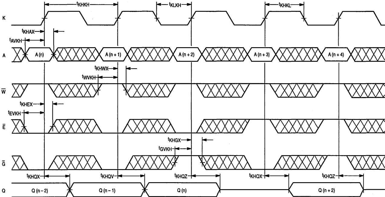
WRITE AND DATA PASS-THROUGH CYCLE TIMING
