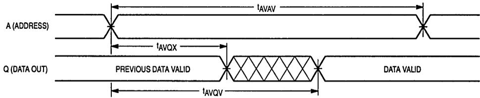
NOTE: Device is continuously selected ( $\bar{E} = V_{IL}$ ,  $\bar{G} = V_{IL}$ ).
