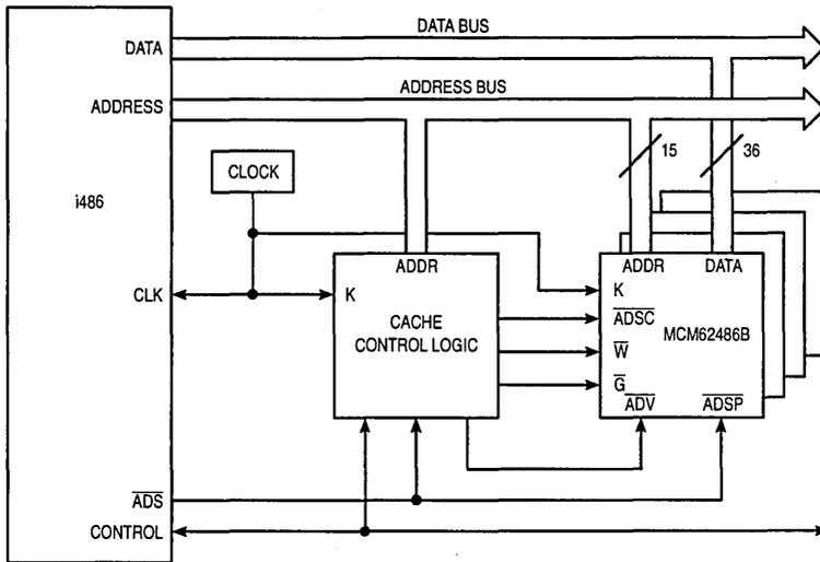
128K BYTE BURSTABLE, SECONDARY CACHE USING
