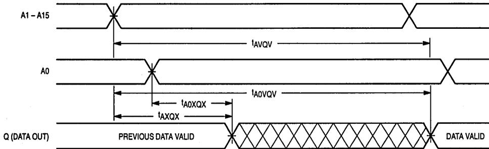
NOTE: Module is continuously selected ( $\overline{DCS}$  or  $\overline{TCS} = V_{IL}$ ,  $\overline{OE} = V_{IL}$ ).
