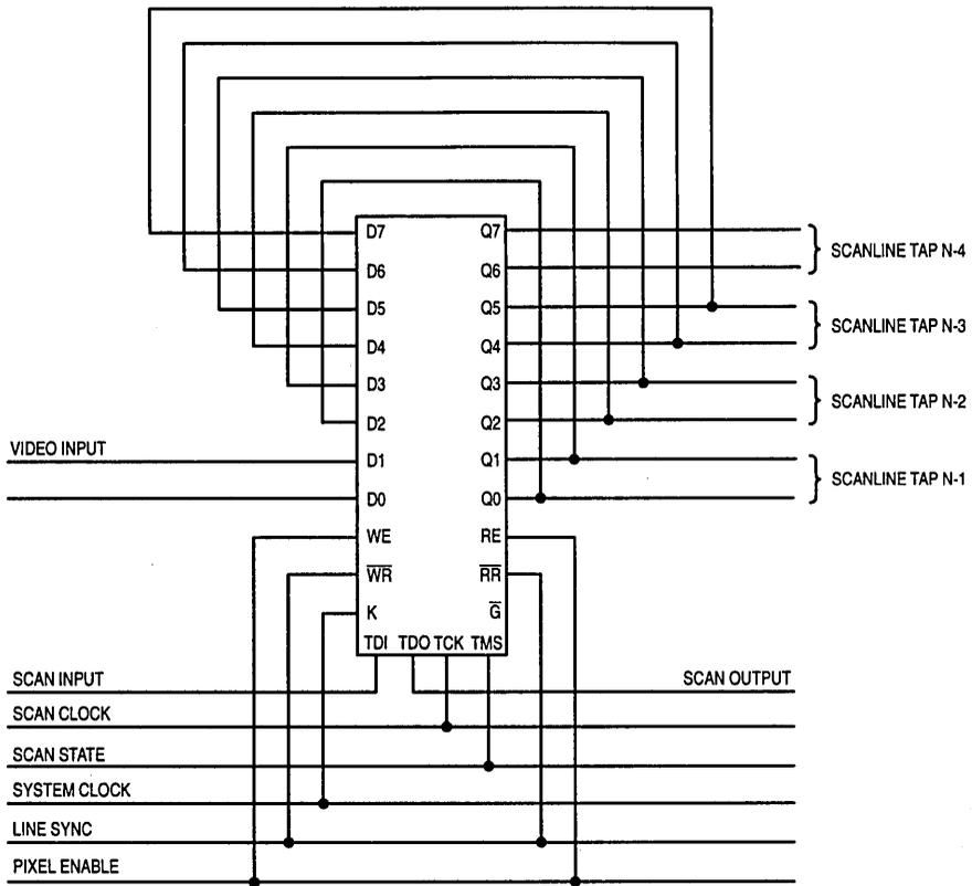
Figure 6. Multi-Stage 2-Bit Video Scanline Delay (8192 Pixels Maximum)
