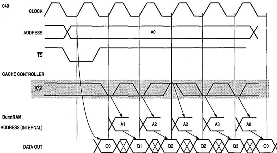
Figure 7. Timing Example of a 2/1/2/1 Burst Read
