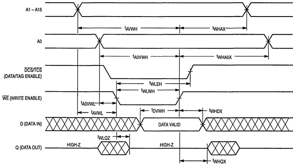
**WRITE CYCLE 2** ( $\overline{\text{DCS}}$  or  $\overline{\text{TCS}}$  Controlled, See Notes 1 and 2)
