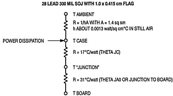
NOTE: Theta JA simulated in Natural Convection 77°C/watt.
