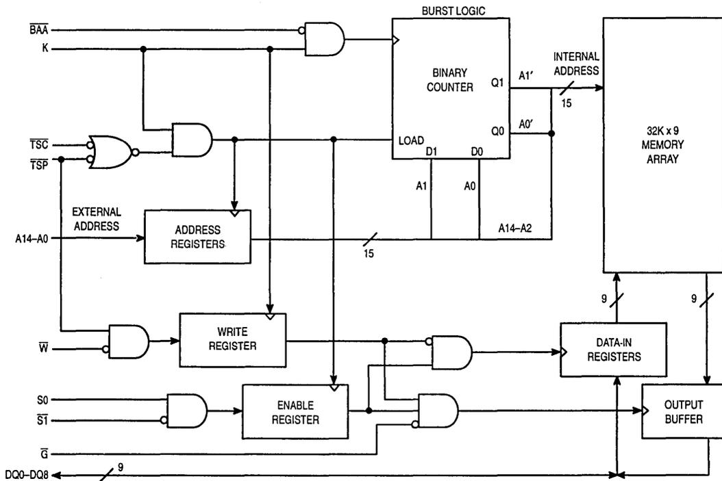
Figure 5. MCM62940A 32K x 9 BurstRAM Block Diagram
