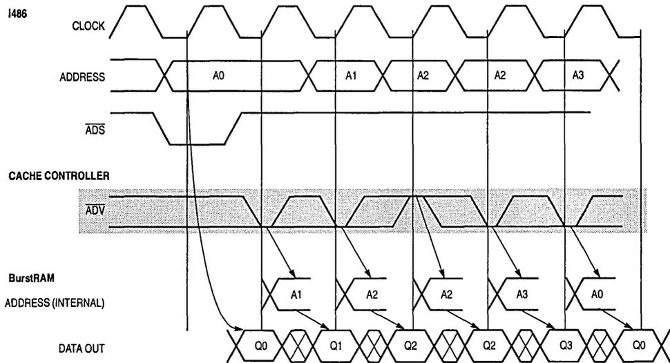
Figure 4. Timing Example of a 2/1/2/1 Burst Read
