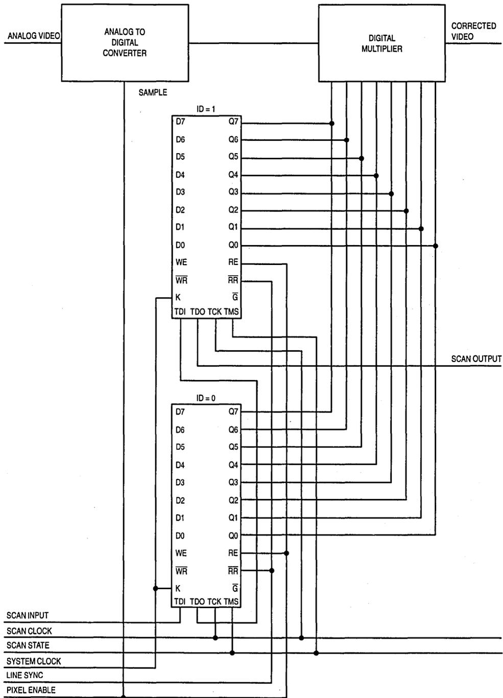
Figure 9. CCD Gain Correction, Buffer Written From Scan Input (16384 Pixels Maximum)
