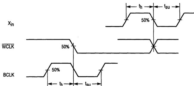
Figure 5.  $\overline{WCLK}$  Timing (All Modes Except  $DMODE = 1$ ,  $WDLY = 1$ )
