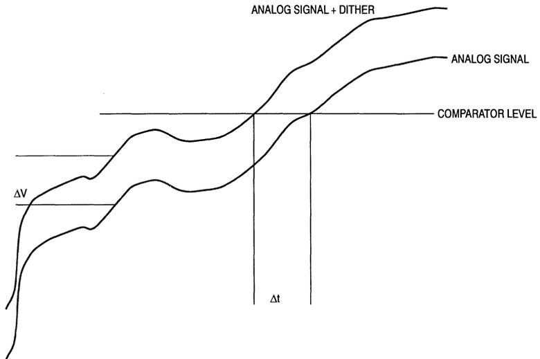
Figure 6. Amplitude Dithering
