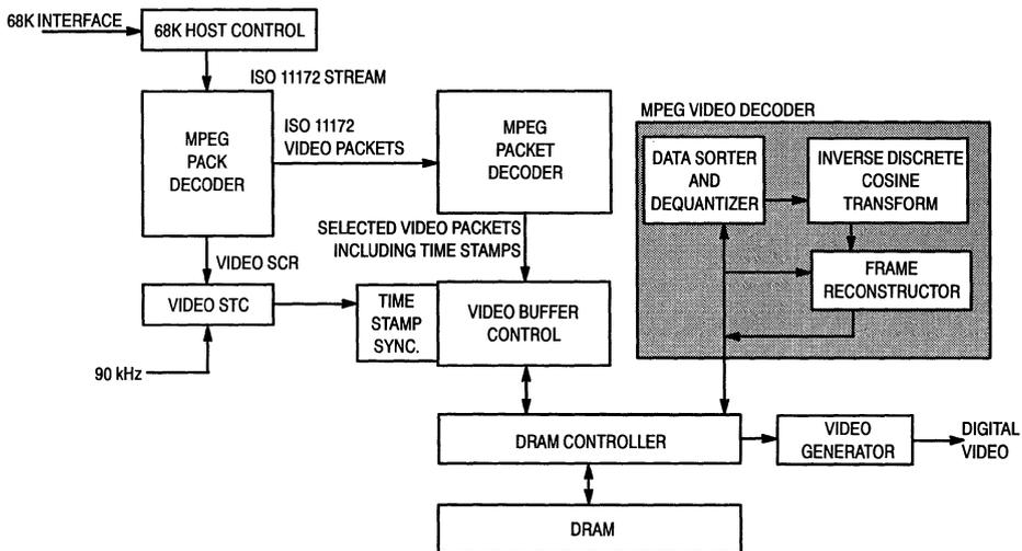
Figure 1. MCD251 Logical Data Flow and Synchronization Diagram
