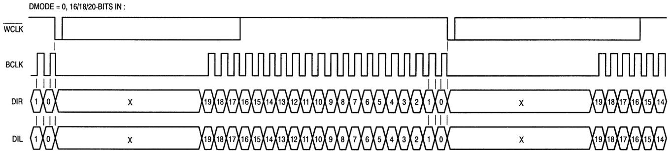
Figure 11. DMODE = 0 Serial Interface Timing Diagram
