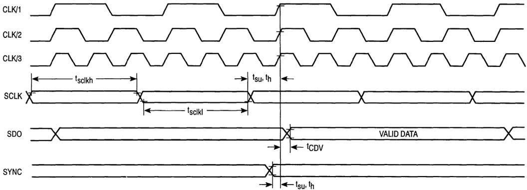
Figure 9. Serial Interface Timing (Slave Mode: ISLAV = 1)
