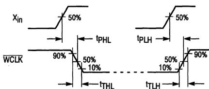
Figure 3.  $\overline{WCLK}$  Out Propagation Delay Timing (Master Mode)
