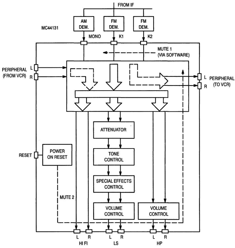
Figure 3. Input/Output Combinations
