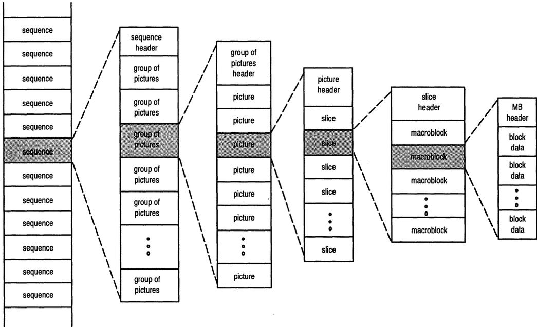
Figure 12. Typical composition of MPEG bit stream
