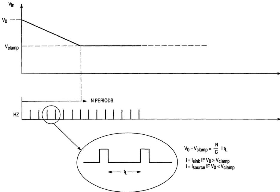
Figure 4. Clamp Network Timing Diagram — Power Up
