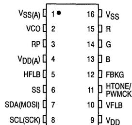
This is a high performance HCMOS device designed to interface with a microcontroller unit to allow colored symbols or characters to be displayed on a color monitor. Its on-chip PLL allows both multisystem operation and self generation of system timing. It also minimizes the MCU's burden through its built-in 493 bytes RAM. By storing a full screen of data and control information, this device has a capability to carry out 'screen-refresh' without any MCU supervision.
