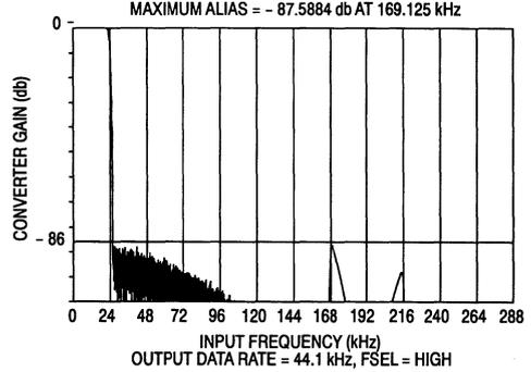
Figure 3. Digital Filter Response (Wideband)
