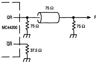
Figure 4. Resistive Load for  $V_{out} = 750 \text{ mV}$
