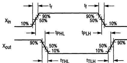
Figure 1.  $X_{out}$  Propagation Delay Timing
