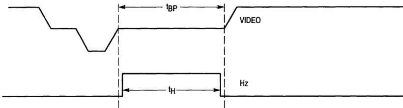
Figure 5. Horizontal Timing
