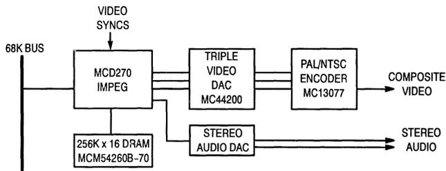
Figure 1. Typical MPEG1 Video and Audio Decoder
