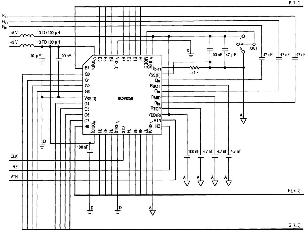
Figure 15. Application Circuit
