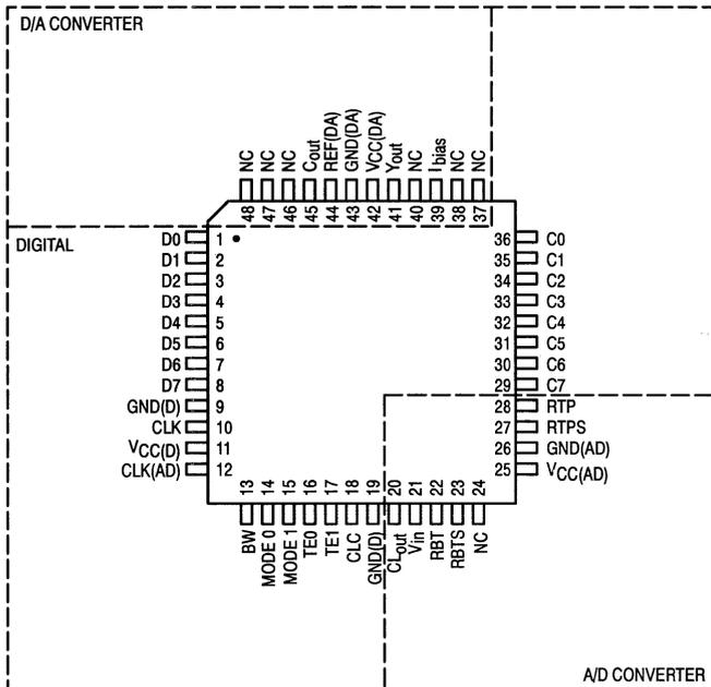
Figure 2. Pin Assignment
