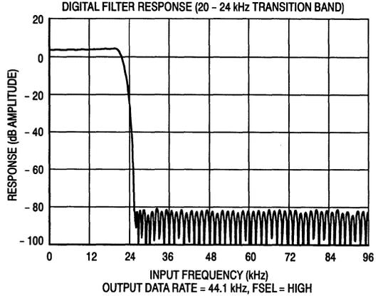
Figure 4. Digital Filter Response (Narrowband)
