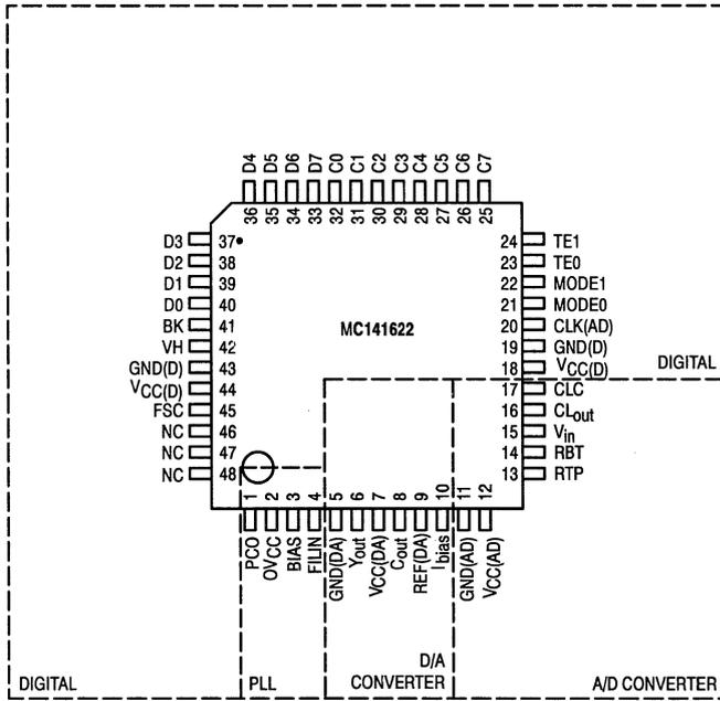
Figure 2. Pin Assignment
