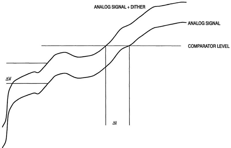
Figure 7. Amplitude Dithering
