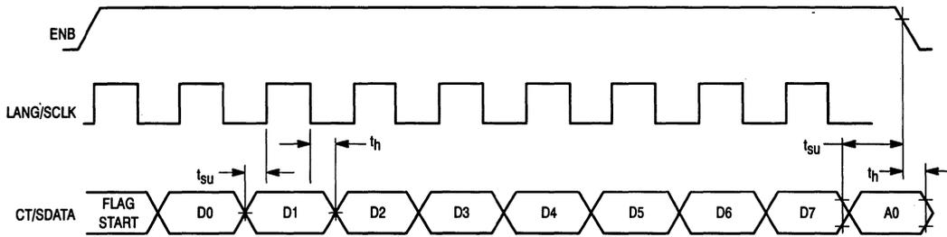
Figure 6. Timing Diagram for Serial Mode (Config = Low)
