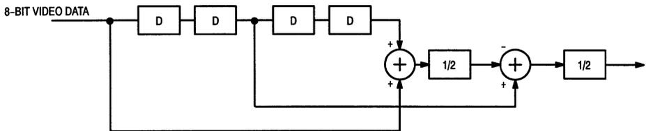
Figure 3. Horizontal Filter
