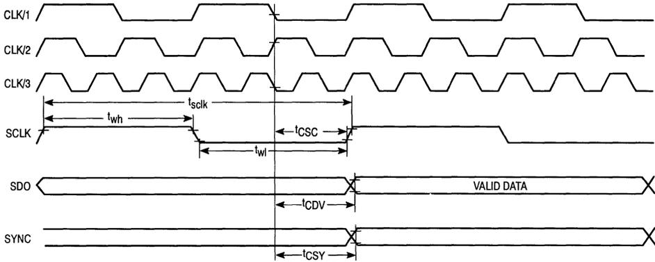
Figure 8. Serial Interface Timing (Master Mode: ISLAV = 0)
