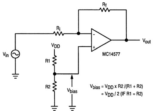
**Figure 8. DC-Coupled Inverting Amplifier with Single-Supply Operation**
