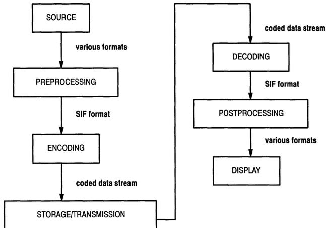
Figure 1. Compression/Decompression Process
