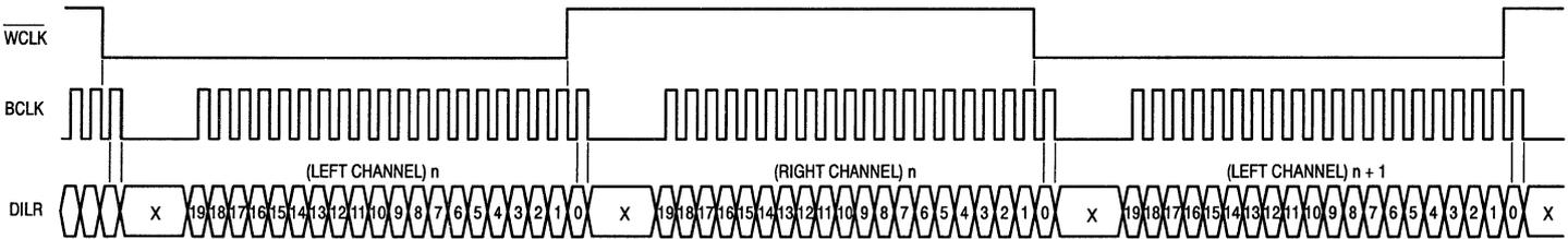
Figure 13. DMODE = 1, WDLY = 1, Serial Interface Timing Diagram
