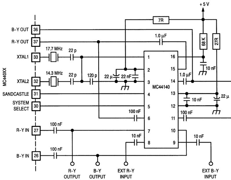
Figure 5. Application Circuit
