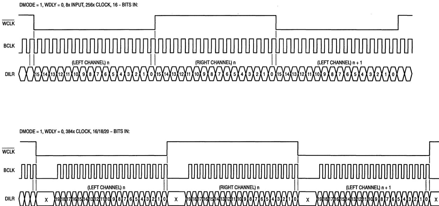
Figure 12. DMODE = 1, WDLY = 0, Serial Interface Timing Diagram
