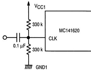
Figure 7. 200 mV p-p to 5.0 V p-p Sine Wave
