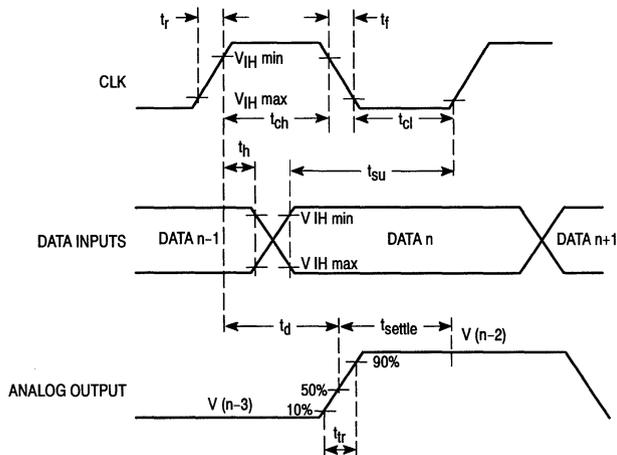
**Figure 1. Clock Input and Output Timing**
