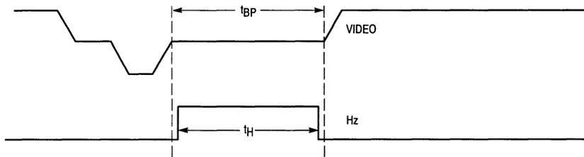
Figure 4. Horizontal Timing
