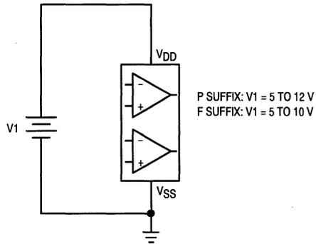
Figure 10. Single-Supply Operation
