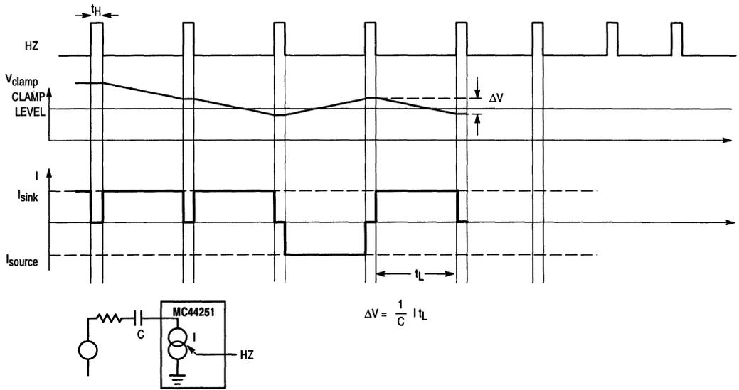
Figure 3. Clamp Network Timing Diagram — Operation
