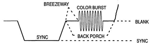
**Color Decoder** — This is the circuit in the video system that uses the chrominance portion of NTSC/PAL to derive the two color difference signals. The color decoder sits right after the Y/C separator and before the color space converter. The color decoder needs a 3.58 MHz (NTSC) or 4.43 MHz (PAL) signal that is accurately phase-locked to the color burst. If it isn't locked well enough, then the color decoder can't figure out the right colors. Also called a chroma demodulator.
