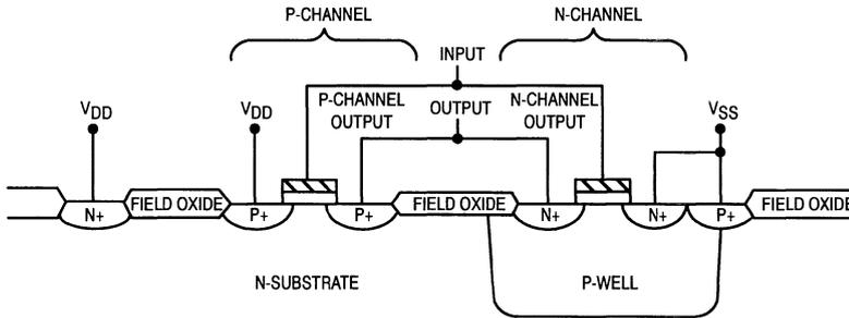
Figure 4. Latch Up Circuit Schematic
