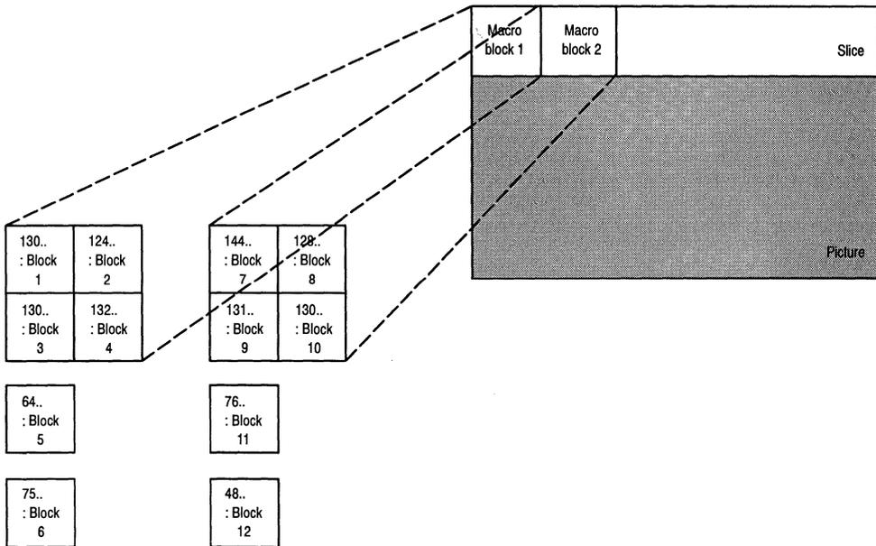
Figure 6. Coding the DC Coefficient Index in I-Pictures
