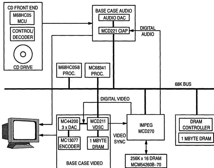
Figure 4. IMPEG/CD-i Architecture
