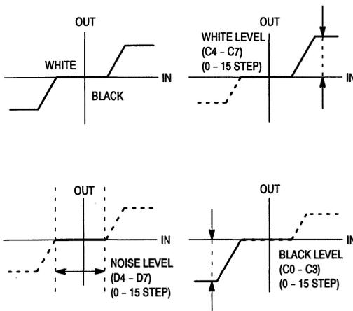
**Figure 3. Coring Characteristics**
