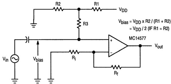
**Figure 6. AC-Coupled Noninverting Amplifier with Single-Supply Operation**
