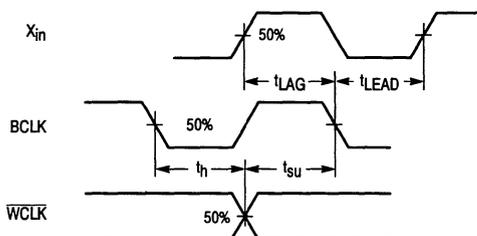
Figure 6.  $\overline{WCLK}$  Timing ( $DMODE = 1$ ,  $WDLY = 1$ )
