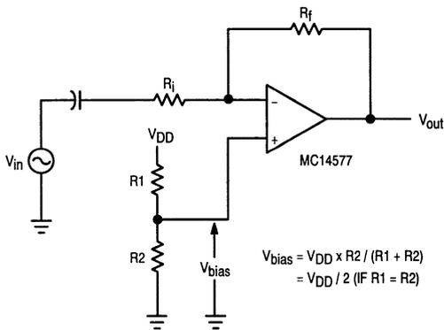
**Figure 7. AC-Coupled Inverting Amplifier with Single-Supply Operation**
