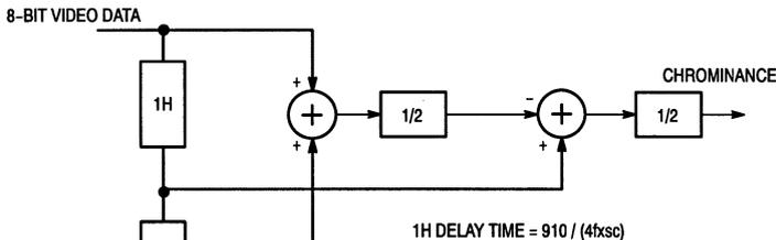
Figure 2. Vertical Filter
