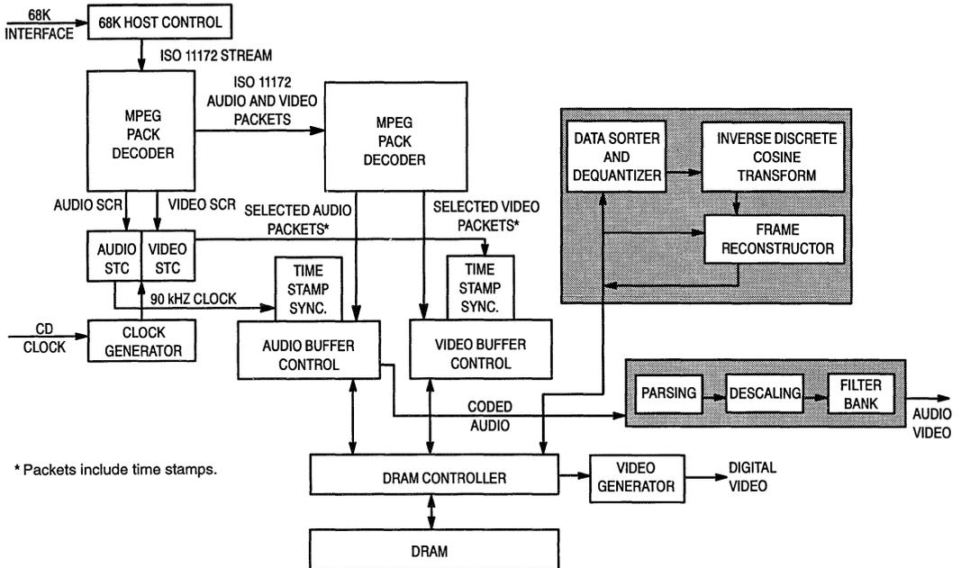
Figure 3. MCD270 Logical Data Flow and Synchronization Diagram
