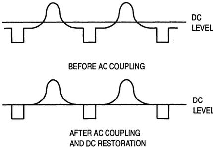
You can see in the figure that not knowing the dc offset means that we don't know exactly where the video signal is. One way to find the signal is to remove the dc offset by ac coupling, and then do dc restoration to add a known dc offset (one that we selected). Another reason ac coupling is important is that it can remove harmful dc offsets.
