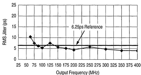
Figure 8. RMS Jitter versus Output Frequency
