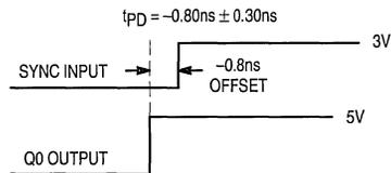
Figure 2. Depiction of the Fixed SYNC to Q0 Offset (t<sub>PD</sub>) Which Is Present When a 1MΩ Resistor Is Tied to V<sub>CC</sub> or Ground
