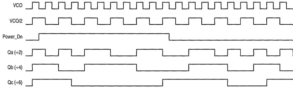
Figure 3. Power\_Dn Timing Diagram
