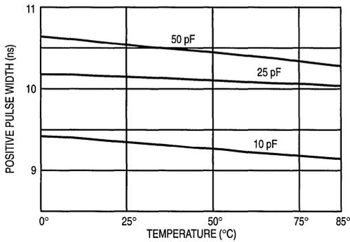
**Figure 5. Temperature versus Positive Pulse Width for 100H640 at 50 MHz and +5.0 V VCC**
