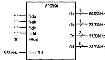
Figure 3. Dual Frequency Configuration
