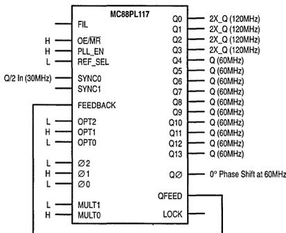
**Figure 3. Output Frequency Configuration 3**
