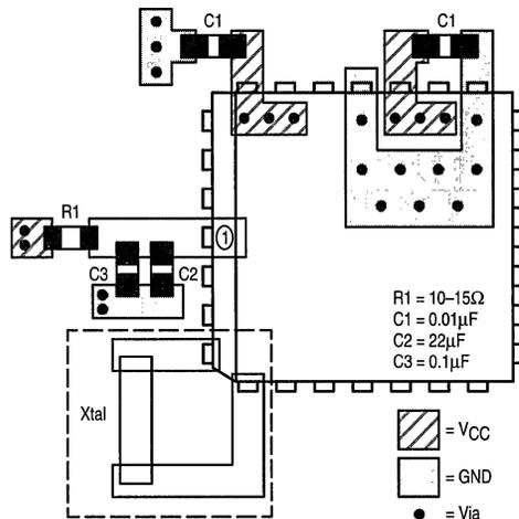
**Figure 4. PCB Board Layout for MC12430**
