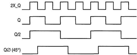
Figure 10. 88PL117 Output Waveforms
