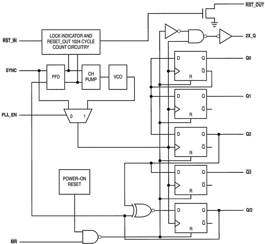
Figure 1. MC88916 Logic Block Diagram
