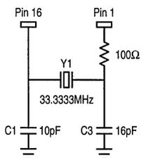
**Figure 3. Crystal Oscillator Interface (Fundamental)**
