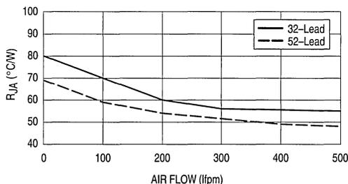
Figure 1. Thermal Resistance of the TQFP Packages
