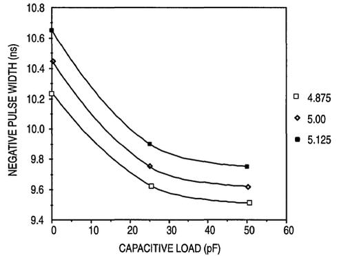
Figure 4. MC10H642 Negative PW versus Load
