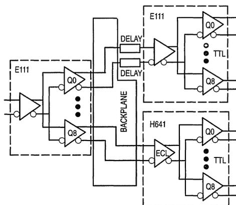
Figure 9. Mixed ECL and TTL Distribution
