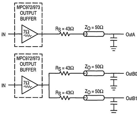
**Figure 9. Single versus Dual Transmission Lines**
