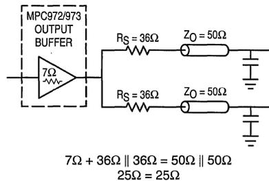
**Figure 11. Optimized Dual Line Termination**
