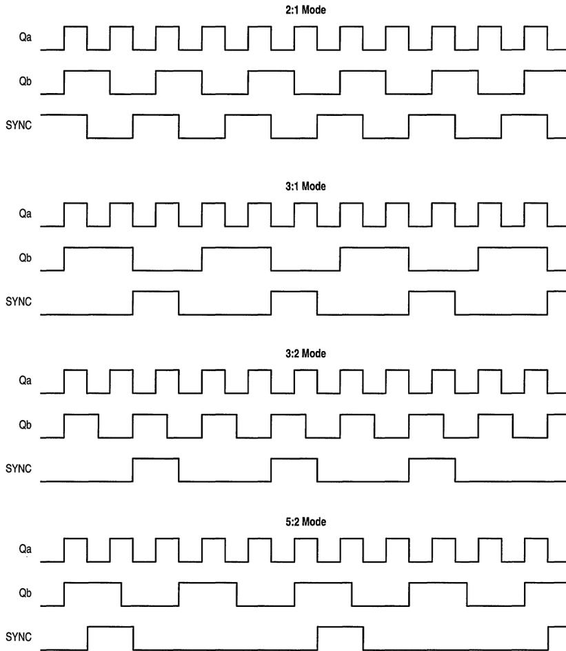
Figure 1. Output Waveforms
