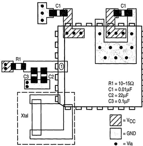
Figure 6. PCB Board Layout for MC12439
