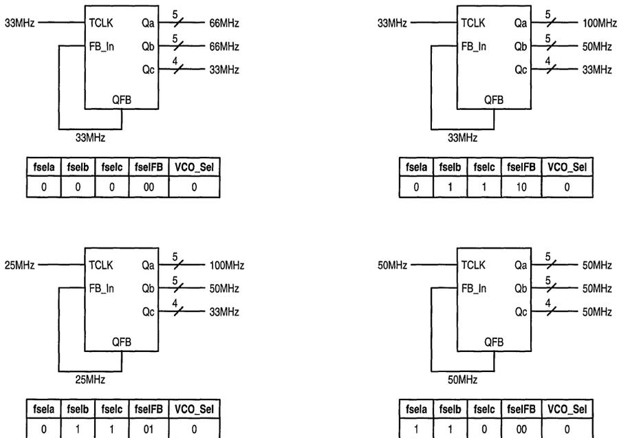
Figure 3. MPC974 Programming Schemes
