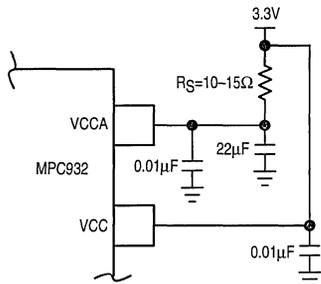
Figure 3. Power Supply Filter
