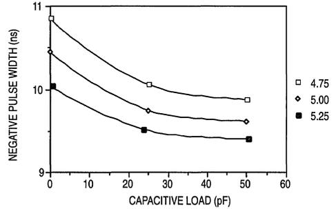
Figure 2. MC10H642 Negative PW versus Load
