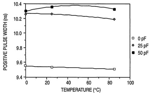
Figure 5. MC10H642 Positive PW versus Temperature,
