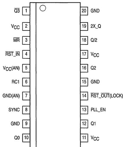
Pinout: 20-Lead Wide SOIC Package (Top View)
