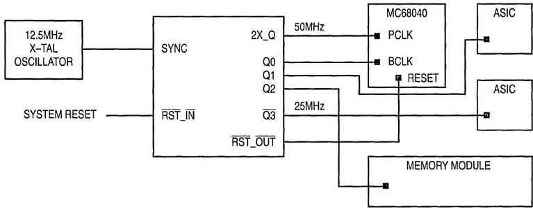
Figure 8. Typical MC88920/MC68040 System Configuration
