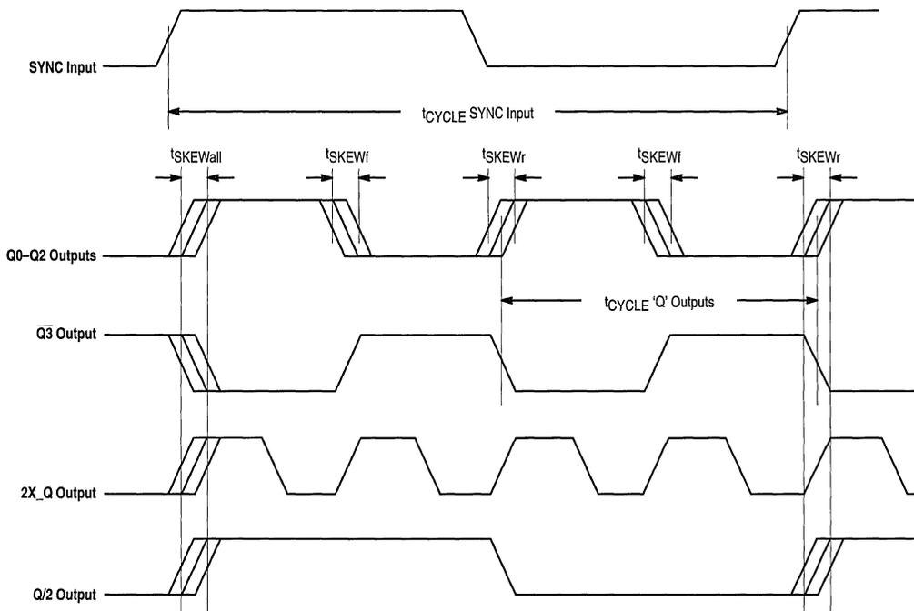
Figure 6. Output/Input Switching Waveforms and Timing Relationships
