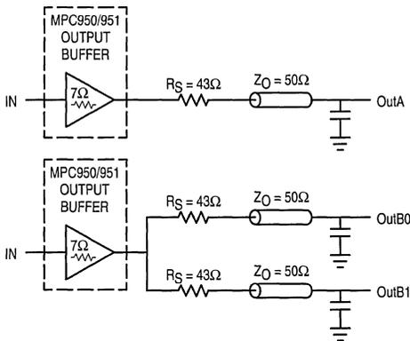
Figure 12. Single versus Dual Transmission Lines
