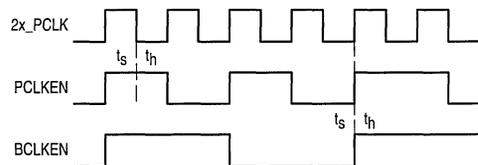
**Figure 13. MPC601 Setup and Hold Times**
