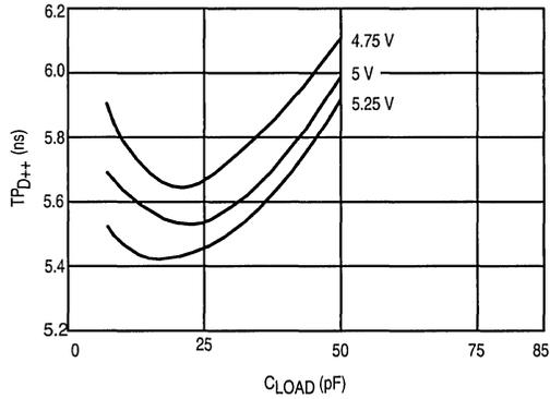
Figure 7. TP versus Load Typical at  $T_A = 25^\circ\text{C}$
