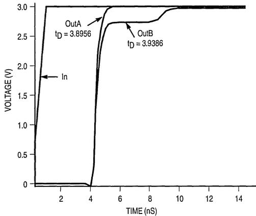
Figure 13. Single versus Dual Waveforms
