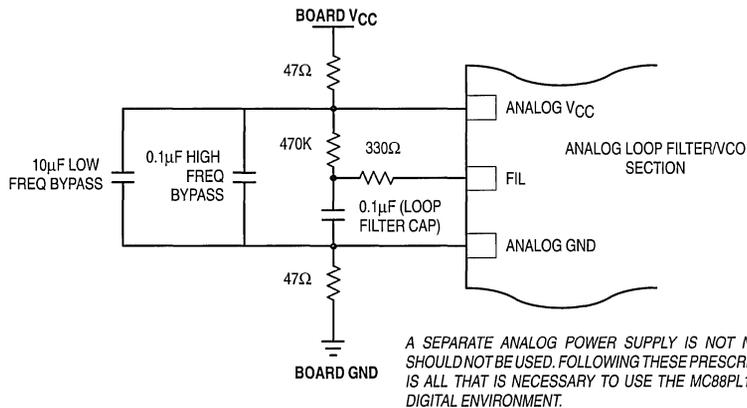
Figure 12. Recommended Loop Filter and Analog Isolation Scheme
