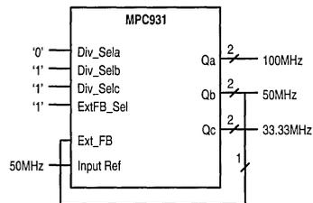
Figure 8. "Zero" Delay Fractional Divider
