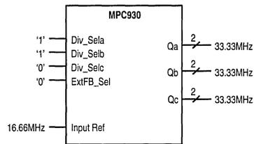
Figure 6. Single Frequency Configuration
