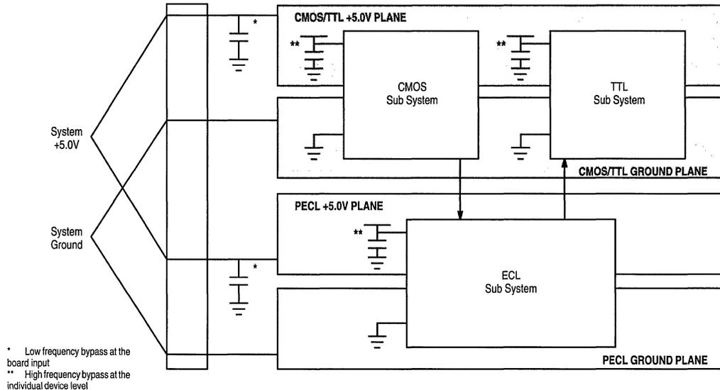
Figure 5. Power Plane Isolation in Mixed Logic Systems
