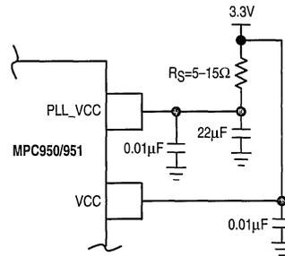
Figure 10. Power Supply Filter
