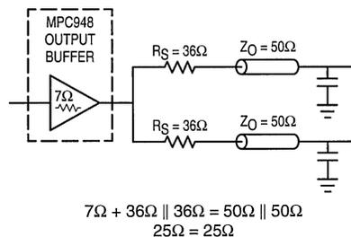
Figure 6. Optimized Dual Line Termination
