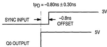
Figure 2. Depiction of the Fixed SYNC to Q0 Offset (t<sub>PD</sub>) Which Is Present When a 470KΩ Resistor Is Tied to V<sub>CC</sub> or Ground
