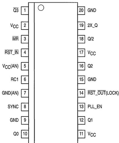
Pinout: 20-Lead Wide SOIC Package (Top View)
