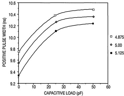
Figure 3. MC10H642 Positive PW versus Load
