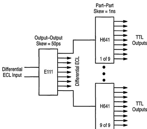
Figure 2. Low Skew Clock Fanout Tree
