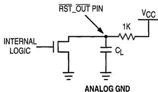
Figure 3. RST\_OUT Test Circuit
