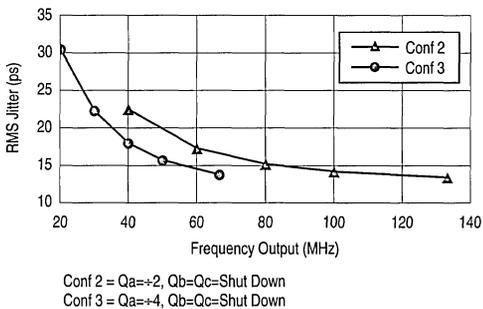
**Figure 13. RMS Jitter versus Output Frequency (Qa0 Output)**
