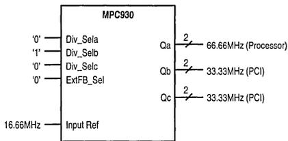
Figure 5. Dual Frequency Configuration
