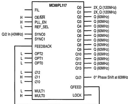
**Figure 1. Output Frequency Configuration 1**
