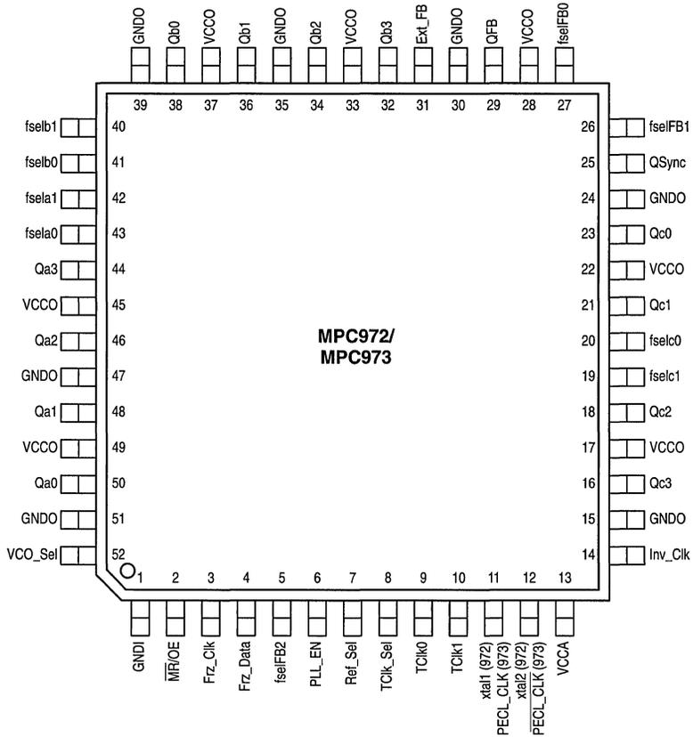
Figure 1.52—Lead Pinout (Top View)
