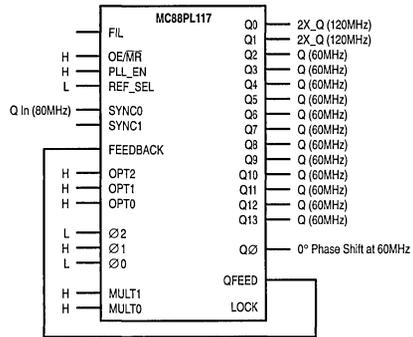
**Figure 6. Output Frequency Configuration 6**
