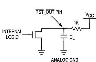
Figure 4. RST\_OUT Test Circuit
