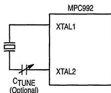
Figure 2. Recommended Crystal Interface
