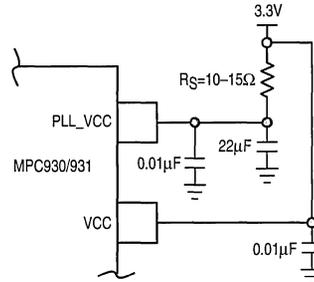
**Figure 14. Power Supply Filter**
