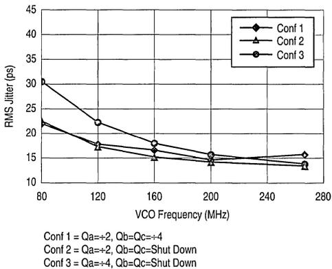
**Figure 12. RMS Jitter versus VCO Frequency (Qa0 Output)**
