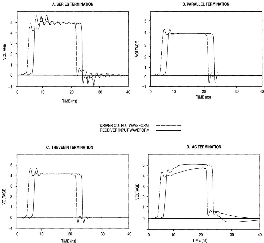
**Figure 6. SPICE Simulation Results for Various Terminations of a 9-Inch  $41\Omega$  Transmission Line. Simulations Were Run with Typical Model Parameters @  $25^\circ\text{C}$  and  $V_{CC} = 5.0\text{V}$**
