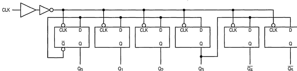
NOTE: This diagram is provided only for understanding of logic operation and should **not** be used to estimate propagation delays
