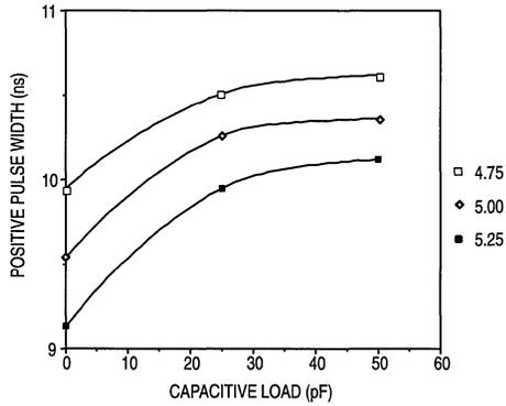
Figure 1. MC10H642 Positive PW versus Load
