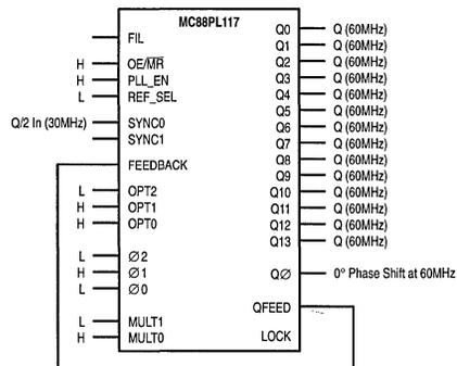
**Figure 4. Output Frequency Configuration 4**
