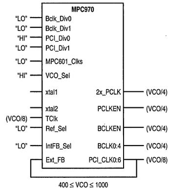
**Figure 5. External Feedback Configuration 2**
