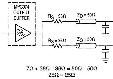
**Figure 7. Optimized Dual Line Termination**
