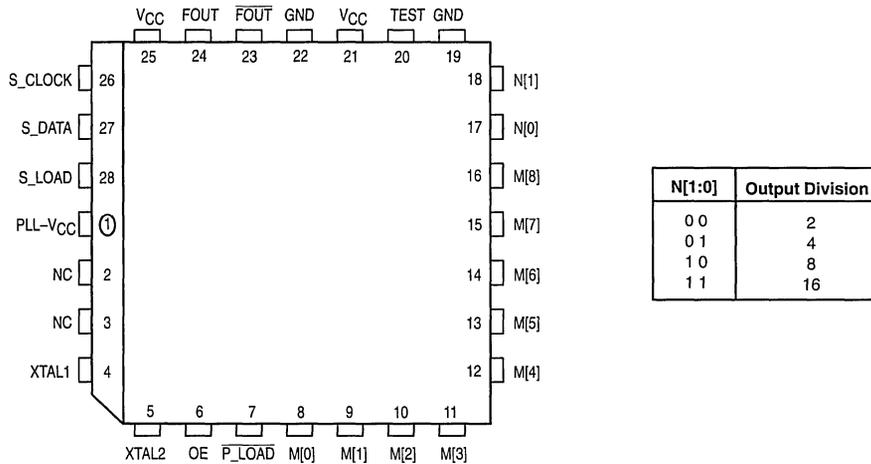
Figure 1. 28-Lead (Top View)
