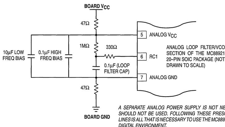
Figure 6. Recommended Loop Filter and Analog Isolation Scheme for the MC88921
