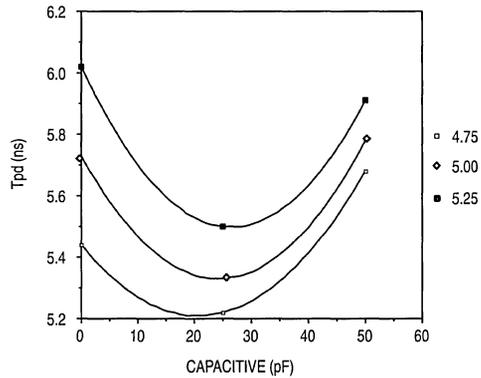
Figure 7. MC10H642 + Tpd versus Load,  $V_{CC} \pm 5\%$ ,  $T_A = 25^\circ C$
