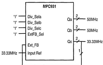
Figure 7. "Zero" Delay Fractional Multiplier
