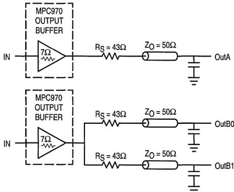
Figure 9. Single versus Dual Transmission Lines
