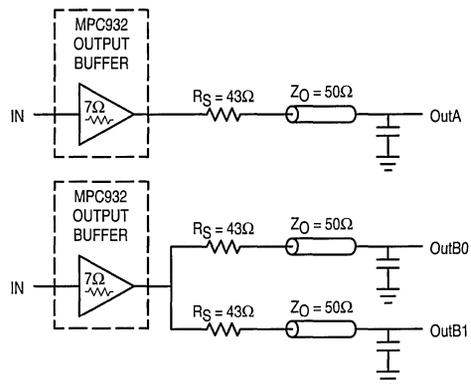
Figure 4. Single versus Dual Transmission Lines
