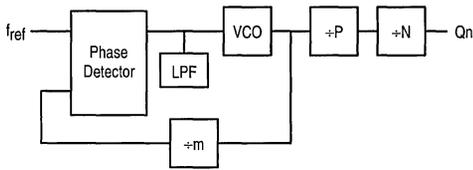
$$f_{\text{ref}} = \frac{f_{\text{VCO}}}{m}, \quad f_{\text{VCO}} = f_{\text{Qn}} \cdot N \cdot P$$
