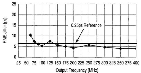
**Figure 6. RMS Jitter versus Output Frequency**
