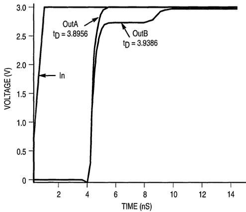
Figure 17. Single versus Dual Waveforms
