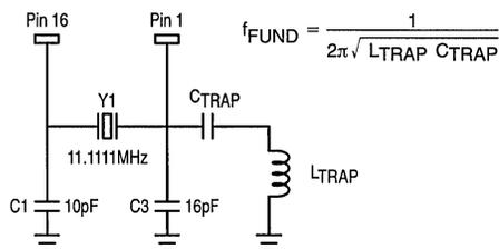
**Figure 4. Crystal Oscillator Interface (3rd Overtone)**
