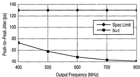
Figure 9. Peak-to-Peak Jitter versus Output Frequency
