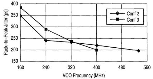
Conf 2 = 4 Outputs at X, 5 Outputs at X/2
