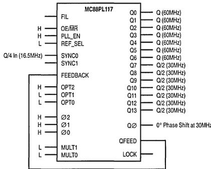
**Figure 5. Output Frequency Configuration 5**
