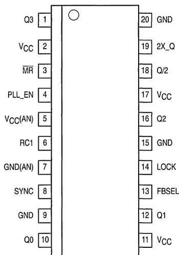
Pinout: 20-Lead Wide SOIC Package (Top View)
