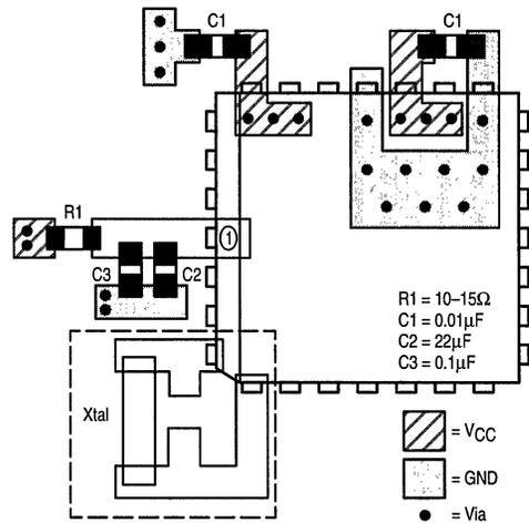
Figure 6. PCB Board Layout for MC12429
