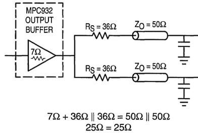
Figure 6. Optimized Dual Line Termination
