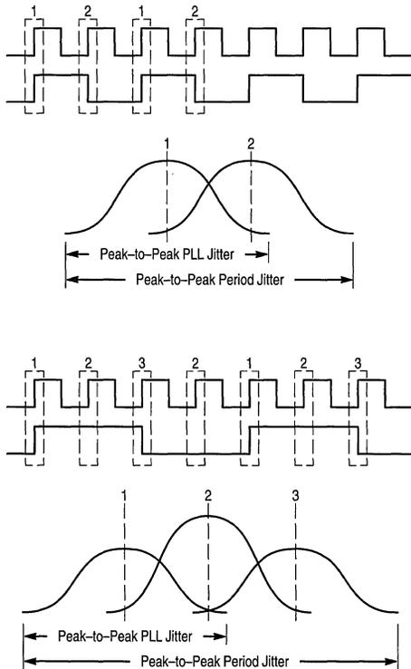
Figure 7. PLL Jitter and Edge Displacement
