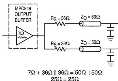
Figure 5. Optimized Dual Line Termination
