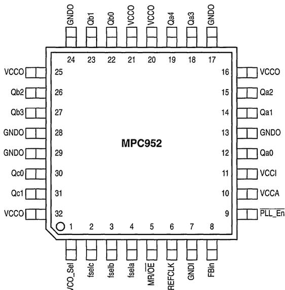
Figure 2. 32-Lead Pinout (Top View)
