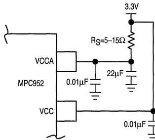
Figure 6. Power Supply Filter
