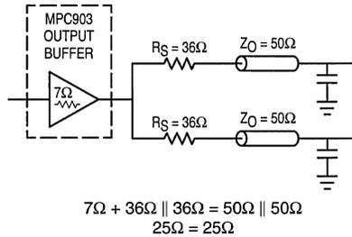
Figure 8. Optimized Dual Line Termination
