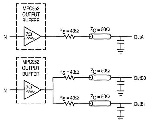
**Figure 3. Single versus Dual Transmission Lines**
