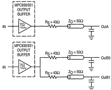
Figure 16. Single versus Dual Transmission Lines
