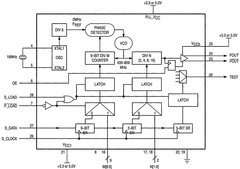
Figure 2. MC12429 Block Diagram
