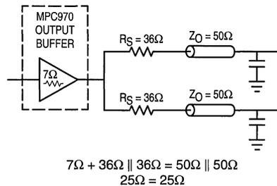
Figure 11. Optimized Dual Line Termination
