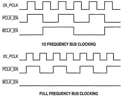
Figure 9. MPC601 Processor Clocking Waveforms
