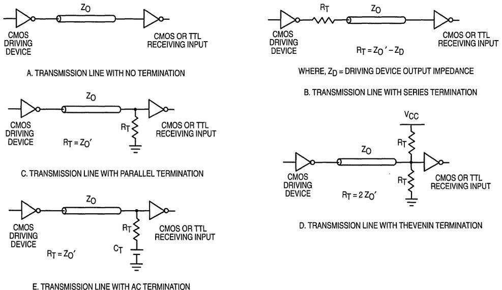
**Figure 5. Schematic Representation of Common Termination Techniques**
