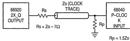
Figure 3. MC68040 P-Clock Input Termination Scheme
