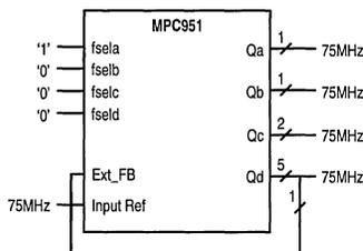
Figure 5. "Zero" Delay Buffer
