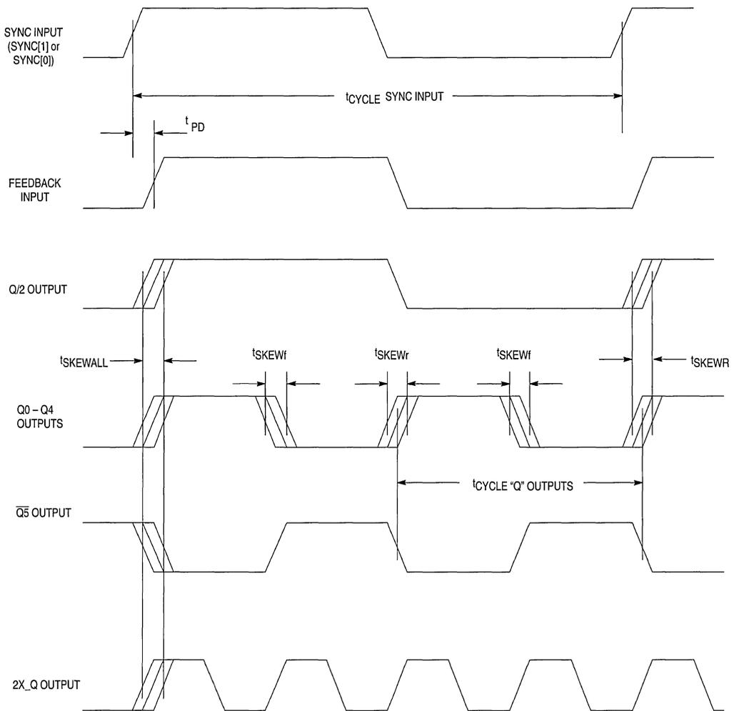
**Figure 4. Output / Input Switching Waveforms and Timing Diagrams**
