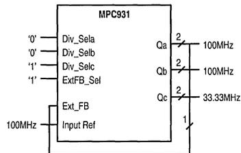
Figure 10. "Zero" Delay Divide by 3 (50% Duty Cycle)
