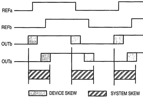
Figure 10. System Skew For PLL Clock Distribution
