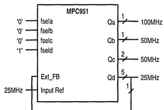
Figure 6. "Zero" Delay Frequency Multiplier
