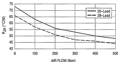
Figure 2. Thermal Resistance of the PLCC Packages
