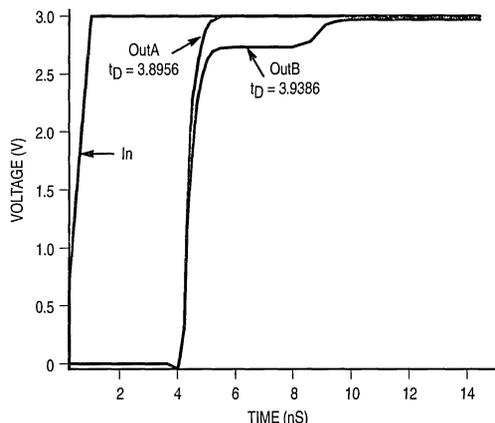
Figure 2. Single versus Dual Waveforms
