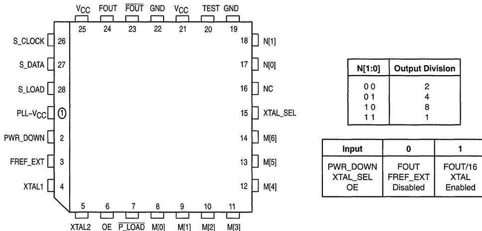
Figure 1. 28-Lead Pinout (Top View)
