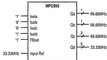
Figure 2. Dual Frequency Configuration
