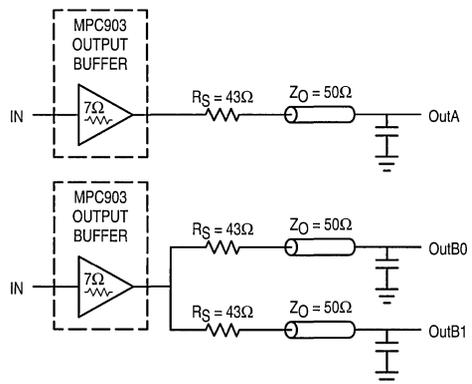
Figure 6. Single versus Dual Transmission Lines
