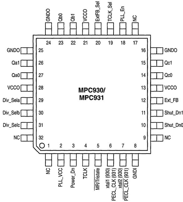
Figure 1. 32-Lead Pinout (Top View)
