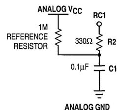
WITH THE 1MΩ RESISTOR TIED IN THIS FASHION THE t<sub>PD</sub> SPECIFICATION, MEASURED AT THE INPUT PINS IS:
