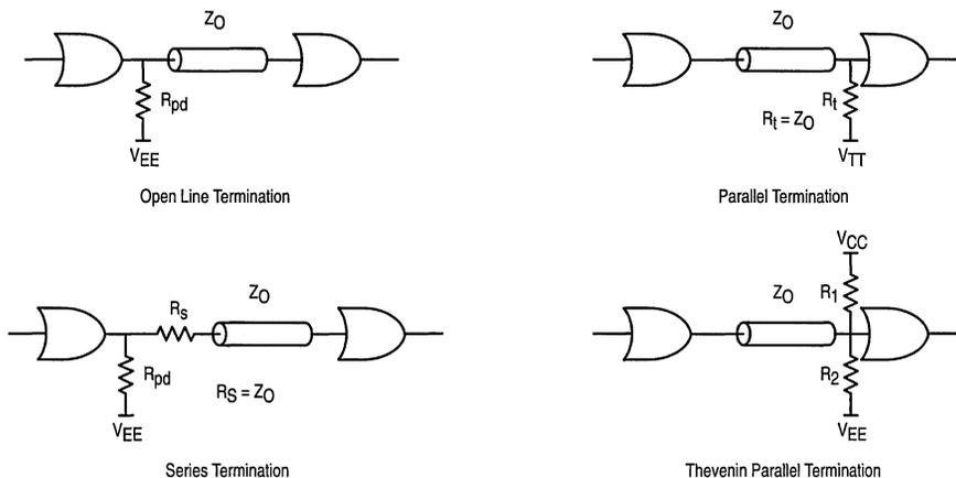
**Figure 3. Termination Techniques for ECL/PECL Devices**
