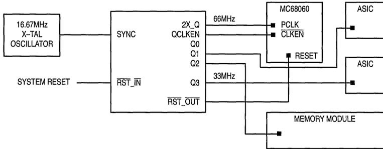
Figure 7. Typical MC88LV926/MC68060 System Configuration
