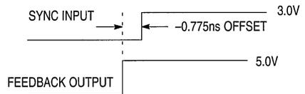
**Figure 2. Depiction of the Fixed SYNC to Feedback Offset (t<sub>PD</sub>) Which is Present When a 1MΩ Resistor is Tied to VCC or Ground**
