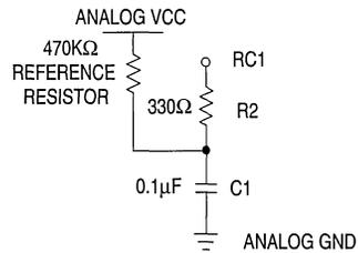
With the 470KΩ resistor tied in this fashion, the  $t_{PD}$  specification measured at the input pins is:
