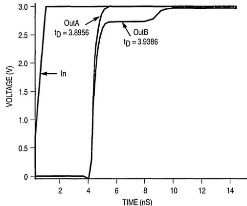
Figure 5. Single versus Dual Waveforms
