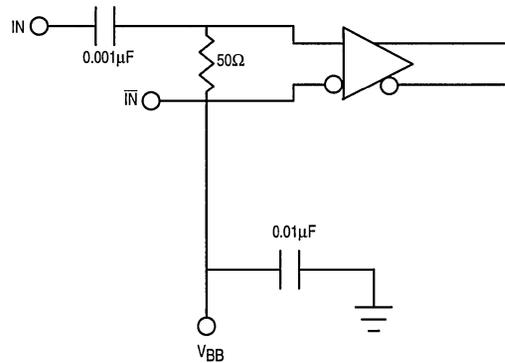
Figure 2a. AC Coupled Input
