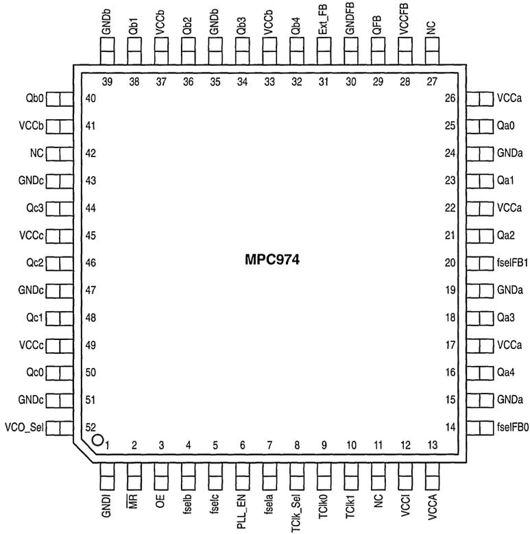
Figure 1. 52-Lead Pinout (Top View)
