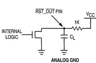
Figure 4. RST\_OUT Test Circuit
