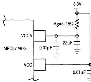
**Figure 8. Power Supply Filter**
