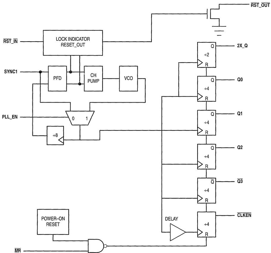
Figure 1. MC88LV926 Logic Block Diagram
