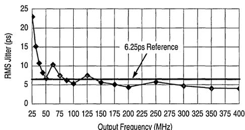
Figure 8. RMS Jitter versus Output Frequency
