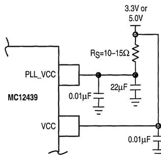
Figure 5. Power Supply Filter
