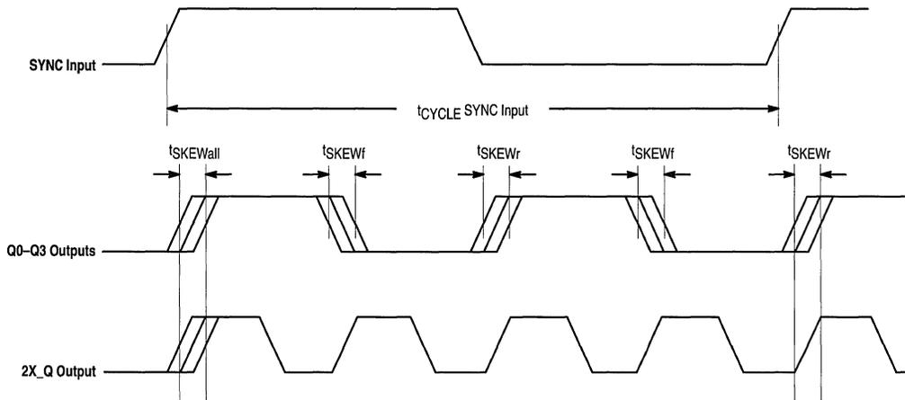
Figure 5. Output/Input Switching Waveforms and Timing Relationships
