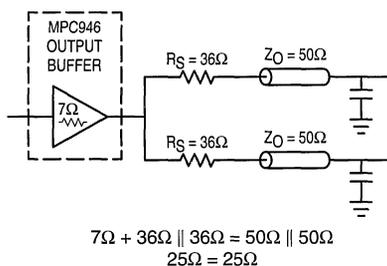
Figure 3. Optimized Dual Line Termination
