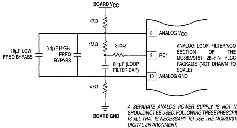
Figure 8. Recommended Loop Filter and Analog Isolation Scheme for the MC88LV915T
