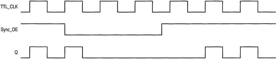
Figure 3. Sync\_OE Timing Diagram
