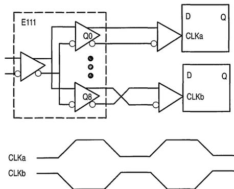
Figure 5.  $180^\circ$  Shifted Two Phase Clocks
