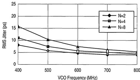
**Figure 5. RMS PLL Jitter versus VCO Frequency**
