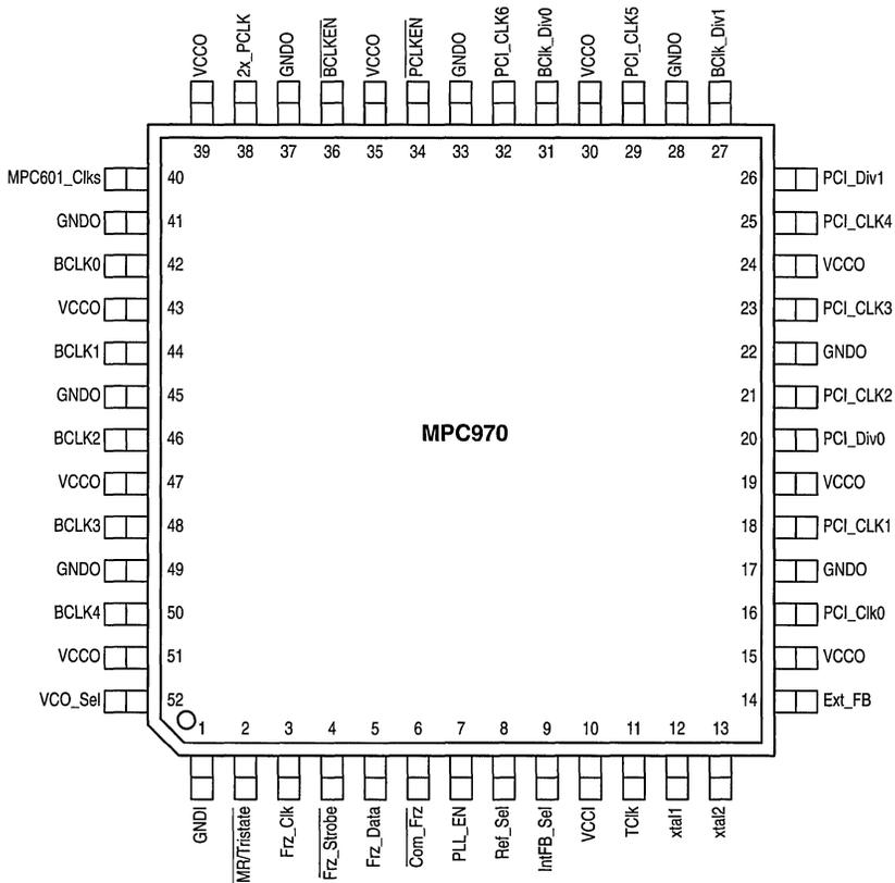
Figure 3. 52-Lead Pinout (Top View)
