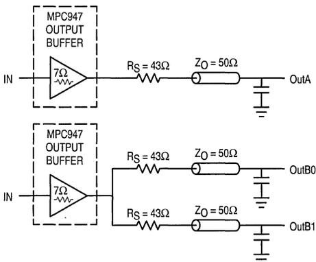
Figure 4. Single versus Dual Transmission Lines
