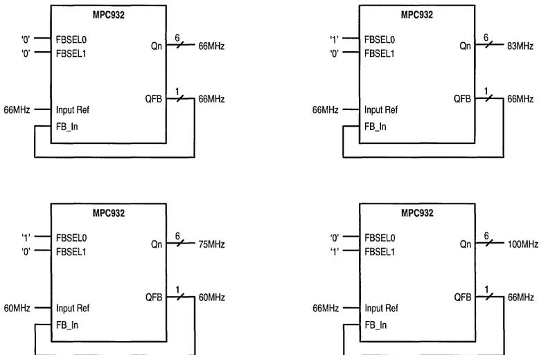
**Figure 2. MPC932 Potential Configurations**
