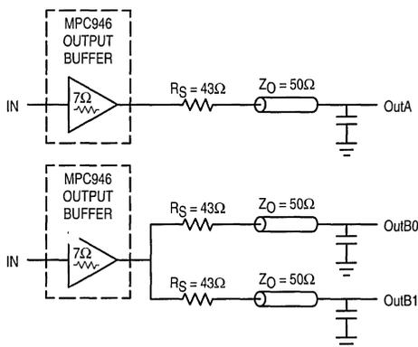
Figure 1. Single versus Dual Transmission Lines
