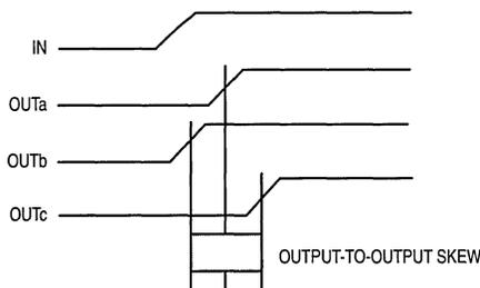
Figure 2. Output-to-Output Skew
