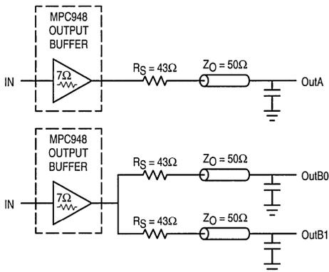
Figure 4. Single versus Dual Transmission Lines
