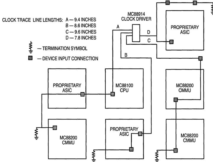
**Figure 2. Scale Representation of an Actual 88000 System PCB Layout**
