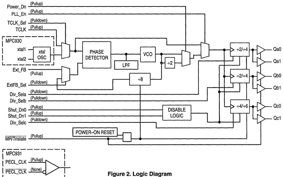
Figure 2. Logic Diagram
