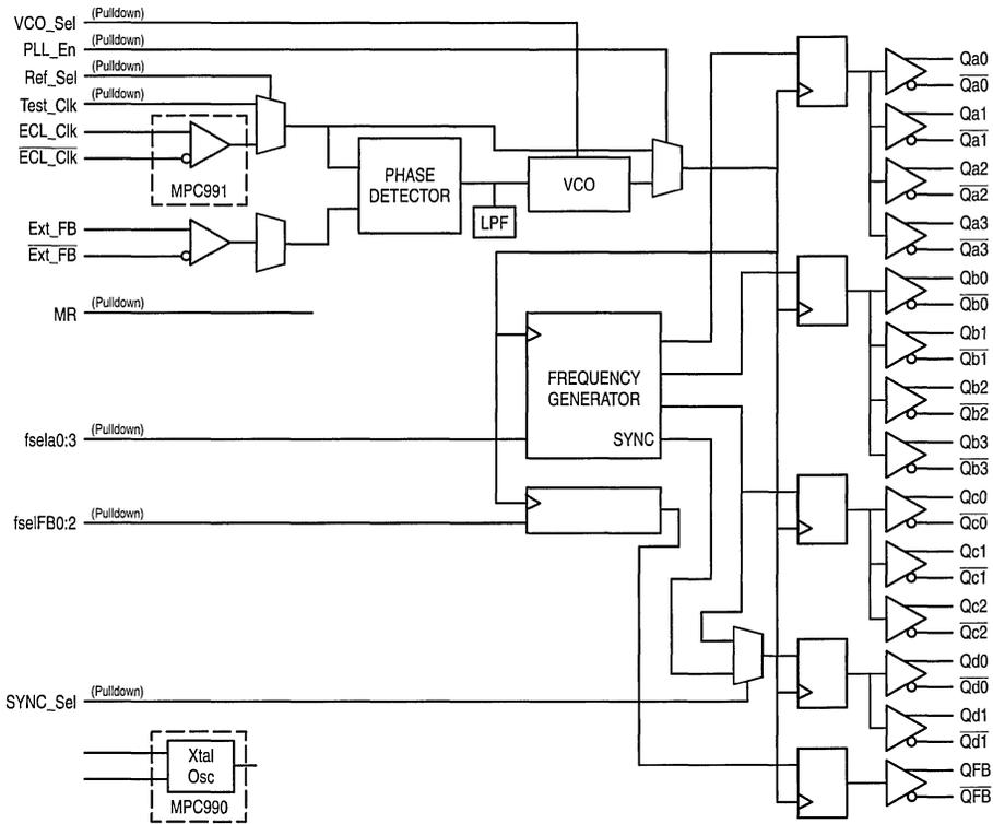
NOTE: ECL\_Clk, Ext\_FB have internal pulldowns, while ECL\_Clk, Ext\_FB have external pullups to ensure stability under open input conditions.
