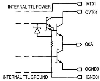
**Figure 1. Output Structure**
