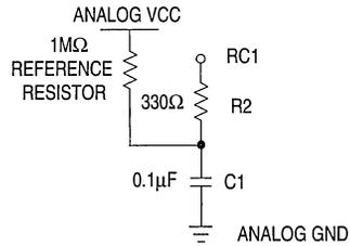
With the 1MΩ resistor tied in this fashion, the t<sub>PD</sub> specification measured at the input pins is:
