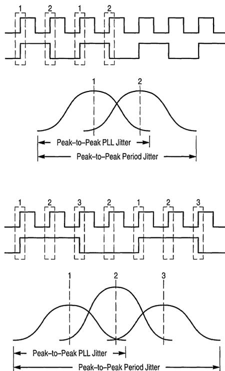
**Figure 11. PLL Jitter and Edge Displacement**
