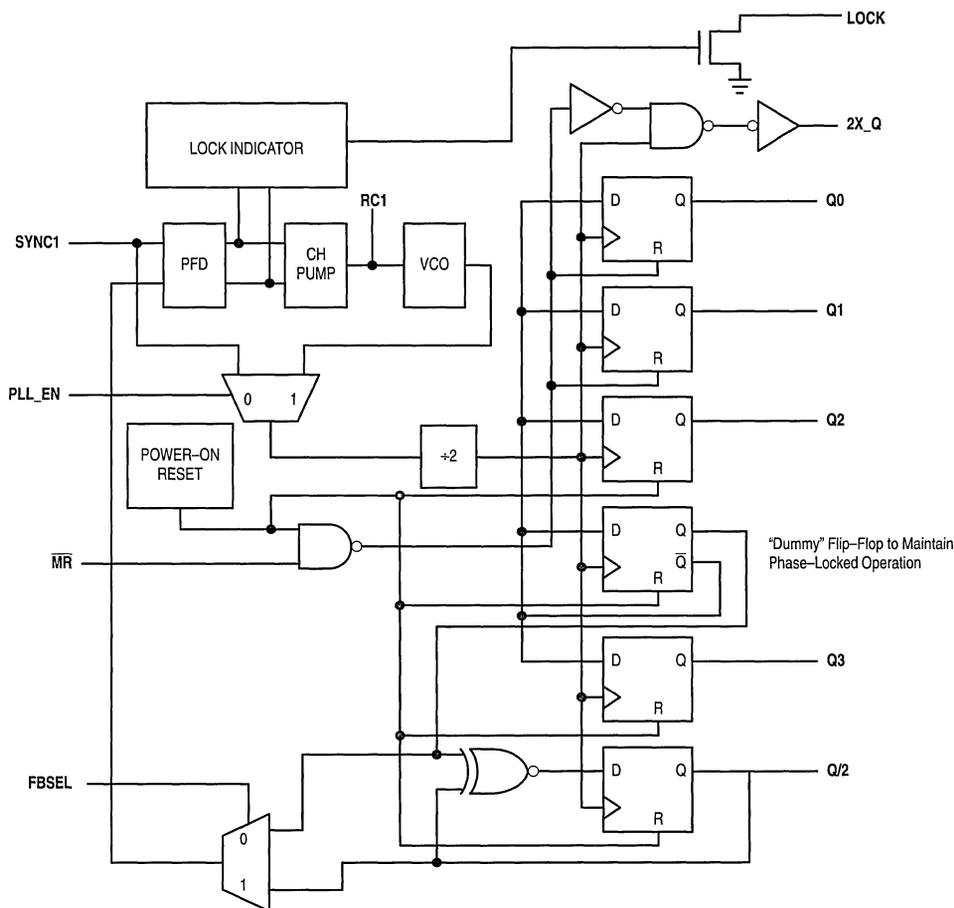
Figure 1. MC88921 Logic Block Diagram
