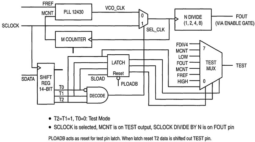
**Figure 2. Serial Test Clock Block Diagram**
