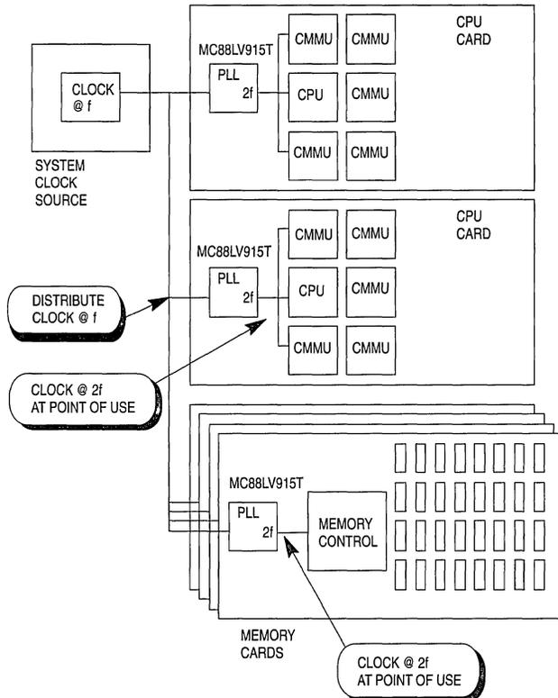
**Figure 9. Representation of a Potential Multi-Processing Application Utilizing the MC88LV915T for Frequency Multiplication and Low Board-to-Board Skew**
