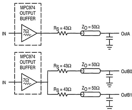
Figure 5. Single versus Dual Transmission Lines
