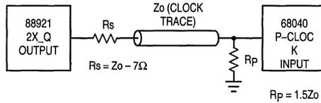
Figure 3. MC68040 P-Clock Input Termination Scheme
