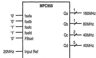
Figure 4. Triple Frequency Configuration
