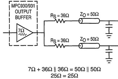
Figure 18. Optimized Dual Line Termination
