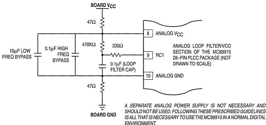
Figure 6. Recommended Loop Filter and Analog Isolation Scheme for the MC88915
