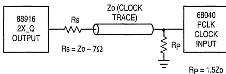
Figure 3. MC68040 PCLK Input Termination Scheme
