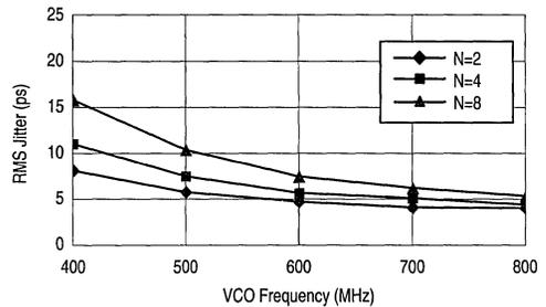
Figure 7. RMS PLL Jitter versus VCO Frequency
