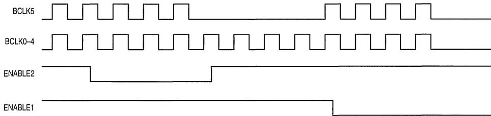
Figure 5. Enable Timing Diagram
