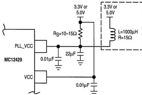
Figure 5. Power Supply Filter
