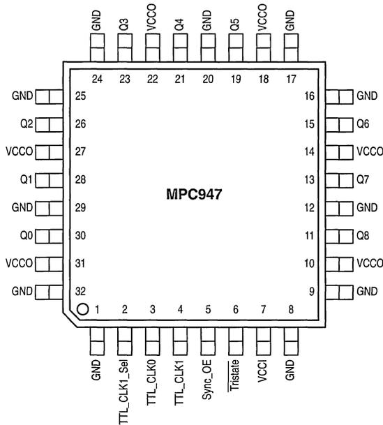
Figure 2. 32-Lead Pinout (Top View)
