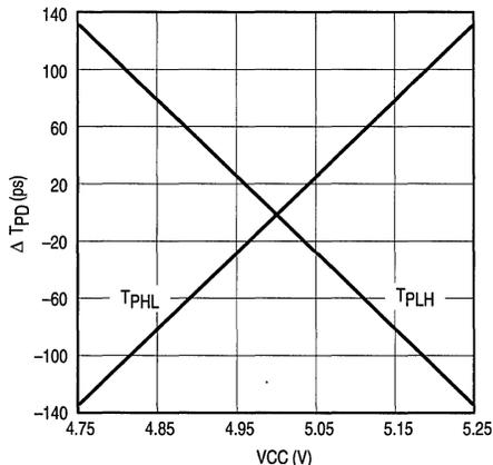
Figure 4.  $\Delta T_{PD}$  versus  $V_{CC}$
