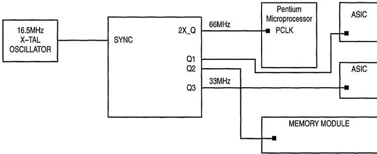
Figure 7. Typical MC88921/Pentium Microprocessor System Configuration
