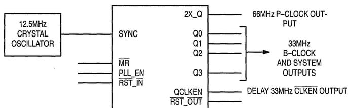
Figure 4. Logical Representation of the MC88LV926 With Input/Output Frequency Relationships
