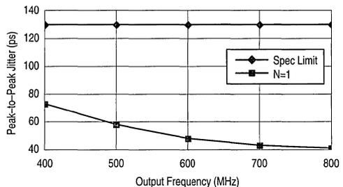
**Figure 7. Peak-to-Peak Jitter versus Output Frequency**
