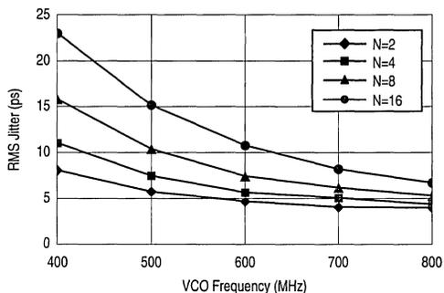
Figure 7. RMS PLL Jitter versus VCO Frequency
