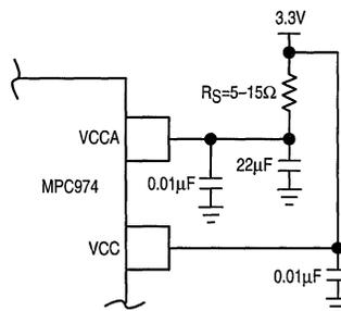
Figure 4. Power Supply Filter
