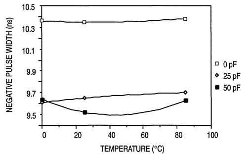
Figure 6. MC10H642 Negative PW versus Temperature,
