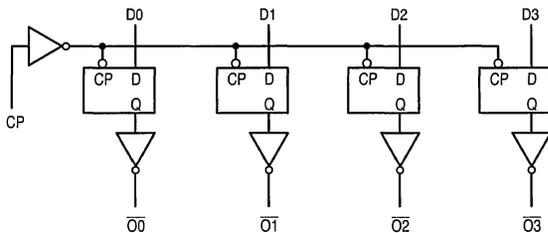
V<sub>CC</sub> = Pin 14; GND = Pins 1,7; NC = Pins 2, 13
