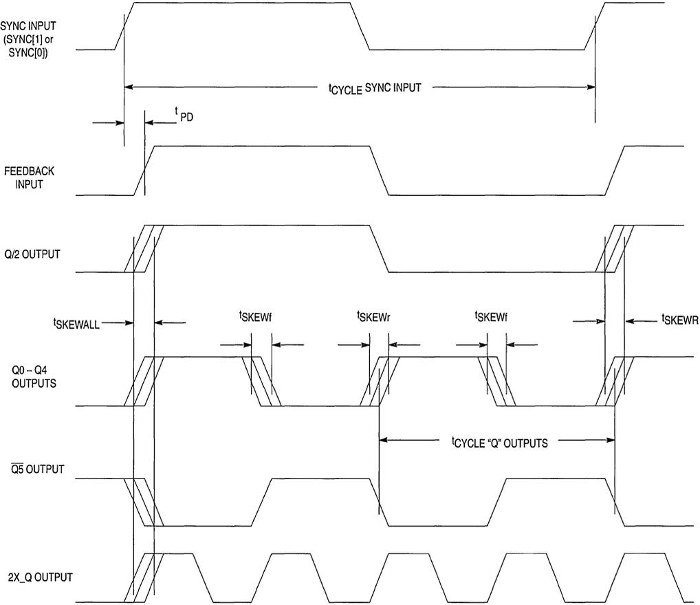
**Figure 4. Output/Input Switching Waveforms and Timing Diagrams**
