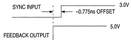
**Figure 2. Depiction of the Fixed SYNC to Feedback Offset ( $t_{PD}$ ) Which is Present When a 470KΩ Resistor is Tied to VCC or Ground**
