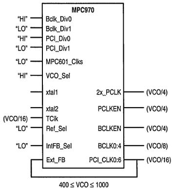
**Figure 7. External Feedback Configuration 4**
