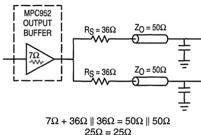
Figure 5. Optimized Dual Line Termination
