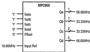
Figure 1. Dual Frequency Configuration
