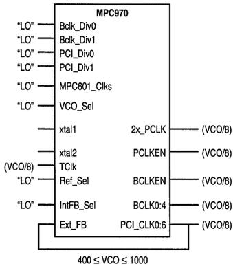
**Figure 4. External Feedback Configuration 1**
