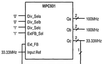
Figure 9. "Zero" Delay Multiply by 3 (50% Duty Cycle)
