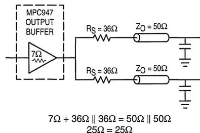
Figure 6. Optimized Dual Line Termination
