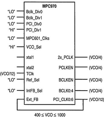
**Figure 6. External Feedback Configuration 3**
