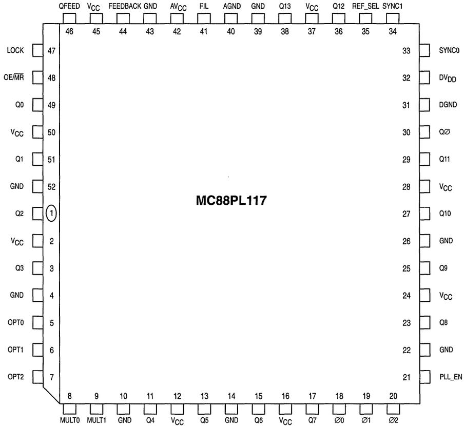
**Pinout: 52-Lead PLCC (Top View)**
