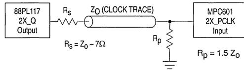
Figure 11. MPC601 2X\_PCLK Input Termination Scheme
