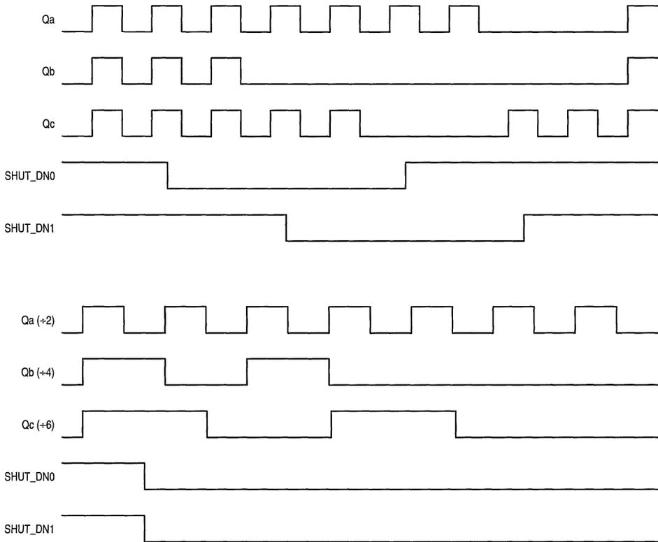
Figure 4. Shut\_Dn Timing Diagram
