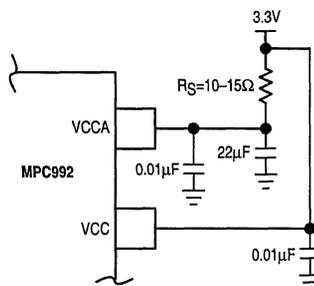
Figure 3. Power Supply Filter
