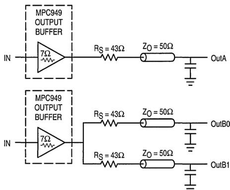
Figure 3. Single versus Dual Transmission Lines
