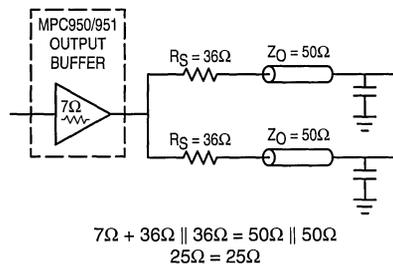
Figure 14. Optimized Dual Line Termination
