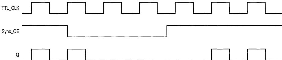
Figure 3. Sync\_OE Timing Diagram
