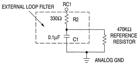
With the 470KΩ resistor tied in this fashion, the  $t_{PD}$  specification measured at the input pins is:
