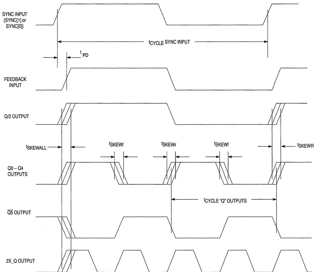
**Figure 6. Output/Input Switching Waveforms and Timing Diagrams**
