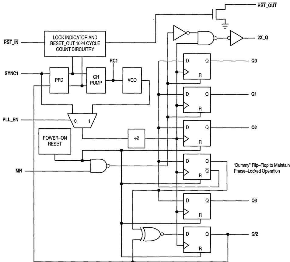
Figure 1. MC88920 Logic Block Diagram
