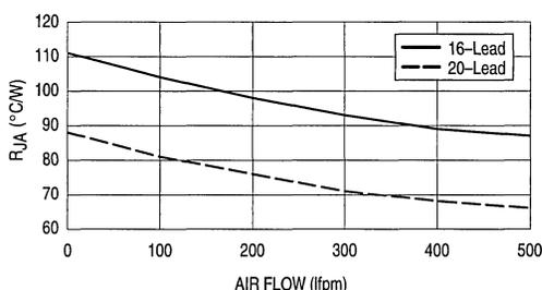
Figure 3. Thermal Resistance of the SOIC Packages
