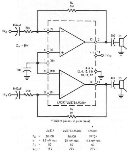
FIGURE 5. Inverting Stereo Amplifier
