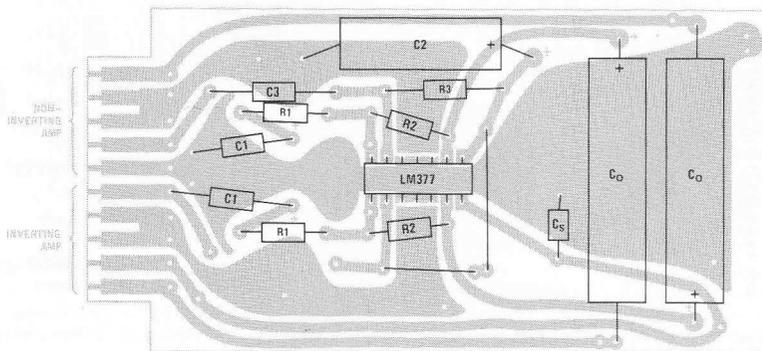
FIGURE 13. Parts Layout for LM377/LM378 Dual Amplifier
