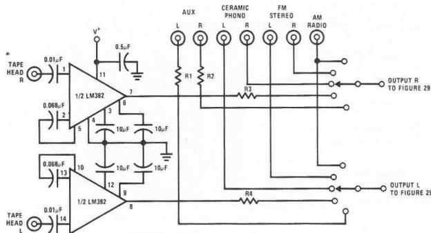
FIGURE 30. Two-Channel Tape-Playback Amplifier and Signal Switching
