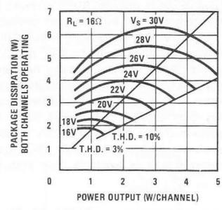
FIGURE A-2. Power Dissipation vs Power Output
