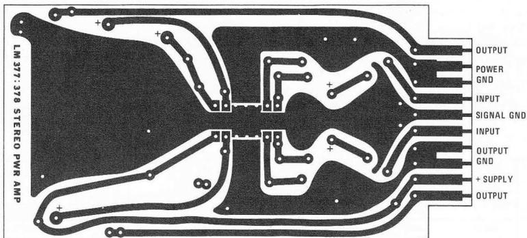
FIGURE 14. PC Board for LM377/LM378 Dual Amplifier
