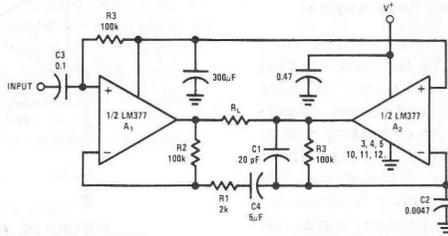
FIGURE 23. 4-Watt Bridge Amplifier with High Input Impedance
