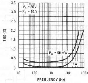
FIGURE 22. Distortion for Bridge Amp of Figure 20
