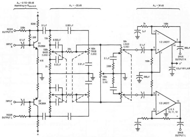
FIGURE 29. Two-Channel Power Amplifier and Control Circuits
