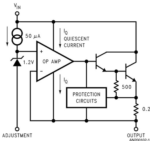
FIGURE 1. Functional Schematic of the LM117
