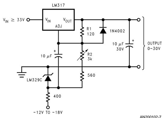
FIGURE 5. General Purpose 0–30V Power Supply
