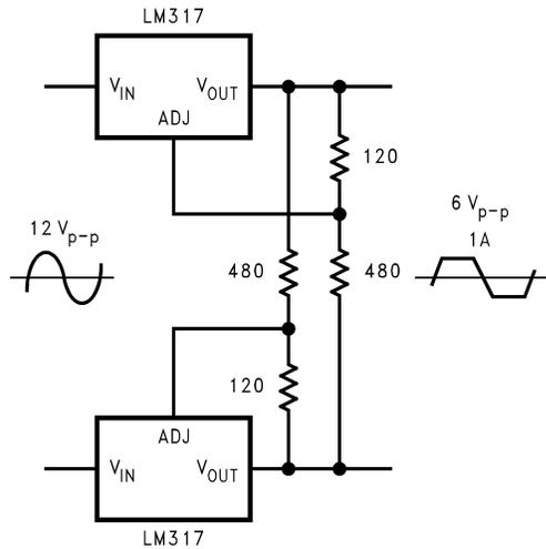
**FIGURE 12. AC Voltage Regulator**
