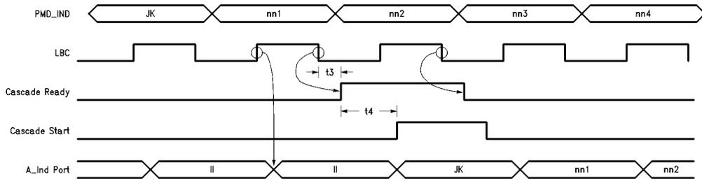
**FIGURE 5b. First PLAYER device to receive a JK symbol in a small skew scenario. The CS signal goes high shortly after assertion of the CR signal, indicating that all of the channels received JK symbols within  $t_4$ .**
