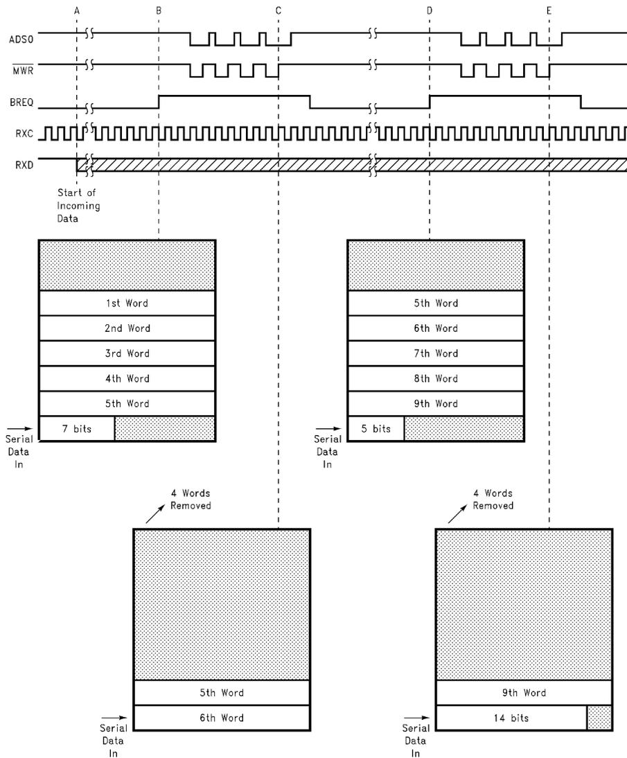
**FIGURE 3. Receive Packet—Word Mode, 4 Word Threshold**
