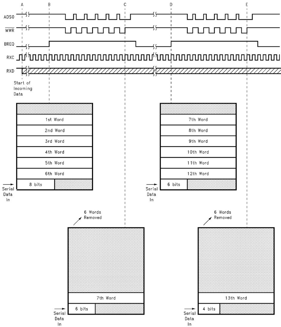
**FIGURE 4. Receive Packet—Word Mode, 6 Word Threshold**
