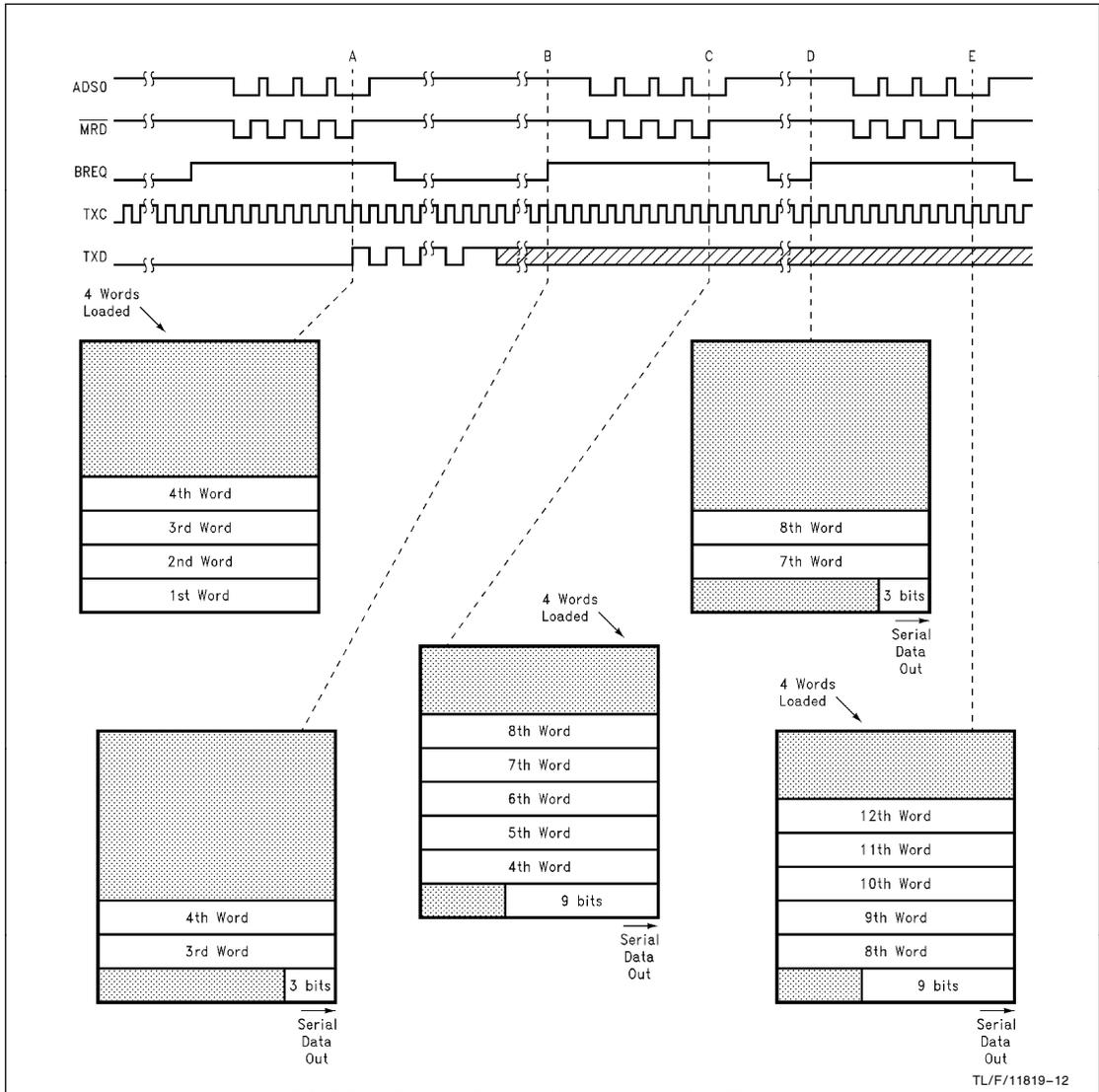
**FIGURE 12. Transmit Packet—Word Mode, 4 Word Threshold**
