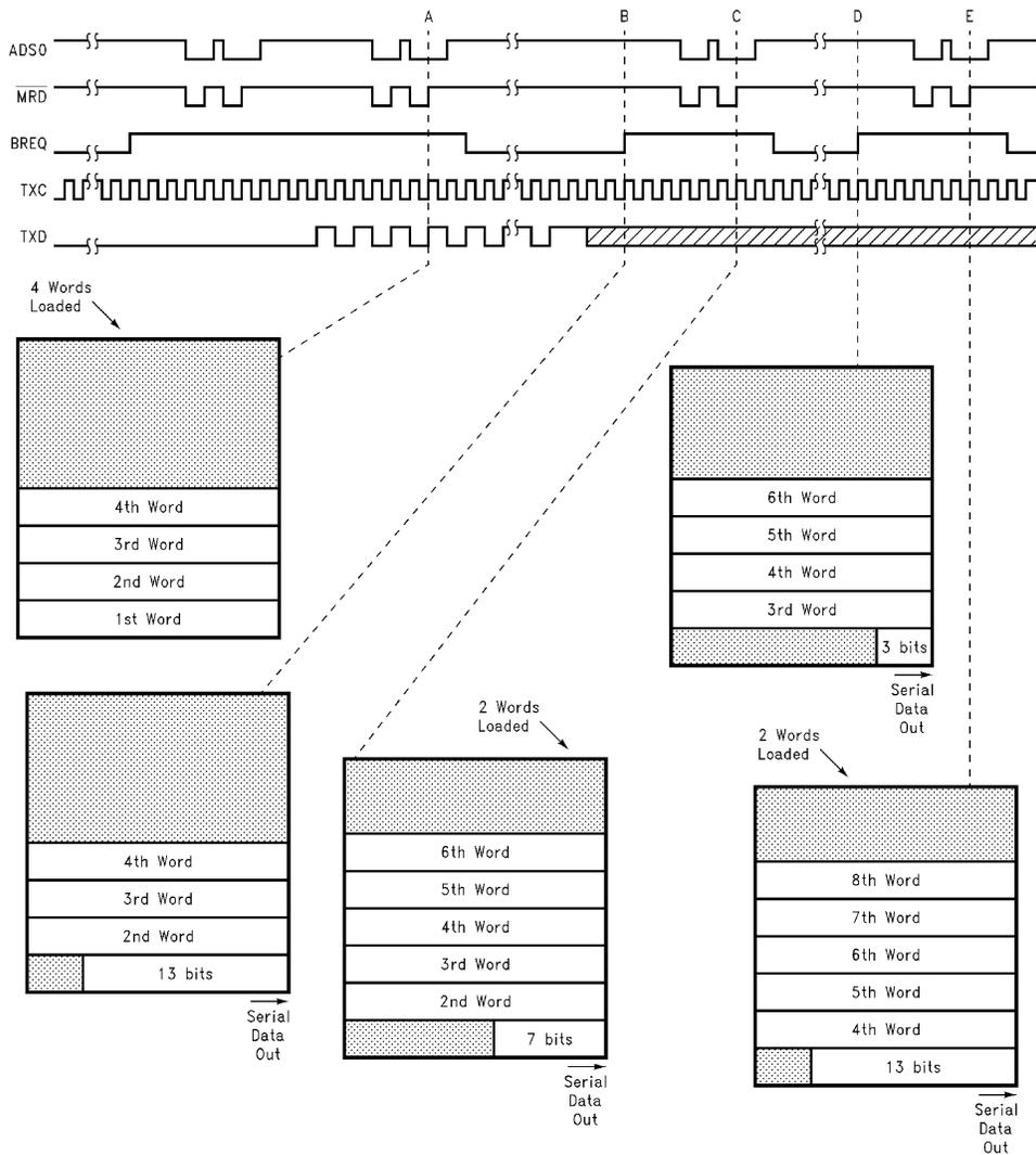
**FIGURE 11. Transmit Packet—Word Mode, 2 Word Threshold**
