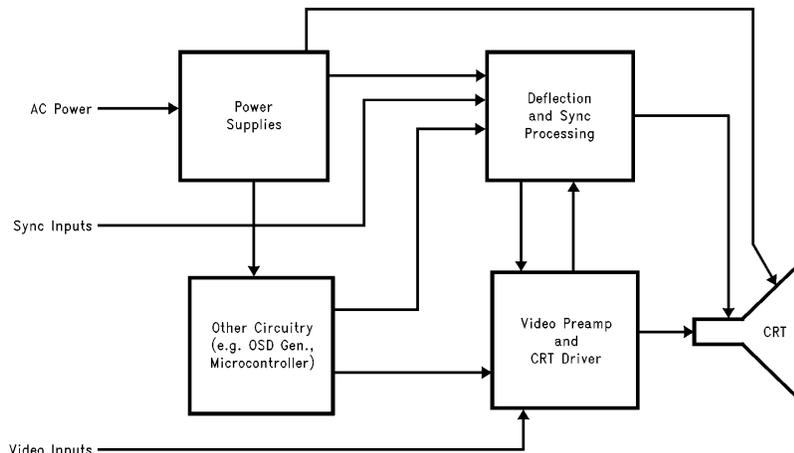
FIGURE 6. Simplified Block Diagram of a CRT Monitor
