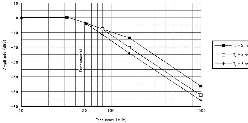
**FIGURE 4. Spectral Envelope for a 1 V<sub>p-p</sub>, 50 MHz Square Wave with Various Rise Times**
