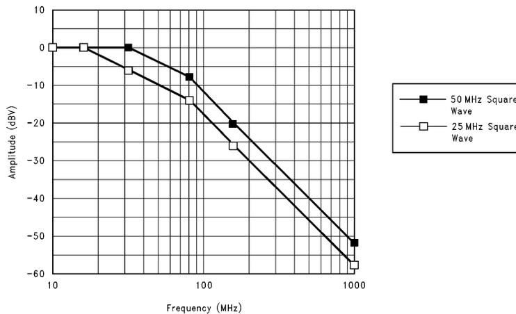
**FIGURE 5. Fourier Envelopes of 4 ns Rise Time, 1 V<sub>p,p</sub> Square Waves**
