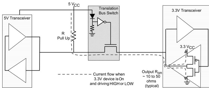
FIGURE 4. CMOS 5V to 3.3V translation using a pull up resistor, showing the current paths through the 3.3V and ground rails this design creates
