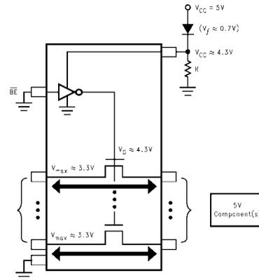
FIGURE 2. 5V to 3.3V Translation Waveform
