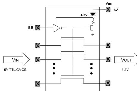
FIGURE 3. Fairchild Semiconductor's FSTD device incorporating the diode translation function and a switch to eliminate current flow during High Impedance mode.
