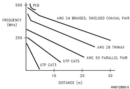
**FIGURE 5. You Can Use Inexpensive Unshielded Twisted-Pair (UTP) Category 3 Cable at Low Frequency and Short Distance. You Need Carefully Constructed Premium Cable at Higher Frequencies and Longer Distances.**
