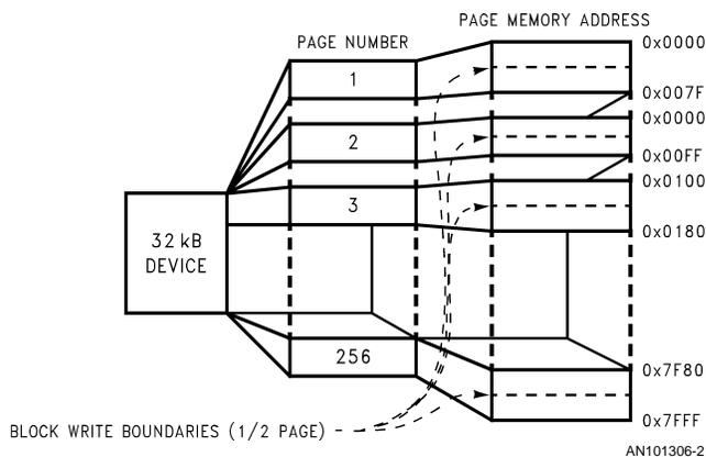
**FIGURE 11. Depiction of a PAGE Segment and the BLOCK\_WRITE Limitation**
