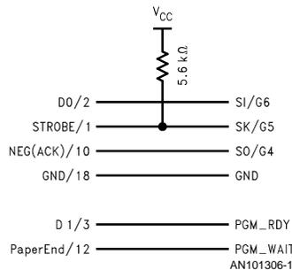
FIGURE 1. Parallel Port Connection Diagram
