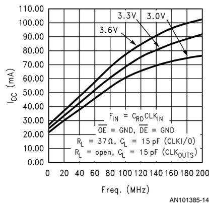
FIGURE 14.  $I_{CC}$  vs Frequency with the  $C_{RD}CLK$  in as the Input, and CLKI/O,  $CLK_{OUT}$  Pins Switching
