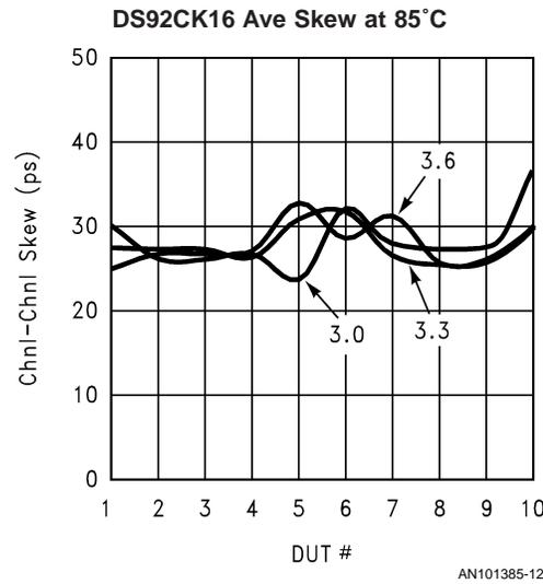
FIGURE 12. Receiver Channel to Channel Skew at 85°C
