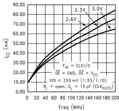
FIGURE 13. Typical  $I_{CC}$  vs Frequency. Input is CLKI/O
