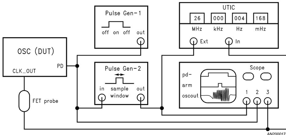
FIGURE 1. Sample Measurement Setup
