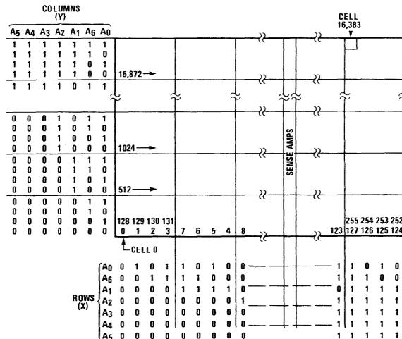
Figure 2. MM5290 Bit Map and Address Decoding
