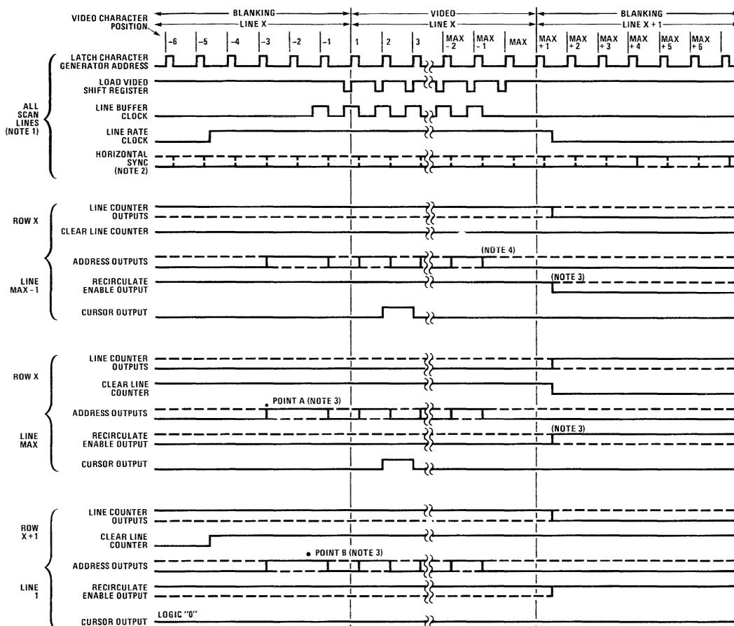
**Note 1:** The load video shift register output is not active during vertical or horizontal blanking (remains in the logic "1" state during these intervals).
