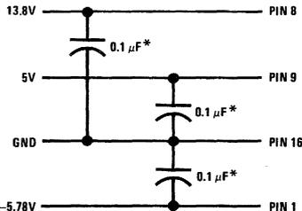
\*0.1  $\mu\text{F}$  capacitors between 5V and GND, -5V and GND alternate every other socket in each column, 0.1  $\mu\text{F}$  capacitors between 12V and GND every socket.
