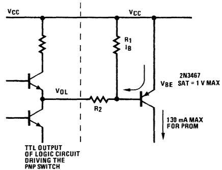
$$I_B = \frac{130 \text{ mA} = I_{CC}}{h_{fe} = 40} = 3.25 \text{ mA}$$
