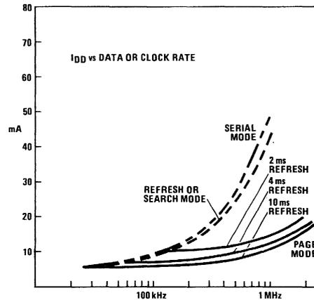
Figure 3.  $I_{DD}$  vs Clock or Data Rate @  $+70^{\circ}C$
