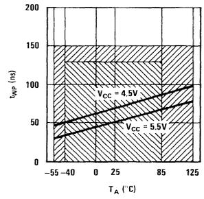
(c) Minimum Write Pulse Width vs Ambient Temperature
