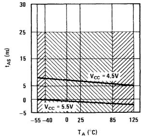
(h) Address Setup Time vs Ambient Temperature
