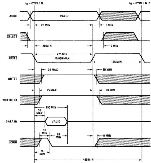
Figure 2. WRITE Cycle Timing
