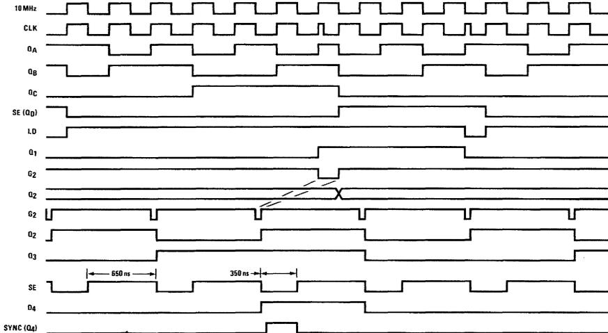
Figure 5. Waveforms for 1 MHz Clock Generator
