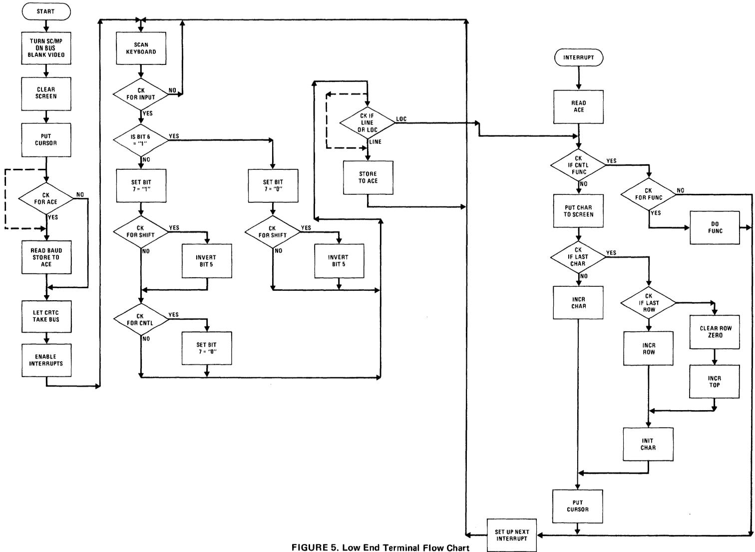
FIGURE 5. Low End Terminal Flow Chart
