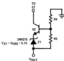
FIGURE 11. Regulator Circuit
