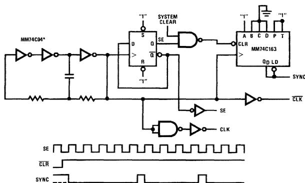
Figure 8. 750 kHz Clock Generation – 50% Duty Cycle SE Clock
