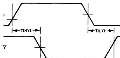
The first interval is the delay from I HIGH to Y LOW and the second from I LOW to Y HIGH.
