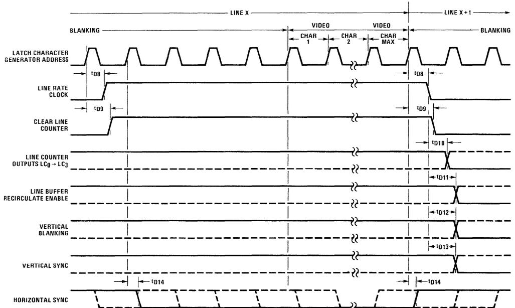
\*THE POSITION OF THE START AND STOP POINTS OF THE HORIZONTAL SYNC PULSE ARE PROGRAMMABLE BY CHARACTER TIME -- WITHIN ONE CHARACTER TIME THE POINTS WILL HAVE THE  $t_{D14}$  TIME RELATIONSHIP.
