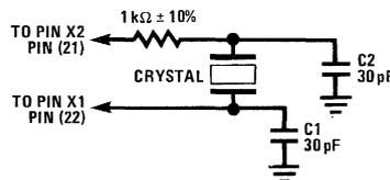
If the DP8350 series is clocked at dot rate by a system clock, pin 22 (X1 input) should be clocked directly using a Schottky series circuit. Pin 21 (X2 input) may be left open.
