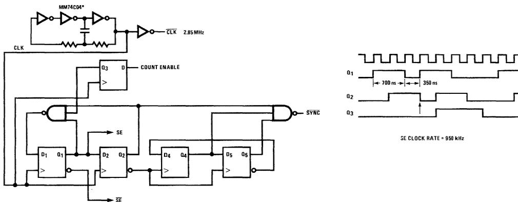
Figure 7. CMOS 950 kHz Clock Generator
