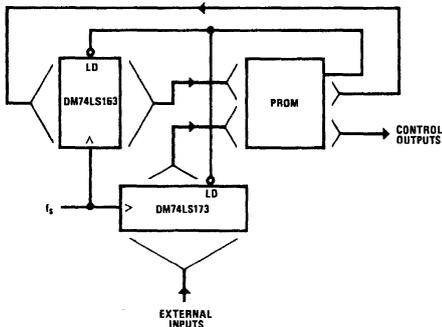
Figure 7. Determination of Next State Using External Inputs
