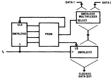
Figure 6. Sequencer Controlling Clocked & Unclocked Devices
