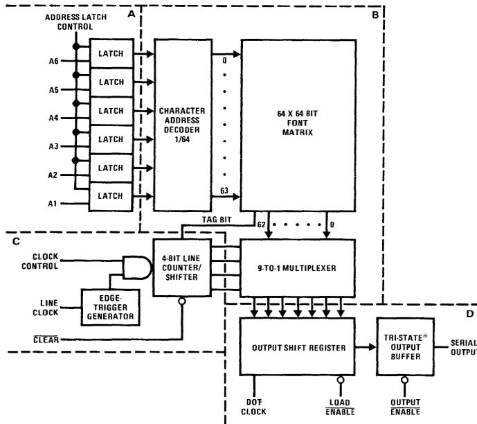
FIGURE 1. Block Diagram
