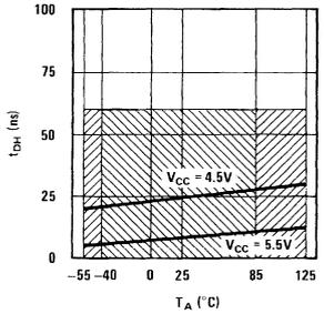
(e) Data-In Hold Time vs Ambient Temperature
