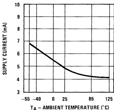
FIGURE 17. Typical DC Supply Current with TTL Input Levels vs Ambient Temperature
