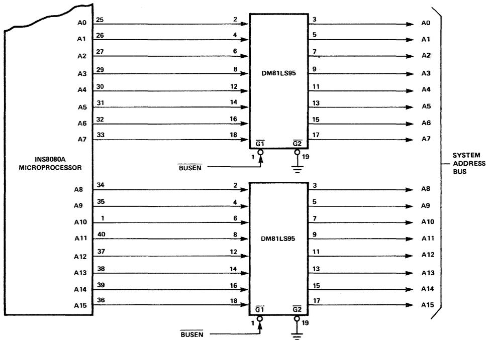
Figure 1. Address Buffer Design Using DM81LS95 Devices
