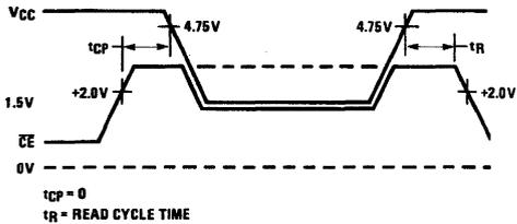
Figure 4. 4k Static Power Down Mode
