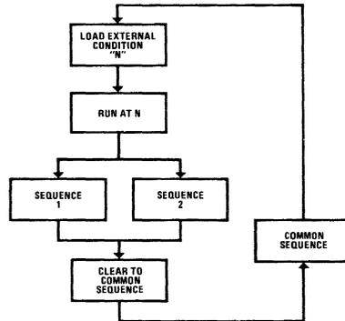
Figure 9. Control Sequence Determined by External Conditions
