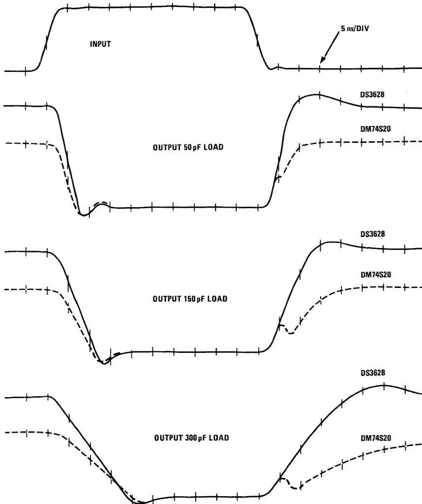
Figure 3. Switching Response with Capacitive Load
