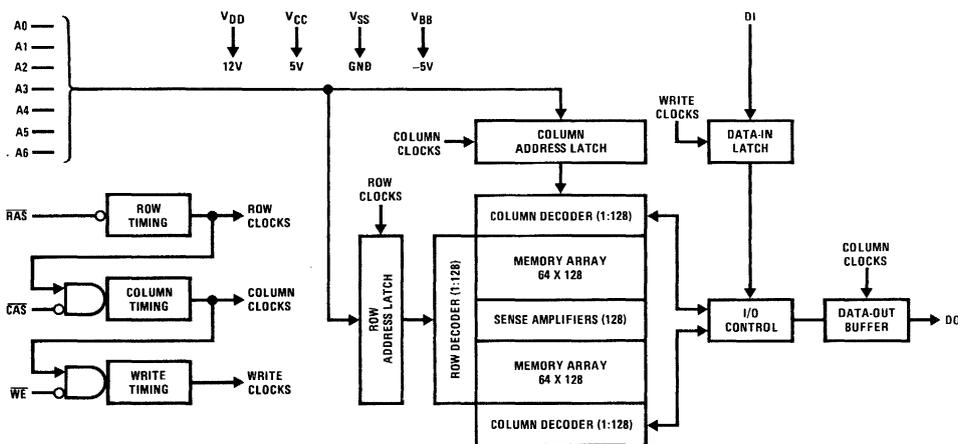
FIGURE 1. MM5290 Block Diagram
