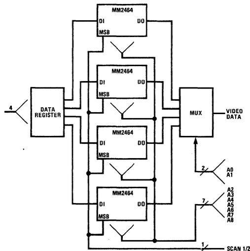
Figure 13. 1/4-Megabit CRT Display Memory Using CCDs
