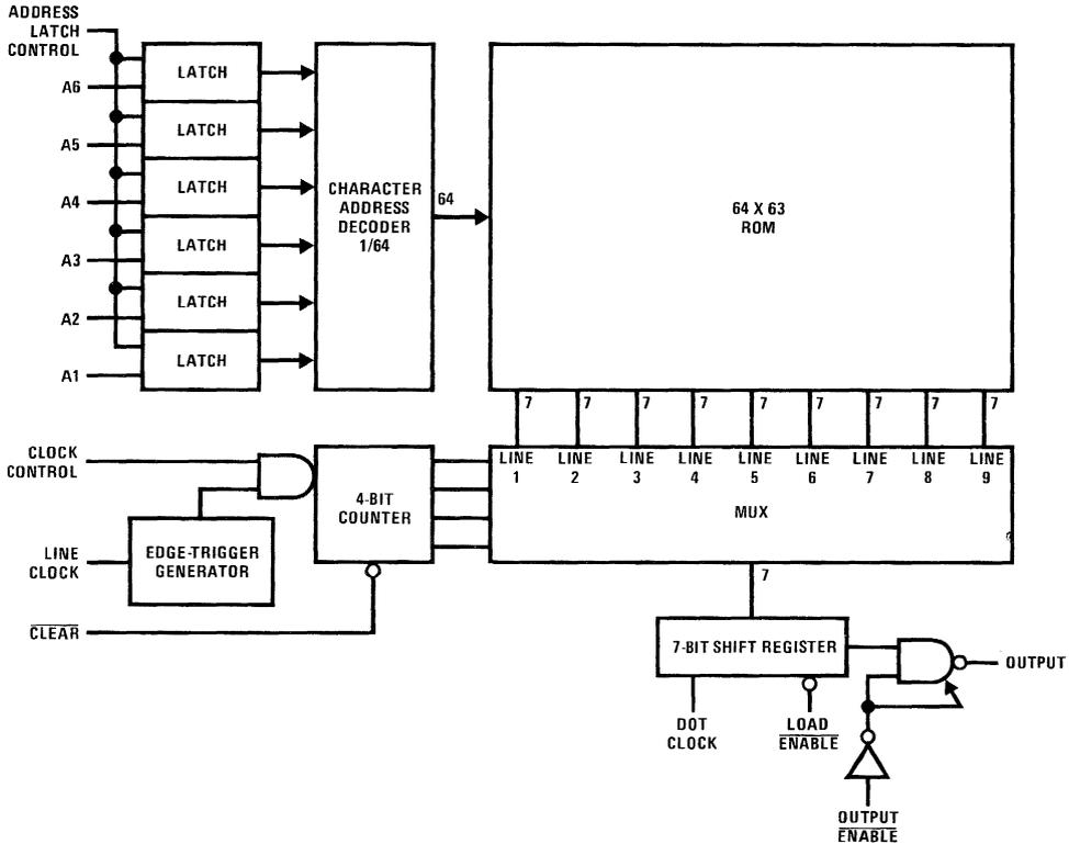
FIGURE 1. Block Diagram
