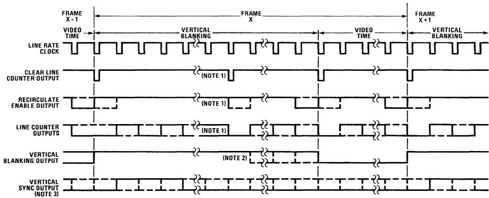
**Note 1:** One full row before start of video the line counter is set to zero state — this provides line counter synchronization in cases where the number of lines in vertical blanking are not even multiples of the number of lines per row.
