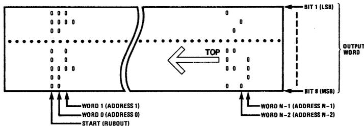
Note: Start with a RUBOUT and enter the output words in sequence from word 0 (address 0) to word  $N-1$  (address  $N-1$ ). There must not be any other characters on the tape. THIS FORMAT IS THE LEAST RELIABLE.
