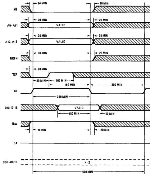
Figure 2. Write Cycle Timing
