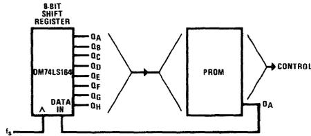
$$Q_A = [Q_A \oplus Q_F \oplus Q_G \oplus Q_H] + Q_A Q_B Q_C Q_D Q_E Q_G Q_H$$
