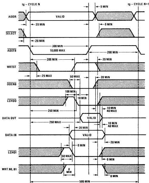
Figure 3. READ/DELAYED WRITE Cycle Timing
