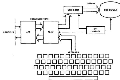
FIGURE 4. Block Diagram of an Interactive Terminal.
