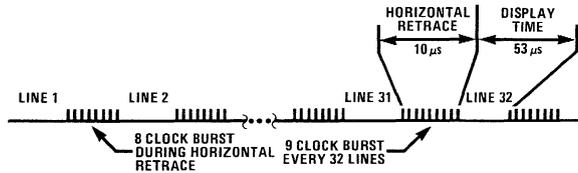
Figure 14. CCD Clock Timing During Display
