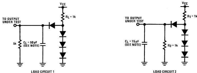
NOTE:  $C_L$  INCLUDES PROBE AND JIG CAPACITANCE
