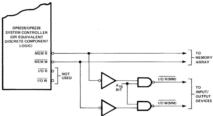
Figure 4. System Control Signals for Memory Mapped Input/Output Addressing
