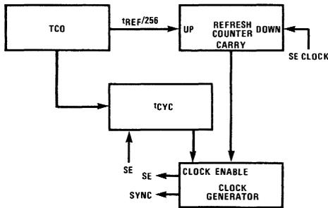
Figure 9. Block Diagram of Adaptive Refresh Circuit
