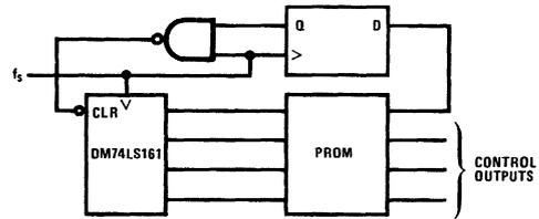
Figure 4a. Controller Using Asynchronous Device
