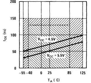
(i) Output Enable Time vs Ambient Temperature
