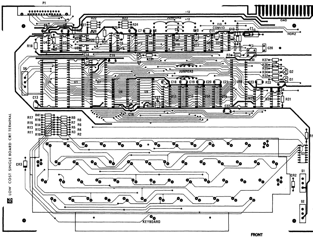
FIGURE 7A. PC Board Layout Assembly
