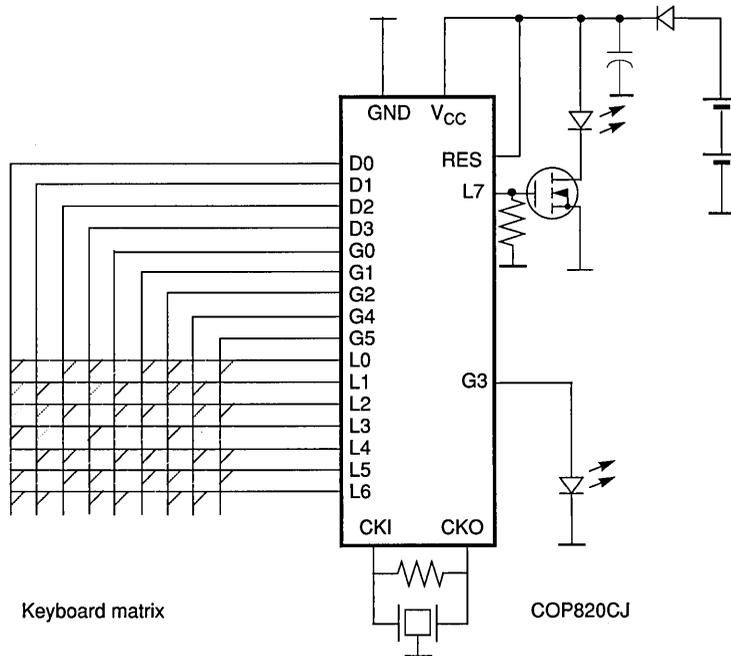
**Figure 10-8** Battery-Powered Remote Control Unit
