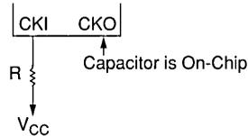
**Figure 2-5** RC Oscillator Circuit for COP840CJ Only
