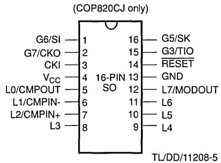
**Figure 10-2** Device Package Pinouts
