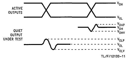
FIGURE 11. Quiet Output Noise Voltage Waveforms
