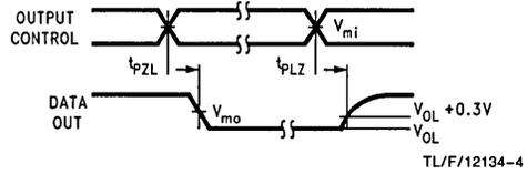
**FIGURE 4. TRI-STATE Output Low Enable and Disable Times**
