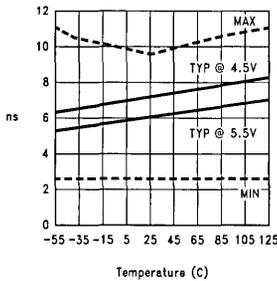
**$t_{PLH}$  (CP to  $O_n$ ) vs Temperature**
