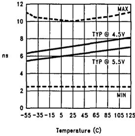
**$t_{PLH}$  (LE to  $O_n$ ) vs Temperature**
