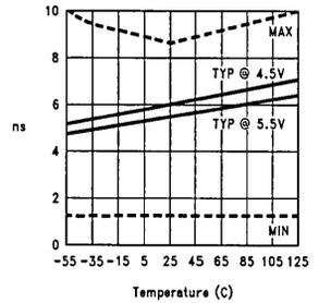
**$t_{pLZ}$  ( $\overline{OE}$  to  $A_n/B_n$ ) vs Temperature**
