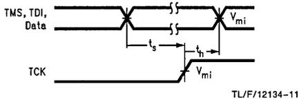
**FIGURE 11. Setup Time, Hold Time and Recovery Time**
