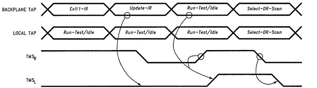
FIGURE 10. Local Scan Port Synchronization from *Parked-RTI* State
