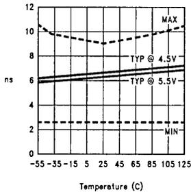
**$t_{PHL}$  ( $I_n$  to  $O_n$ ) vs Temperature**
