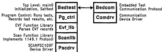
FIGURE 5. SCAN EASE Code Is Modular
