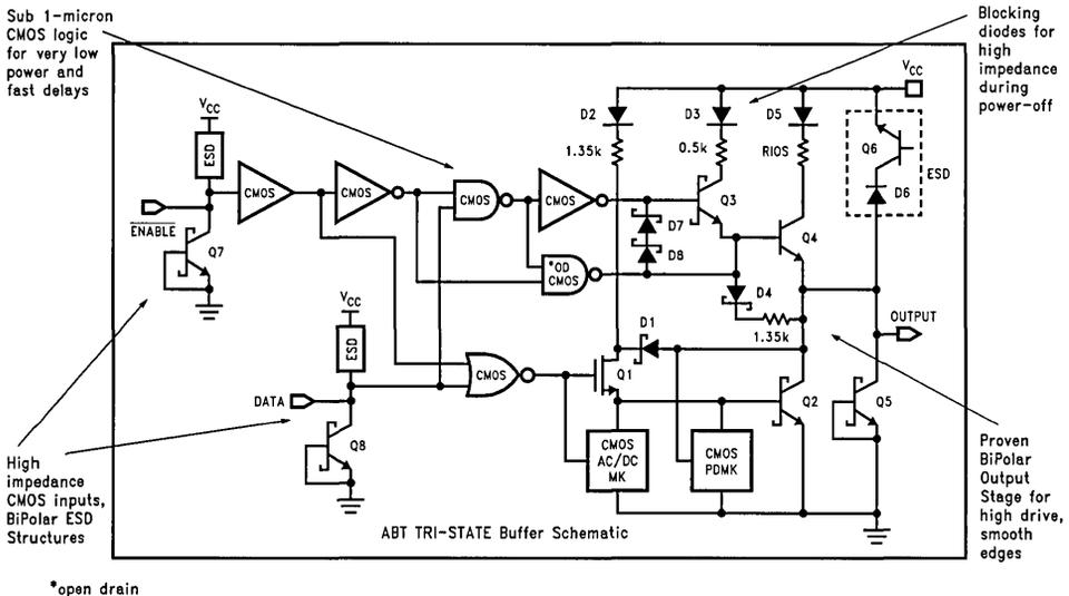
FIGURE 3. Basic ABT TRI-STATE Buffer Schematic
