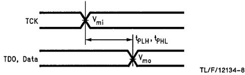
**FIGURE 8. Propagation Delay**
