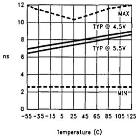
**$t_{PHL}$  (CP to  $O_n$ ) vs Temperature**
