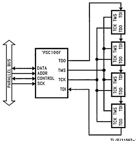
**FIGURE 1. Parallel/Serial Converter, National's Embedded Boundary Scan Controller, SCANPSC100F, General Application**
