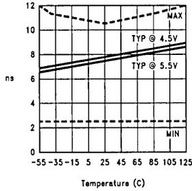
**$t_{PHL}$  (LE to  $O_n$ ) vs Temperature**
