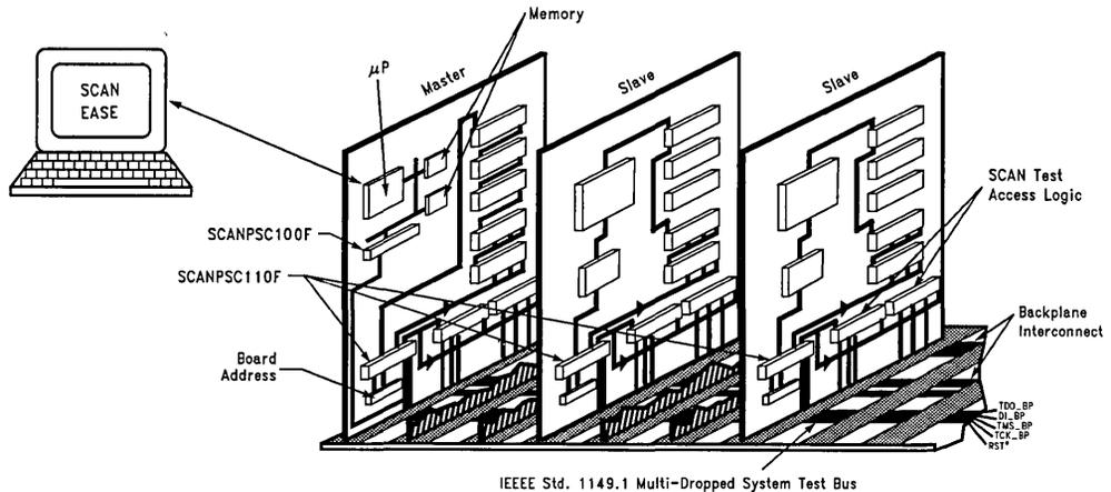
FIGURE 3. Embedding SCAN EASE for System Level Test
