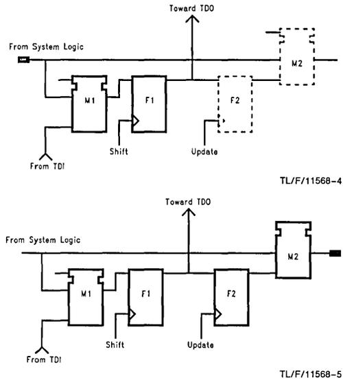
**FIGURE 4. With IEEE 1149.1 I/O Pins May Capture the Data Arriving at a Pin and They May Be Used to Control Output Pins. Test Circuits Such as These May Also Test Internal System Logic. Circuits Such as These are Added to All System Pins**
