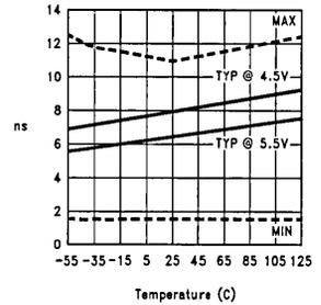
**$t_{pZL}$  ( $\overline{OE}$  to  $A_n/B_n$ ) vs Temperature**
