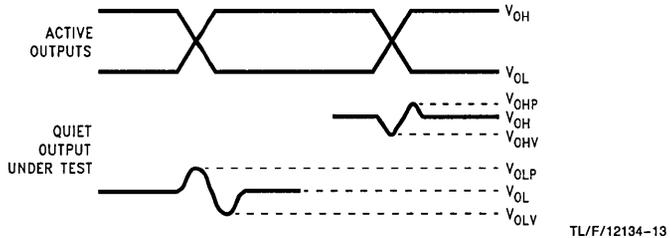
**FIGURE 13. Quiet Output Noise Voltage Waveforms**
