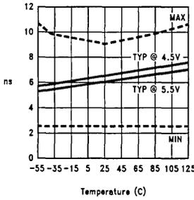
**$t_{PHL}(I_n \text{ to } O_n)$  vs Temperature**
