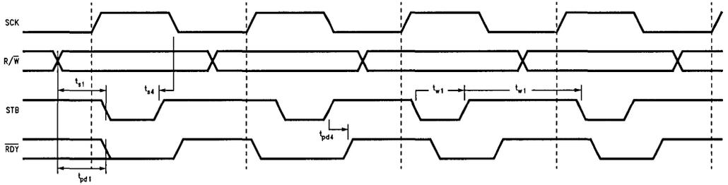
FIGURE 6. Read/Write or Write/Read (best case timing)
