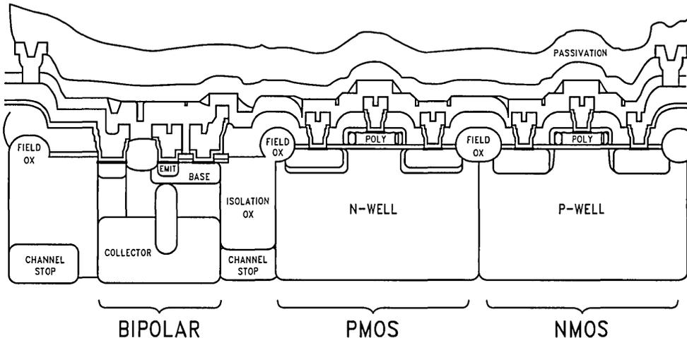
FIGURE 10. 1.0  $\mu\text{m}$  BCT Process Cross Section
