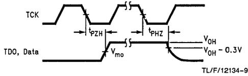
**FIGURE 9. TRI-STATE Output High Enable and Disable Times**
