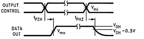
**FIGURE 3. TRI-STATE Output High Enable and Disable Times**
