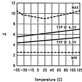
**$t_{PLH}$  ( $I_n$  to  $O_n$ ) vs Temperature**
