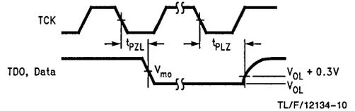
**FIGURE 10. TRI-STATE Output Low Enable and Disable Times**
