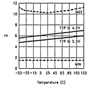
**$t_{pHZ}(\overline{OE} \text{ to } O_n)$  vs Temperature**
