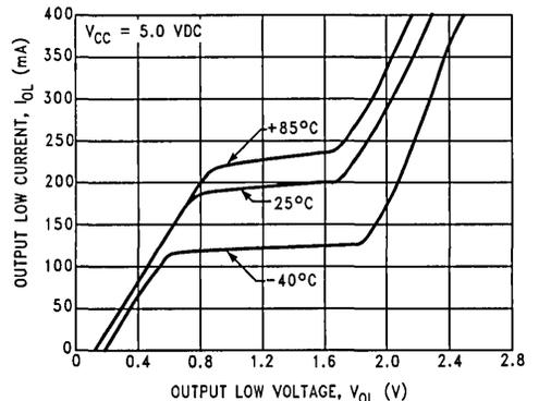
**FIGURE 7. Output Low Characteristics**
