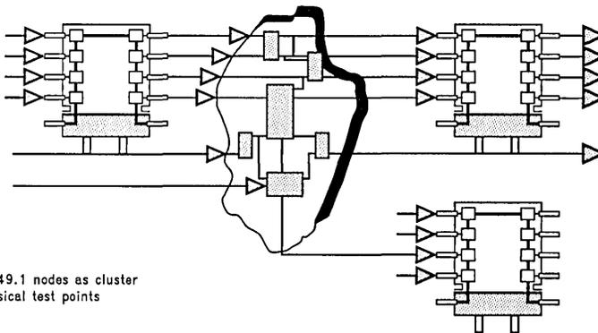
Treating non-IEEE 1149.1 nodes as cluster can eliminate ICT physical test points
