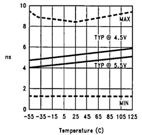
**$t_{pHZ}$  ( $\overline{OE}$  to  $A_n/B_n$ ) vs Temperature**
