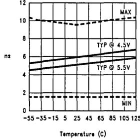
**$t_{pHZ}$  ( $\overline{OE}$  to  $O_n$ ) vs Temperature**
