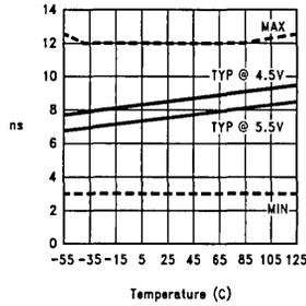
**$t_{PLH}$  (LE to  $O_n$ ) vs # Outputs Switching**
