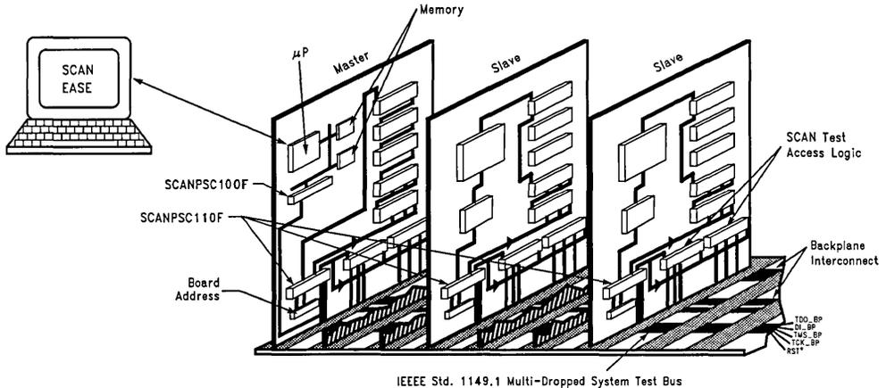
**FIGURE 3. Multidrop Configuration Using Boundary-Scan**
