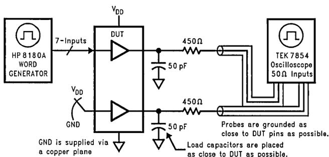
FIGURE 12. Simultaneous Switching Test Circuit
