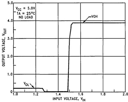
**FIGURE 4. Buffer Transfer Function @ Room Temperature**
