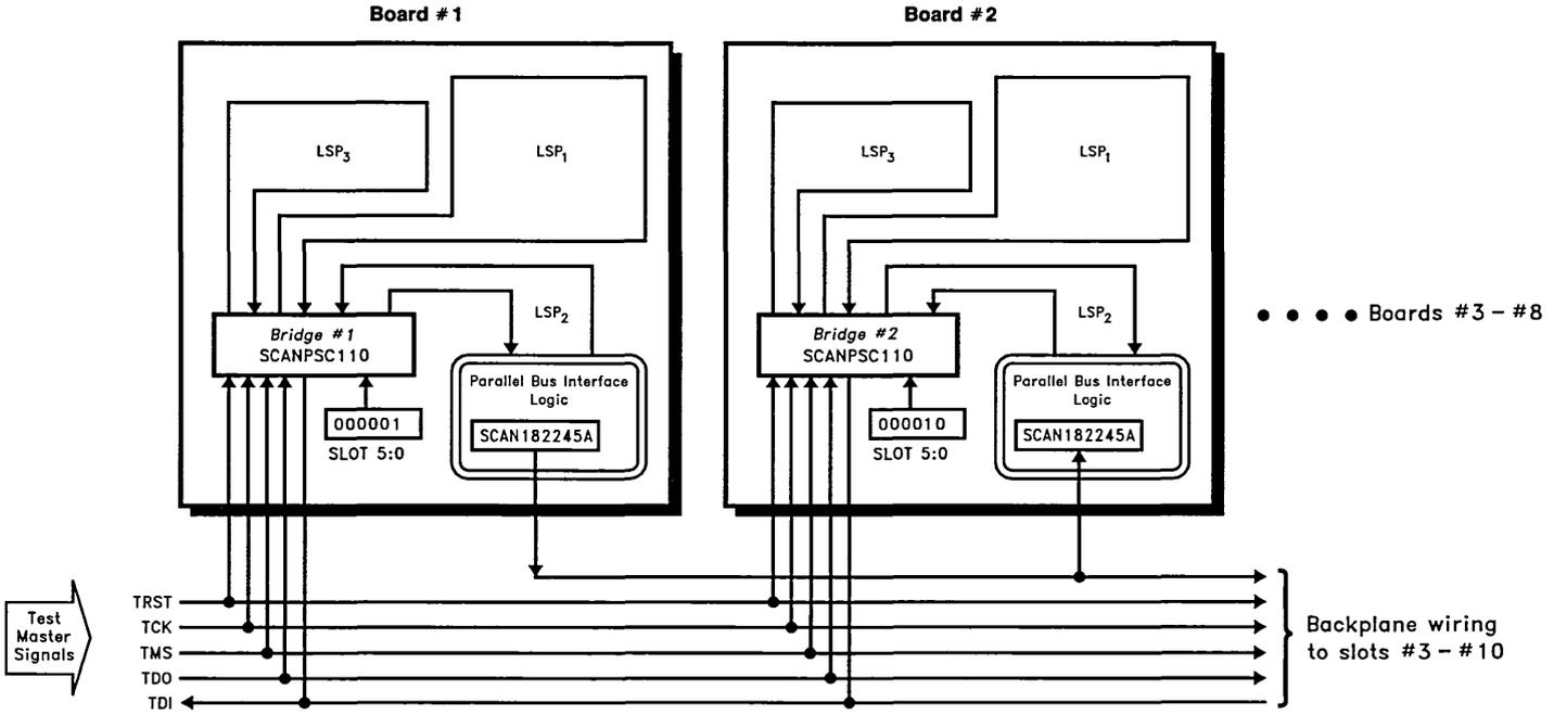
FIGURE 19. Testing the Backplane Interconnections
