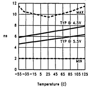
**$t_{PZH}(OE \text{ to } O_n)$  vs Temperature**
