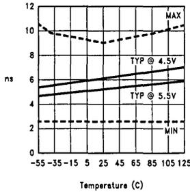
**$t_{PLH}(I_n \text{ to } O_n)$  vs Temperature**
