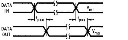
**FIGURE 1. Waveform for Inverting and Non-Inverting Functions**
