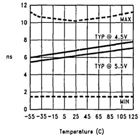
**$t_{pLZ}(\overline{OE} \text{ to } O_n)$  vs Temperature**
