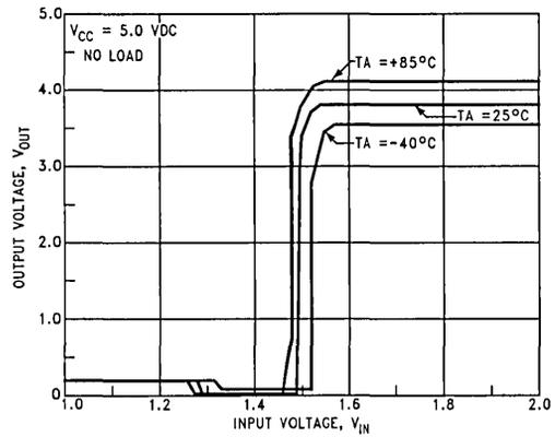
**FIGURE 6. Transfer Function vs Temperature**
