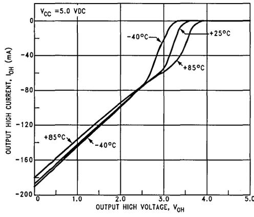
FIGURE 8. Output High Characteristics
