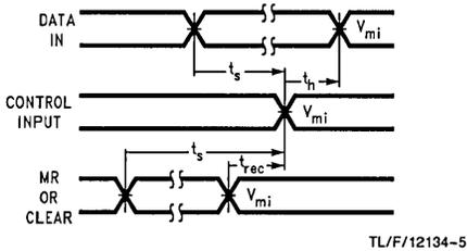
**FIGURE 5. Setup Time, Hold Time and Recovery Time**
