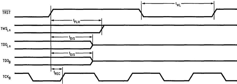
FIGURE 15. Reset Waveforms
