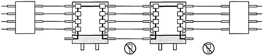
Boundary scan works with an ICT to provide access to inaccessible nodes and/or to reduce ICT physical test points
