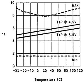
**$t_{PHL}$  (A to B/B to A) vs Temperature**
