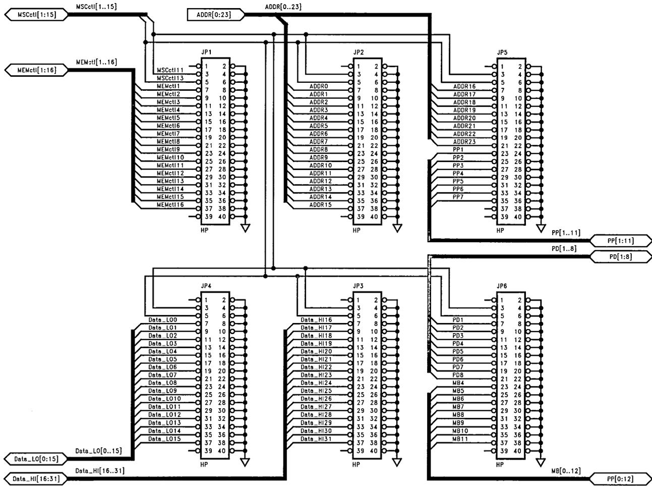
FIGURE 14. HP Logic Analyzer Interface
