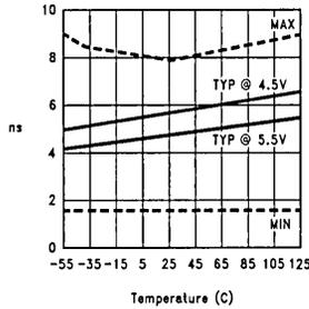
**$t_{PLH}$  (A to B/B to A) vs Temperature**
