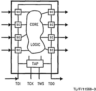
**FIGURE 3. Bed-of-Nails Test Access Has Been Replaced by Adding Embedded Test Probes to Each IC Input and by Providing Test Drivers at Each Output. Driving Outputs and Sampling Inputs is Called EXTEST**
