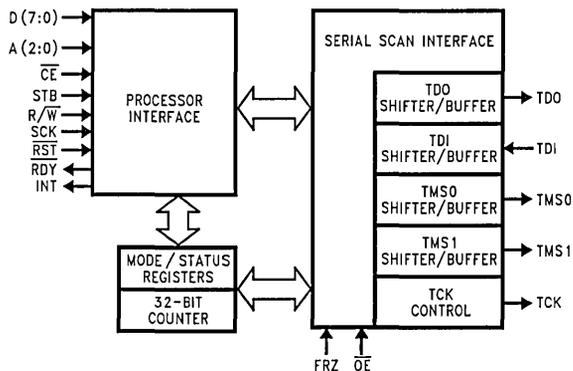
FIGURE 2. Embedded Boundary Scan Controller, SCANPSC100F Architecture
