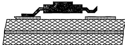
**FIGURE 5. Lifted IC Leads, Not Accessible with Bed-of-Nails by the Embedded Probes of the Driving and Receiving IC, if they Implement Boundary-Scan**
