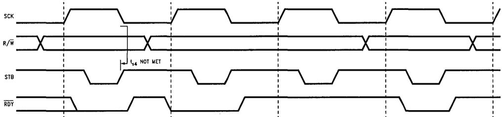
FIGURE 7. Read/Write or Write/Read (worst case timing)
