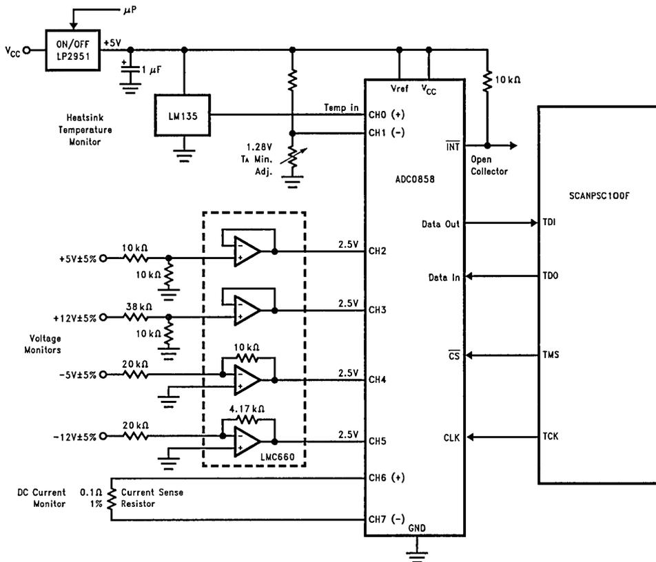
ADC0858CMJ/883 Monitors System Temperature, Voltage and Current
