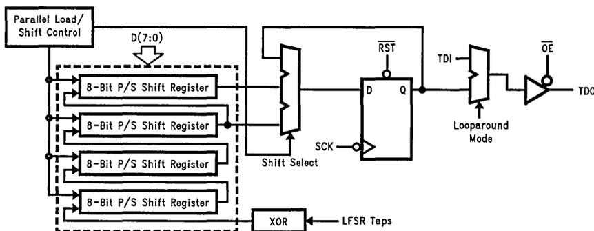
FIGURE 11. TDO Shifter/Buffer Block Diagram Register Hookup
