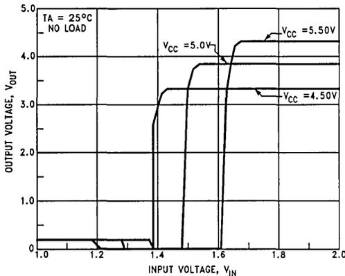
**FIGURE 5. Transfer Function vs  $V_{CC}$**
