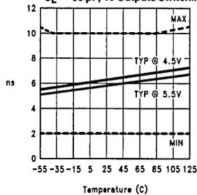
**$t_{pLZ}$  ( $\overline{OE}$  to  $A_n/B_n$ ) vs # Outputs Switching**
