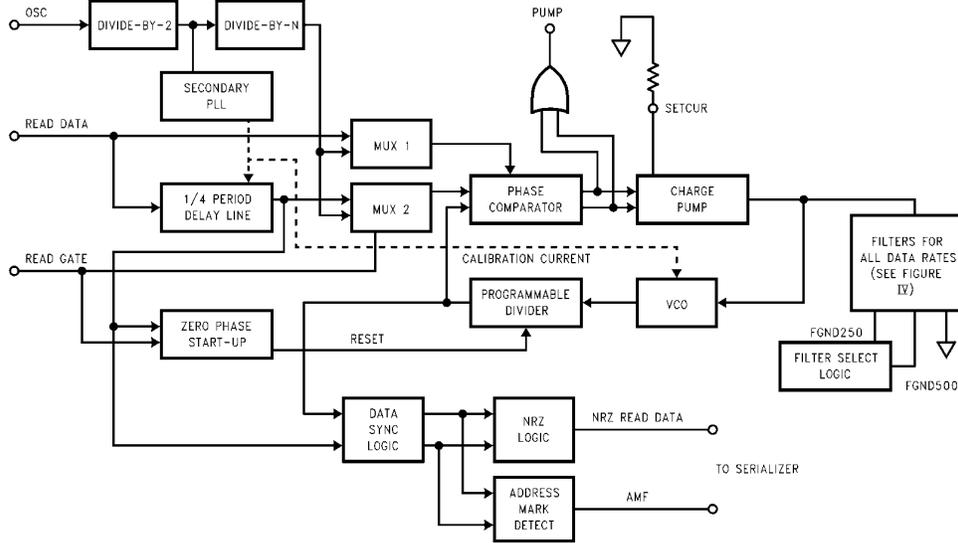
FIGURE 3. Block Diagram of DP8473's Data Separator
