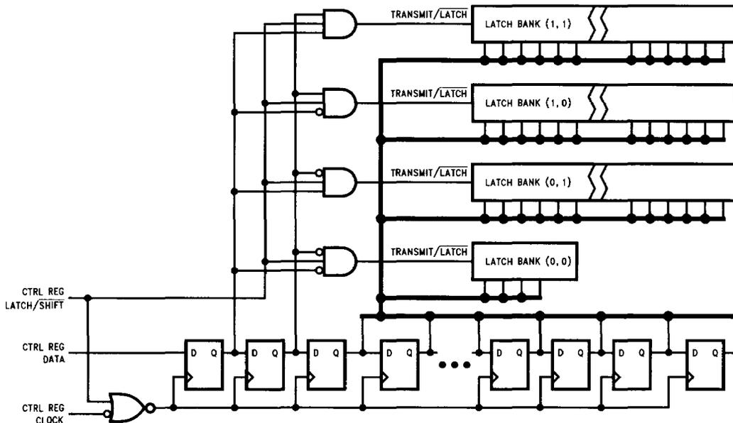
FIGURE 5. Control Register Block Diagram
