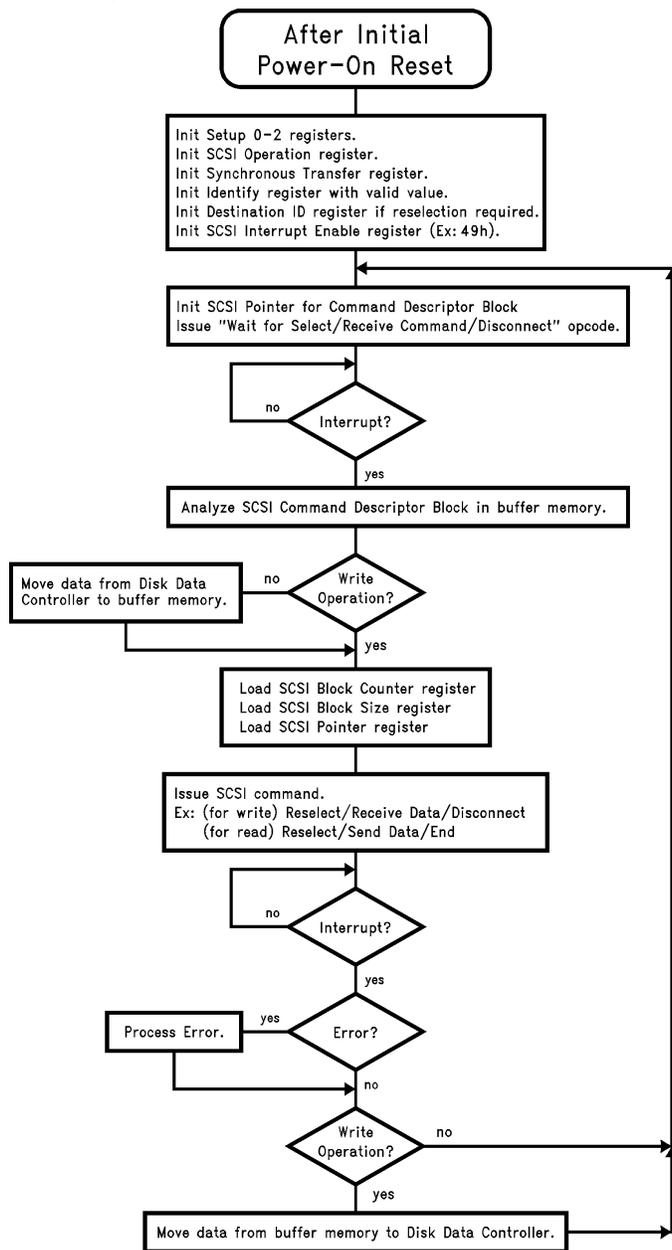
FIGURE 4.11. Software Flowchart for Simple SCSI Operation
