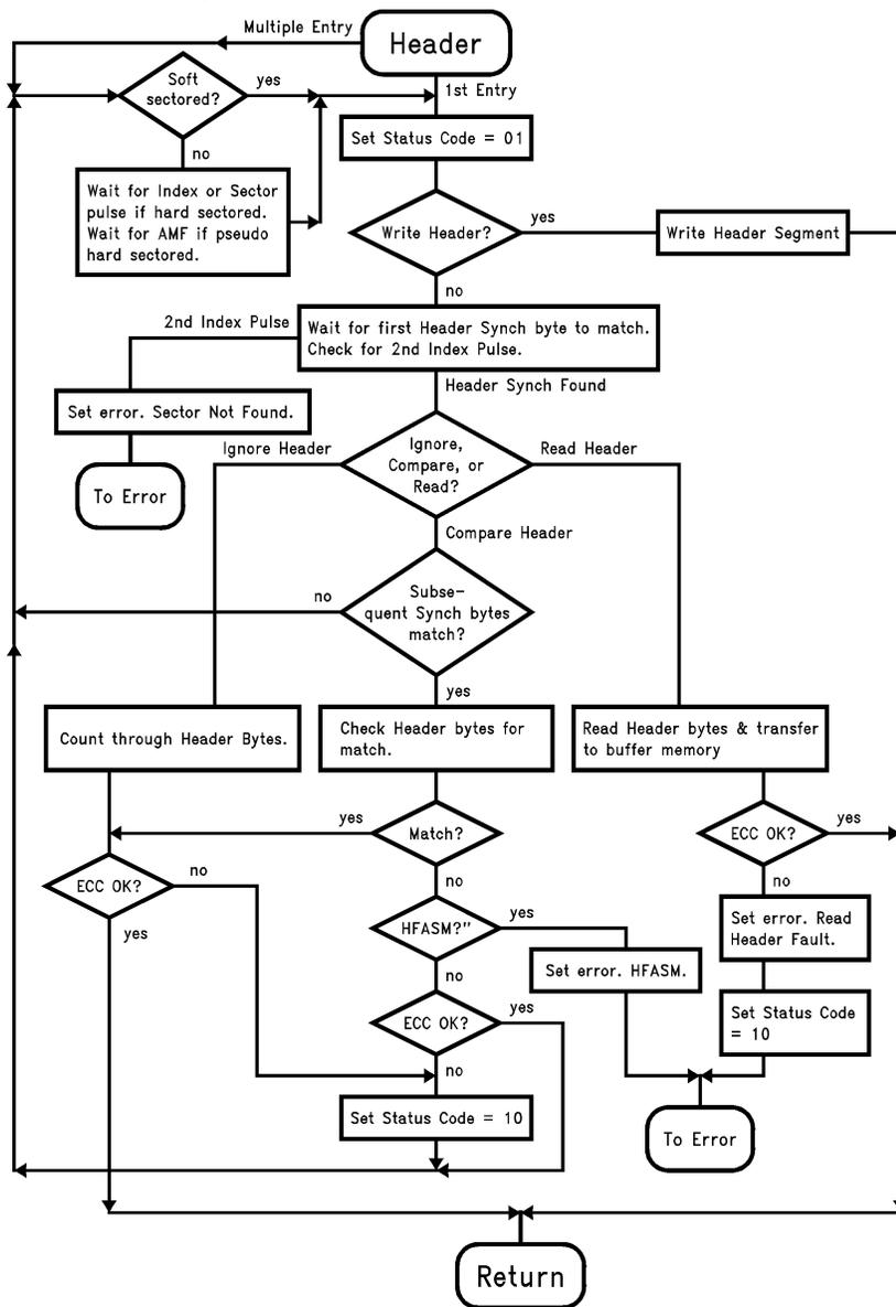
Note: HFASM = Header Failed Although Sector Matched as enabled in the Header Byte Control registers.
