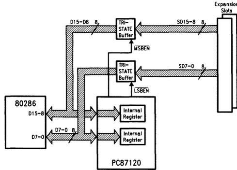
(a) 16-Bit Transfer During Expansion Bus Access
