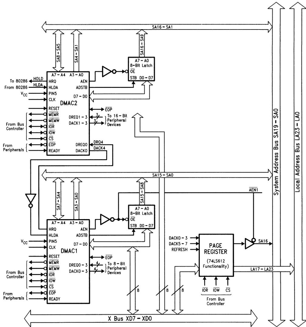
FIGURE 10-1. PC87120 DMA System
