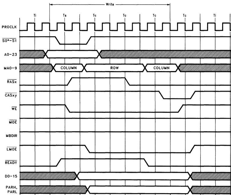
FIGURE 6-15. Page Interleaving Mode Write Cycle Page-Miss
