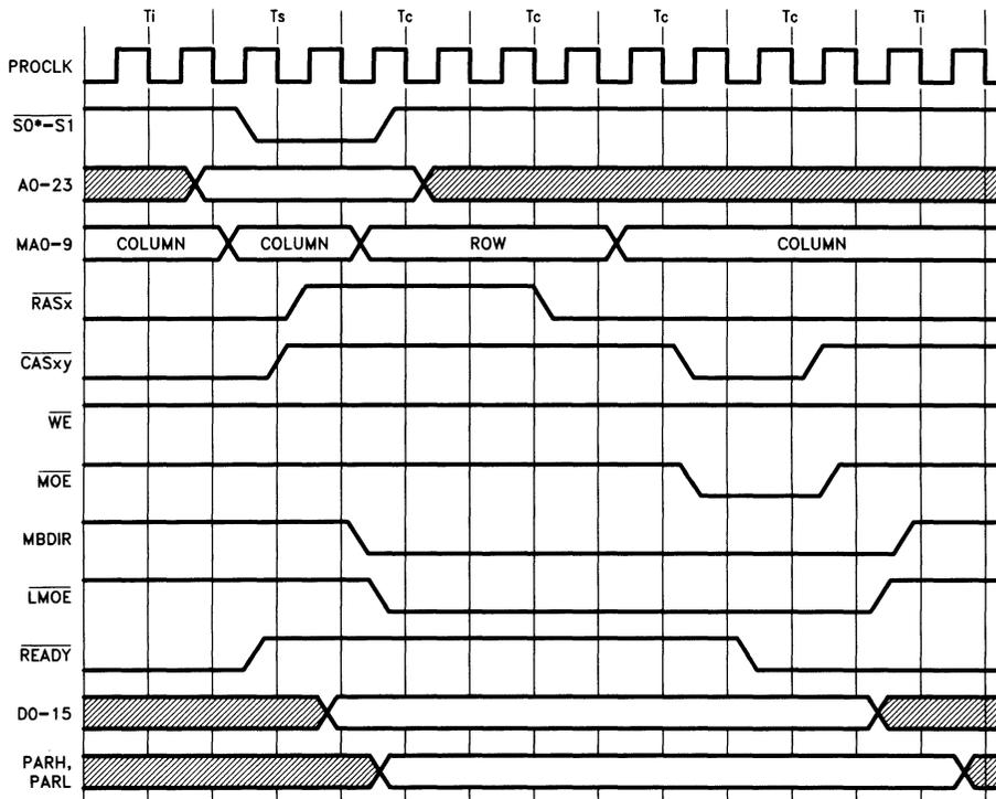
FIGURE 6-16. Page Interleaving Mode Read Cycle Page-Miss
