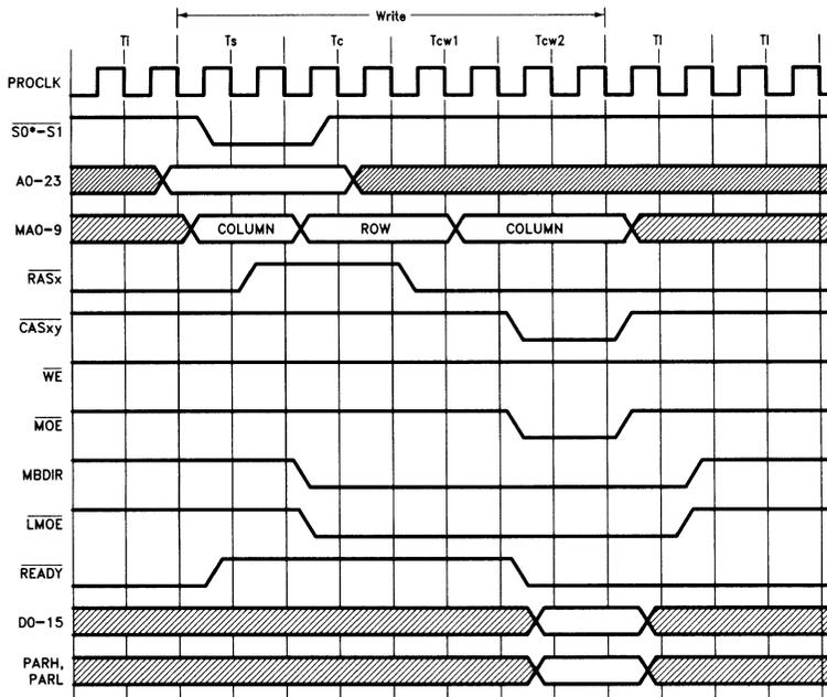
FIGURE 6-21. Enhanced Page-Interleaving Mode Page-Miss Read Cycle
