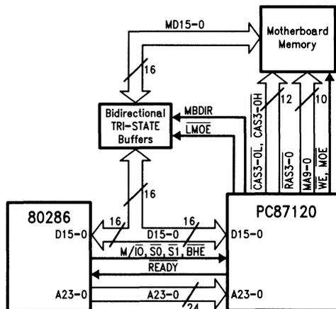
FIGURE 6-1. Typical Memory Data Bus Interface
