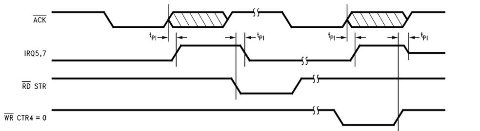
**FIGURE 9-15. Parallel Port Interrupt Timing (Extended Mode)**
