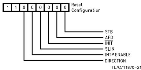
This register provides all output signals to control the printer. It is a read and write register, except for bit 5.
