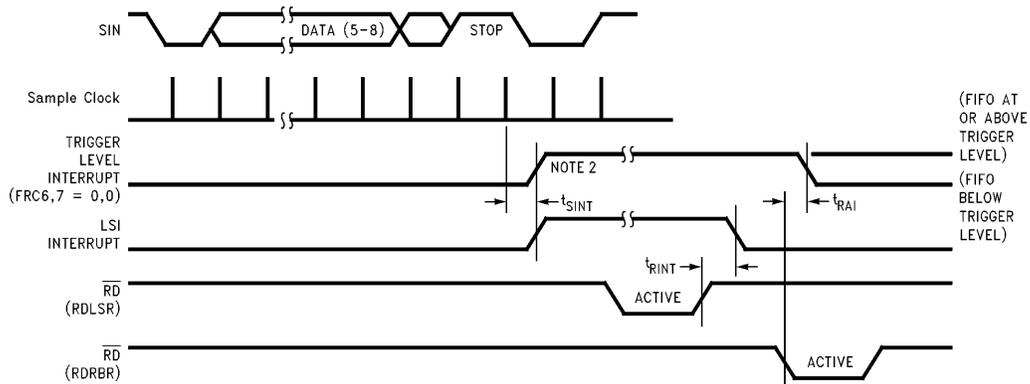
**Note 2:** If SCRO = 1, then  $t_{SINT}$  = 3 RCLKs. For a Timeout interrupt,  $t_{SINT}$  = 8 RCLKs.
