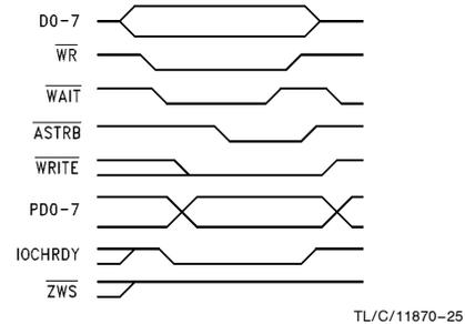
FIGURE 7-4. EPP 1.9 Address Write
