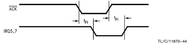
**FIGURE 9-14. Parallel Port Interrupt Timing (Compatible Mode)**
