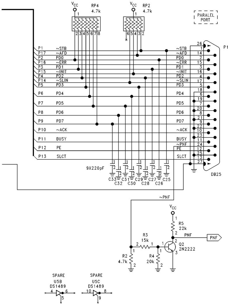
FIGURE 10-3. PC87322VF Adapter Card Schematic (Continued)
