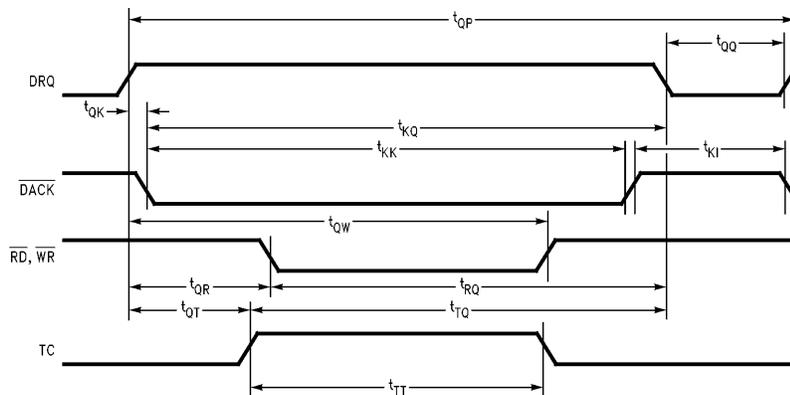
FIGURE 9-8. DMA Timing
