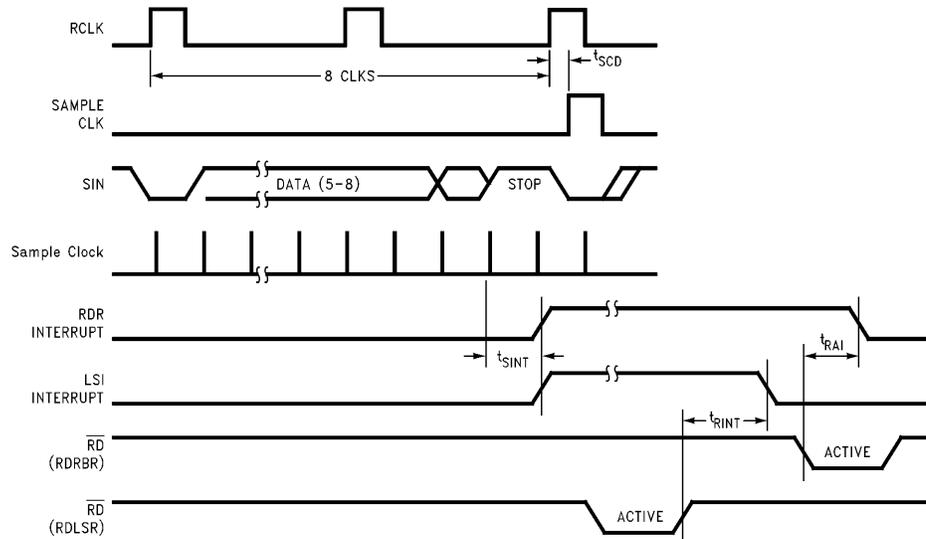
**FIGURE 9-6a. Receiver Timing**
