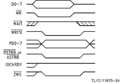
FIGURE 7-3. EPP Write with ZWS
