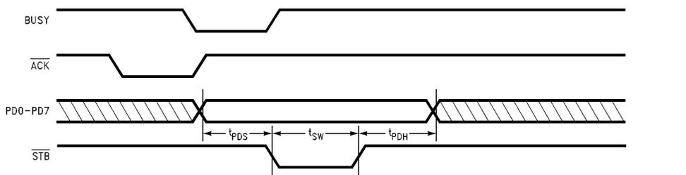
**FIGURE 9-16. Typical Parallel Port Data Exchange**
