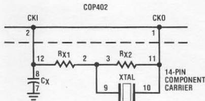
Figure 3.1. Crystal Oscillator Component Carrier Schematic
