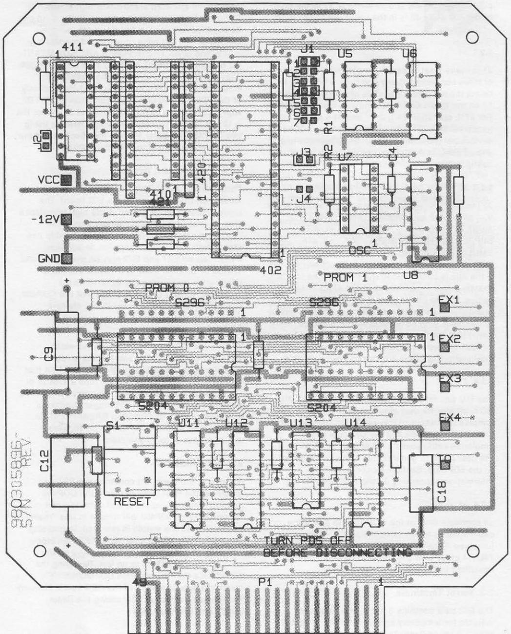
Figure 2.1. COP400-E02 In-Circuit Emulator Layout
