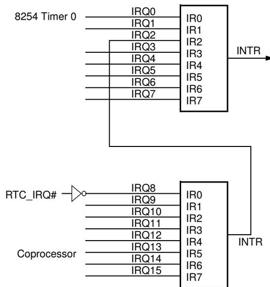
**Figure 4-15. PIC Interrupt Controllers**
