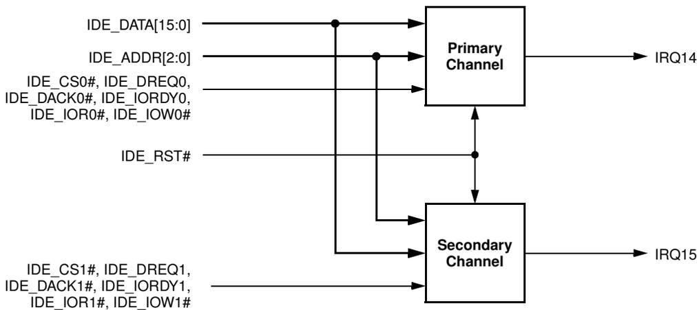
Figure 4-19. CS5530A and IDE Channel Connections
