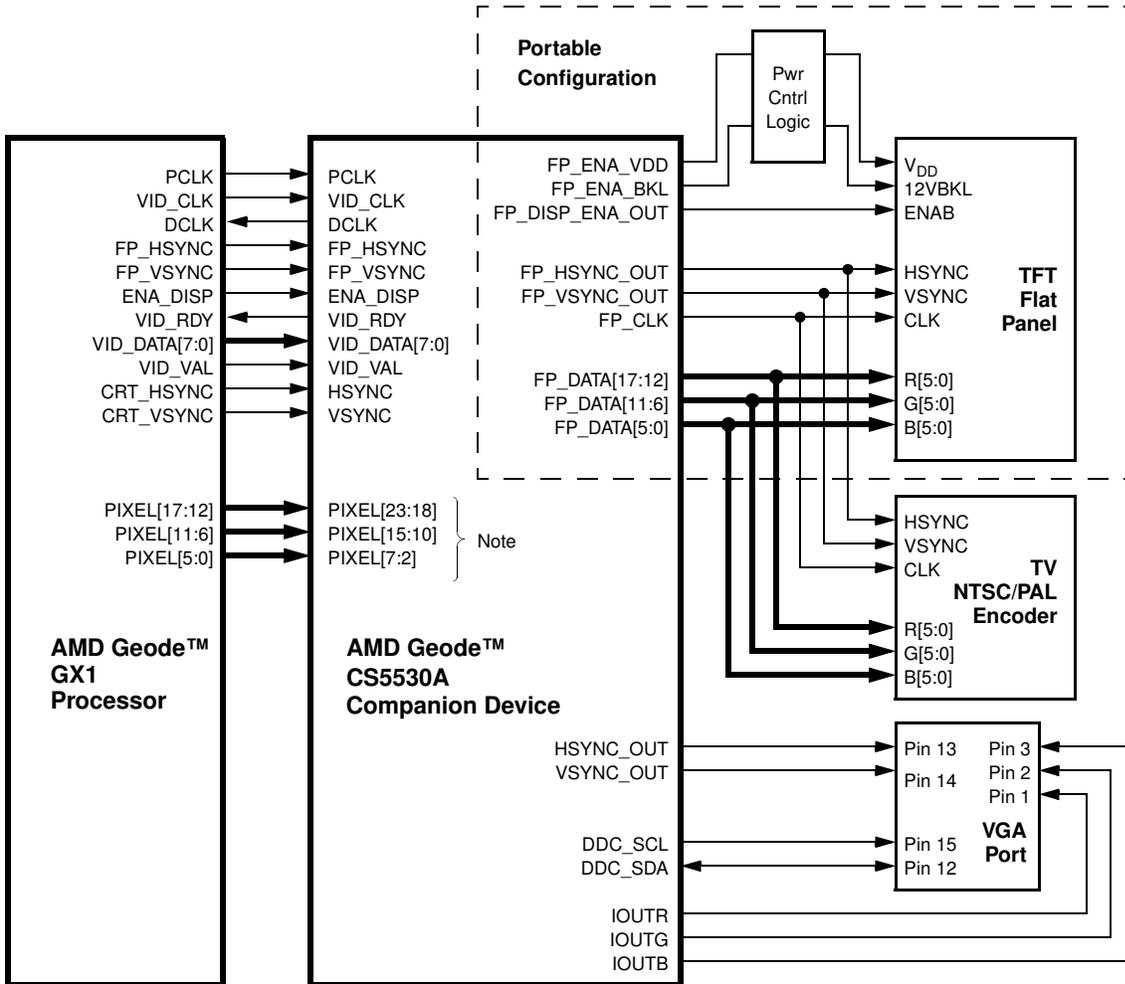
**Note:** Connect PIXEL[17:16], PIXEL[9:8], and PIXEL[1:0] on the CS5530A to ground. See Figure 4-3 "PIXEL Signal Connections" on page 50.
