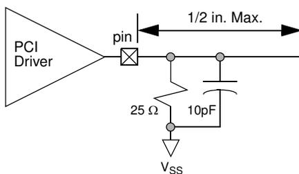
Figure 6-3. PCI Rising Edge ( $t_{LH}$ ) Test Circuit
