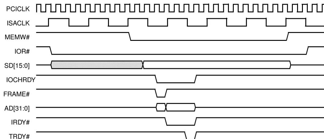
Figure 4-13. ISA DMA Write To PCI Memory
