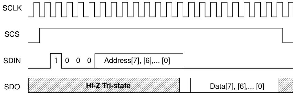
**Figure 3-3. Serial Interface Read Cycle Timing Diagram**
