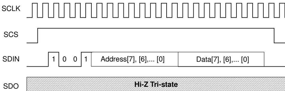
**Figure 3-4. Serial Interface Write Cycle Timing Diagram**
