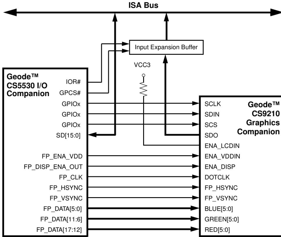
**Figure 3-2. Connection Method Using Input Expansion Buffer**
