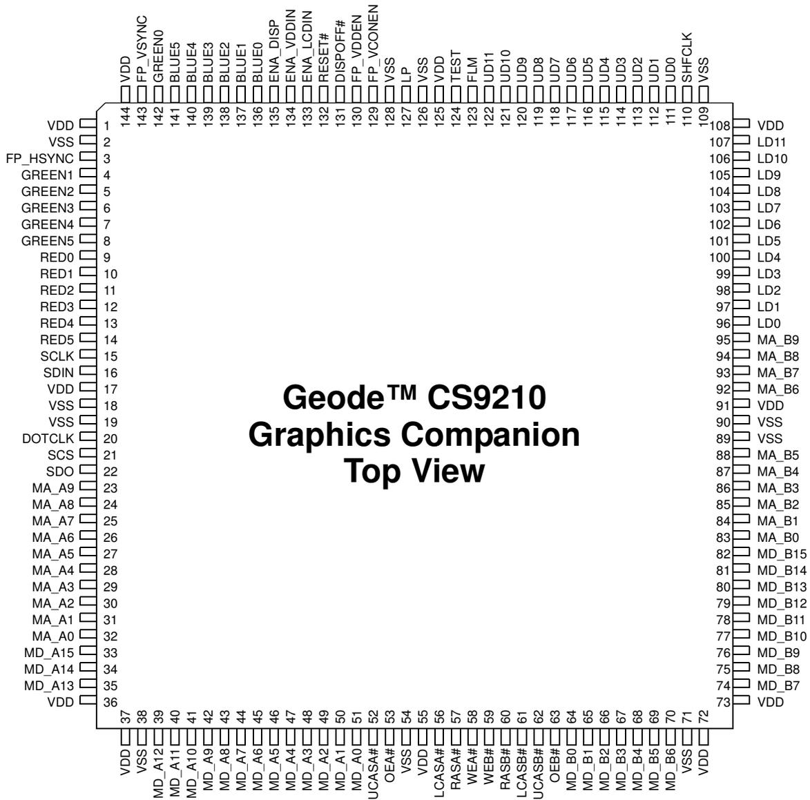
Figure 2-2. 144-Pin LQFP Pin Assignment Diagram
