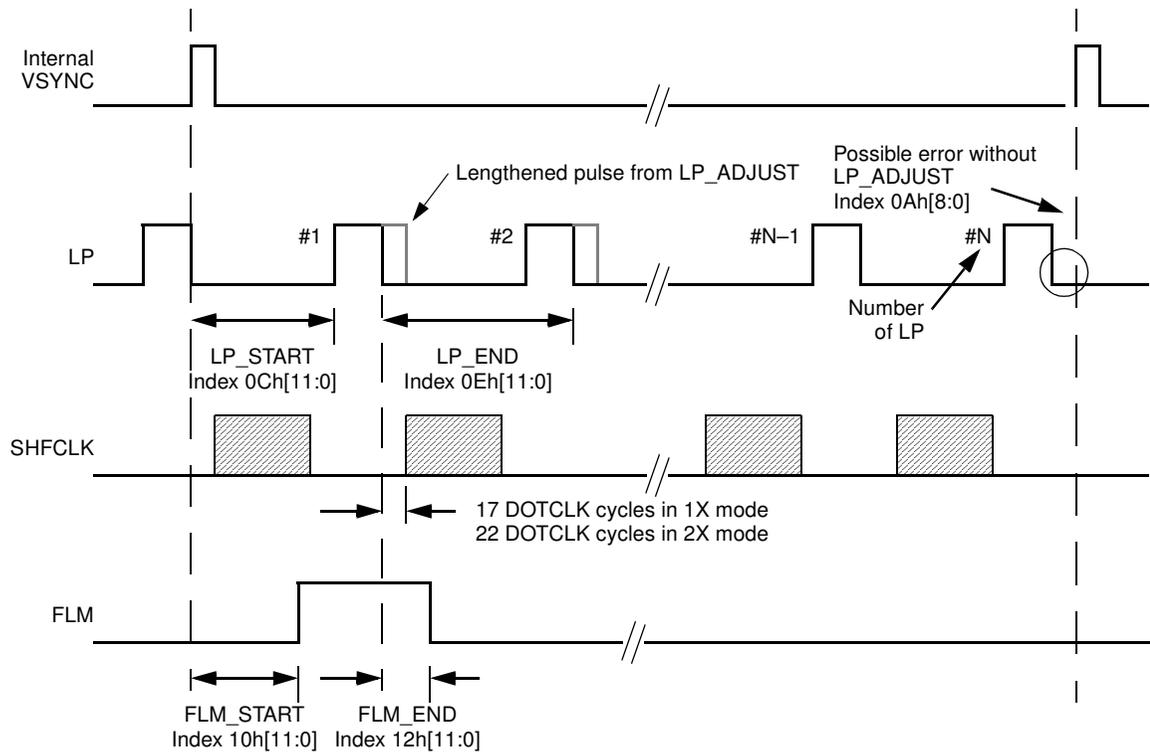
**Note:** Internal VSYNC is a pulse internal to the CS9210, triggered by a rising edge on the FP\_VSYNC input.
