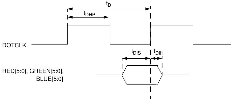
**Figure 5-2. Pixel Port Interface Signals**
