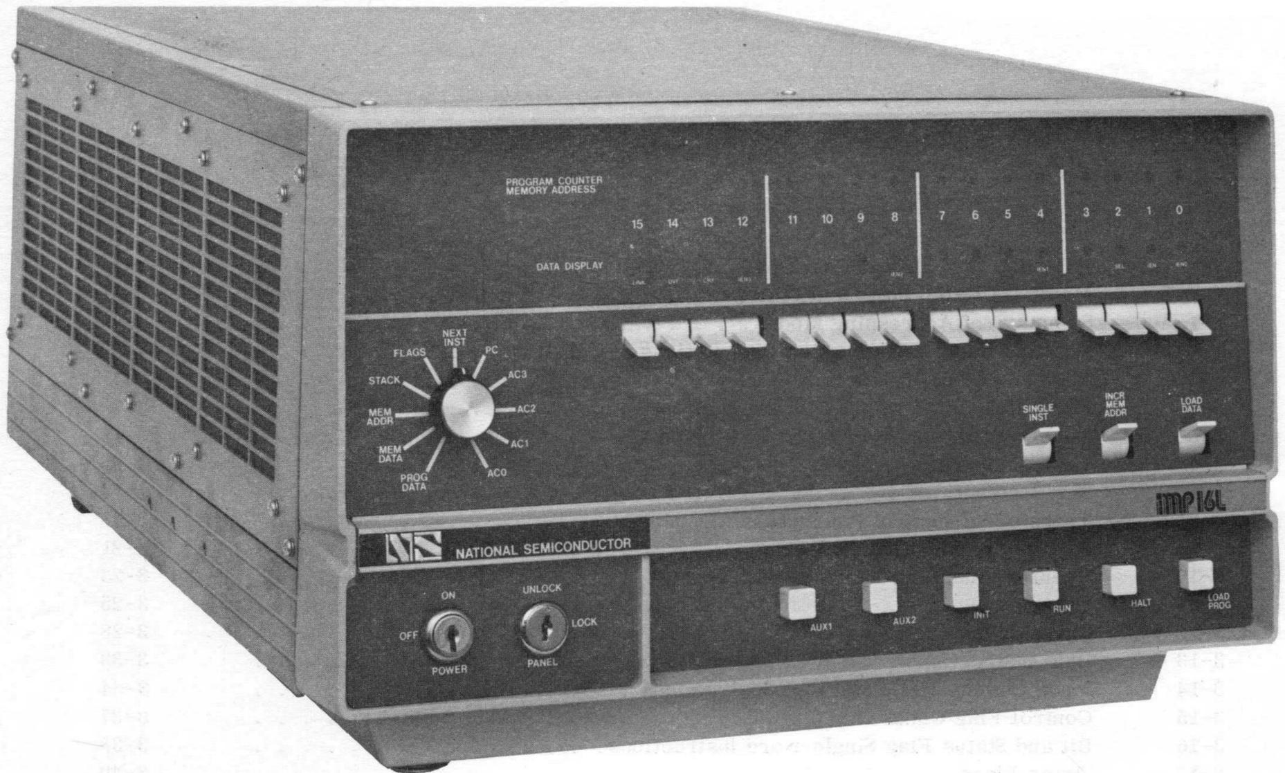
Figure 1-1. IMP-16L Microcomputer
