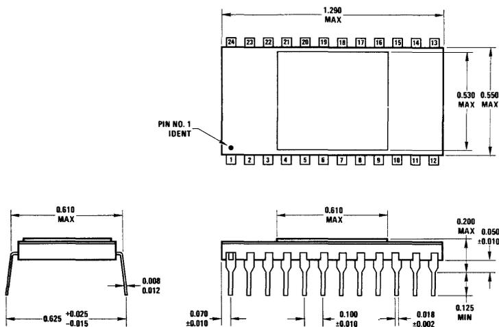
Cavity Dual-In-Line Package (D)
