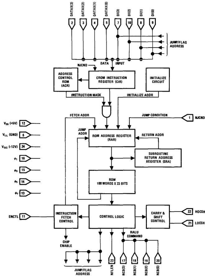
FIGURE 1. CROM Block Diagram
