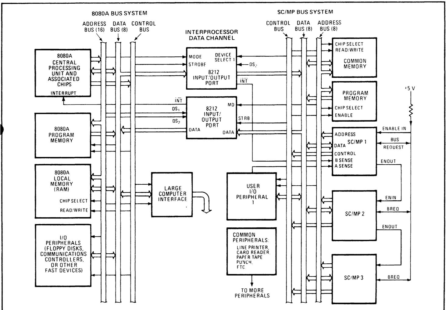
**1. Multiprocessor.** One 8080 and three SC/MPs are combined, each type of device handling jobs appropriate to its capability. SC/MP 1 supervises transfer of data between the other processors, as well as serving an interface with the operator's I/O device.
