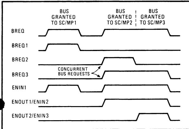
**4. Bus access.** The SC/MPs are connected in a priority arrangement for access to the common bus. SC/MP 1 has the highest priority, and even if SC/MP 3 has a concurrent request with SC/MP 2, it must wait until SC/MP 2 completes its operations.
