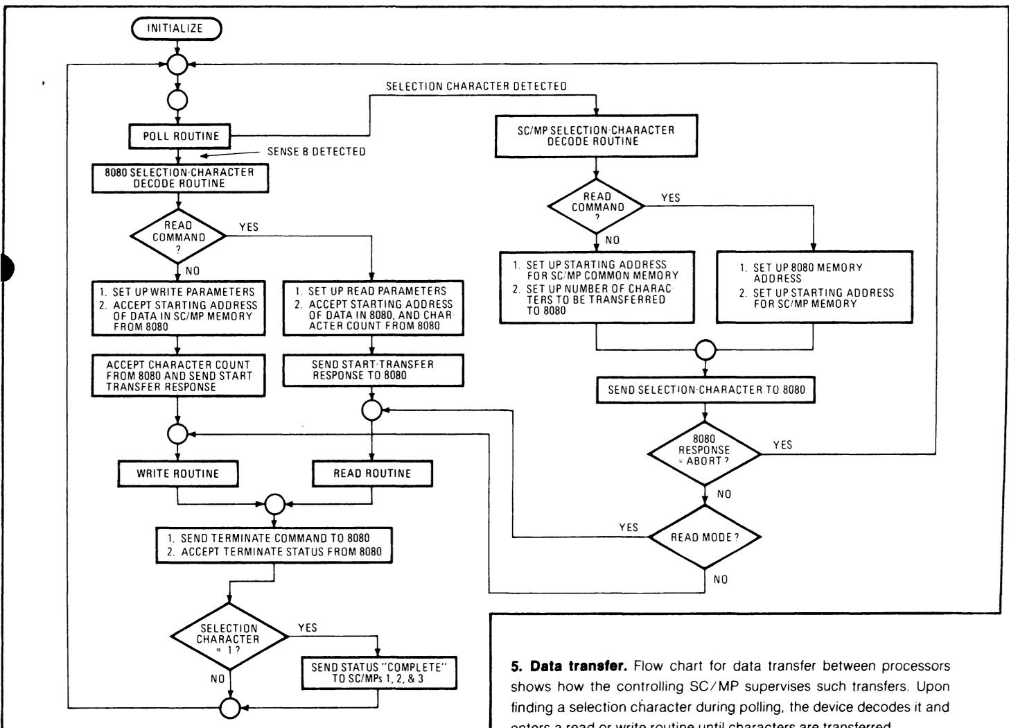
**5. Data transfer.** Flow chart for data transfer between processors shows how the controlling SC/MP supervises such transfers. Upon finding a selection character during polling, the device decodes it and enters a read or write routine until characters are transferred.
