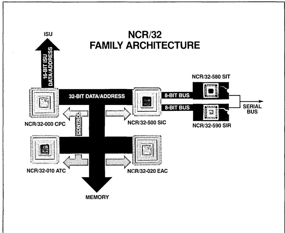
The NCR/32 VLSI Processor family consists of the Central Processor Chip (CPC), the Address Translation Chip (ATC), and the System Interface Controller (SIC). Additional members of the family include the Extended Arithmetic Chip (EAC), the System Interface Transmitter (SIT) and Receiver (SIR) chips, and the Bus Assist Chip (BAC).
