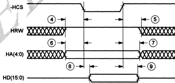
Figure 10 Host Interface Read Timing
