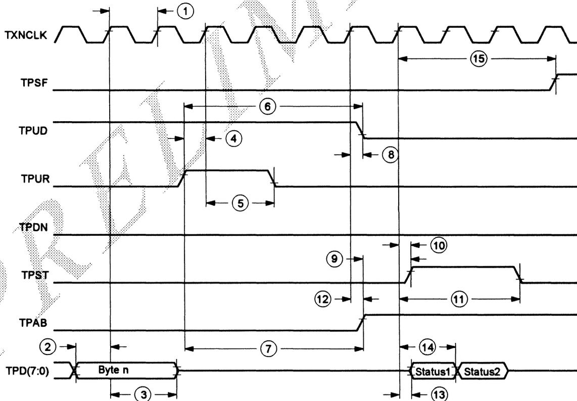
Figure 14 Buffer Management Interface Transmit Underrun Abort Timing
