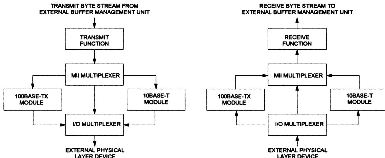
Figure 6 Transmit and Receive Data Paths
