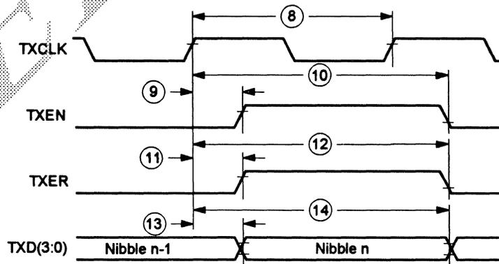
Figure 17 MII Transmit Function Timing
