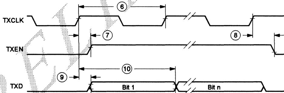
Figure 24 10BASE-T Transmit Function Timing
