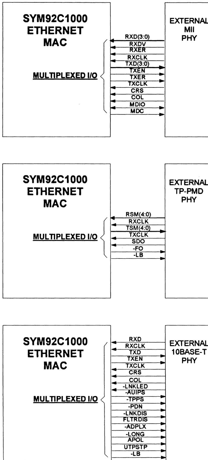
**Figure 4 Three Options for Multiplexed I/O**
