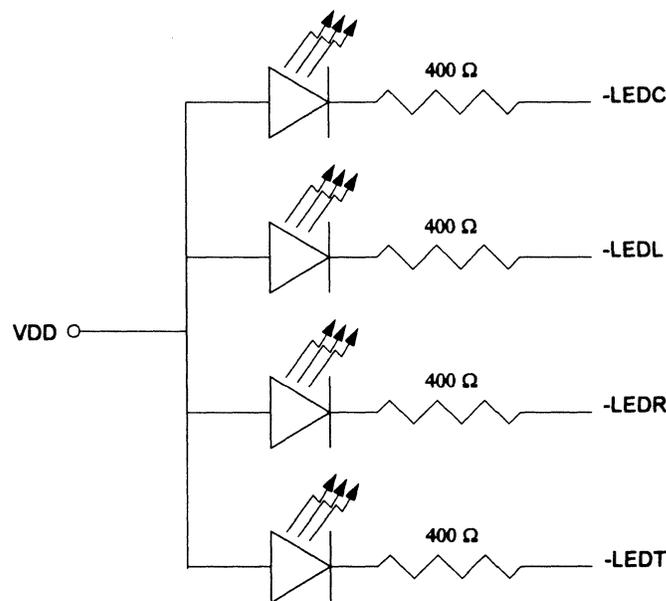
Figure 5 Typical LED Circuit
