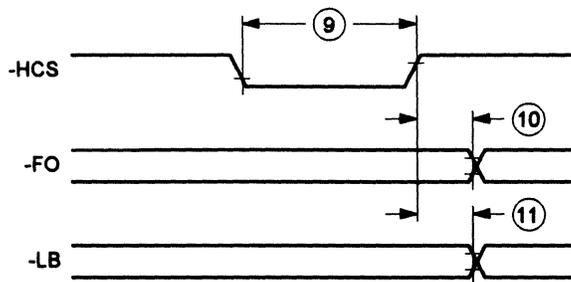
Figure 22 TP-PMD Control Function Timing
