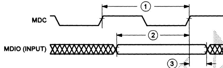
**Figure 18 MII Management Input Timing**
