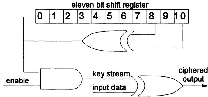
**Figure 8 Ciphering Circuit**
