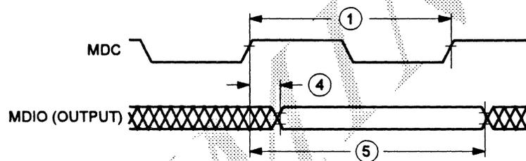
**Figure 19 MII Management Output Timing**
