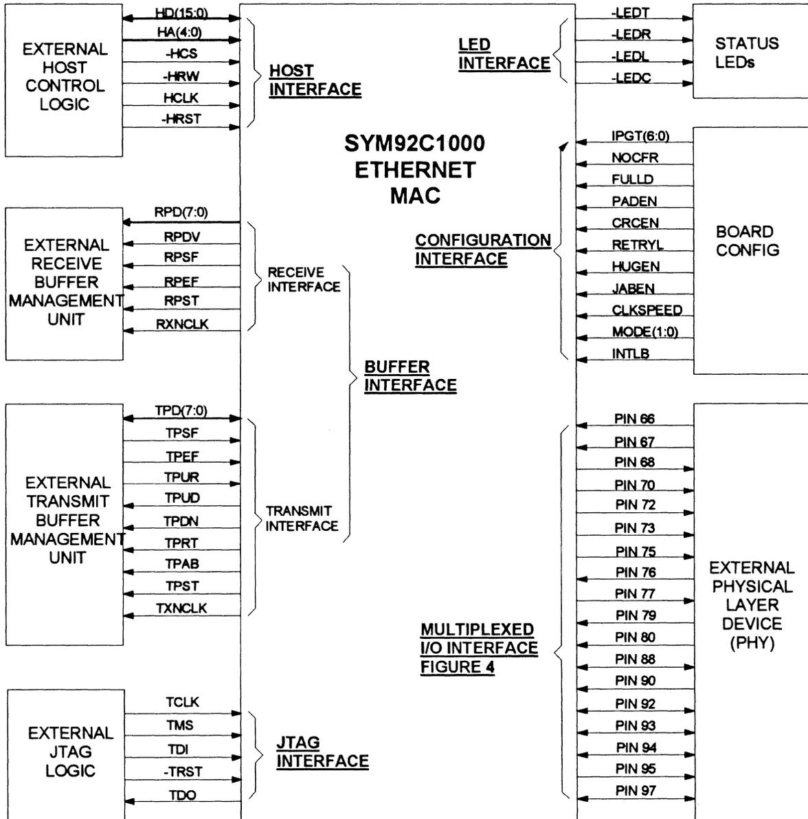
**Figure 3 System Block Diagram**
