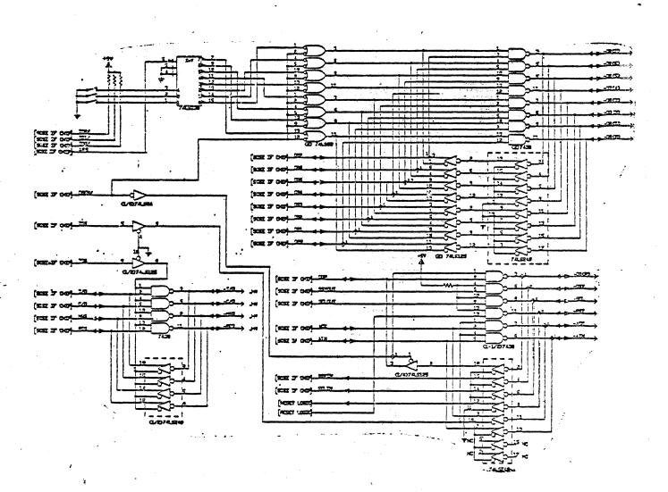
Figure D3. Suggested Interface to SCSI Single-Ended Drivers/Receivers
