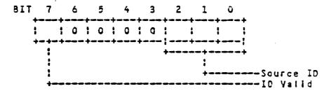
The IC Valid bit indicates that the source device placed its own ID bit on the SCSI bus during the Selection phase and therefore the chip has encoded that ID and placed it in bits 2-0. This information remains valid until the chip disconnects from the SCSI bus.
