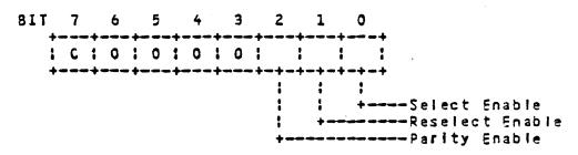
Bit 2 Parity Enable When the Parity Enable bit is a \*1\*, the chip generates and checks parity on all transfers on the SCSI bus. When the Parity Enable bit is a \*0\*, the chip generates, but does not check parity on bus transfers.
