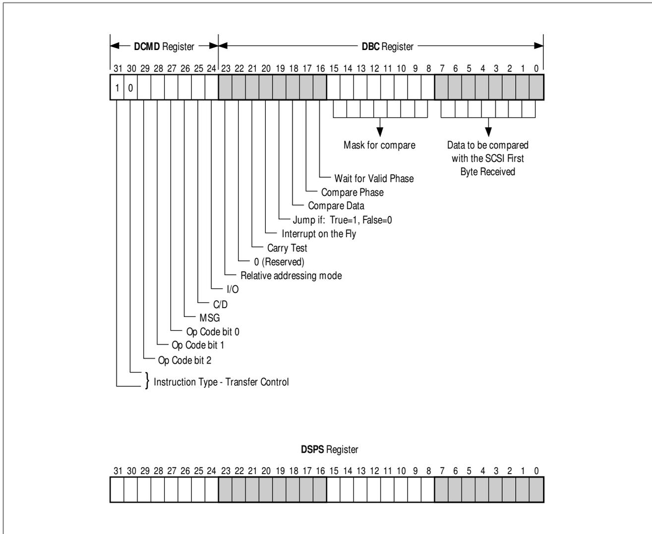
**Figure 5-5: Transfer Control Instruction Register**
