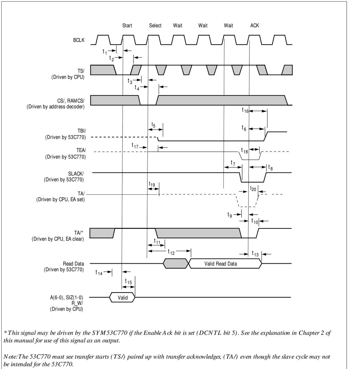
**Figure 6-17: Bus Mode 2 Slave Read Waveforms**
