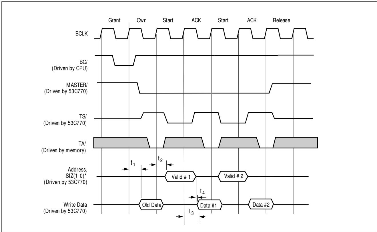
**Figure 6-26: Mux Mode Write Cycle (Non-Cache Line Burst)**
