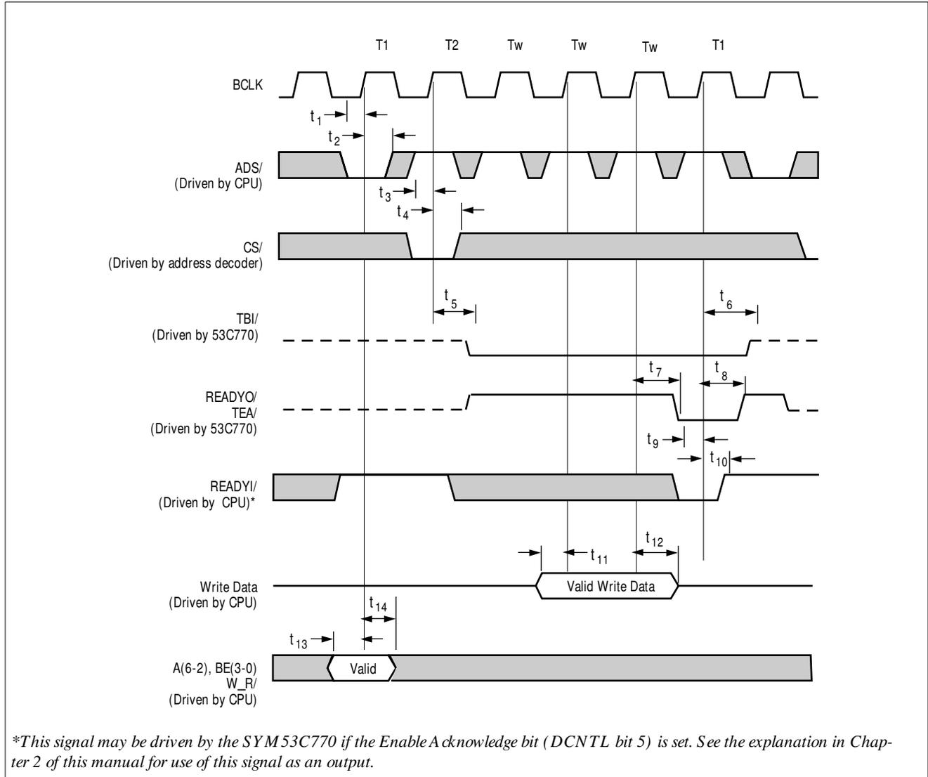
**Figure 6-29: Bus Mode 3 and 4 Slave Write Cycle**
