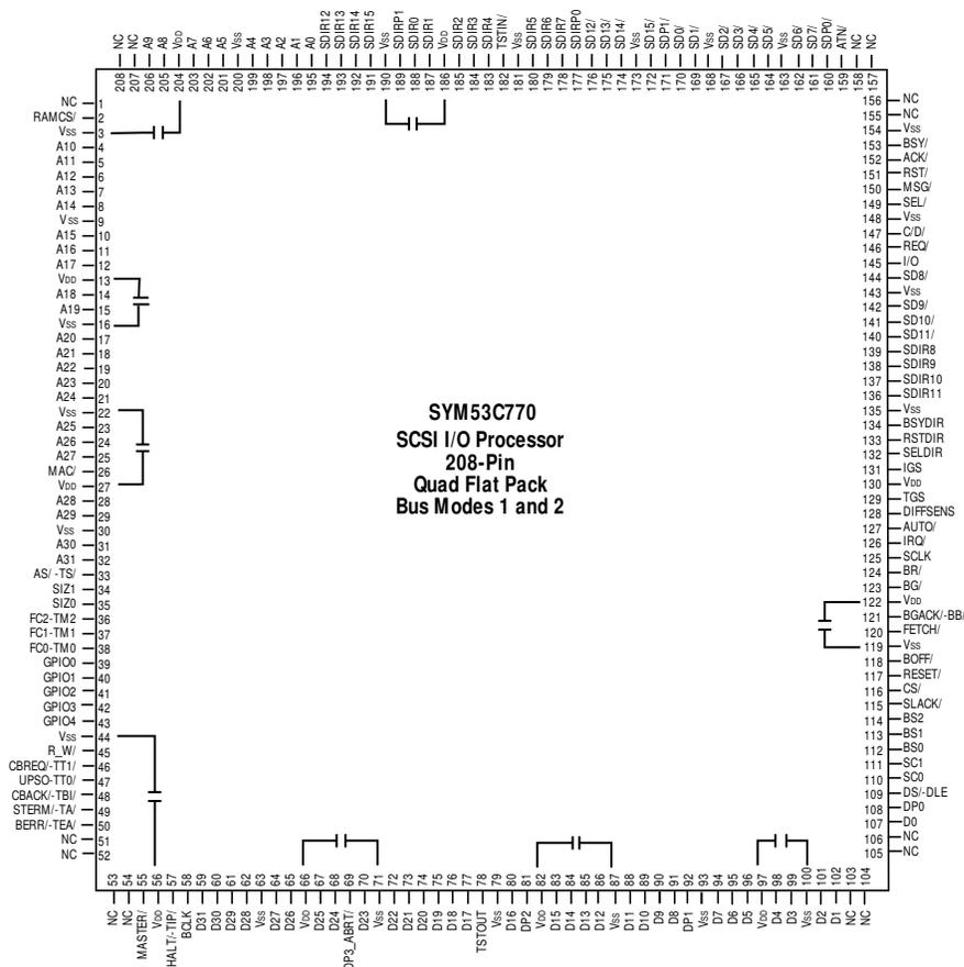
Note: the decoupling capacitor arrangements shown above are recommended to maximize the benefits of the internal split ground system. Capacitor values between 0.01 and 0.1  $\mu\text{F}$  should provide adequate noise isolation. Because of the number of high current drivers on the SYM53C770, a multi-layer PC board with power and ground planes is required.
