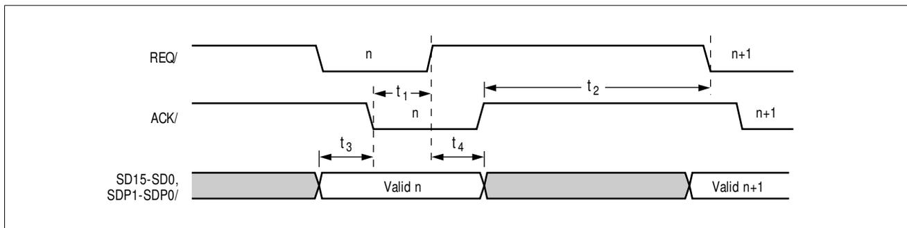
Figure 6-41: Target Asynchronous Receive
