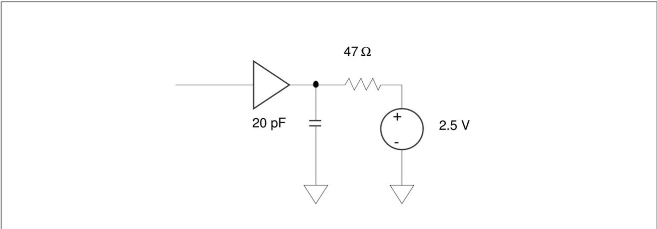
**Figure 6-1: Rise and Fall Time Test Conditions**
