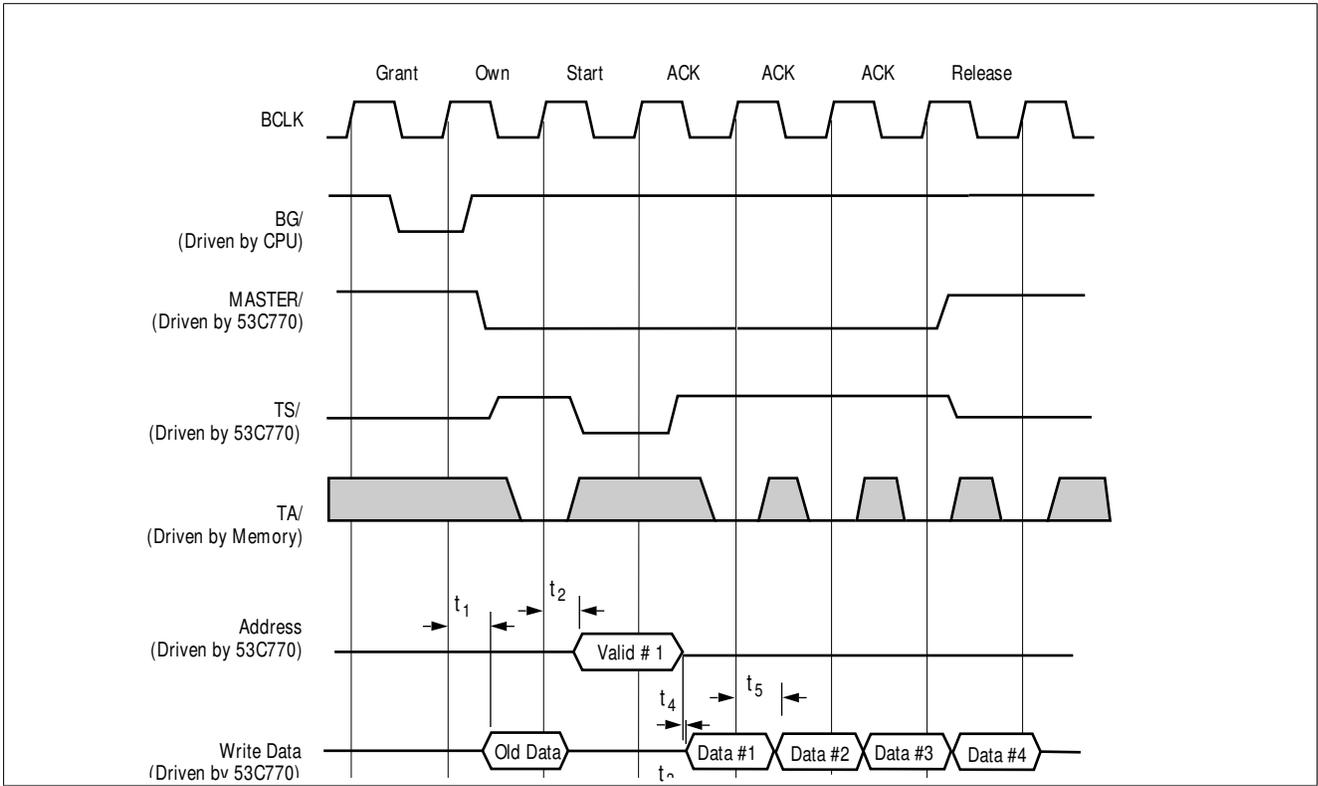
**Figure 6-27: Mux Mode Write Cycle (Cache Line Burst)**
