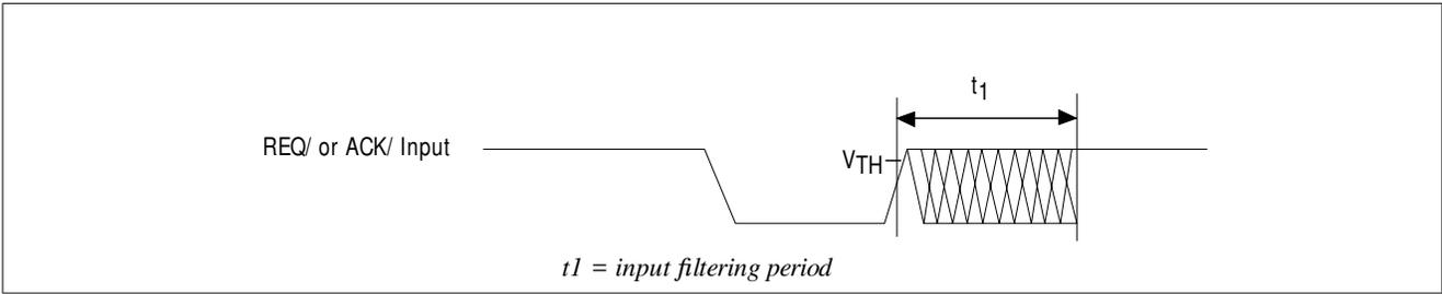
**Figure 6-2: SCSI Input Filtering**
