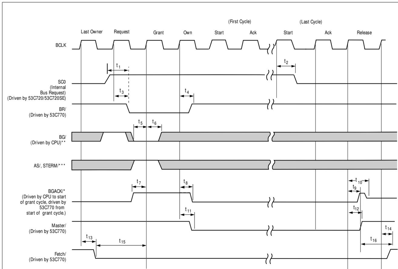
\*If the Fast Arbitration bit is set (DCNTL bit 1), the SYM53C770 will drive the BGACK/ signal as soon as it receives a Bus Grant. One clock cycle of arbitration will be saved.
