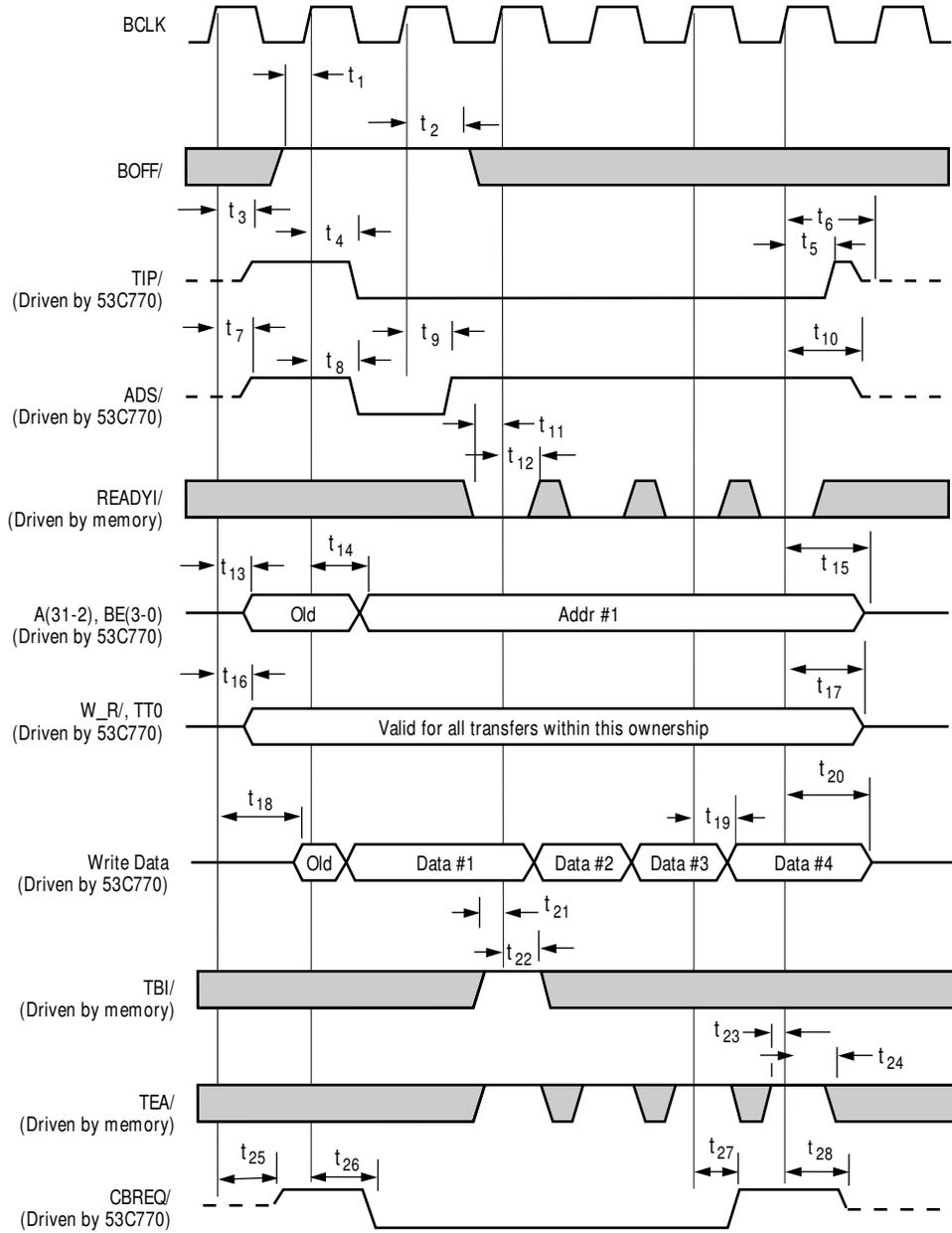
Note: this diagram shows one cache line burst of four.
