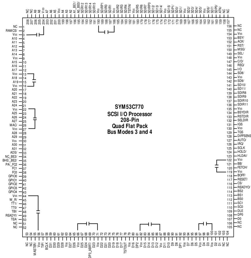
Note: the decoupling capacitor arrangements shown above are recommended to maximize the benefits of the internal split ground system. Capacitor values between 0.01 and 0.1  $\mu$ F should provide adequate noise isolation. Because of the number of high current drivers on the SYM53C770, a multi-layer PC board with power and ground planes is required.
