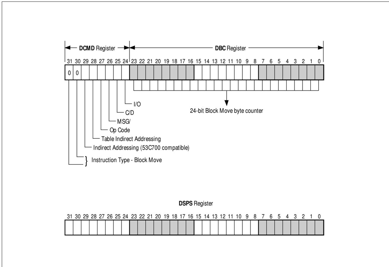
**Figure 5-1: Block Move Instruction Register**
