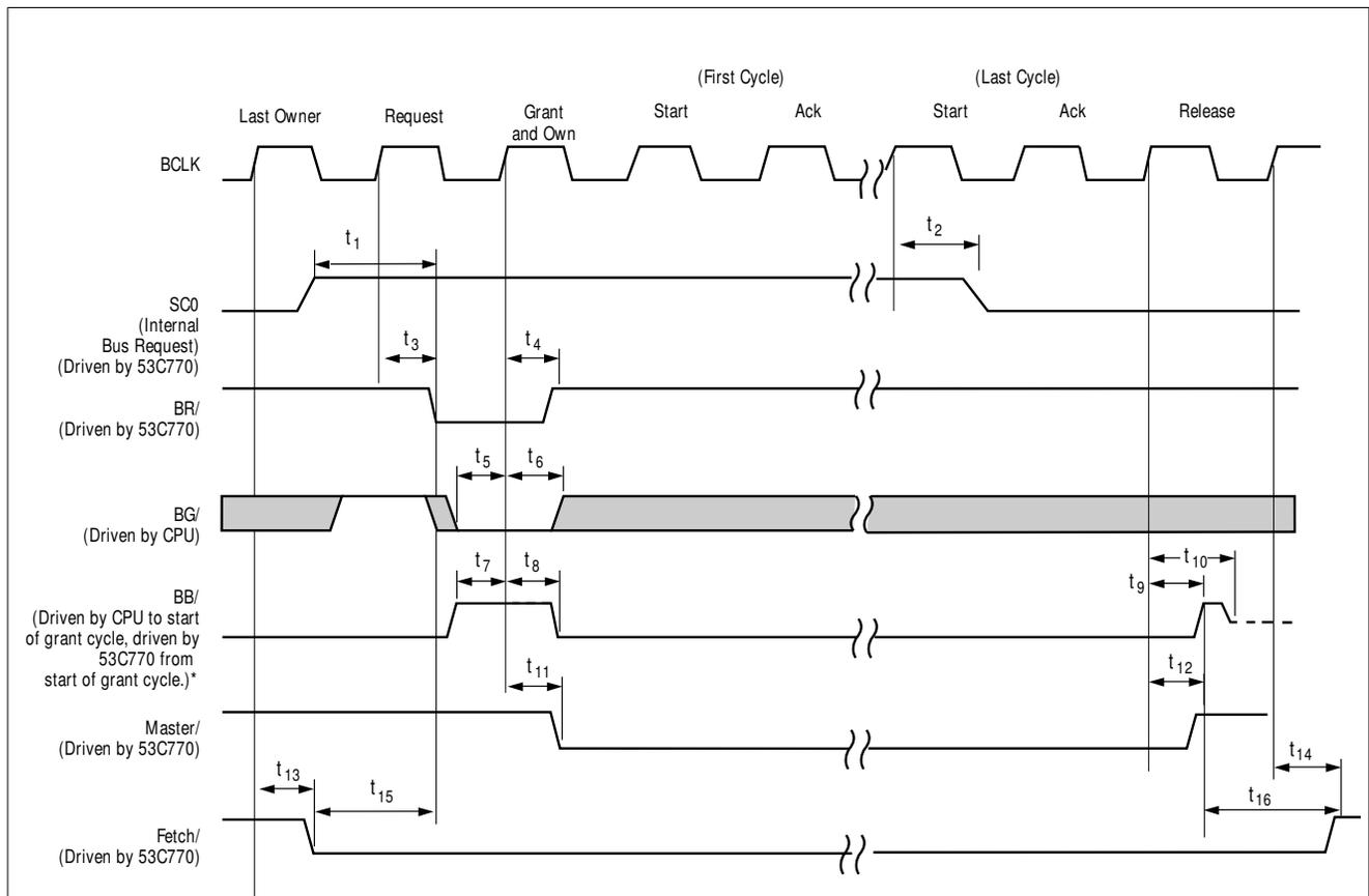
\* If the Fast Arbitration bit is set (DCNTL bit 1), the SYM53C770 will drive the Bus Grant Acknowledge signal as soon as it receives a bus grant. One clock cycle of arbitration will be saved.
