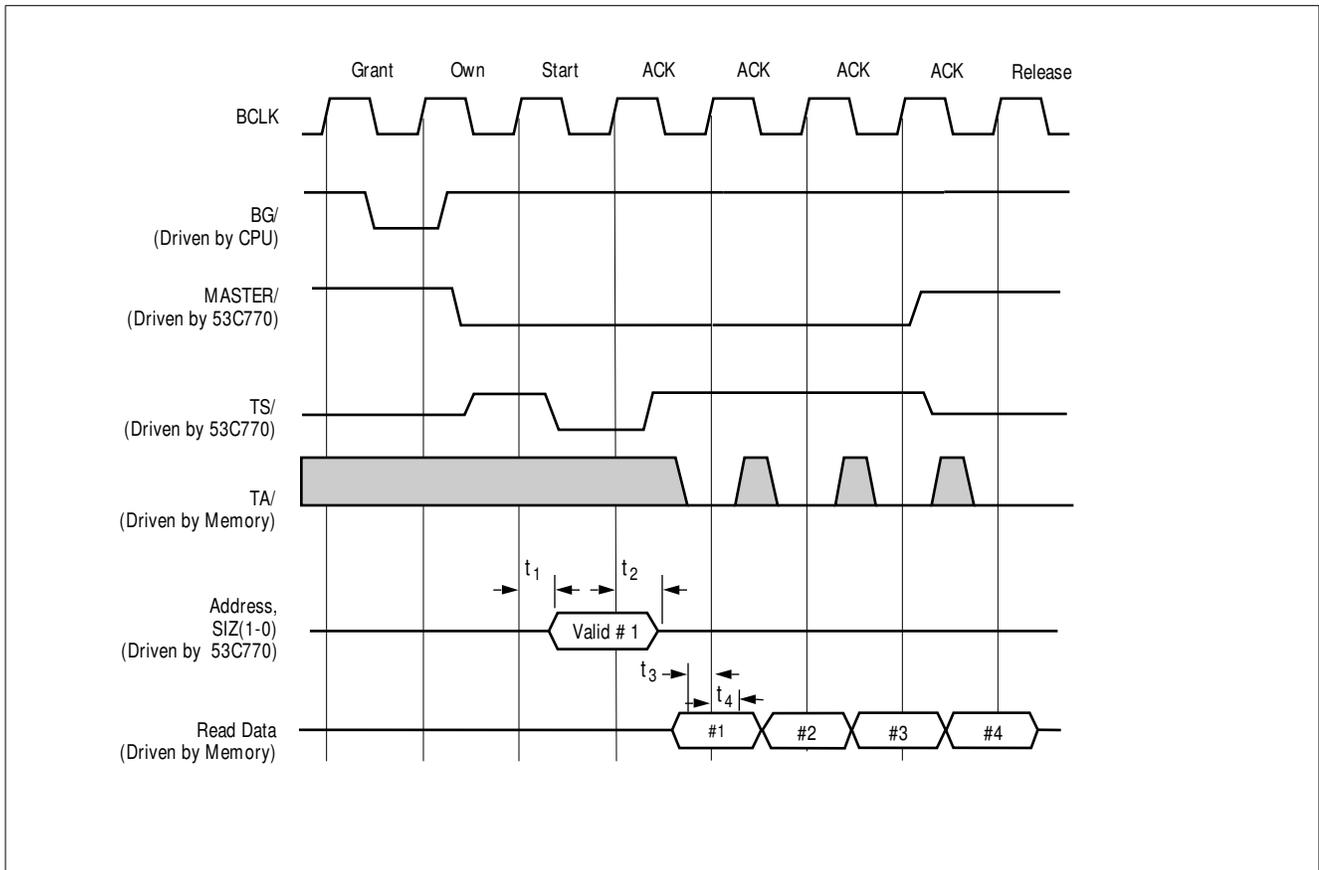
**Figure 6-25: Mux Mode Read Cycle (Cache Line Burst)**
