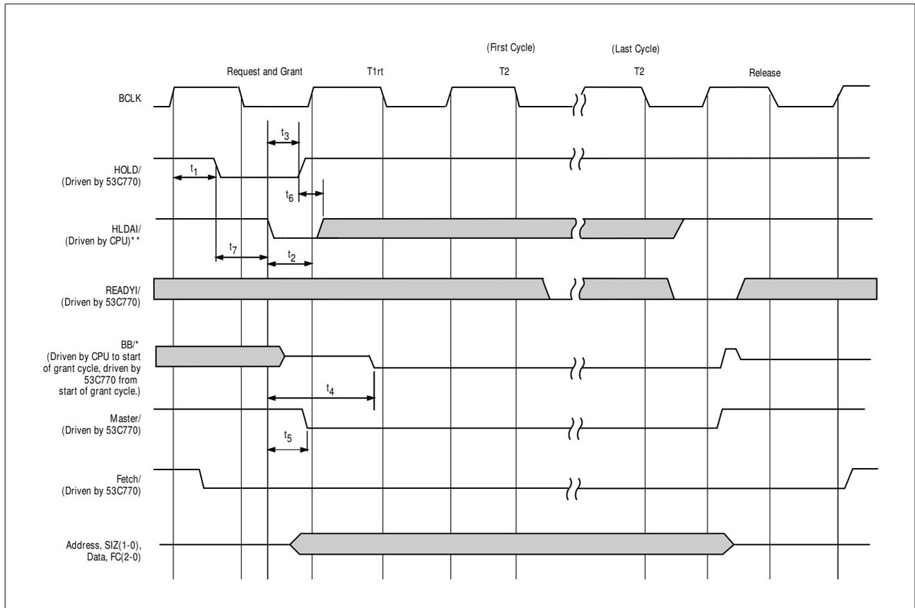
**Figure 6-31: Bus Mode 3 and 4 Fast Arbitration**
