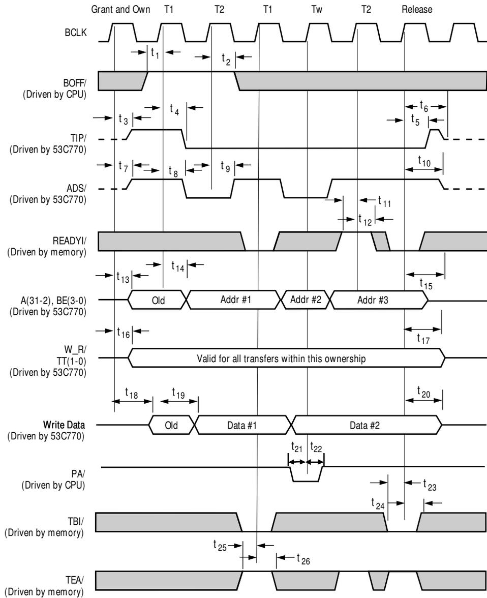
Note: this diagram shows two back-to-back transfers for a burst size of two.
