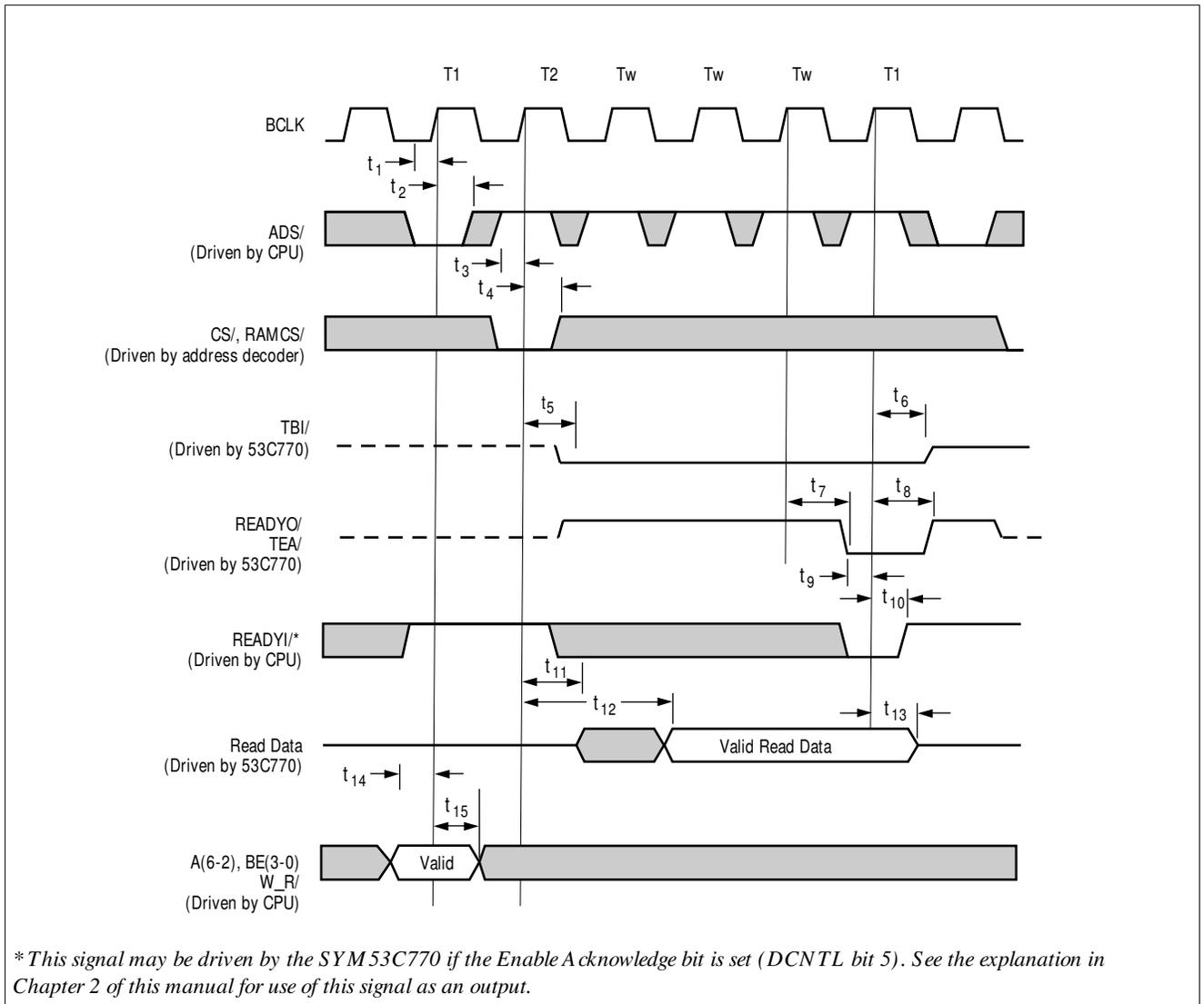
**Figure 6-28: Bus Mode 3 and 4 Slave Read Cycle**
