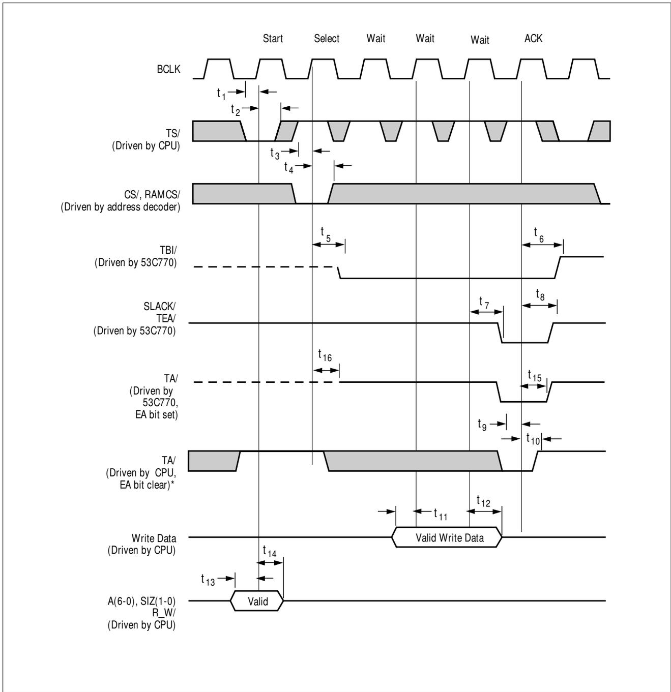
**Figure 6-18: Bus Mode 2 Slave Write Waveforms**
