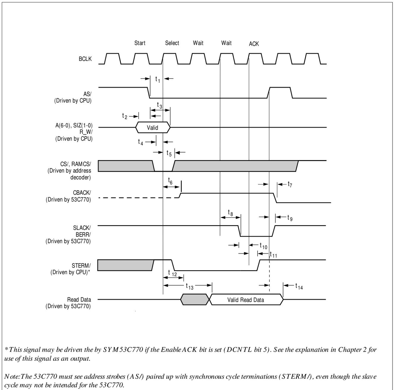
**Figure 6-9: Bus Mode 1 Slave Read Waveforms**
