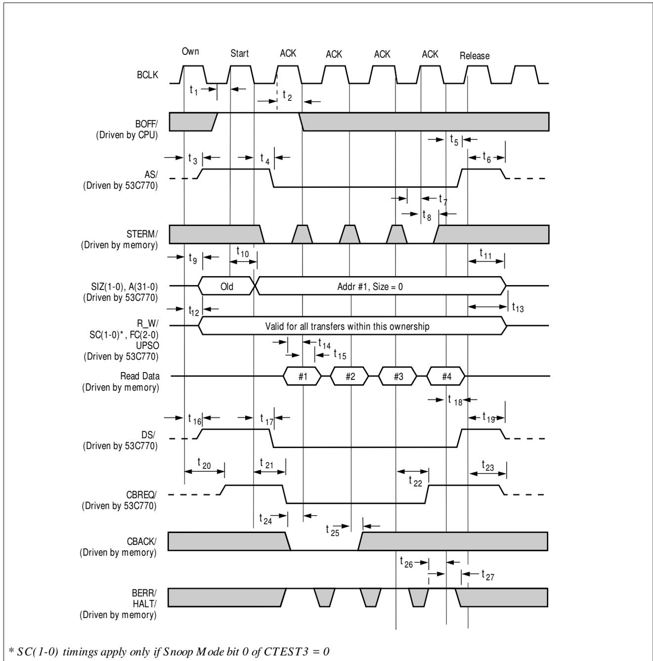
**Figure 6-14: Bus Mode 1 Bus Master Read (Cache Line Burst)**
