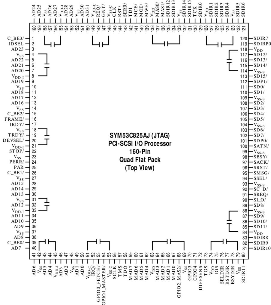
The decoupling capacitor arrangement shown above is recommended to maximize the benefits of the internal split ground system. Capacitor values between 0.01 and 0.1 $\mu$ F should provide adequate noise isolation. Because of the number of high current drivers on the SYM53C825A, a multi-layer PC board with power and ground planes is required.
