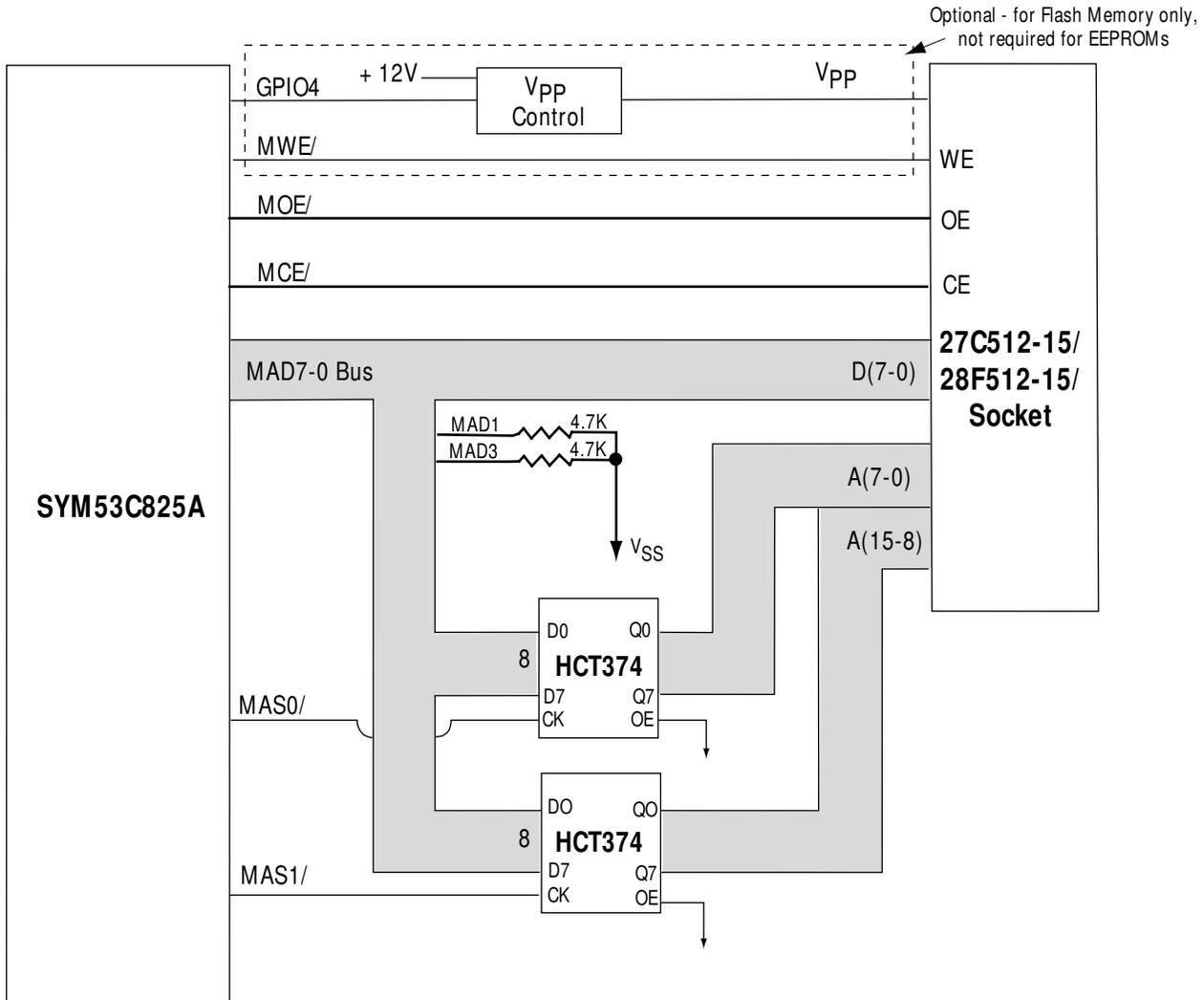
MAD Bus Sense Logic Enabled for 64 KB of fast memory (150 ns Device @ 33MHz)
