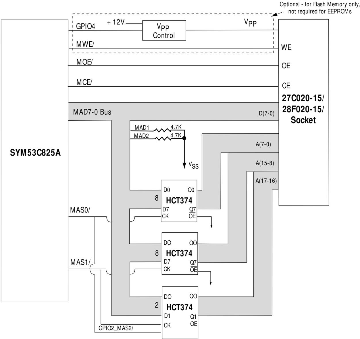
MAD Bus Sense Logic Enabled for 256 KB of fast memory (150 ns Device @ 33MHz).
