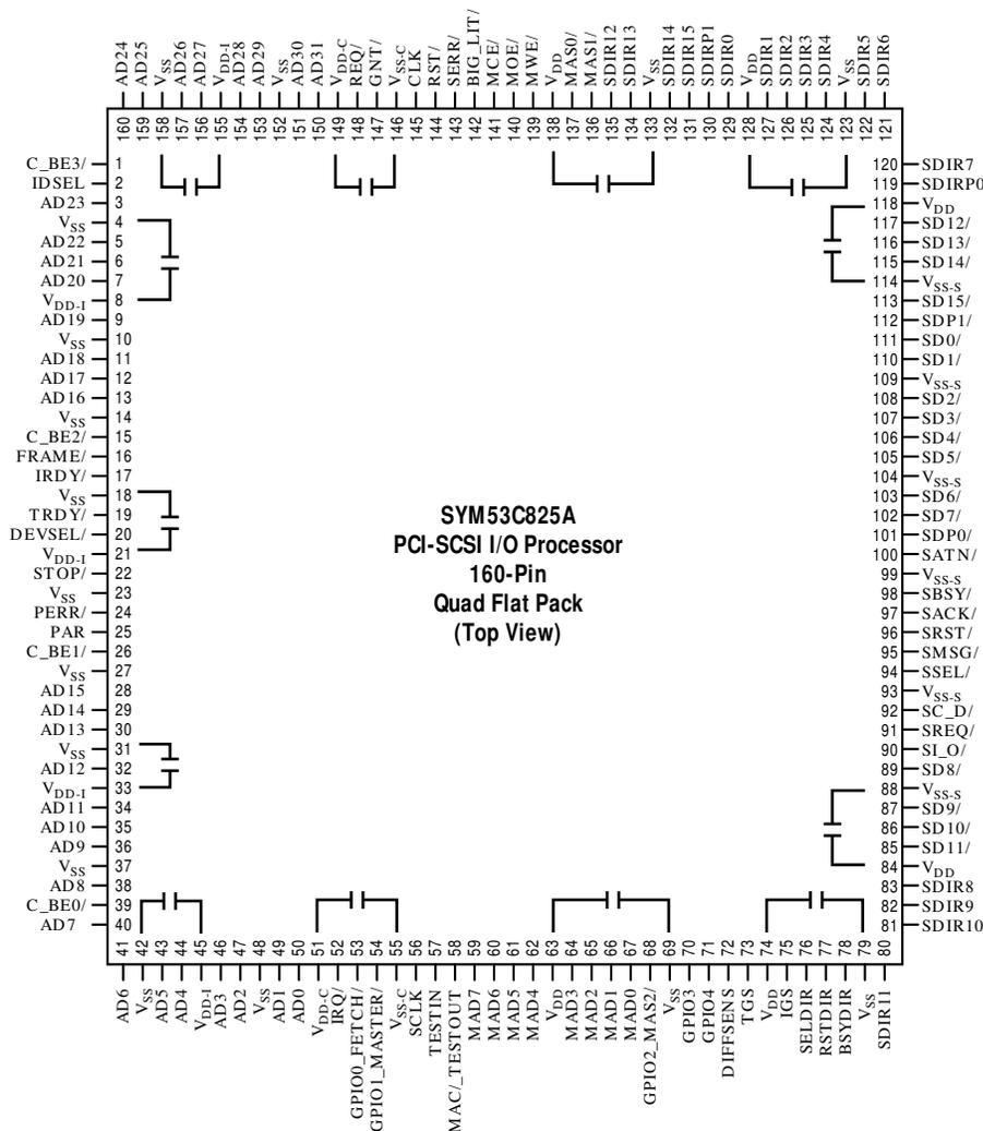
The decoupling capacitor arrangement shown above is recommended to maximize the benefits of the internal split ground system. Capacitor values between 0.01 and 0.1µF should provide adequate noise isolation. Because of the number of high current drivers on the SYM53C825A, a multi-layer PC board with power and ground planes is required.
