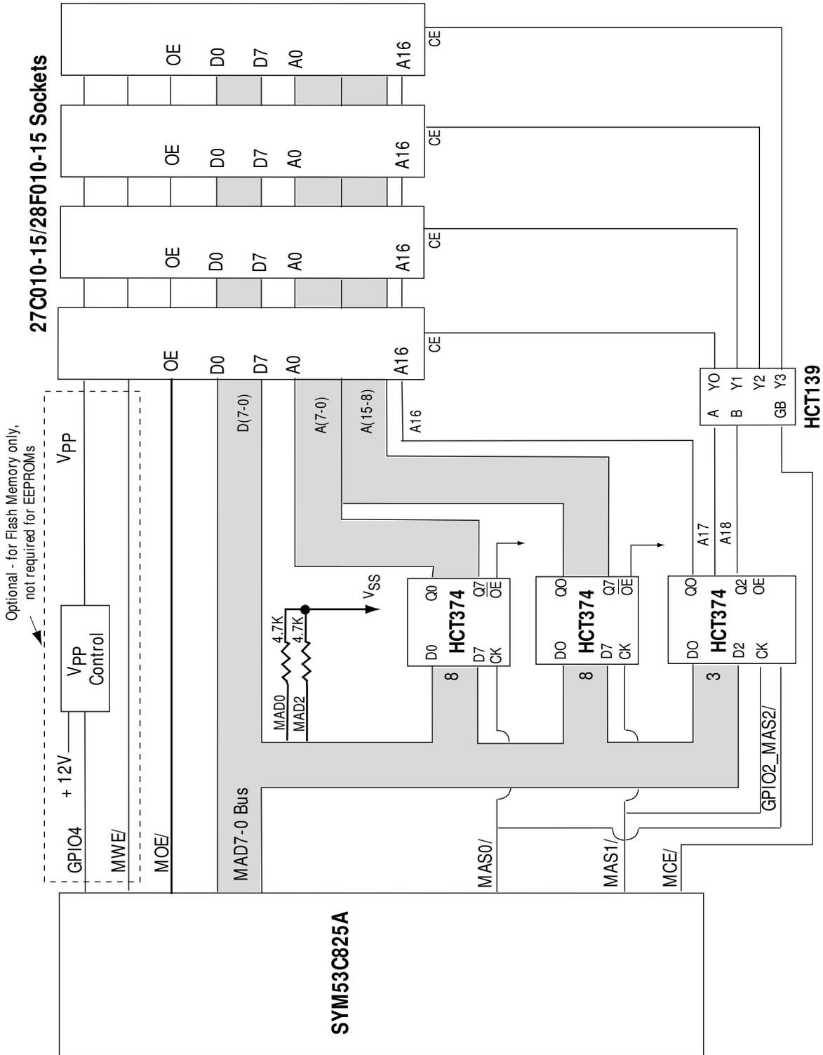
MAD Bus Sense Logic Enabled for 512 KB of slow memory (150 ns Devices, additional time required for HCT139 @ 33MHz).
