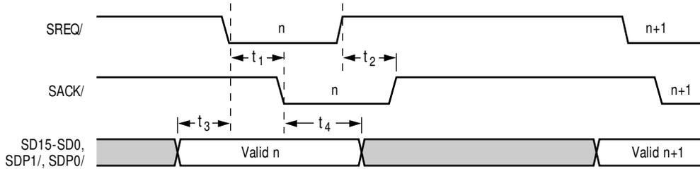
Figure 7-34: Target Asynchronous Receive
