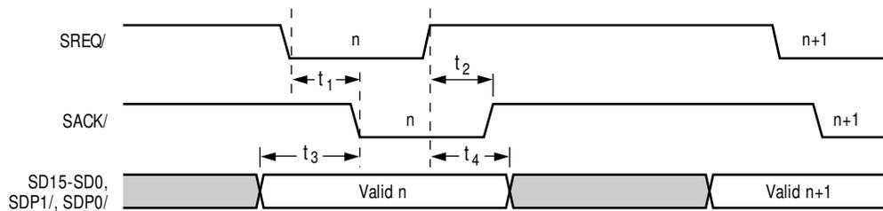
**Figure 7-32: Initiator Asynchronous Receive**
