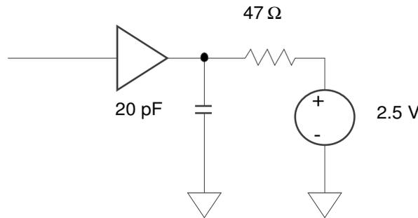
Figure 7-1: Rise and Fall Time Test Conditions
