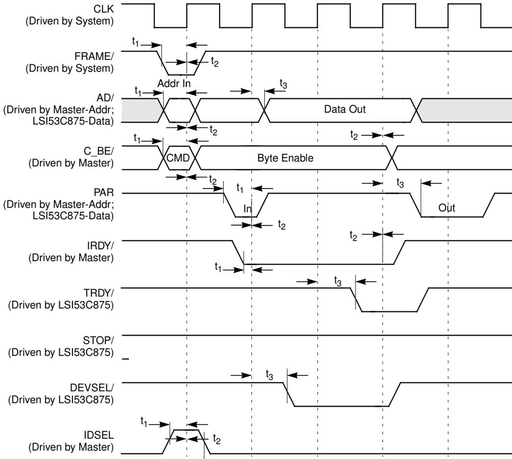
**Figure 7.10 PCI Configuration Register Write**
