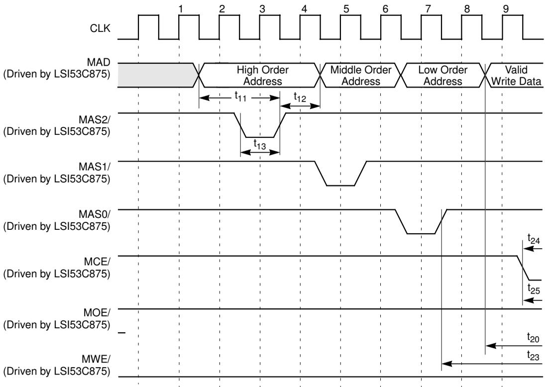
**Figure 7.22 Write Cycle, Normal/Fast Memory ( $\geq 64$  Kbytes), Single Byte Access (Cont.)**
