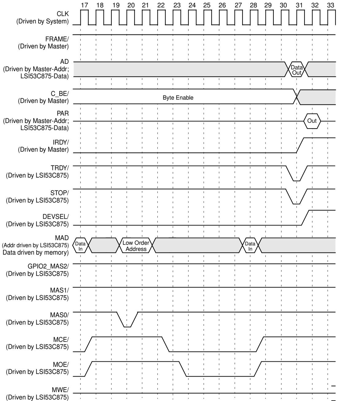
**Figure 7.24 Write Cycle, Normal/Fast Memory ( $\geq 64$  Kbyte), Multiple Byte Access**
