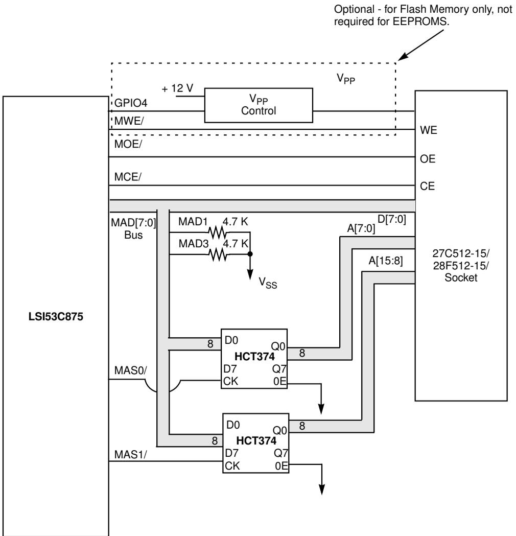
Note: MAD bus sense logic enabled for 64 Kbytes of fast memory (150 ns device @ 33 MHz).
