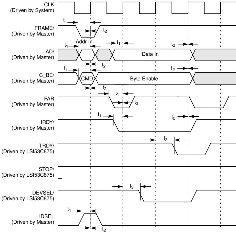
**Figure 7.11 Operating Register/SCRIPTS RAM Read**
