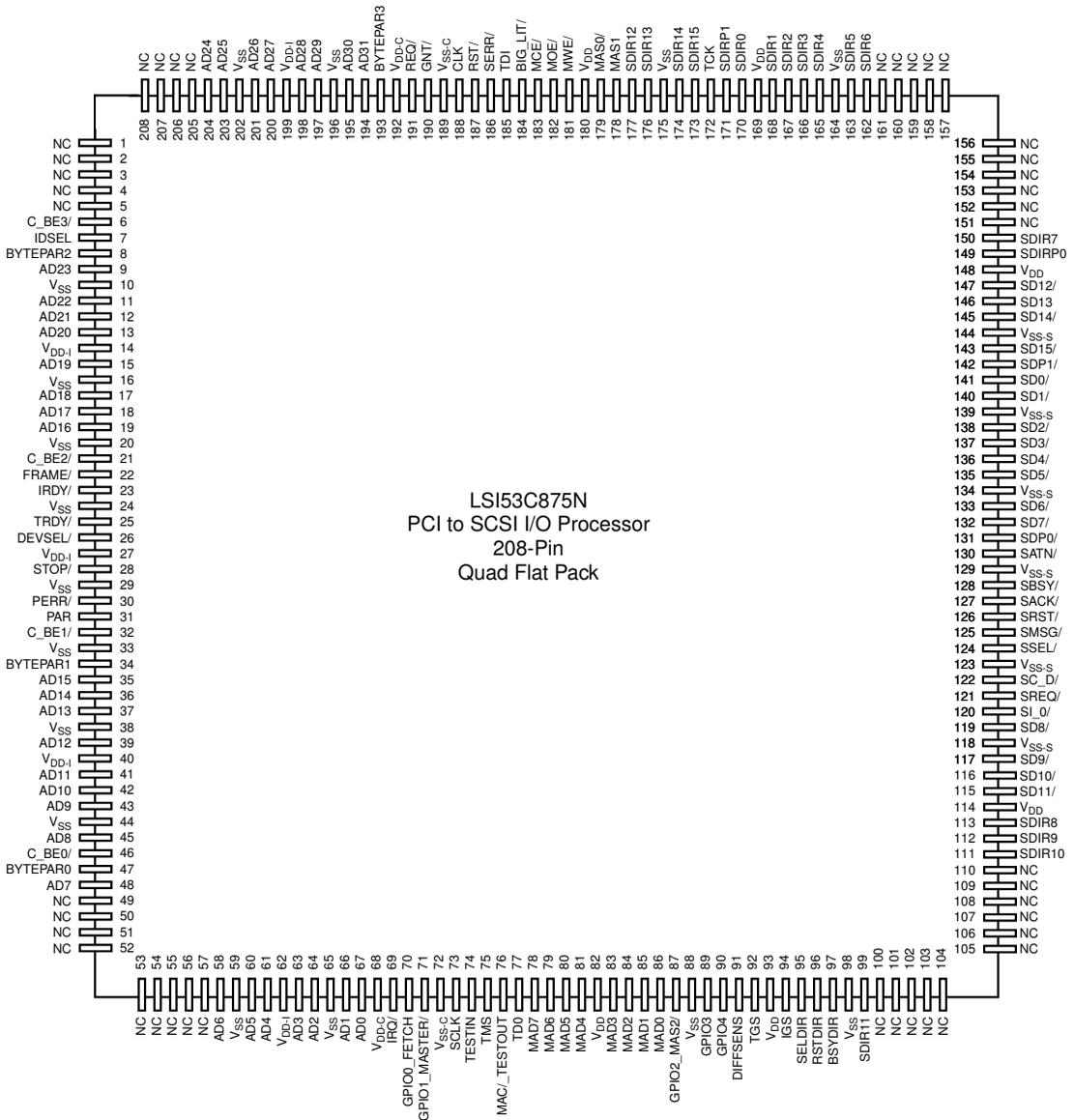
Note: The decoupling capacitor arrangement shown in Figures 4.1 and 4.2 is recommended to maximize the benefits of the internal split ground system. Capacitor values between 0.01 and 0.1  $\mu\text{F}$  should provide adequate noise isolation. Because of the number of high current drivers on the LSI53C875, a multilayer PC board with power and ground planes is required.
