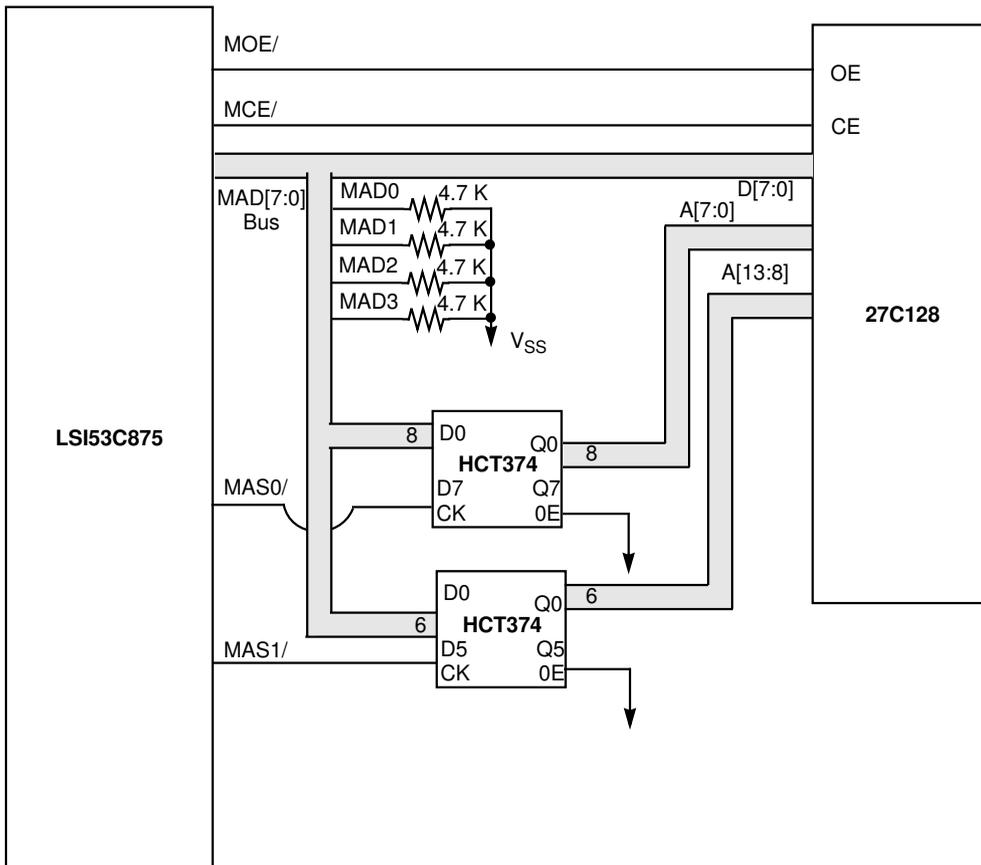
Note: MAD bus sense logic enabled for 16 Kbytes of slow memory (200 ns device @ 33 MHz).
