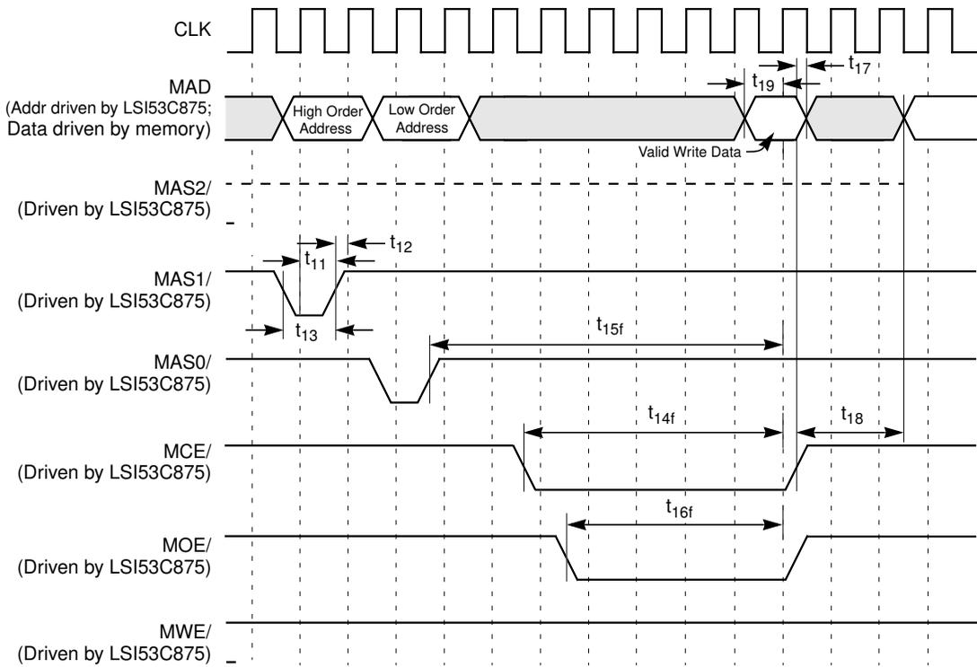
**Figure 7.28 Write Cycle, Normal/Fast Memory ( $\geq 64$  Kbyte)**
