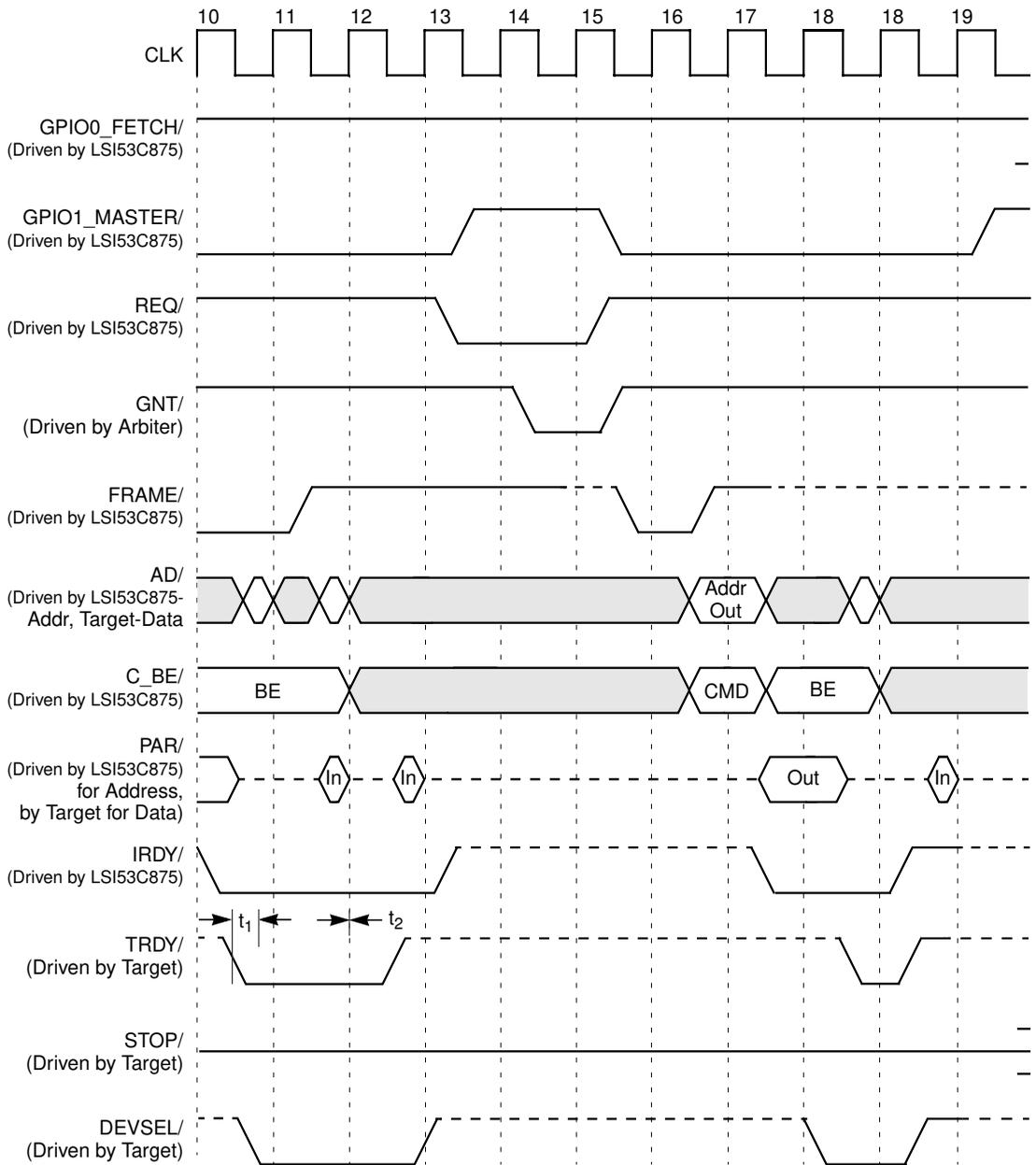
**Figure 7.20 Burst Write**
