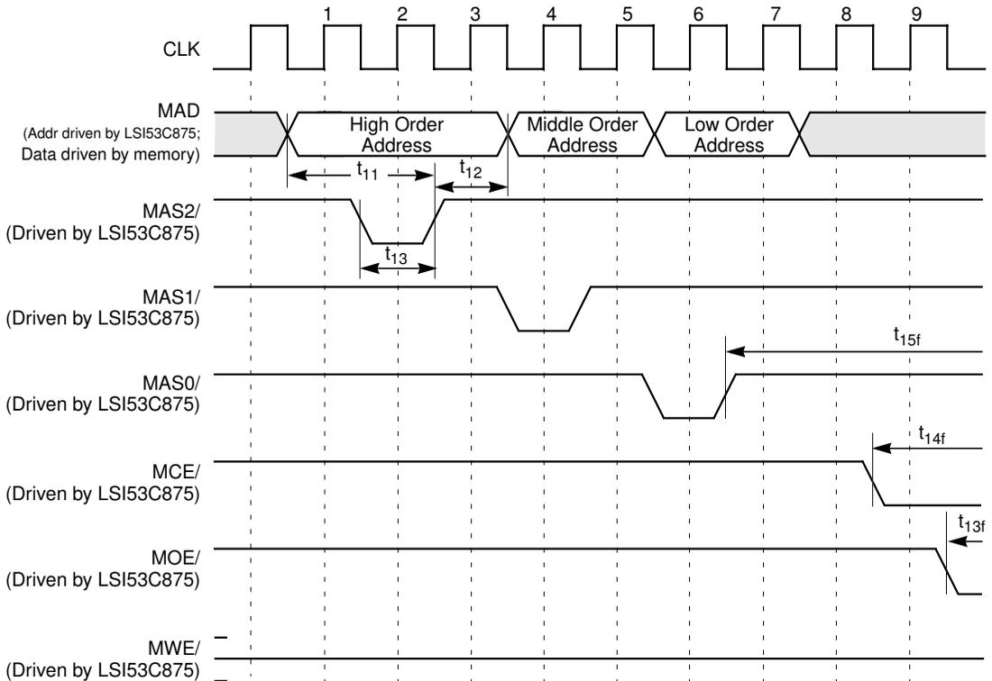
**Figure 7.21 Read Cycle, Normal/Fast Memory ( $\geq 64$  Kbytes), Single Byte Access (Cont.)**
