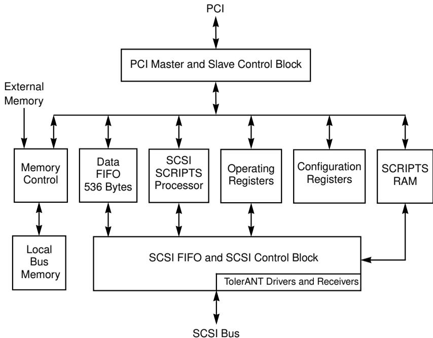
The LSI53C875 integrates a high-performance SCSI core, a PCI bus master DMA core, and the LSI Logic SCSI SCRIPTS processor to meet the flexibility requirements of SCSI-3 and Ultra SCSI standards. It is designed to implement multithreaded I/O algorithms with a minimum of processor intervention, solving the protocol overhead problems of previous intelligent and nonintelligent adapter designs.
