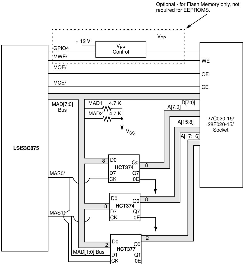
Note: MAD bus sense logic enabled for 256 Kbytes of fast memory (150 ns device @ 33 MHz). The HCT374s may be replaced with HCT377s.
