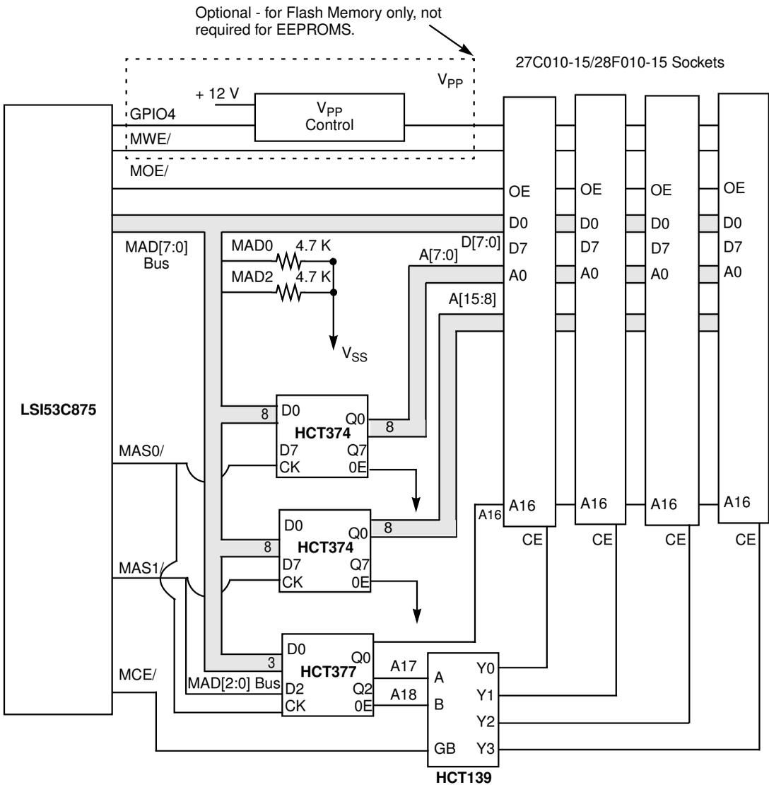
Note: MAD bus sense logic enabled for 512 Kbytes of slow memory (150 ns devices, additional time required for HCT139 @ 33 MHz). The HCT374s may be replaced with HCT377s.
