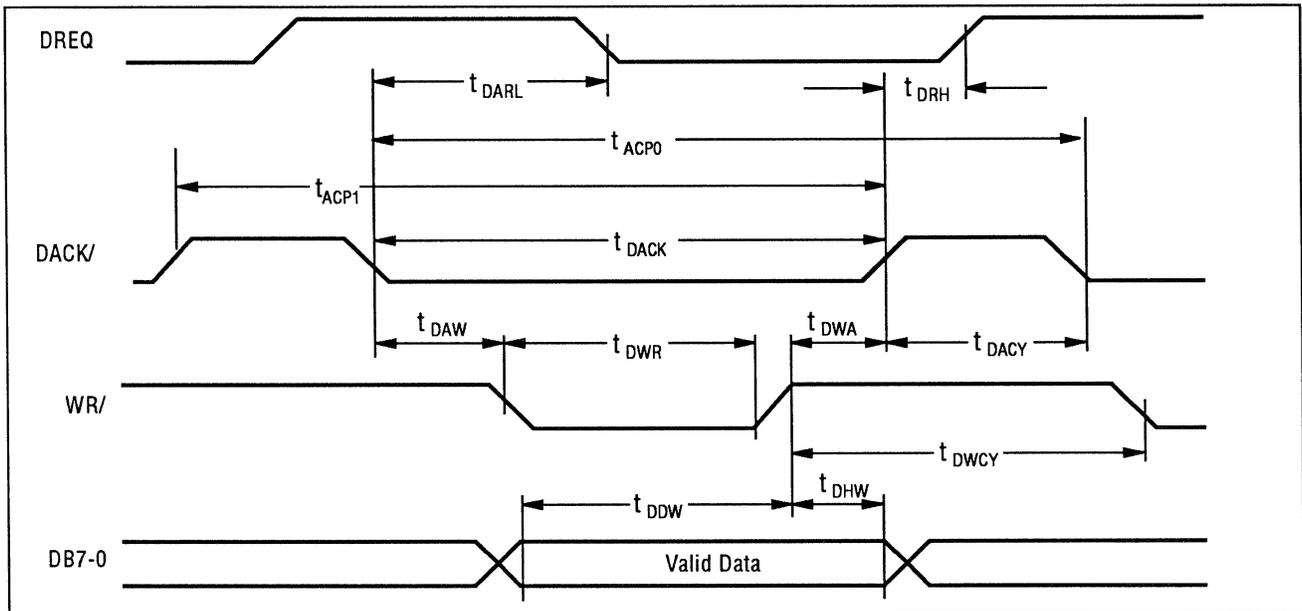
1) For synchronous data transfers DACK/ low to DACK/ high must equal or exceed  $2t_{CP}$  and  $t_{CS} + 35 - t_{DACY}$
