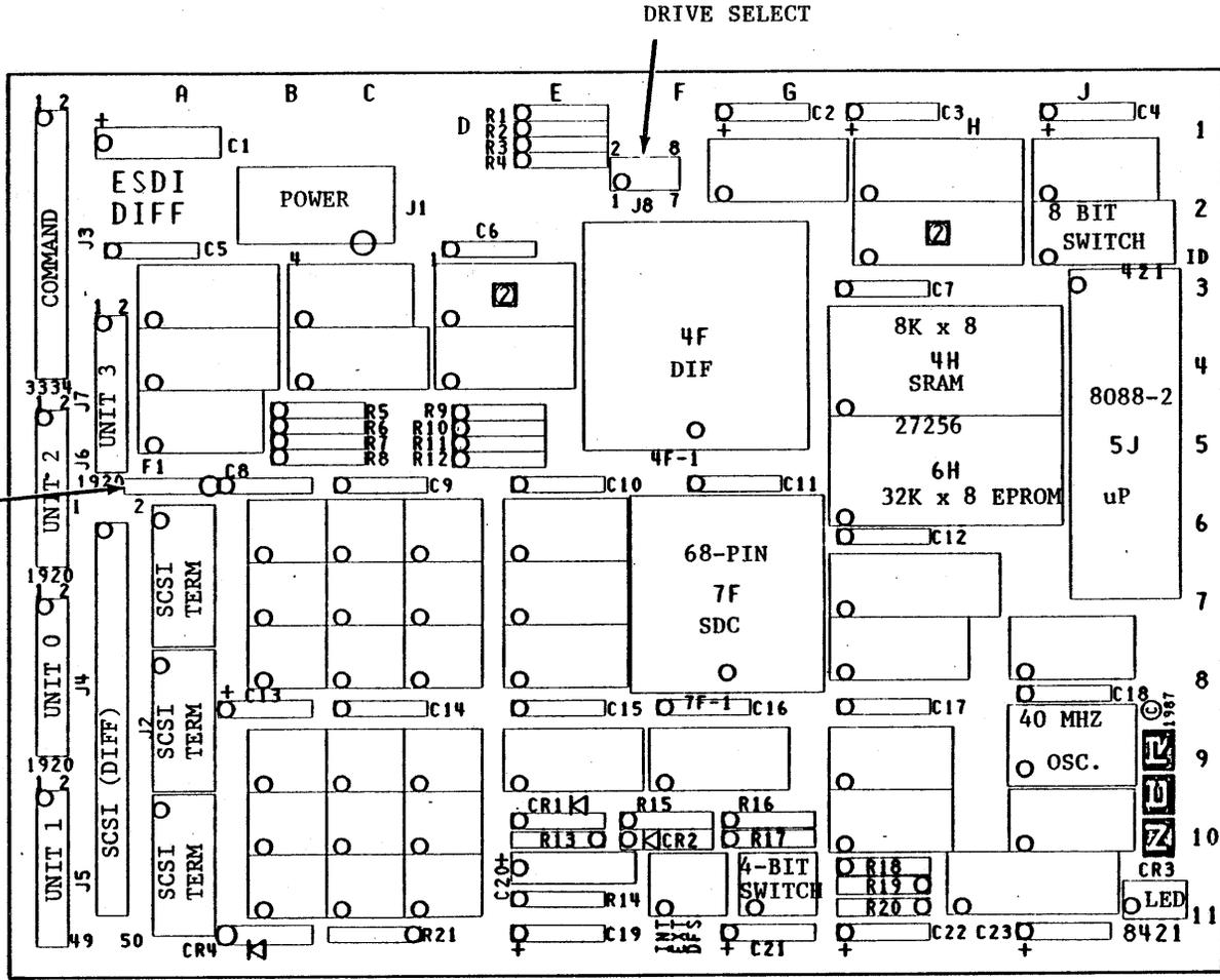
Figure 4-11 NCR ADP-47-04 ESDI Differential Controller board
