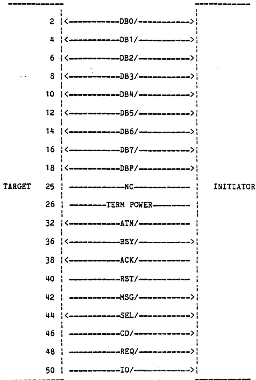
\* All odd-numbered pins, except Pin 25, are connected to ground. Pins 19 through 24 and Pin 34 are also connected to ground.
