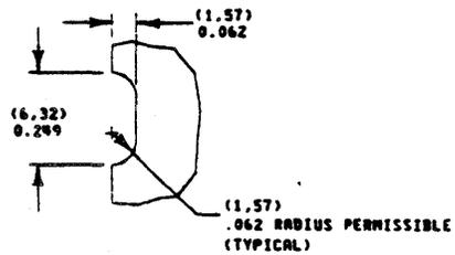
Figure 9. Dimensional Drawing of ADP-55
