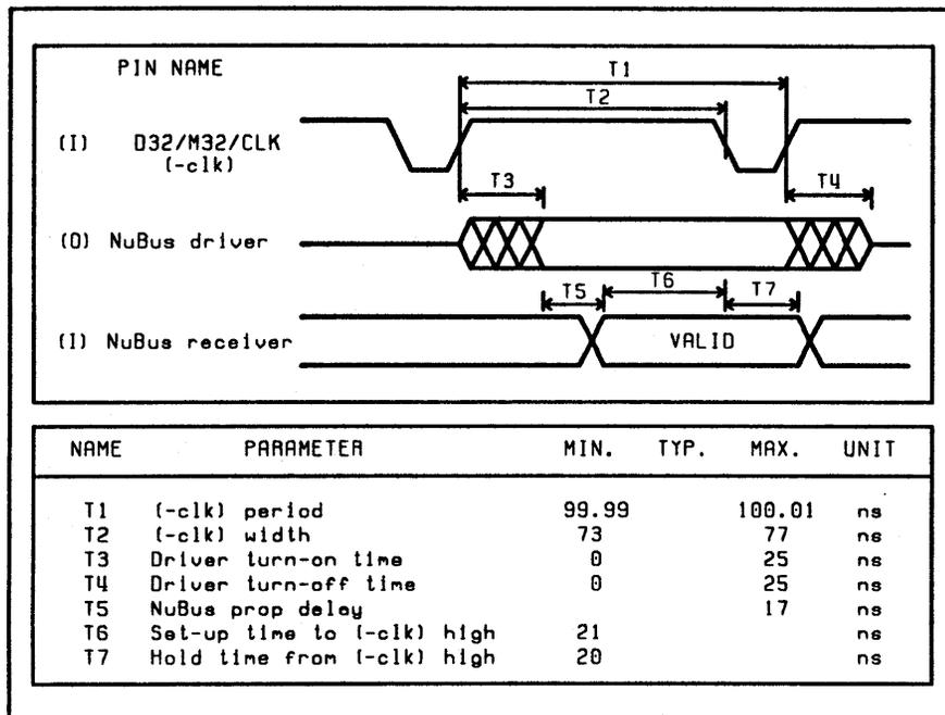
Figure 4-22. NuBus Data Transfer Timing Characteristics
