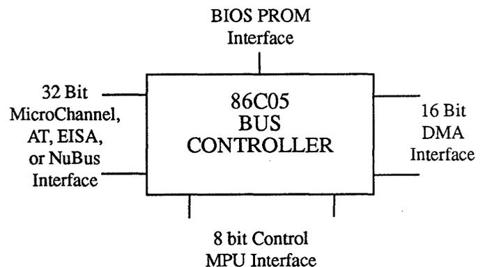
Figure 1. Data Flow through the 86C05
