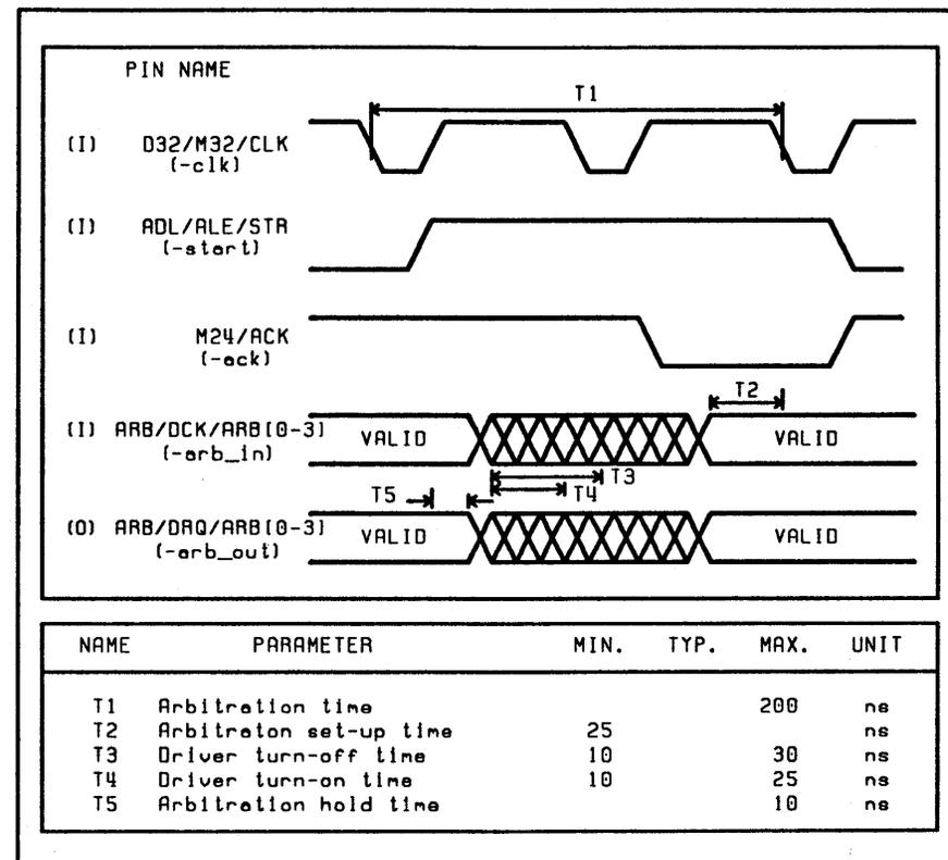
Figure 4-23. NuBus Arbitration Timing Characteristics
