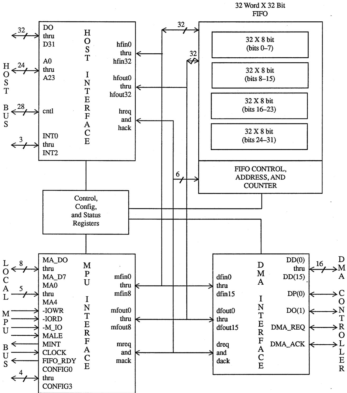
Figure 2. Block diagram of the 86C05
