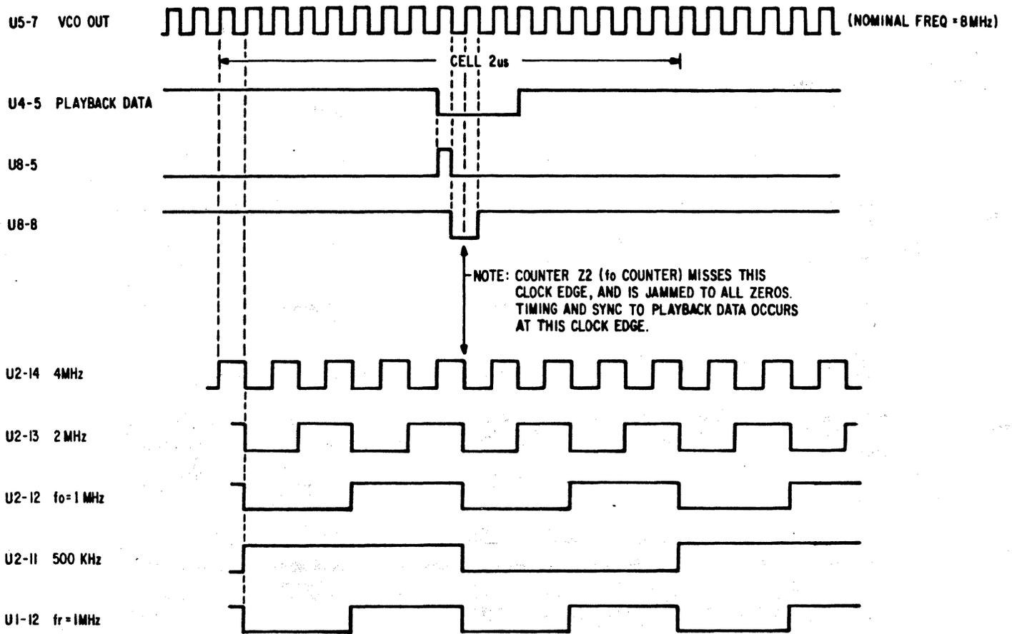
NOTE: fr AND fo ARE PHASE LOCKED AFTER LOOP HAS ACQUIRED AND LOCKED.
