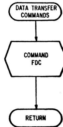
NOTE: FDC AUTOMATICALLY ENTERS EXECUTION PHASE UPON COMPLETION OF COMMAND PHASE. RECEIPT OF EITHER DMA REQUESTS OR INTERRUPT SIGNALS INDICATES BEGINNING OF EXECUTION PHASE.
