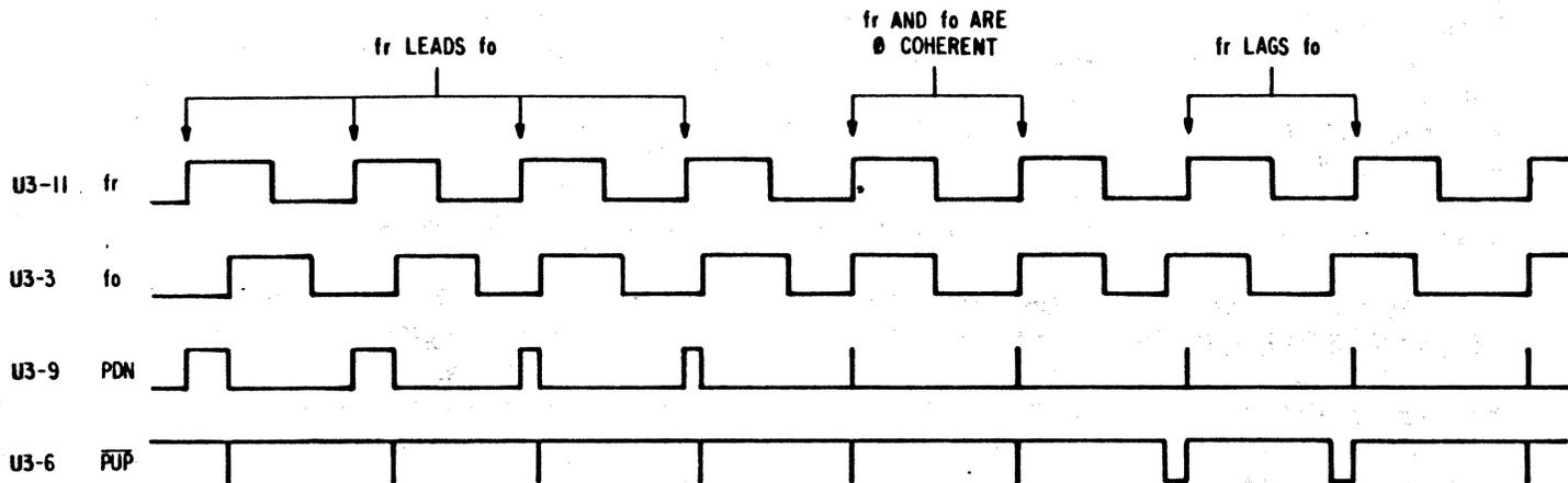
NOTE: PDN CONTROLS Q1, AND PUP CONTROLS Q2, WHICH DISCHARGE AND CHARGE CAPACITOR C1. RESISTOR CAPACITOR NETWORK R4, R7, R8 AND C1 CHANGE THE PULSE WIDTH MODULATED SIGNALS PDN AND PUP (WHICH ARE A DIRECT FUNCTION OF PHASE DIFFERENCES BETWEEN  $f_r$  AND  $f_o$ ), INTO A D.C. LEVEL, AS SEEN AT U5-2. THE LEVEL AT U5-2 IS NORMINALLY +3.25V.
