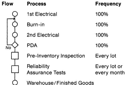
During the first electrical test, DC parameters are tested in accordance with electrical specifications, on 100% of each lot. This prescreen performance is prior to the infant mortality testing. As an integral part of the standard production process, 100% burn-in is performed.
