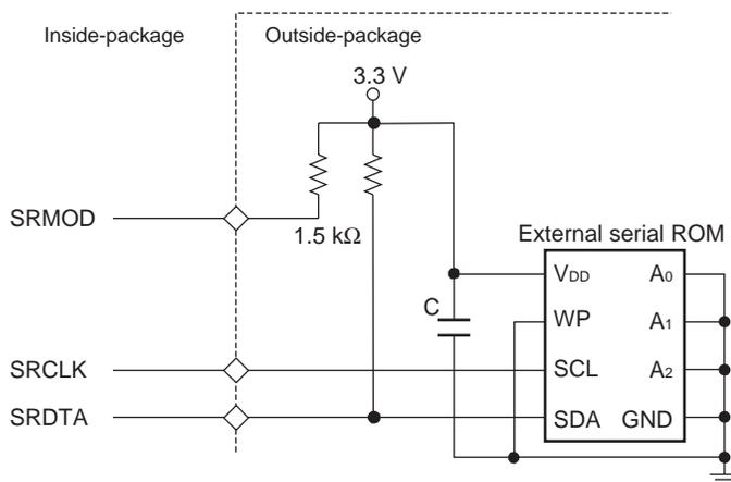
These pins for external serial ROM can be opened, when serial ROM is not necessary on board.
