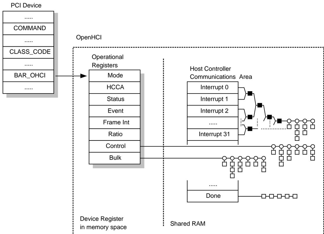
4.2.1 Mapping of operational registers for OHCI host controller #1
