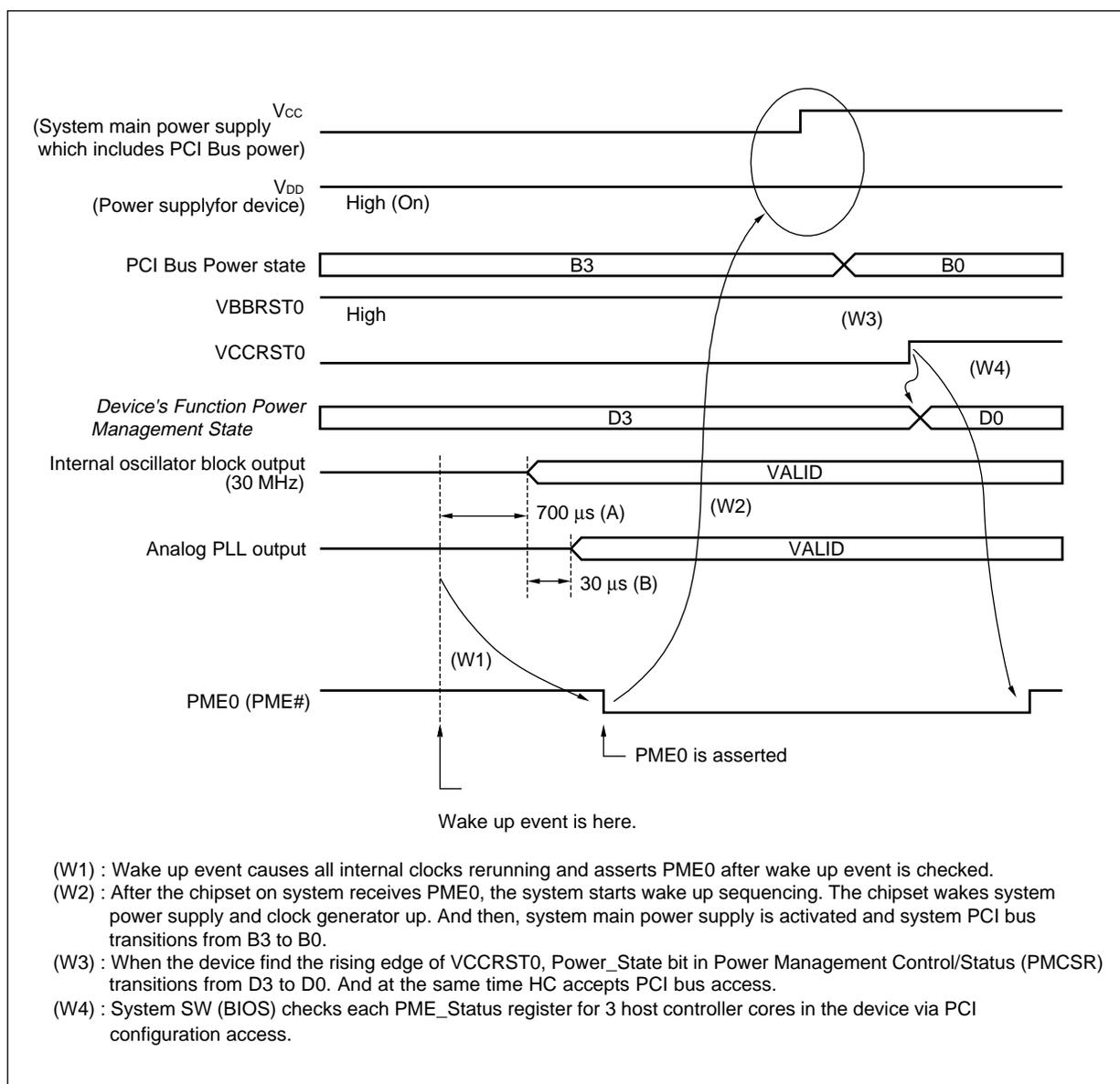
Figure 7-5. Clock Operation Diagram (Using 48-MHz Oscillator)
