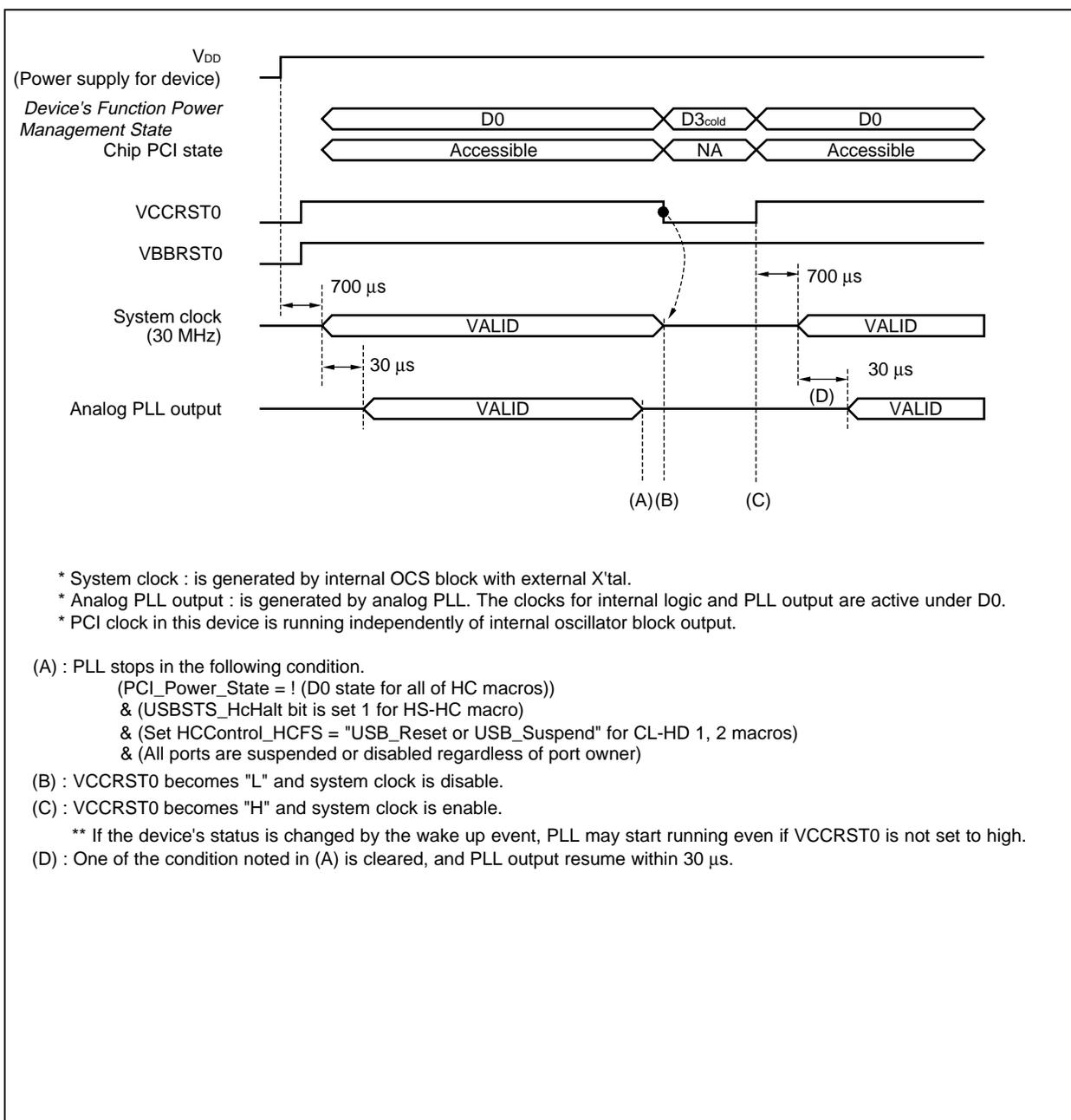
Figure 7-2. Wake Up State Transition from D3<sub>cold</sub> (Using 48-MHz Oscillator)
