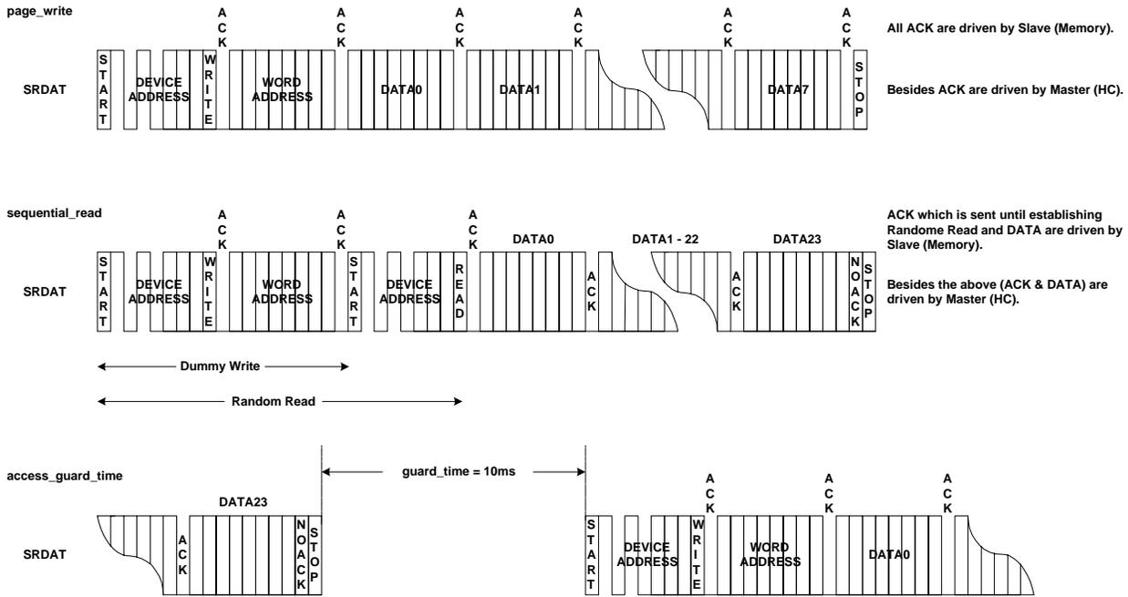
It takes about 2 ms to complete page\_write command. more than 12 ms shall be waited before starting next page\_write or sequential\_read command. On the other hands, It takes about 5 ms to complete sequential\_read command. So, more than 15 ms shall be waited before starting next page\_write or sequential\_read command. And also more than 5 ms shall be waited before reading PCI configuration register after sequential\_read command starts.
