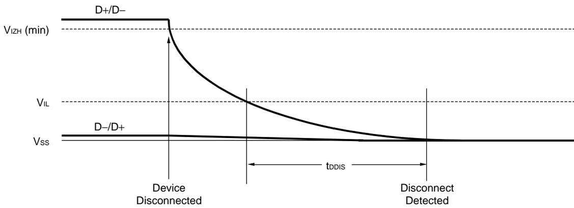
**Full-/high-speed device connect detection**
