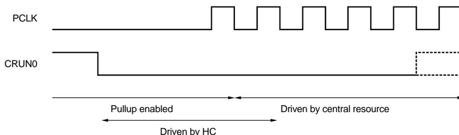
HC asserts CRUN0 asynchronously and it holds CRUN0 asserted until it detects two rising edge of PCLK. After the second clock edge, HC disables its open drain buffer. The central resource drives CRUN0 low at any time after it detects that the line asserted by HC, but not later than on 3<sup>rd</sup> clock. It also must not drive CRUN0 high earlier than on 5<sup>th</sup> clock.
