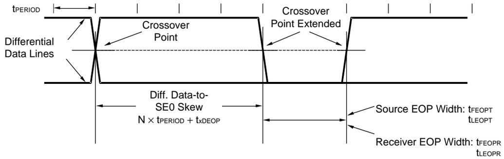
**USB receiver jitter tolerance for low-/full-speed**
