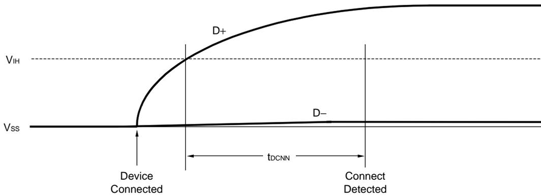
**Low-speed device connect detection**
