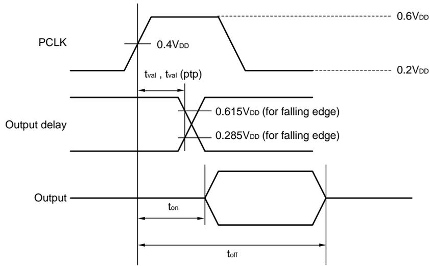
PCI input timing measurement condition
