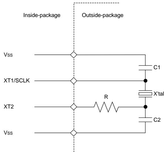
The following crystals are evaluated on our reference design board. Table 9-1 shows the external parameters.
