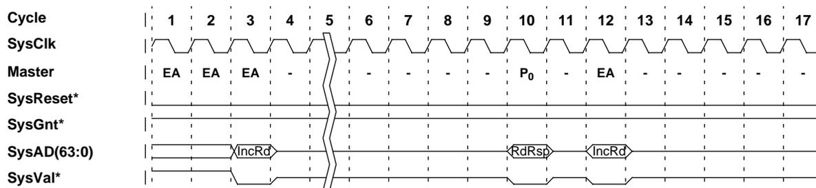
Figure 15-6 Cache Test Mode Auto-Increment Read Protocol
