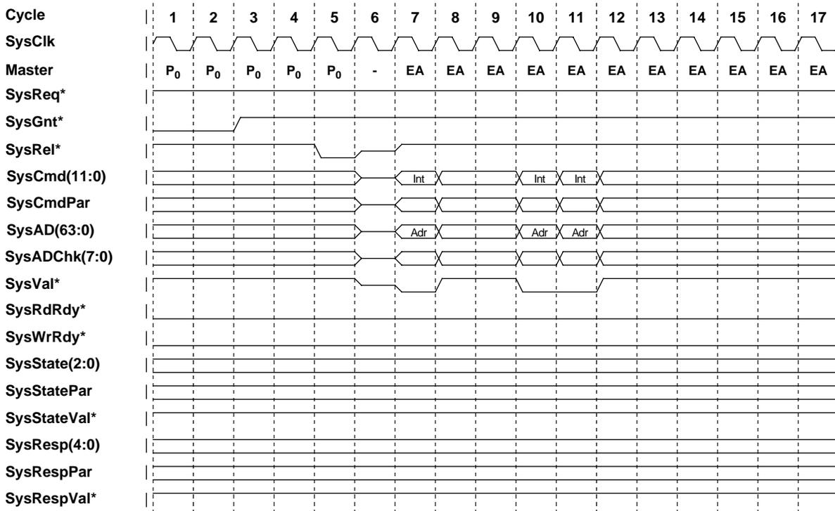
Figure 6-23 External Interrupt Request Protocol
