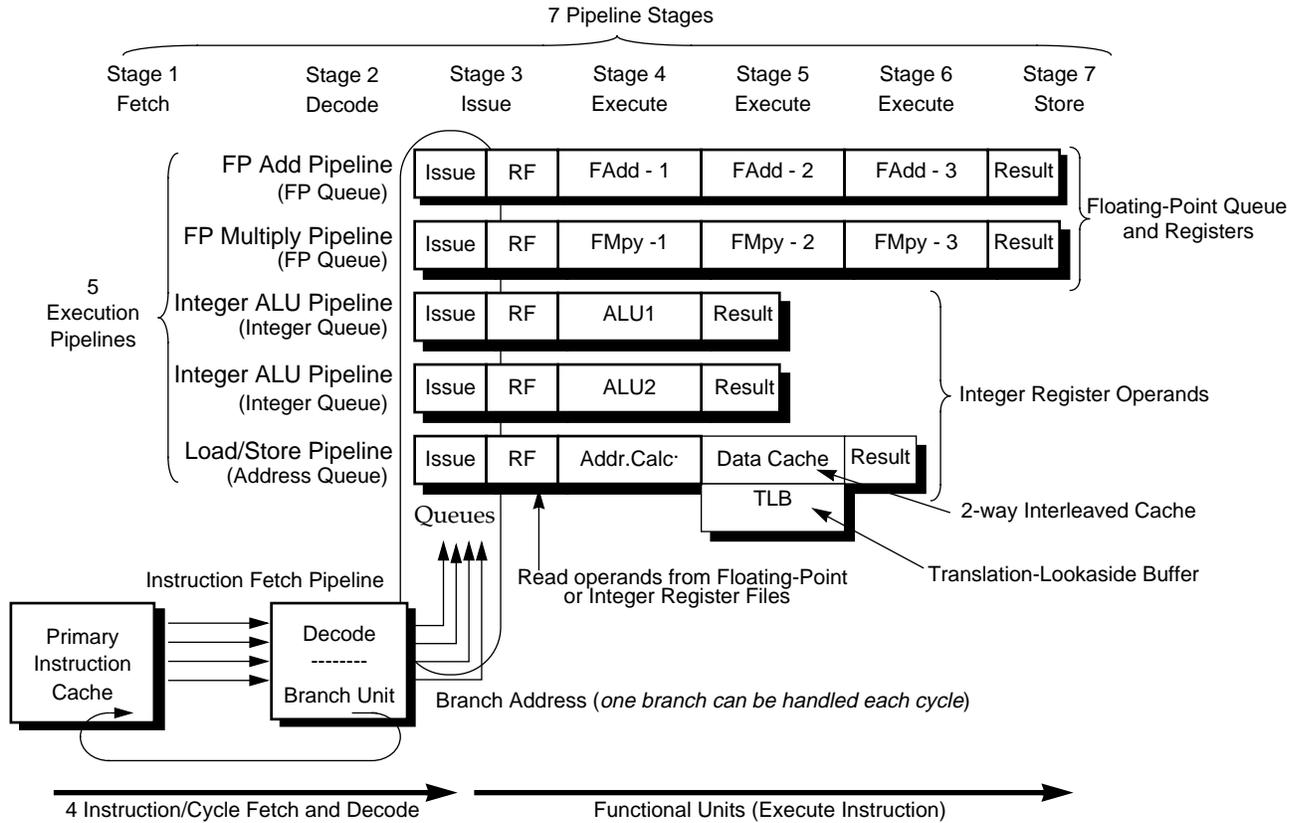
Figure 1-4 Superscalar Pipeline Architecture in the R10000
