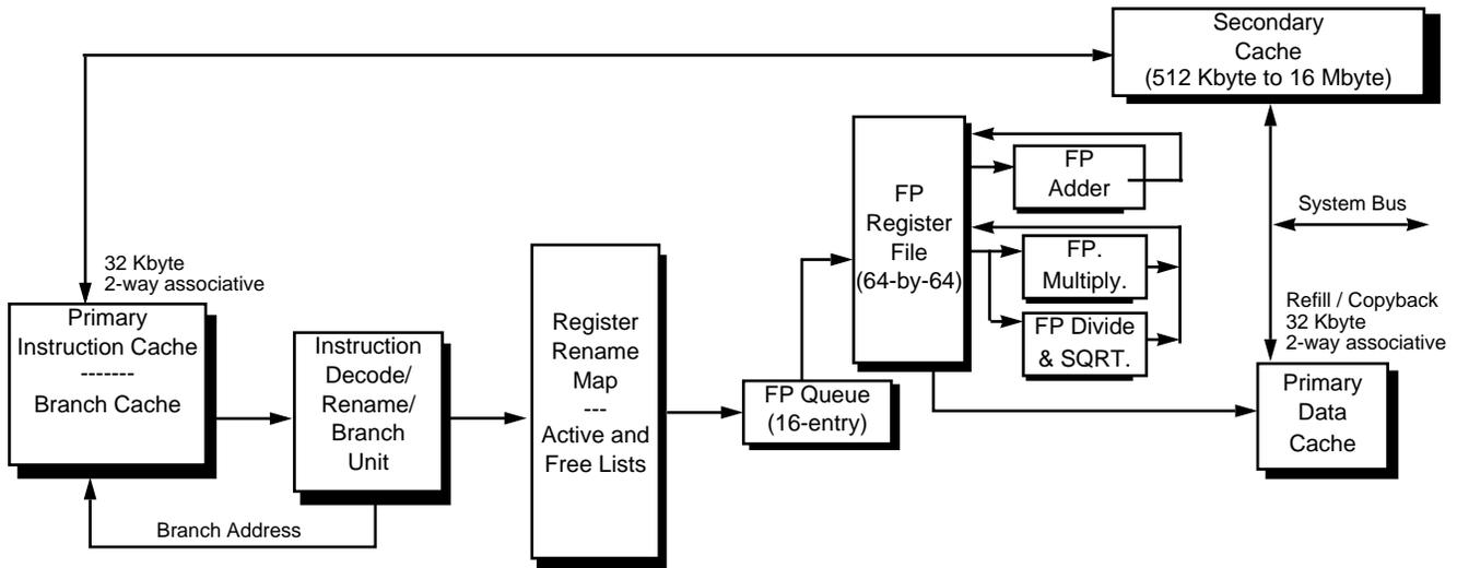
Figure 12-1 Logical Diagram of FP Operations
