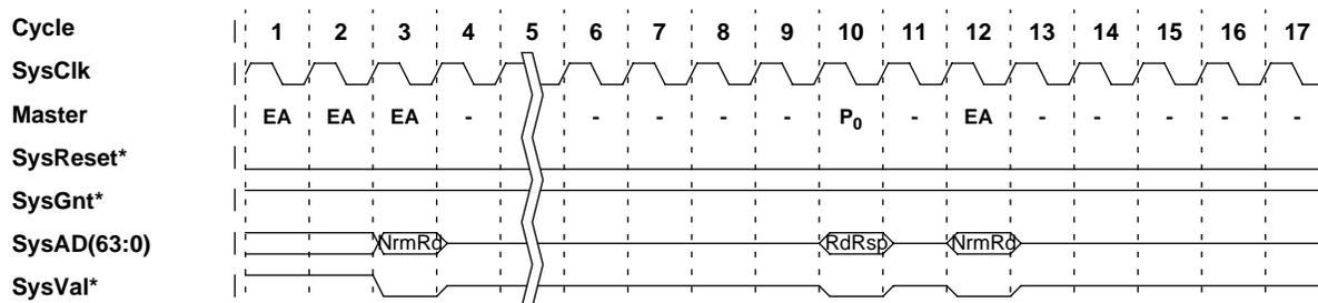
Figure 15-5 Cache Test Mode Normal Read Protocol
