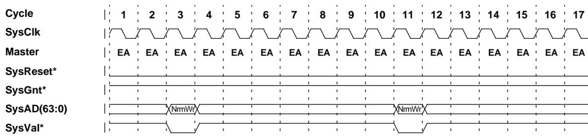
Figure 15-3 Cache Test Mode Normal Write Protocol
