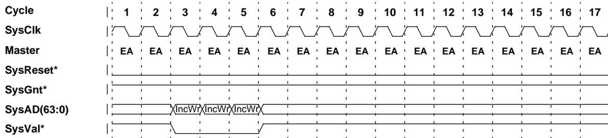
Figure 15-4 Cache Test Mode Auto-Increment Write Protocol
