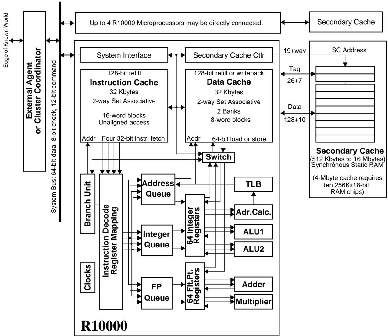
Figure 1-5 Block Diagram of the R10000 Processor
