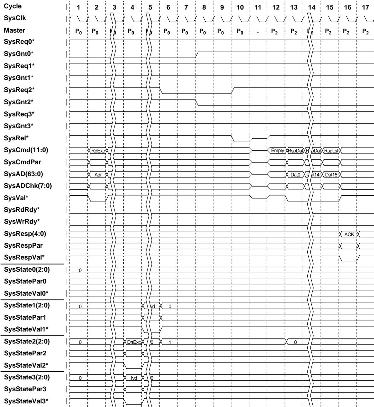
Figure 6-27 R10000 Multiprocessor Cluster Processor Read Request Example
