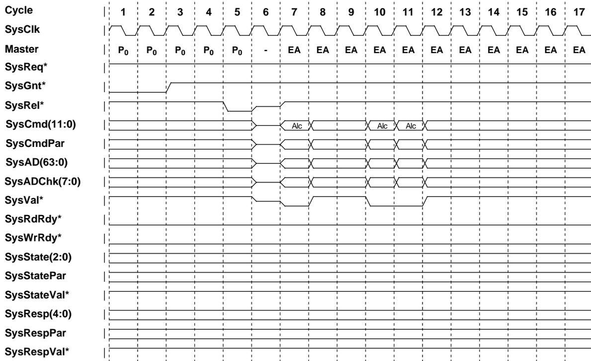
Figure 6-21 External Allocate Request Number Request Protocol
