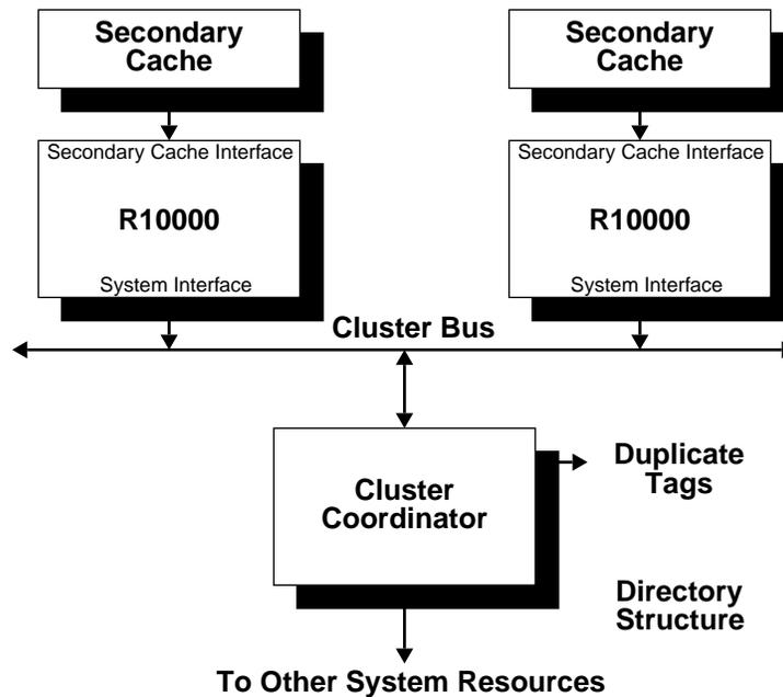
Figure 2-3 Multiprocessor System Organization Using the Cluster Bus
