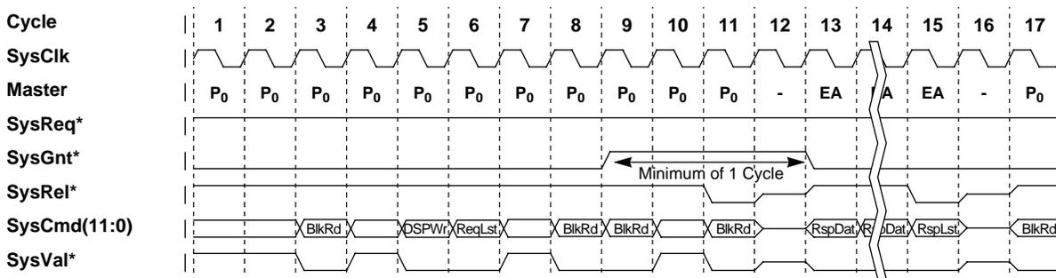
Figure 6-7 Arbitration Protocol for Uniprocessor System
