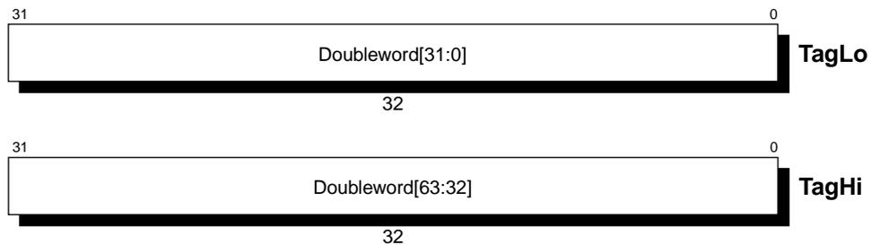
Figure 11-34 *TagHi/Lo Register Fields in Secondary Cache When CacheOp is Index Load/Store Data*
