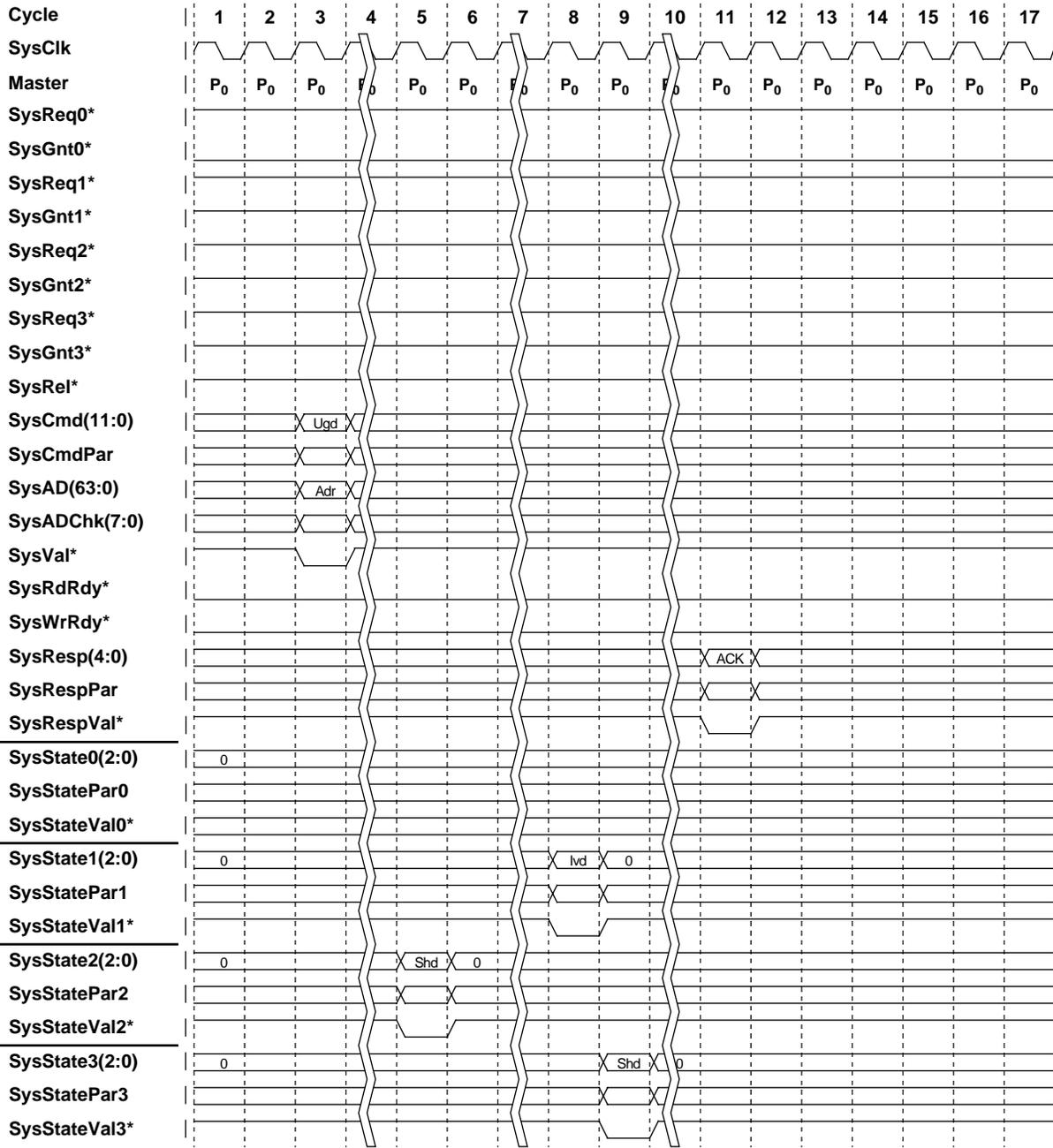
Figure 6-28 R10000 Multiprocessor Cluster Processor Upgrade Request Example
