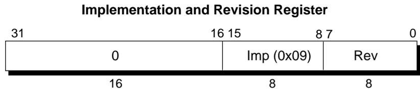
Figure 12-6 *FP Implementation and Revision Register Format*
