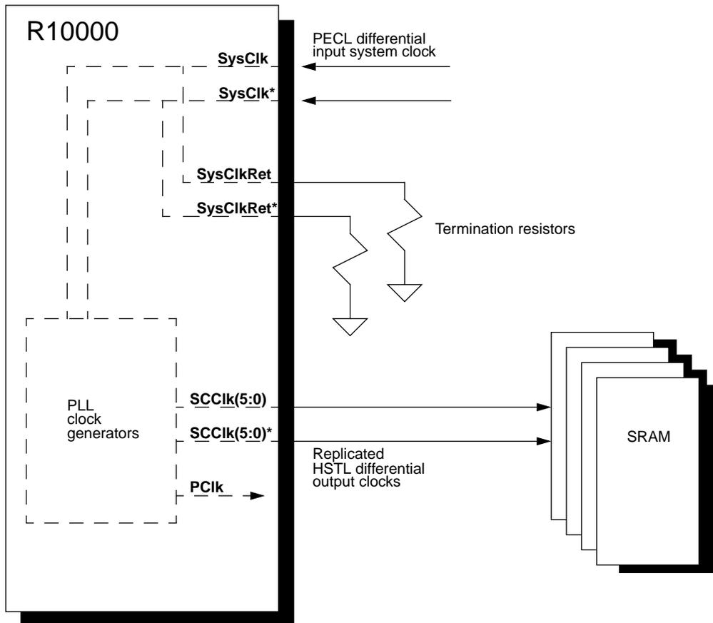
Figure 7-1 R10000 System and Secondary Cache Clock Interface
