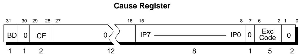
Figure 11-13 Cause Register Format
