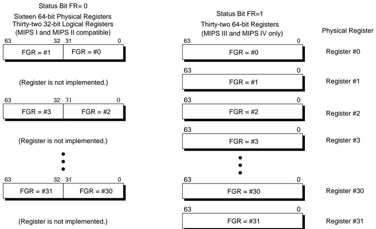
Figure 12-2 Floating-Point Registers
