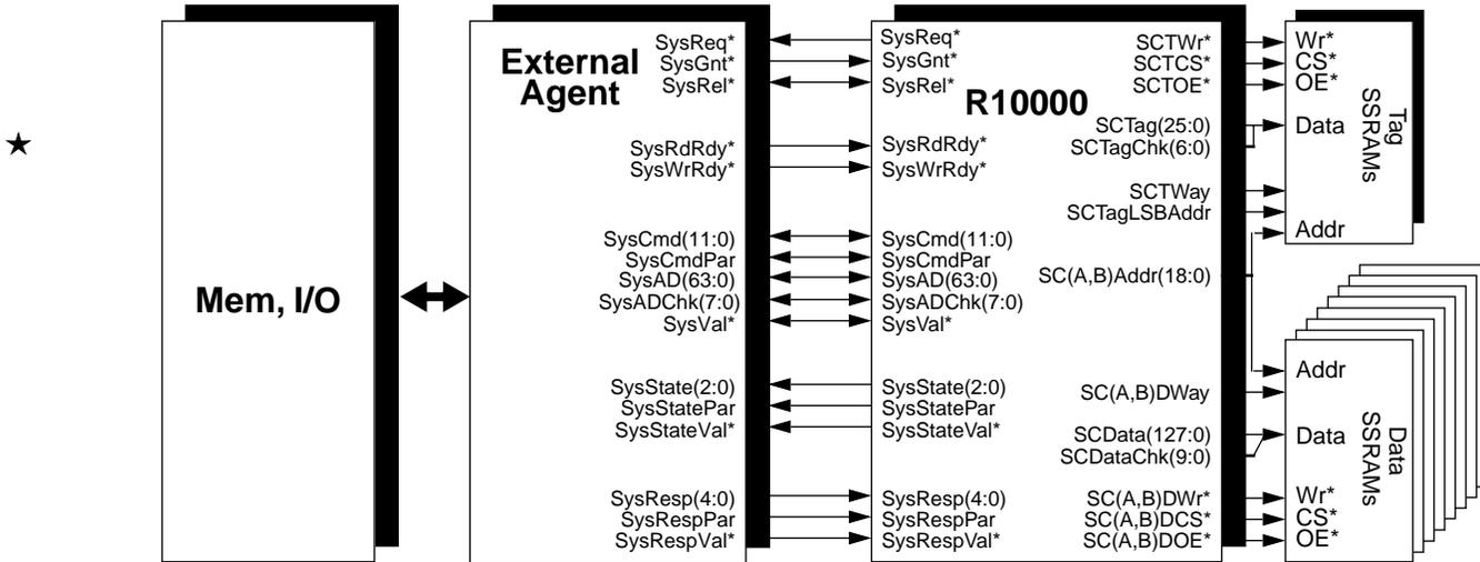
Figure 6-2 System Interface Connections for Uniprocessor System
