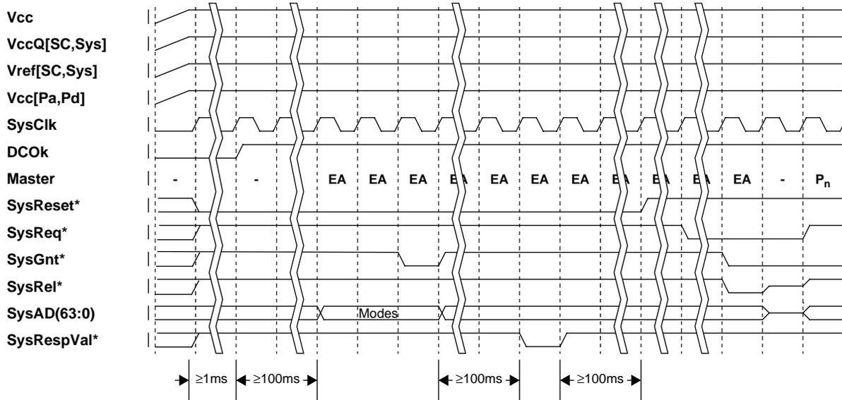
Figure 8-1 Power-On Reset Sequence
