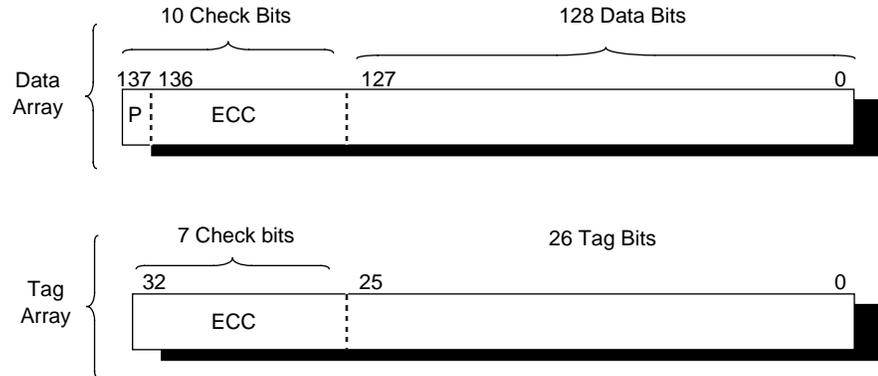
Figure 5-1 Secondary Cache Data and Tag Array
